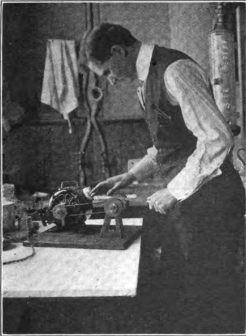
SHARPENING CUTLERY AND POLISHING METALWARE ARE TWO OF THE TASKS EFFICIENTLY PERFORMED BY A SMALL MOTOR
