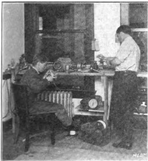
A TYPICAL SCENE IN AN ELECTRICIAN'S SHOP—WINDING MOTOR ARMATURES BY HAND
