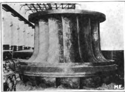
ROTATING MEMBER OF ONE OF THE WATER TURBINES
