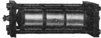
FIG. 4.—THE NEW COMPRESSED AIR SPARK GAP
