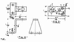
care must be taken in the making of this part, and twice out of every three times it will be necessary to make it over again, for the reason that silicon differs, one piece not being as sensitive as another in the detection of the waves.
