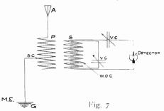
ing-out coil; S.C., sliding contact; V.C., variable condenser; A, aerial; G, ground.
