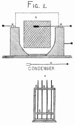
condenser made of 50 sheets of tinfoil with paraffined paper as insulation are required.
