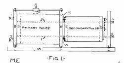
circle when drawn on B. Make a point 1 inch directly below the center of B and another the same distance directly above center. At these points bore a hole slightly less than 3/16 inch, through B and C, as shown by dotted lines. (Fig. 1.)
