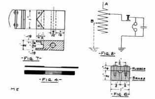
entire length of the cage, making 275 turns of wire all told; finish off by entering a hole in the bottom and connecting to the binding post on the standard.
