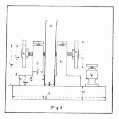
brass standards (b and c), hard rubber base (f), four binding posts (g), two discs of hard rubber (d and e), two battery terminal screws, two thumb screws from old binding posts (h and i), two brass springs (j and k), and two brass bolts (2).
