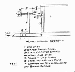
inches longer than "1" as shown on drawing. Mount coil on same 5/8 inch from one end. Next procure some 1/8 inch, or better, some 1/4 inch copper or brass, one inch wide, and about 5 1/2 inches long. About 1 inch from one end bend same over until a perfect right angle is formed. If the experimenter is handy, this part may be cast. This is the standard marked "7" on drawing. The brass thumbscrew "5" was taken from an old "Edison" primary battery, but
