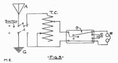
the set screw, and then moving the silicon around under the point until the signals are heard loudest. More or less pressure should be given on the point, according to the sensitiveness of the particular piece of sili-
