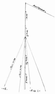
wires (Fig. No. 1), but if it is to be raised 80 or 100 feet, it will of course need two sets, one near the top, the other approximately half way down (Fig. No. 2).
