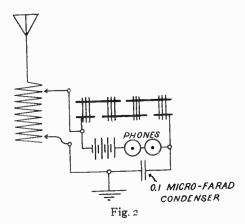
The two tuning coils are of course variable and have an inductance equal to that formed by about 350 feet of No. 16 copper wire when wound closely together.
