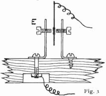
The connections are shown in Fig. 1, the wires leading from the magnets are connected to the binding posts FF, the standard holding the armature and the upright holding the set screw E (Fig. 3), are connected to the binding posts EE.
