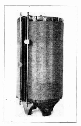
position so that the sliders move freely up and down the coil bearing on the rubber, and the springs bearing on the contact strip and passing each other without touching, and then screw the brass plates into the
