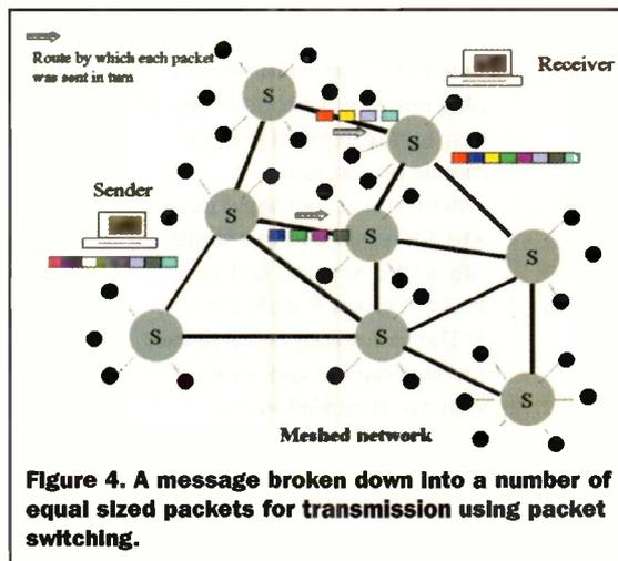
**Figure 4. A message broken down into a number of equal sized packets for transmission using packet switching.**
