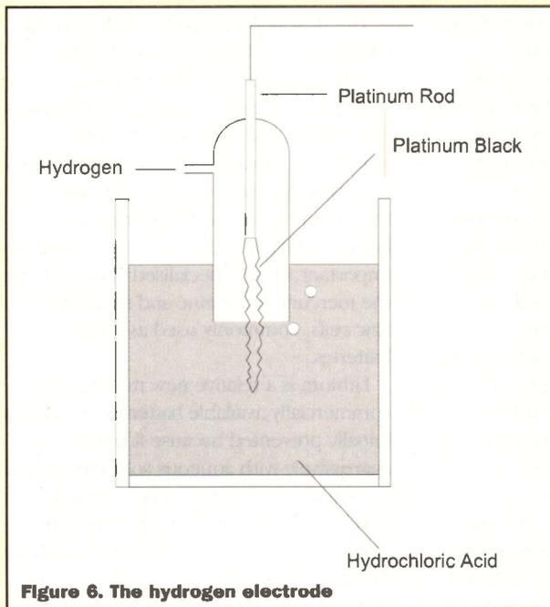
Figure 6. The hydrogen electrode
