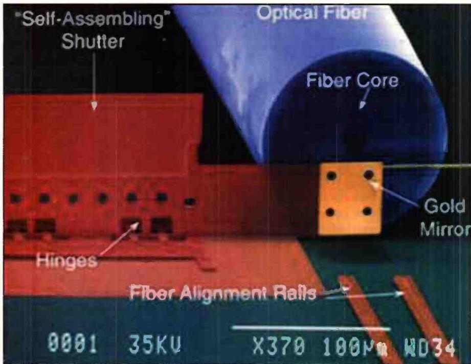
**Example of first practical micro electro mechanical optical switch. When the bar is lowered (as shown) the signal on the left is deflected to the rear fibre. When raised the signal path continues to the fibre on the right without interaction.**
