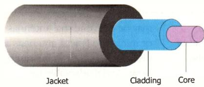
**Figure 5a. An optical fibre guiding light by total internal reflection in section (a) and plan (b).**
