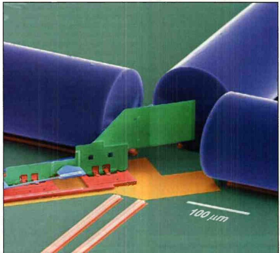
**Further example of microelectro mechanical optical switch**
