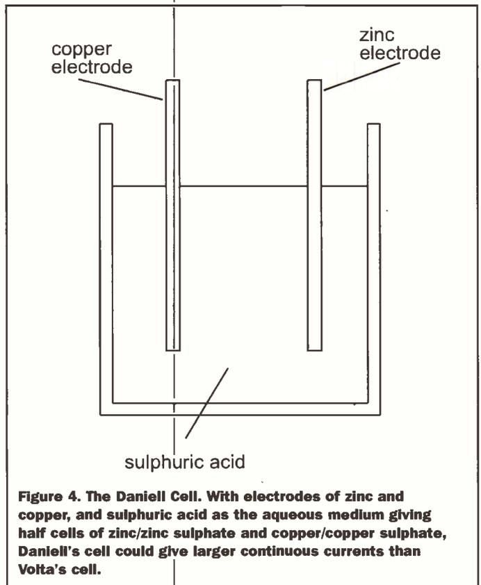
Figure 4. The Daniell Cell. With electrodes of zinc and copper, and sulphuric acid as the aqueous medium giving half cells of zinc/zinc sulphate and copper/copper sulphate, Daniell's cell could give larger continuous currents than Volta's cell.
