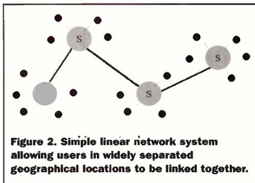
**Figure 2. Simple linear network system allowing users in widely separated geographical locations to be linked together.**
