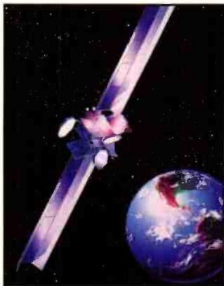
The most powerful communications satellite built to date, 17.5kW Anik F1 satellite built for Telesat Canada, was launched on an Ariane rocket from the Guiana Space Centre in French Guiana in mid-November.
