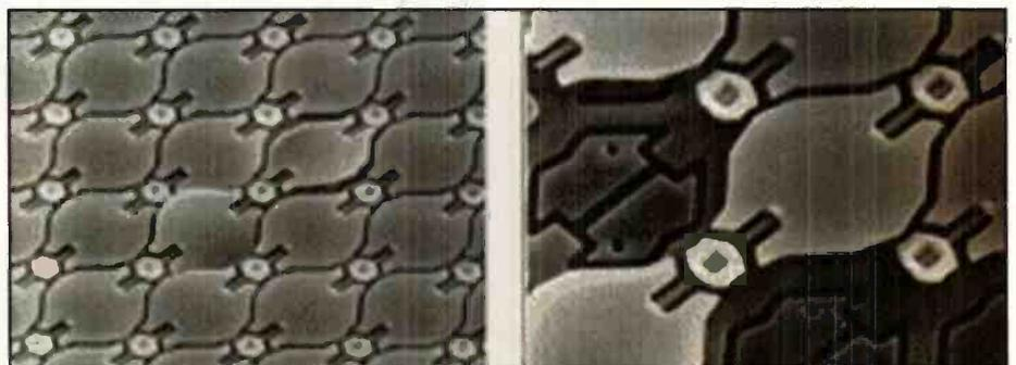
**Complex MEMS system of array of independently actuated mirrors to control colour on a display module.** Courtesy Texas Instruments
