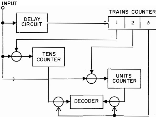
Figure 16—Register circuit.
