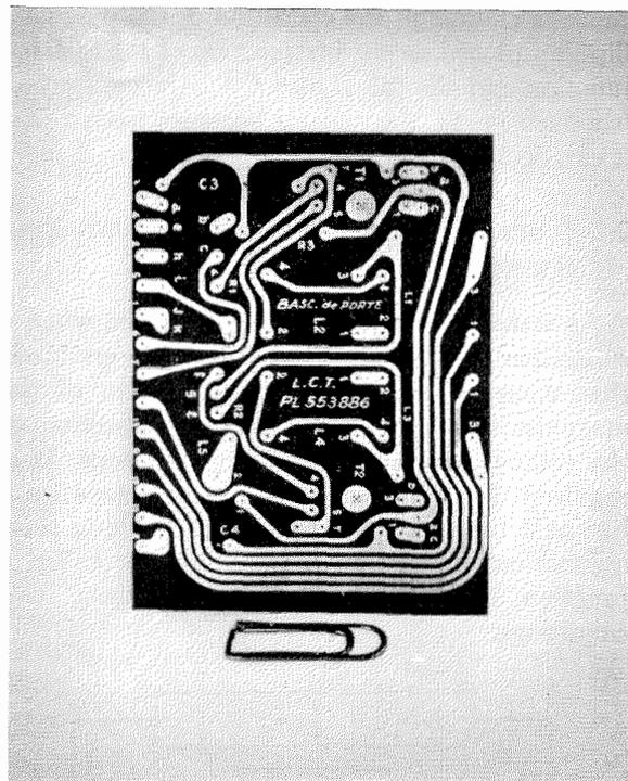
Figure 12—Rear of flip-flop panel.
