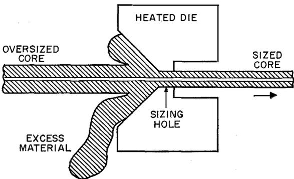
hole is maintained at a substantially uniform temperature along its length. This sizing hole is of uniform diameter and normally smaller than the diameter of the cylindrical plastic form. At the entrance to the sizing hole, there is provided a conical opening that assimilates the body fluid
