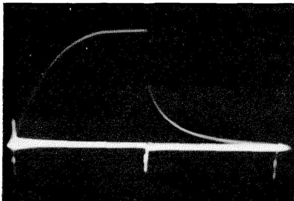
Figure 1—Distortion in scanner output pulse caused by the shunt capacitance of the gates.
