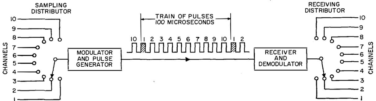
Figure 7—Principle of a time-division multiplex system.
