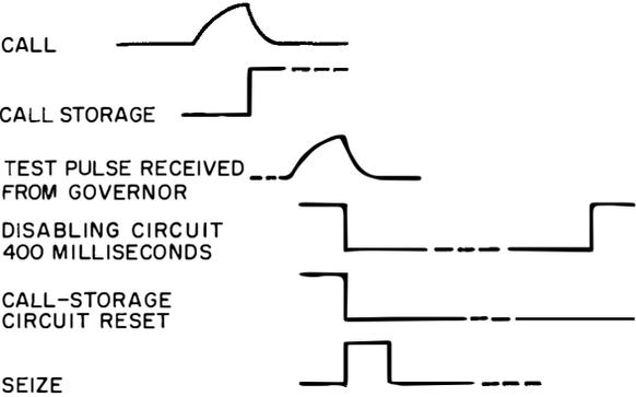
Figure 14—Series of waveforms during the engaging of an *A* governor by a call detector for the arrangement in Figure 13.
