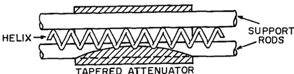
patent. The attenuator consists of a concentrated body of resistive material shaped so that only the central portion of this mass is in contact with the conductors of the helical line. Thus a high degree of attenuation is concentrated over a small length of the helical line and because of the taper an impedance match is also achieved.
