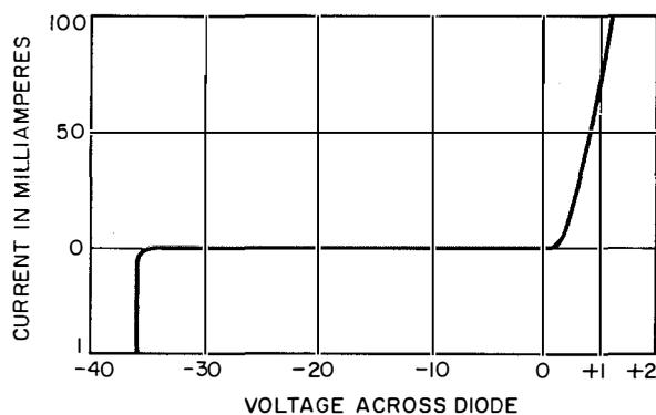
Figure 1—Current-voltage characteristic of silicon junction diode designed for telephone switching. Note change of scale for reverse current and voltage.
