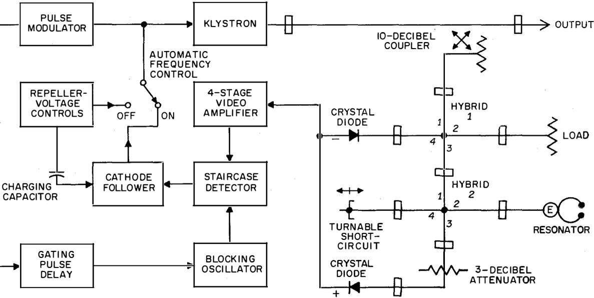
Figure 1—Block diagram of automatic-frequency-control system.
