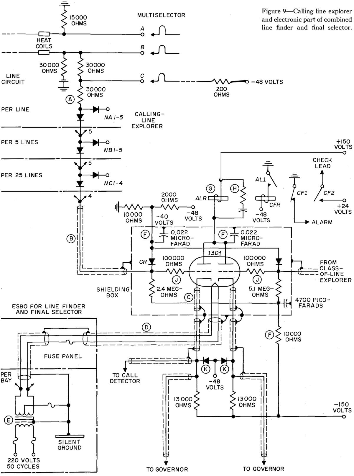
Figure 9—Calling line explorer and electronic part of combined line finder and final selector.
