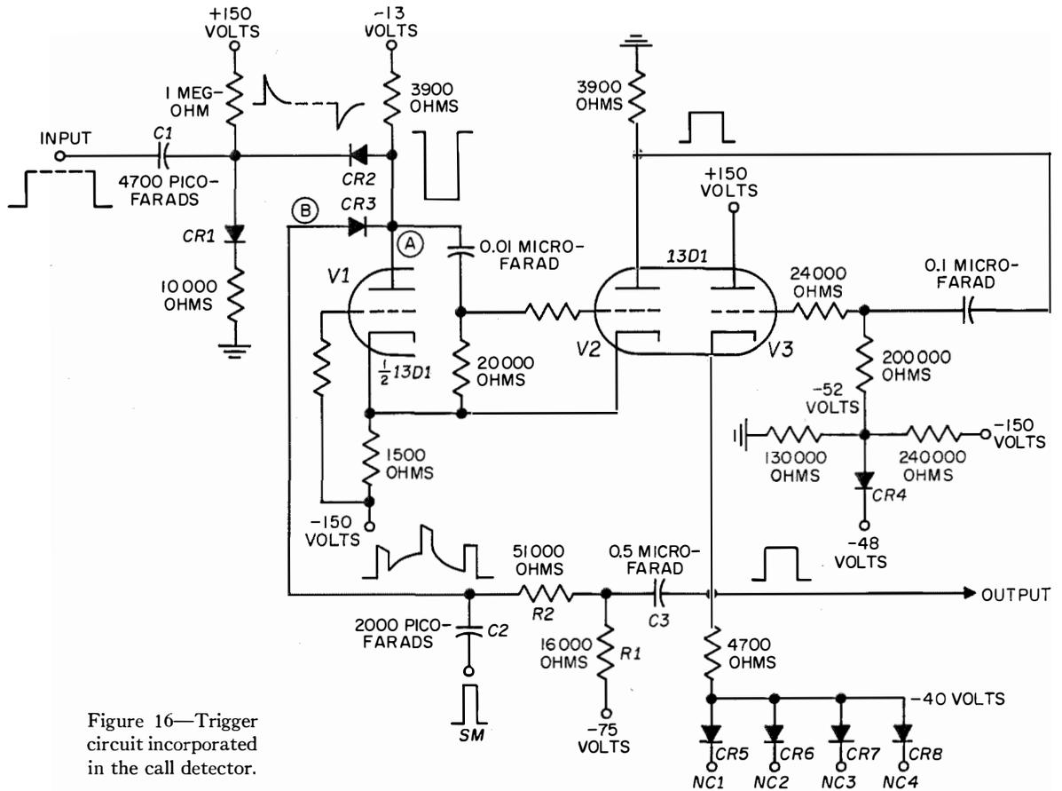
Figure 16—Trigger circuit incorporated in the call detector.
