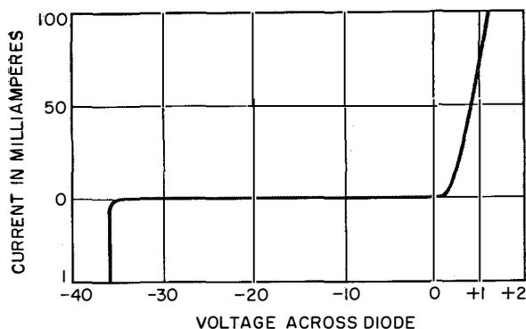
Figure 5—Typical characteristic of a silicon  $p-n$  junction diode by Laboratoire Central de Télécommunications.
