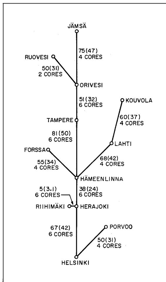
Figure 1—Route diagram of the Helsinki-Tampere coaxial-cable system. Repeater stations are spaced approximately 10 kilometers (6.2 miles) apart. The numbers indicate distances between the adjacent places in kilometer (miles) and the number of coaxial cores is also noted.
