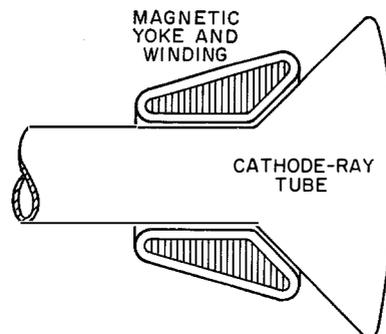
the deflection windings are flared so that they will extend not only along the neck of the tube but an appreciable distance over the flared portion of the tube as well.
