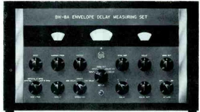
Fig. 4 - RCA Type BW-8A envelope delay measuring set.
