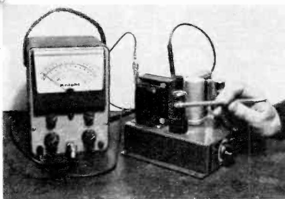
leave the meter's common lead clipped where it is, switch to the 15-volt scale, and touch the free probe to terminal 7 of tube C, 2 of B, 7 of A and 2 of E. Identical readings of 12 to 13 volts are obtained at all these points.
