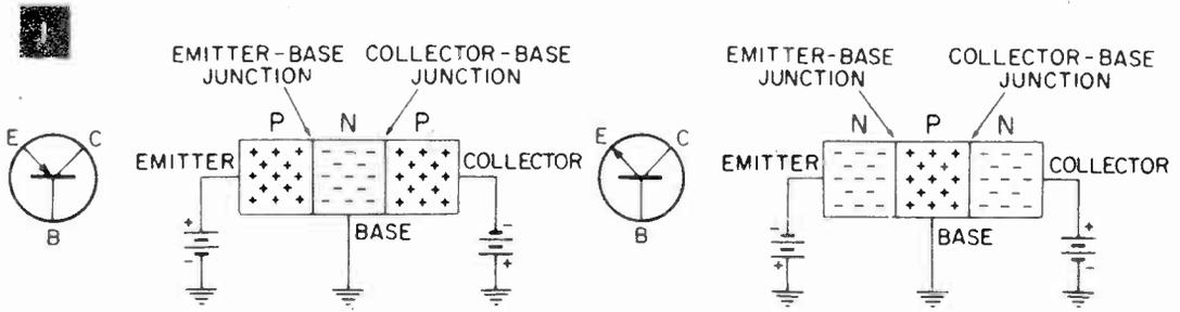
If new batteries don't solve transistor-radio trouble, remove transistors and check them on a tester, such as the new Paco T-65. Tweezers are handy for removing them from tight space and getting leads into the tester sockets. Figure 1, immediately above, shows construction of PNP and NPN transistors.
