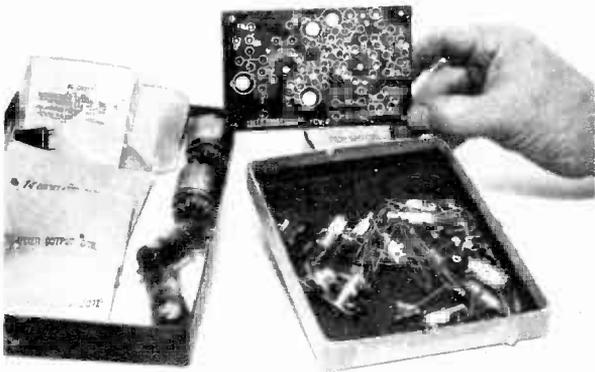
The FCV-2 converter is seen above receiver at left without its shield can, which is simply an aluminum box. The printed-circuit board directly above is part of the kit and makes construction simple. Numbers on board serve to identify parts.
