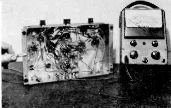
Metal chassis is usually common "ground" and "B" negative side of circuit. Measuring DC voltage, clip VTVM's "common" terminal to chassis, touch "hot" spots with the positive probe of your meter.
