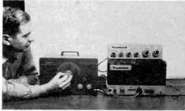
For checking overall frequency response, use an audio generator
