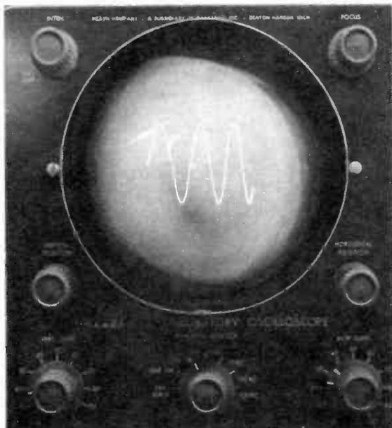
Number of AC cycles produced on C. R. tube is ratio of input signal frequency to sweep frequency. Here the input is 60 cps but sweep has been reduced to 30, for two "sine wave" shapes.
