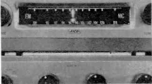
Completed tuner, used with an Eico HF-12 amplifier. It is not tuned to station accurately. The exclamation-point-shaped plate of DM-70 glows brightly overall, meaning no signal or weak one.
