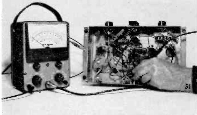
Warning! Never grasp the DC probe of the meter near its exposed end as shown here. It is a fine way to get a bad shock from high-voltage point of equipment you are troubleshooting.
