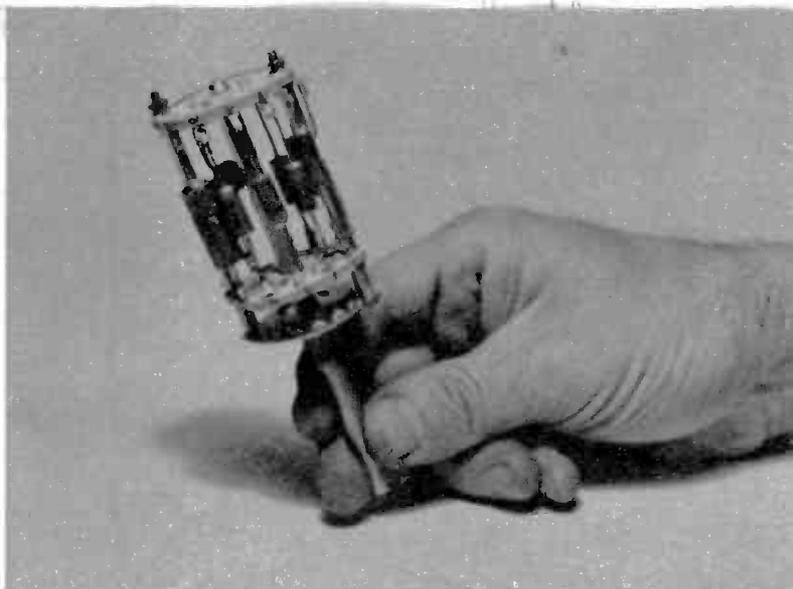
Construction of the AG-10 from a kit is interesting and instructive. All members of the chassis are preformed and punched so that assembly of the instrument is rather simple.
