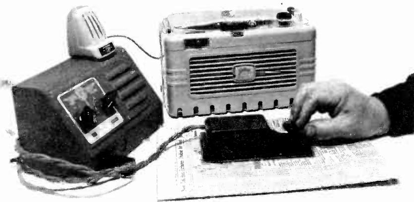
Simple setup for taping code practice is above. Mike of the recorder picks up signals from the oscillator's speaker. Playback is demonstrated at the right. If you can copy your own sending, you have the makings of a good radio operator.
