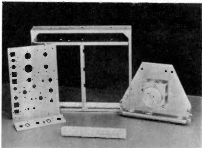
Chassis members include main tuning capacitor support and drive, completely punched main chassis and subchassis plates, expanded scale drum that turns with the bandswitch.
