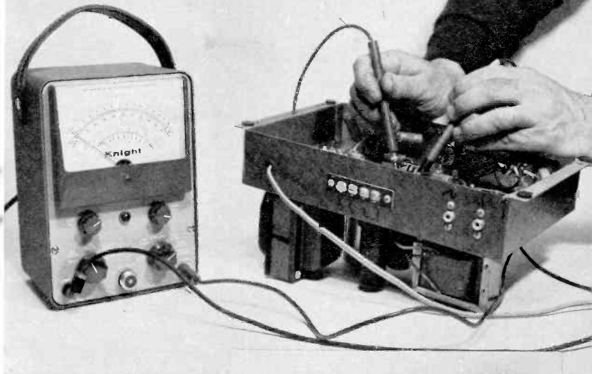
For checking AC voltages and making resistance measurements, it is usually convenient to use two long-handled probes with the VTVM (vacuum tube voltmeter) as demonstrated above.
