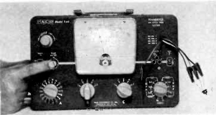
Four switches along bottom of the tester are set according to transistor type. "Read Meter" button is then pressed. The transistor checked at the left is a good one. Terminal arrangements of four popular styles of transistors are in Fig. 4, below.
