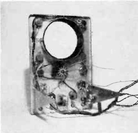
To front panel (left) have been added brackets to support main chassis, preformed wiring harness, and a few small resistors and capacitors.
