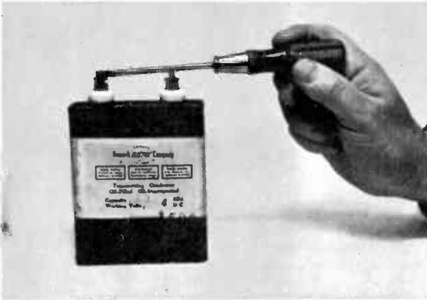
Avoid shock danger; discharge filter capacitors.
