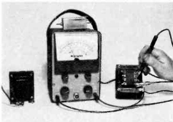
Suspected "shorts" can be cleared or verified by tapping with equipment on. Rectifier tube is the suspected one here; meter checks output voltage.
