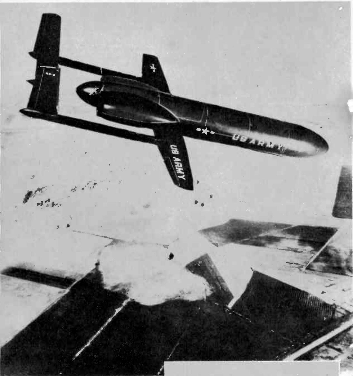
Combat commanders will "see" many miles with radio-controlled drone planes, such as fighter-size, experimental, classified version of artist's rendition above. Drone at right is moved on carriage behind jeep. Pneumatic prop spinner starts its engine, and it climbs in jet-assisted take-off to circle vastness of Electronic Proving Ground in Arizona at relatively low speed, under the control of a radio director on the ground.
