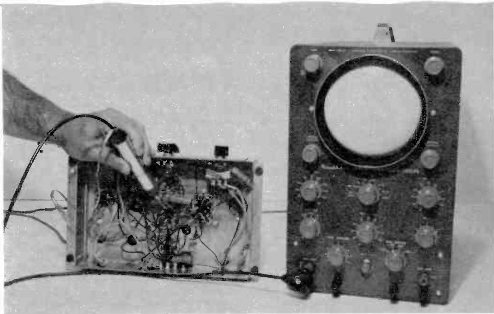
Signal or circuit position to be checked is connected to the vertical input posts of the oscilloscope through various probes that are similar in appearance to those employed with voltmeters.
