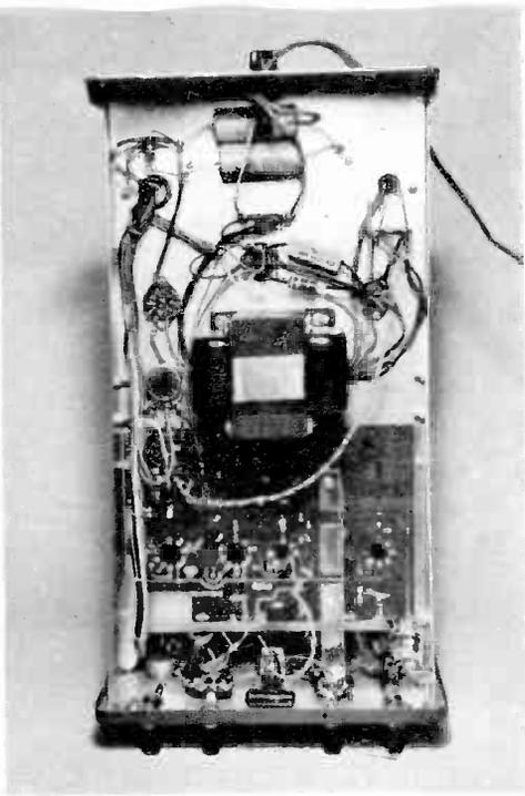
The O-11 oscilloscope stands upright on its front panel, photograph at the left, to show neat appearance of chassis' underside. Placing of the scope's ten tubes is all that remains to be done.
