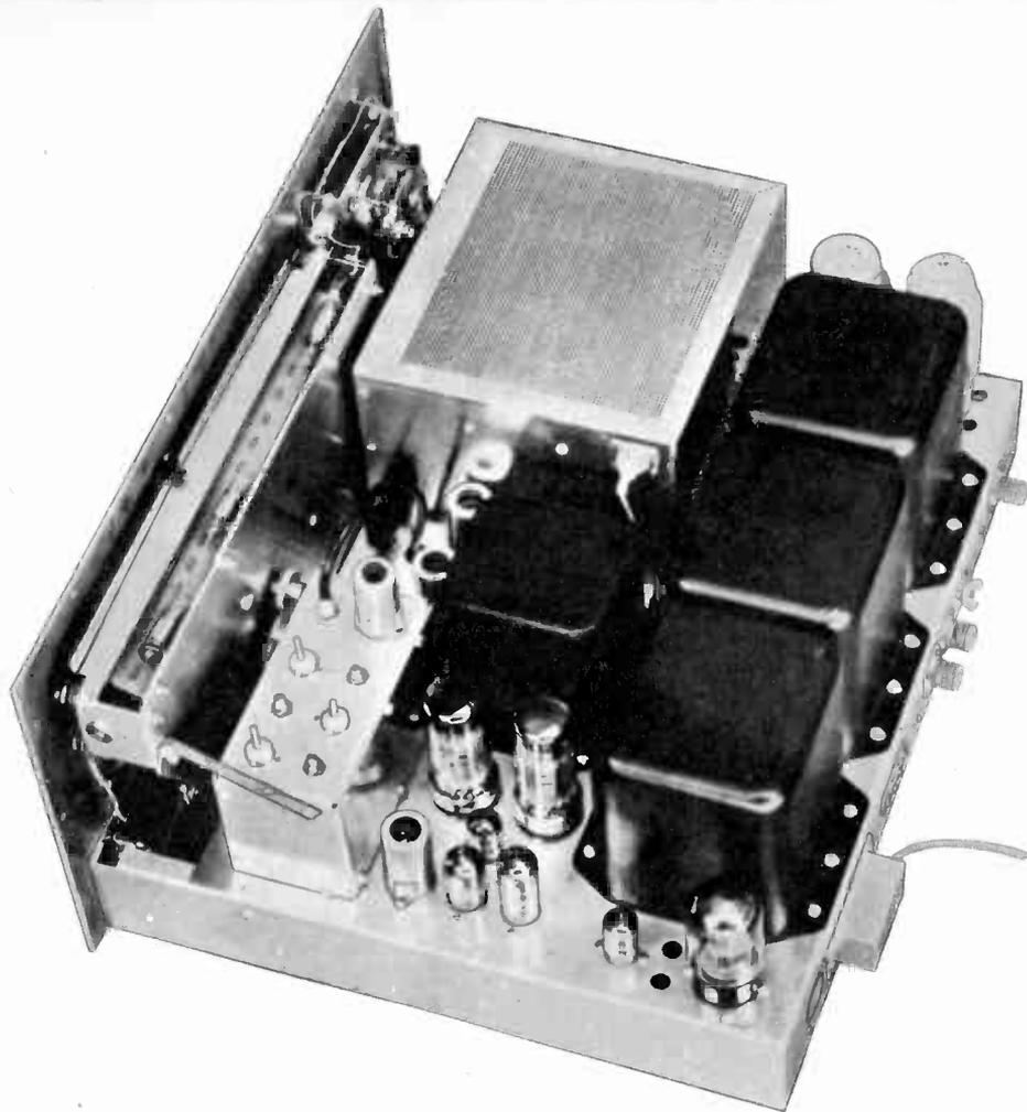
Rugged construction of the Apache is evident above. Note cage at the top of photograph. It serves to protect the final amplifier stage.
