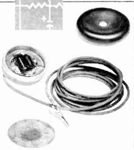
An entire receiver in an earphone! Coil, diode, capacitor of Fig. 2 fit in case. Wire with clip on end is for antenna connection.
