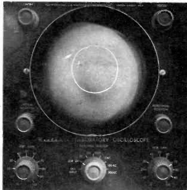
With ordinary AC signals of same frequency on horizontal and vertical deflection systems, pattern depends on "phase." A perfect circle results when they are 90 or 270° out of phase.
