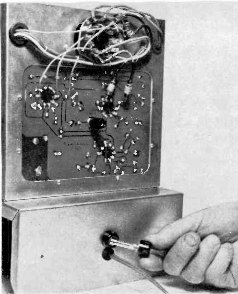
Wiring is complete and large socket is in place over base of C. R. tube. Important step is the insertion of line fuse. Electronic equipment often fails merely because this little detail has been overlooked.
