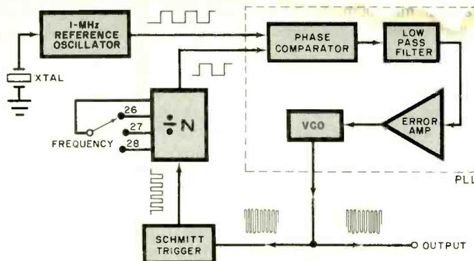
Fig. 1. A basic digital frequency synthesizer. Many frequencies can be generated using one reference crystal.
