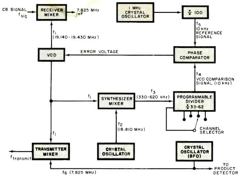
Fig. 2. A digital (PLL) synthesizer for AM/SSB use.
