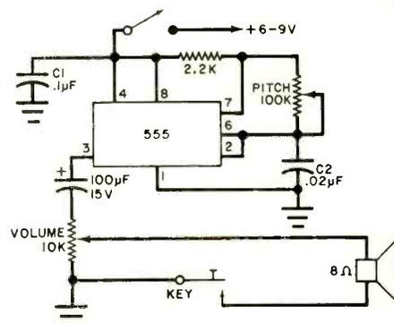
Fig. 2. Code practice oscillator. Capacitors are 25-V disc ceramics, resistor is 1/2-W carbon. 555 IC is Signetics or equiv.
