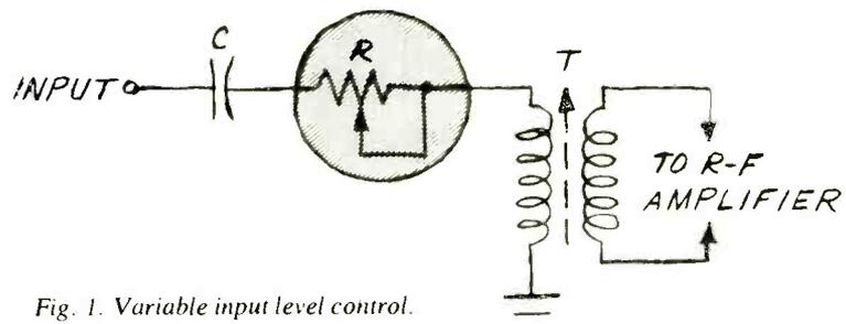
Fig. 1. Variable input level control.
