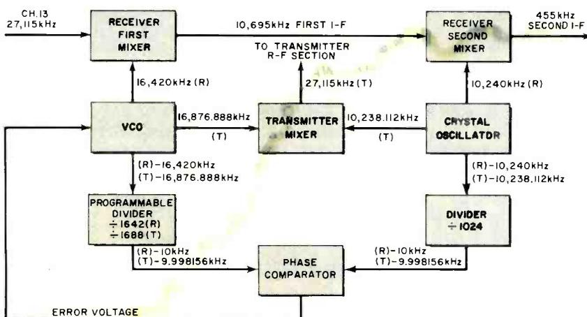
Fig. 3. Digital synthesizer for AM with dual conversion on receive.
