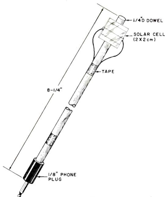
Fig. 4. Construction of final section of detector arm, which is folded to permit door closing.
