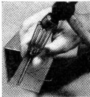
"Stake" the edges of the screw hole with a broad-bladed screwdriver or small dull chisel. All it takes is a few light taps with a hammer.
