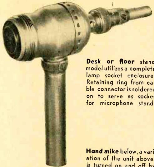
**Desk or floor stand model** utilizes a complete lamp socket enclosure. Retaining ring from cable connector is soldered on to serve as socket for microphone stand.
