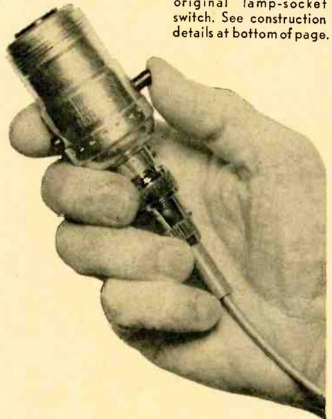
**Hand mike** below, a variation of the unit above, is turned on and off by original lamp-socket switch. See construction details at bottom of page.
