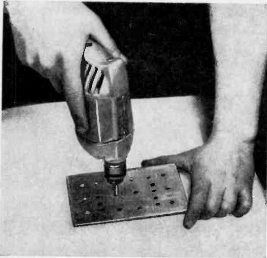
**Template** for making the fixed plate of the tweeter. Use a  $\frac{1}{4}$ " bit to drill the  $\frac{1}{8}$ " steel plate. Two holes must be countersunk for heads of bolts to fit flush.
