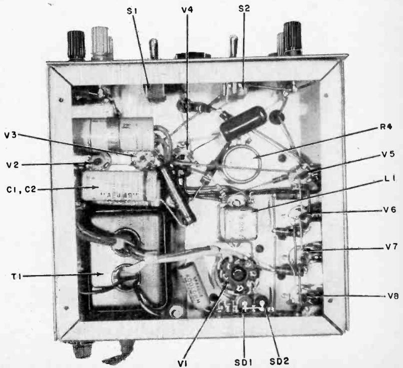
stock carbon resistors if an accurate means of resistance measurement is available, or they could be wound of resistance wire. Since the exact ohms-per-foot value of resistance wire is always specified, very accurate resistances can be determined by careful measurement of the length of the wire.
