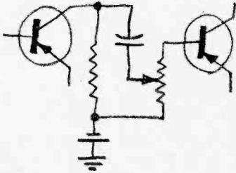
“If you run into volume control problems such as distortion at low volume, abrupt changes in volume as you move the control, or just excessive noise from the control, check to make sure that you’re not goofing up the bias in some way and that there isn’t too much current flowing through the control.”
