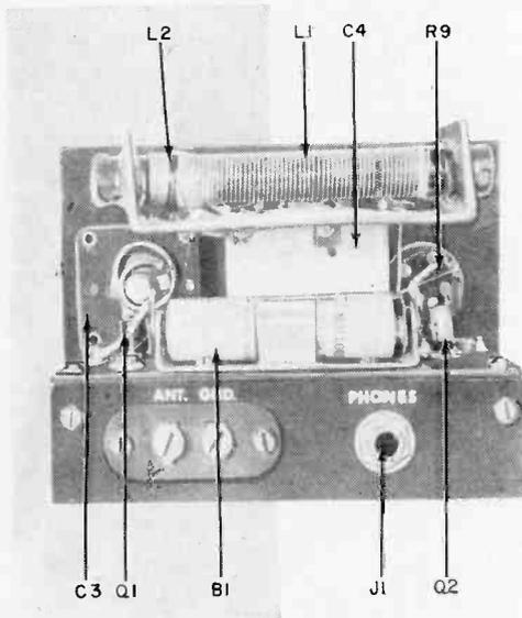
to and as far as possible from L1. Place L3 so that you will have easy access to its adjustment screw. Other than this, parts layout is not critical.
