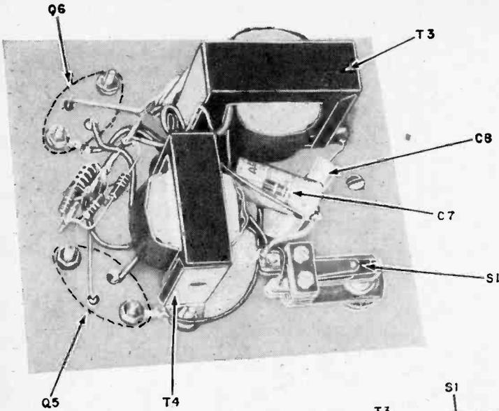
**Top panel**, at left, is the mounting base for the two power transistors and the transformers of the "talk-back" section. Assembled unit, below, shows relative placement of panels. "Listen" amplifier is mounted on panel opposite rear of horn.
