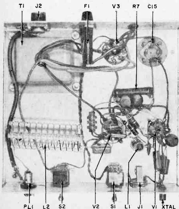
**Pictorial diagram** above details the connections to tube sockets V1 and V2. The leads need not be as long as this but should connect to points indicated.
