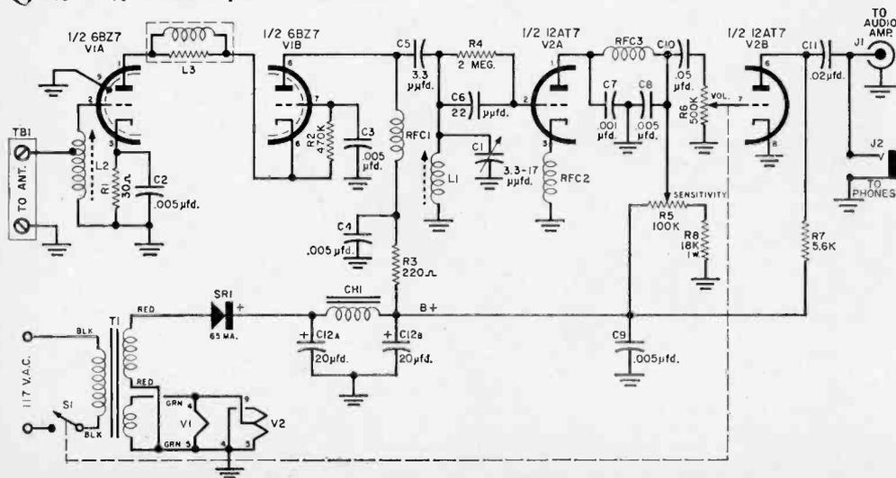
noise in the phones will drop to a level dependent on the strength of the received carrier. A fairly strong signal will cause the hiss to drop out completely. As you tune past the signal, or if it leaves the air, the hiss will return. The sensitivity control shown on the front panel is not critical in its setting; it can be adjusted once for best
