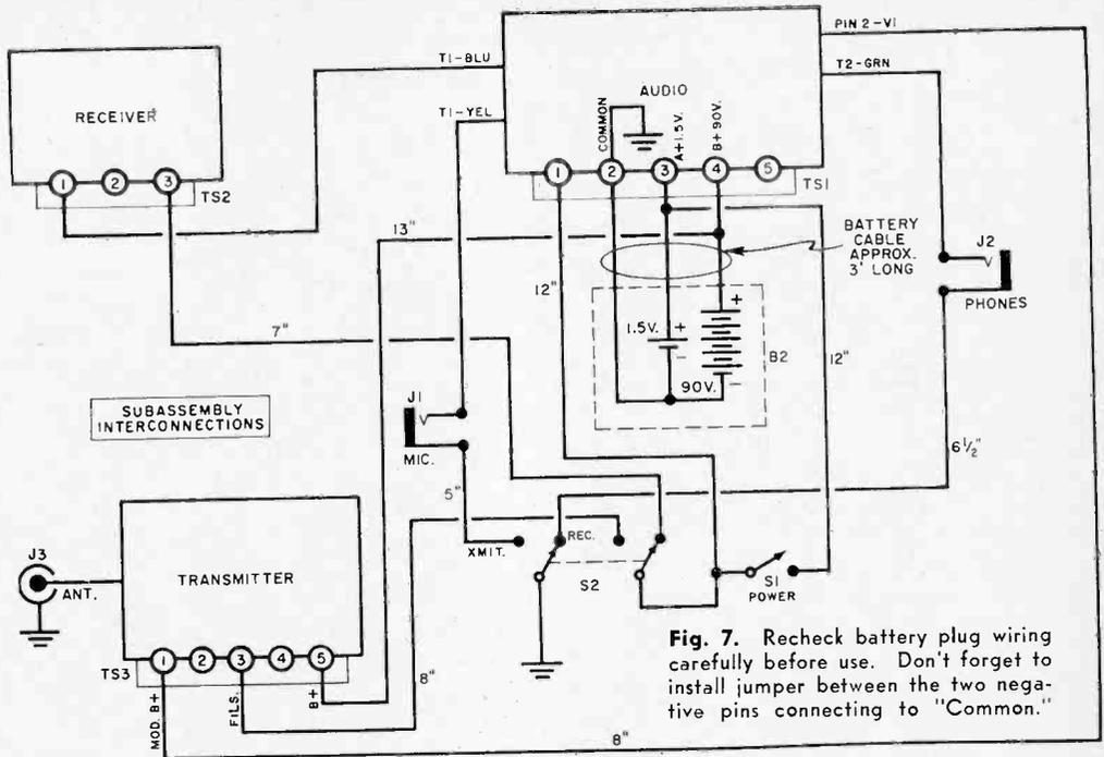
Fig. 7. Recheck battery plug wiring carefully before use. Don't forget to install jumper between the two negative pins connecting to "Common."
