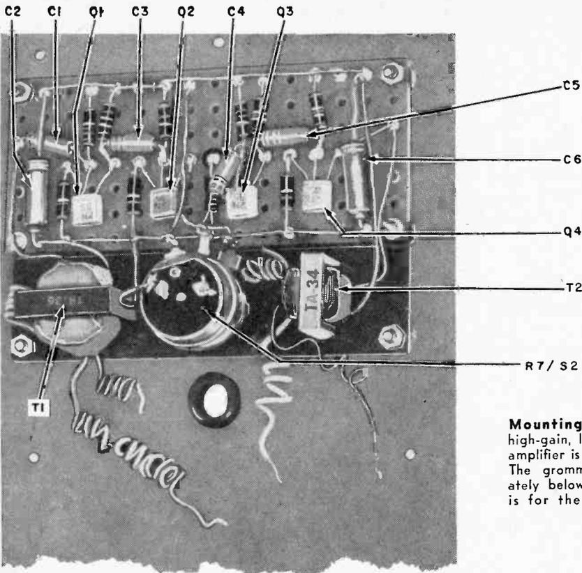
**Mounting plate** of the high-gain, low-power "listen" amplifier is box's back panel. The grommet hole immediately below gain control R7 is for the handset cable.
