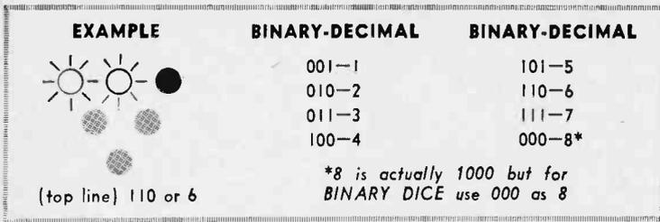
**How to convert binary numbers to the decimal system.** Only the top line of bulbs is read, giving eight possible "on-off" combinations.
