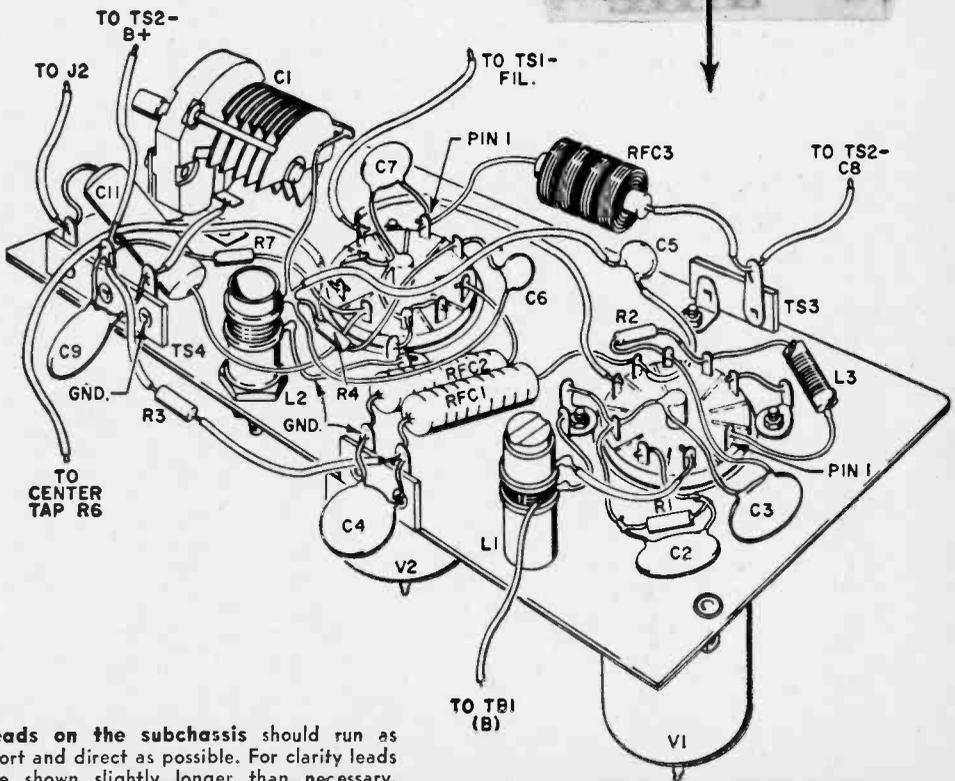
Leads on the subchassis should run as short and direct as possible. For clarity leads are shown slightly longer than necessary.
