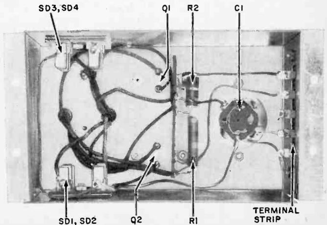
**Parts arrangement** beneath the chassis is non-critical. Holders for the silicon rectifiers may be fuse clips or special diode clips. Make sure that all components are properly insulated and polarized.
