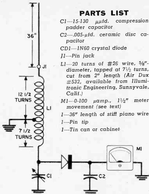
*C1*. Connect the banded end of *CD1* to the plus terminal of *M1*. Then connect the .005- $\mu$ fd. capacitor (*C2*) across the meter terminals, and wire last connections.
