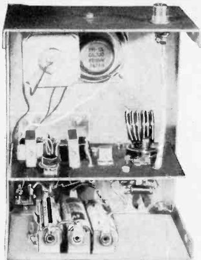
the cabinet. A  $\frac{1}{4}$ "-o.d. and  $\frac{3}{16}$ "-i.d. sleeve will be needed to couple the dial to the shaft of *C1*. Once the vernier dial is properly aligned with *C1*, drill the holes and mount.
