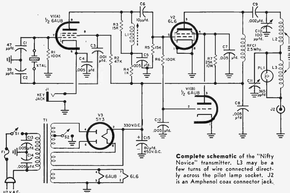
**Complete schematic** of the "Nifty Novice" transmitter. *L3* may be a few turns of wire connected directly across the pilot lamp socket. *J2* is an Amphenol coax connector jack.
