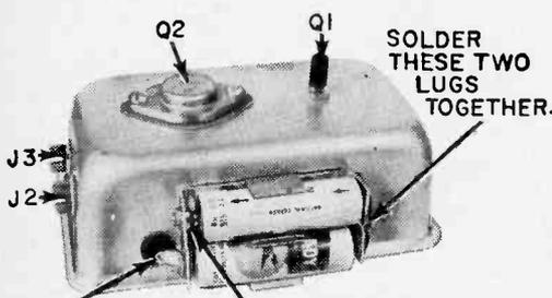
**4** Rear view of completed chassis. Insulated phone tip jacks are used for J2 and J3. The battery holder terminals are connected so the two cells are in series with the positive end grounded.
