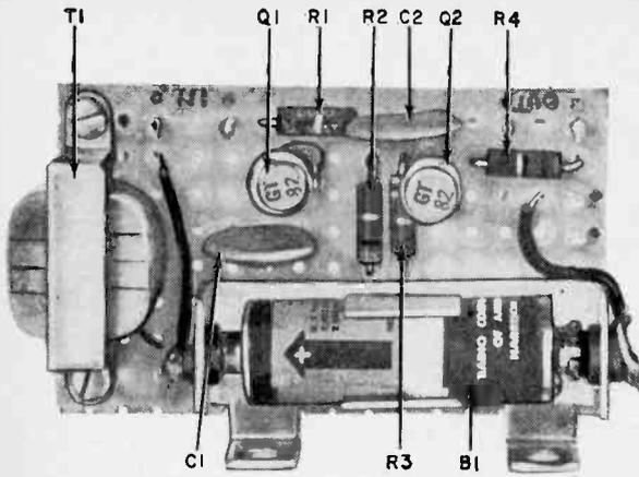
**Front and back views** of transistor amplifier board. The small brackets are used to mount it to the side of the cabinet. Parts placement is not critical but should follow a logical order from input to output. Certain microphones may not require transformer T1 for proper match to the input impedance of transistor Q1.
