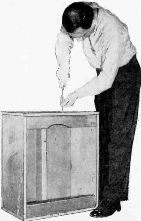
**3** After back panel is glued and nailed in place, 2" x 4" cross-braces are installed. Wood screws and glue are used to tighten rear panel to the 2" x 4" rear brace and to secure cross-braces. Cracks should be calked with wood putty to prevent air leaks.
