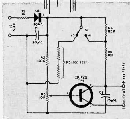
This circuit can be constructed on any type of chassis. Built-in current limiting factor prevents transistor burn out. *C1* is a 150-volt unit; *C2*, 25 volts.
