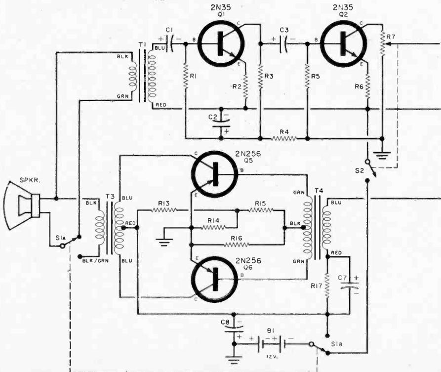
compact, the unit presented here combines a ten-watt power trumpet with a second high-gain amplifier that can convert the sound of an approaching automobile into that of a roaring avalanche. It's completely transistorized and, except for the flaring horn and the telephone handset, is contained complete with batteries in a 5" x 6" x 7" aluminum cabinet.
