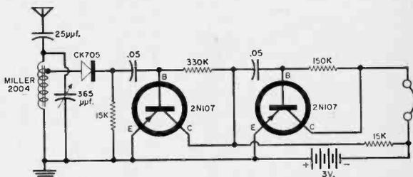
Two Transistor Special Radio
