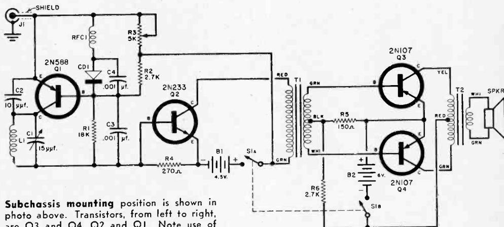
**Subchassis mounting** position is shown in photo above. Transistors, from left to right, are *Q3* and *Q4*, *Q2* and *Q1*. Note use of two battery supplies for increased stability.
