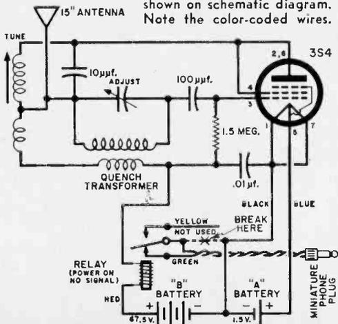
The construction details given here for the R/C train are intended as a guide—your exact setup will depend on the components you use. There are many other possible installation techniques. The locomotive modification shown above permits normal operation when the miniature phone plug is removed.
