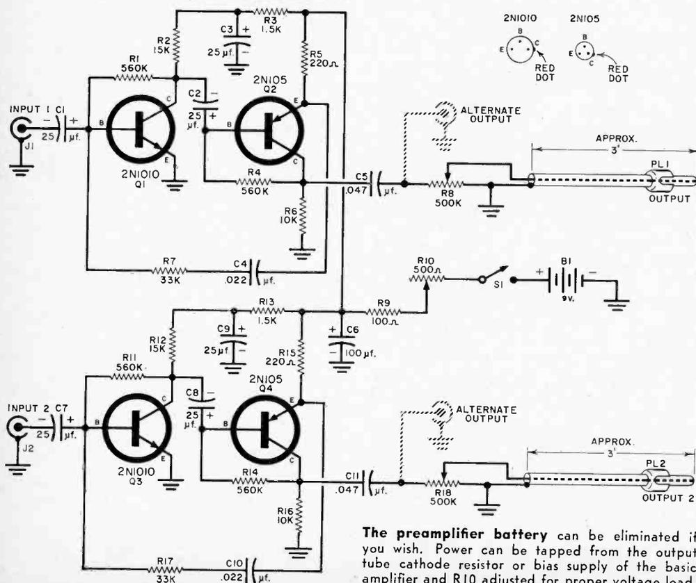
The preamplifier battery can be eliminated if you wish. Power can be tapped from the output tube cathode resistor or bias supply of the basic amplifier and *R10* adjusted for proper voltage load.
