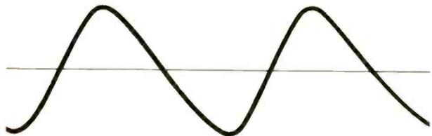
**WAVEFORM WITH VTA-ERROR DISTORTION**
