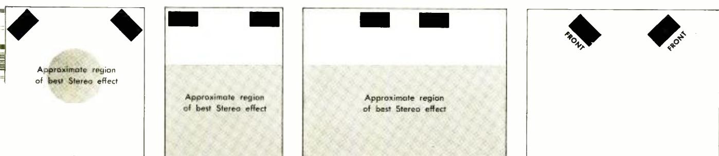
*Various arrangements of speakers for stereo listening, differing with types of rooms. The setup at the far left is no longer much used.*
