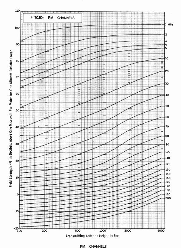
ESTIMATED FIELD STRENGTH EXCEEDED AT 50 PERCENT OF THE POTENTIAL RECEIVER LOCATIONS FOR AT LEAST 50 PERCENT OF THE TIME AT A RECEIVING ANTENNA HEIGHT OF 30 FEET
