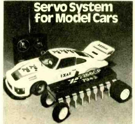
A complete receiver and servo controller on one chip, EXAR's XR-2266 can receive and act on all commands necessary to control every function of this radio-operated model car, even to turning on the directional signals and back up lights. It may be the heart of next year's Christmas best-sellers.
