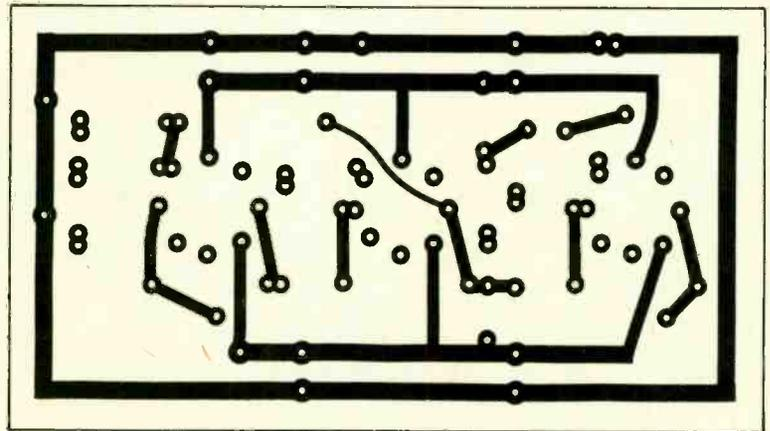
This is the exact scale template for etching the filter board. Leave at least 1/4-inch around all four sides to allow for the drilling of mounting holes with which to secure the circuit board to the chassis. Use a number 67 drill bit for making the holes.
