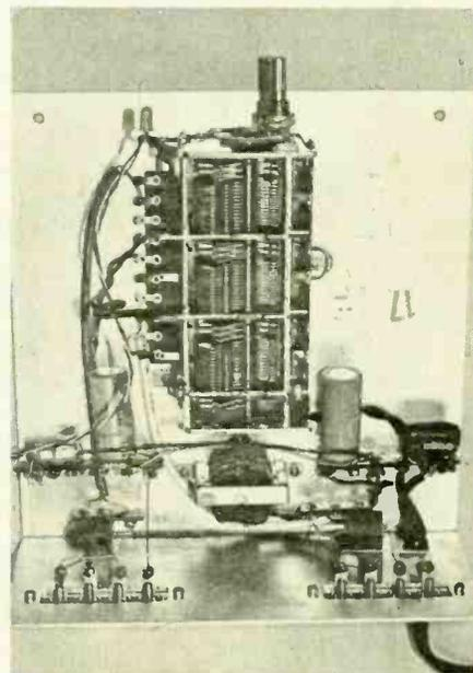
This interior view shows the massive triple-ganged tuning capacitor. Amplifier circuitry is at lower left, power supply at right. Circle 79 on reader service coupon.
