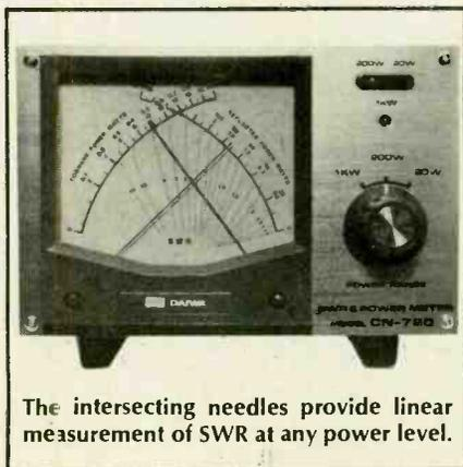
The intersecting needles provide linear measurement of SWR at any power level.
