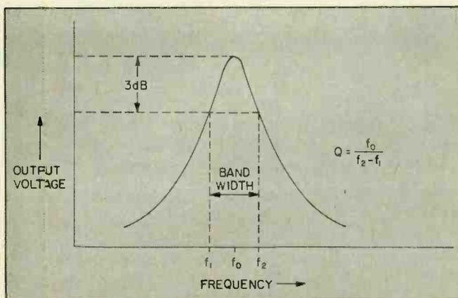
Fig. 1. Above is a sample graph depicting the bandpass curve for a theoretical filter derived from the formula at the left of the graph. This formula demonstrates the manner in which "Q" derives.
