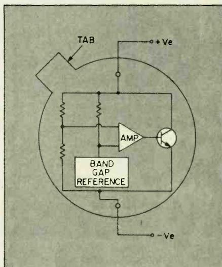
Here is an internal schematic of the band gap zener diode, which serves as the heart of the calibrator. Use the tab on the case as the reference point for making circuit connections. No heatsink is required here.
