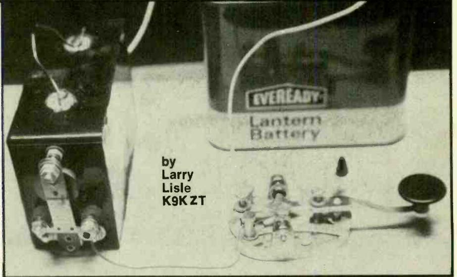
The contacts of the interrupter would then close as the magnetism of the core subsided and the cycle would repeat, usually 10 to 50 times per second.
