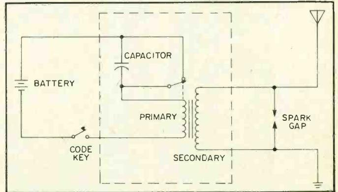
Fig. 2. Marconi's first transmitter, although remarkably similar to Hertz's, had the addition of a grounded spark gap and high antenna.
