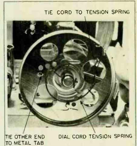
Fig. 5. Start the re-stringing by securing the cord to a tab or hole on the drum. End by securing the cord to the tension spring.
