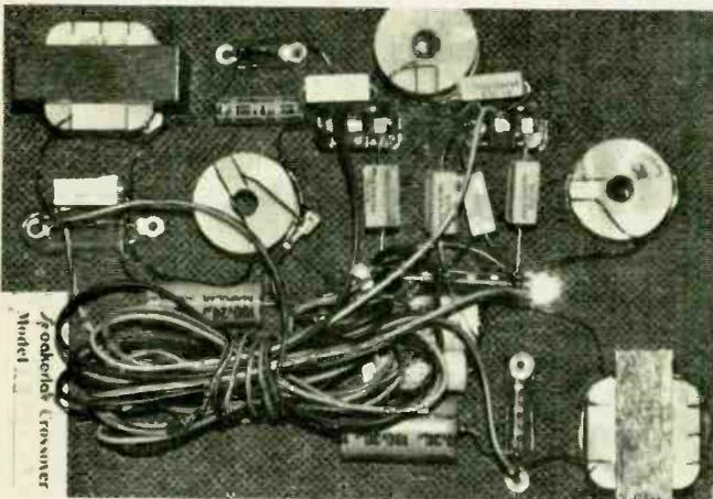
Next, glue the crossover network in place so that the control switches fit into the opening in the back panel. Untangle and separate the wires but don't pull any loose from the board. Be sure there are no air leaks around it.
