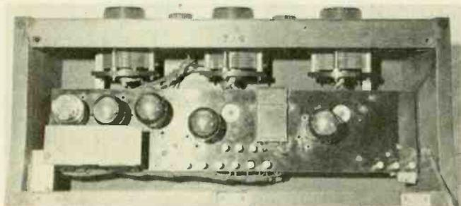
This interior view of the Federal shows the clean, rugged construction. The 3 small terminals at the lower right of the chassis are antenna and ground connection points.
