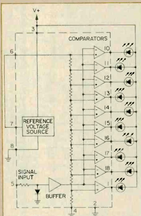
This is essentially a flow diagram of the LM 3914, with the LED output indicators in position (for reference). See the text for a more detailed explanation of the workings of the chip and the circuit as a whole.
