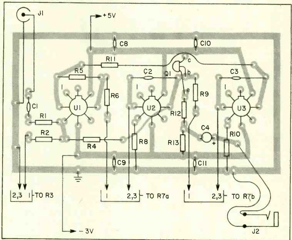
Here is the component layout diagram for the filter printed circuit board. Note the marked, off-board connections for R7a&b, R3, J1, J2 and V+. Make certain to match up the R7 connections exactly as shown on the schematic, or your filter will work only in reverse.
