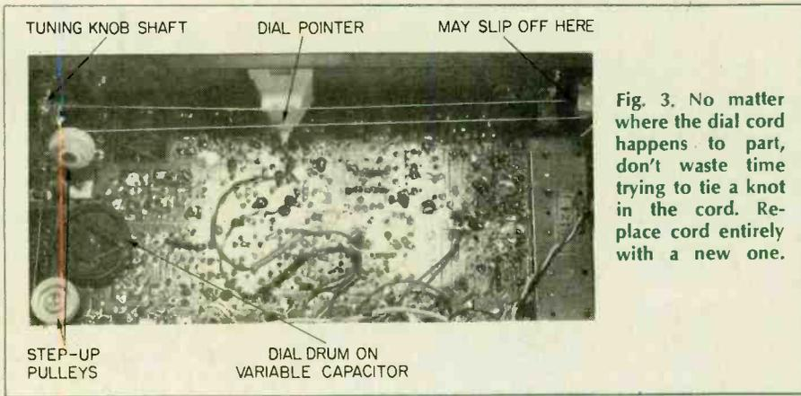
Fig. 3. No matter where the dial cord happens to part, don't waste time trying to tie a knot in the cord. Replace cord entirely with a new one.
