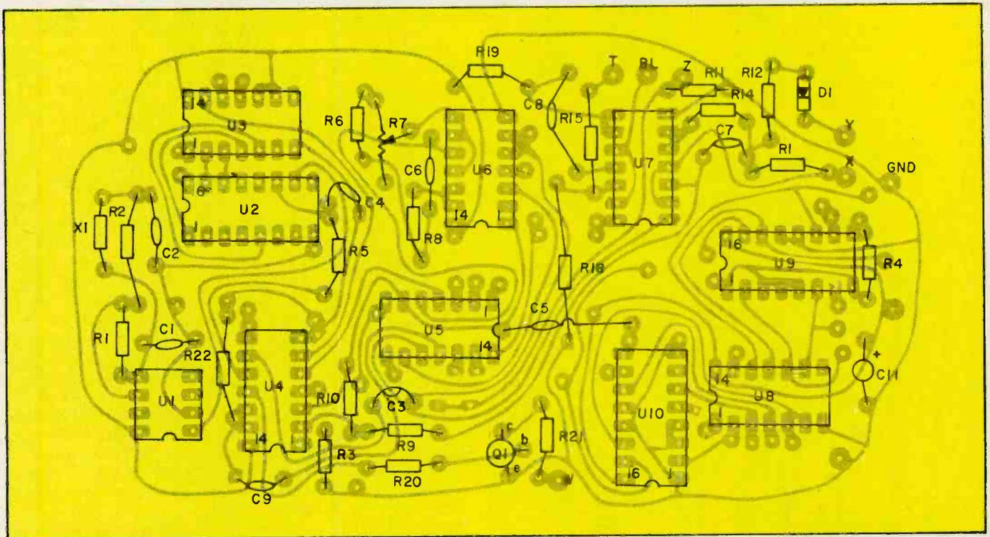
The component placement diagram above indicates the location of all parts on the main board. We suggest that you install the IC sockets last, because several components must be installed close enough to the sockets that there might be problems in fitting them in. After the components are installed, see the jumper location diagram two pages ahead to complete the board assembly.
