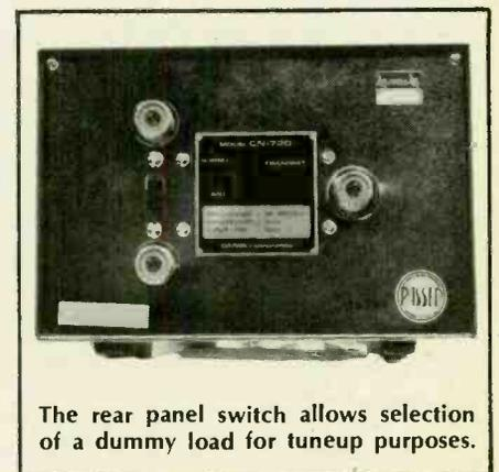
The rear panel switch allows selection of a dummy load for tuneup purposes.
