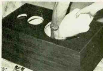
Slip the front panel into place and allow the glue to dry. Add sound deadening material.
