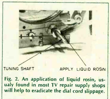
Fig. 2. An application of liquid rosin, usually found in most TV repair supply shops will help to eradicate the dial cord slippage.
