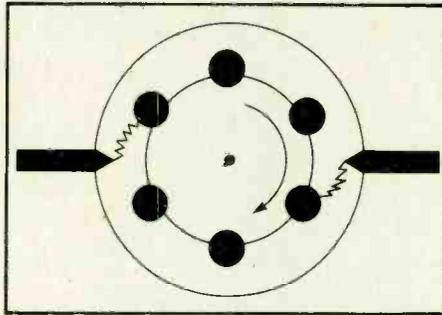
Fig. 4. The rotary spark gap mechanism was the first method used to increase the spark frequency in the later spark gap units.
