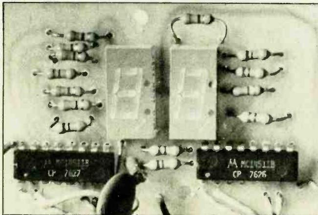
This is the finished display board, showing the two 7-segment LEDs in position. You may wish to utilize IC sockets (14-pin) for them as well, in order to provide additional clearance from the PC board to the front.
