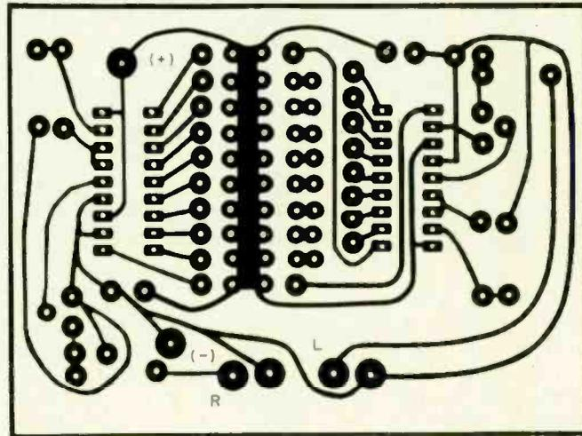
This is the full scale etching guide for the printed circuit board, seen foil side up. Check your finished board carefully for foil bridges and other errors.
