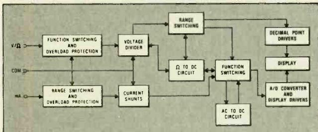
is then passed into a DC voltmeter which consists of an automatic offset correction (auto zero) circuit, a dual slope integrator, and a digital processing and multiplexing device. The reference voltage is derived from a highly stable Zener diode.
