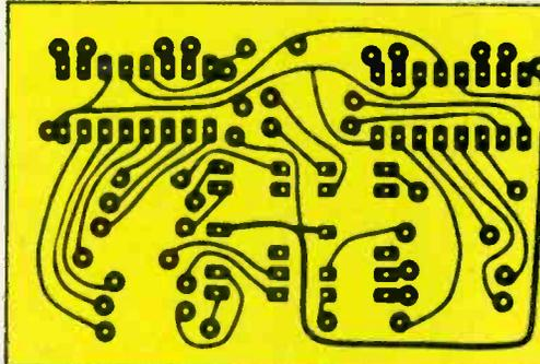
This is the full-scale template for etching the printed circuit used on the display board. Cut the board itself to allow a 1/2-inch margin around the edges. This is done in order to accommodate different chassis mounting schemes, something which you can decide yourself in later phases of construction.
