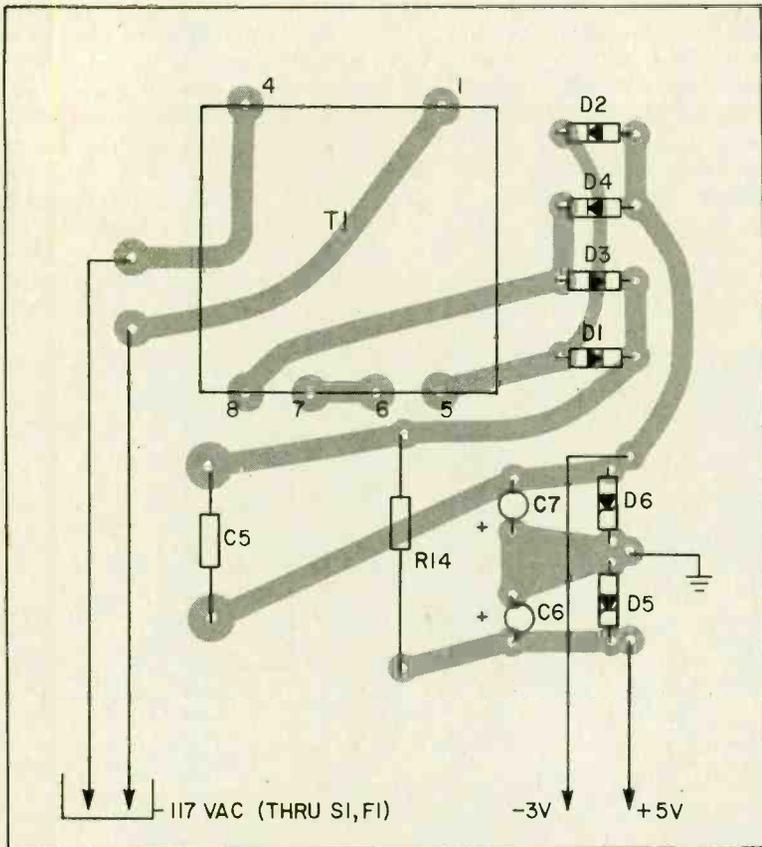
The component layout for the power supply board was deliberately made spacious to allow for the differences in component sizes of different manufacturers. Observe polarity of diodes and capacitors.
