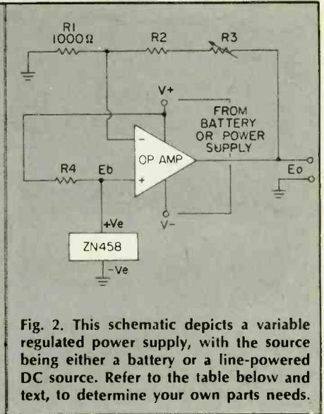
Fig. 2. This schematic depicts a variable regulated power supply, with the source being either a battery or a line-powered DC source. Refer to the table below and text, to determine your own parts needs.
