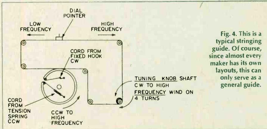
Fig. 4. This is a typical stringing guide. Of course, since almost every maker has its own layouts, this can only serve as a general guide.
