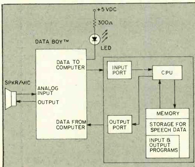
This flow diagram illustrates the function of the Data Boy with the computer's central processor and memory storage. In effect, the Data Boy acts as an analog-to-digital and digital-to-analog converter. While this method is not perfect, it is the most economically feasible means of allowing for speech reproduction on the hobby computer level.
