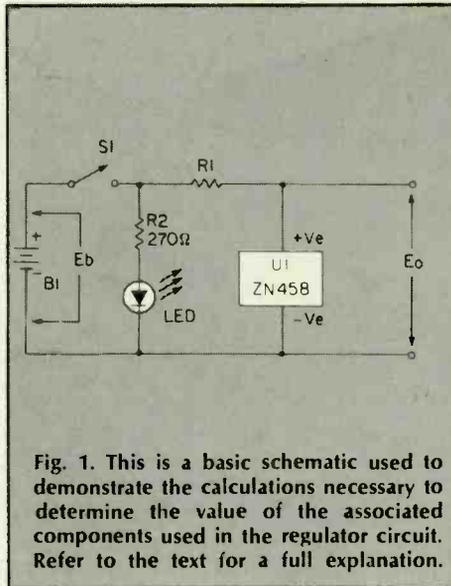
Fig. 1. This is a basic schematic used to demonstrate the calculations necessary to determine the value of the associated components used in the regulator circuit. Refer to the text for a full explanation.
