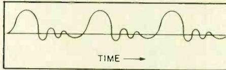
This is the analog waveform of a vowel. It must be converted to a digital signal.
