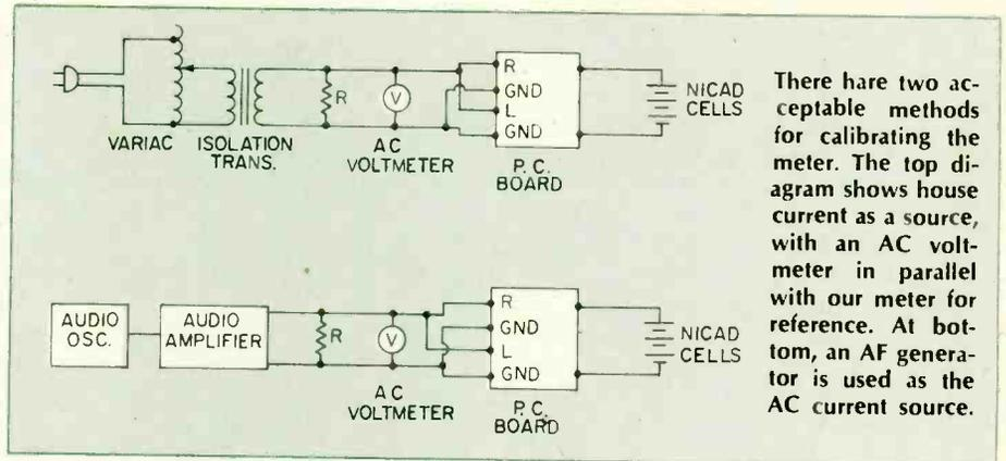
There are two acceptable methods for calibrating the meter. The top diagram shows house current as a source, with an AC voltmeter in parallel with our meter for reference. At bottom, an AF generator is used as the AC current source.
