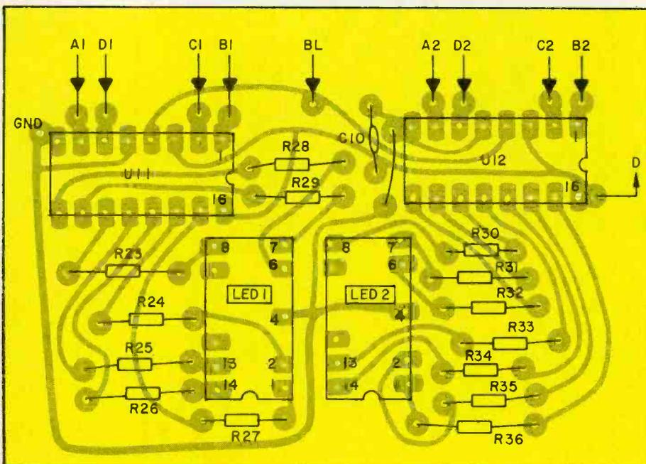
The component placement diagram for the display board also shows the attachment points for the wiring coming from the main board at top. Note the lone jumper used on this board, located between C10 and U12. Put it in first because it's very easy to forget.
