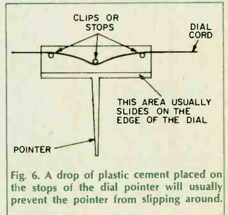
Fig. 6. A drop of plastic cement placed on the stops of the dial pointer will usually prevent the pointer from slipping around.
