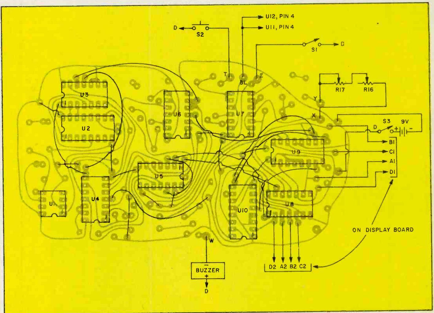
The jumper location diagram above also includes the wiring connections for the remainder of the off-board components, as well as the interconnections between it and the display circuit board. Point D at S3 is a junction for several connections (hot side of buzzer, hot side of S1 and S2). Simply attach all incoming leads to the terminal on the switch back (switch S3) after mounting.
