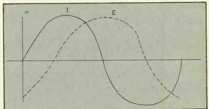
Any measurement of voltage under these conditions must take into consideration the changing nature of voltage and current flows and the impedance of the measuring device.
