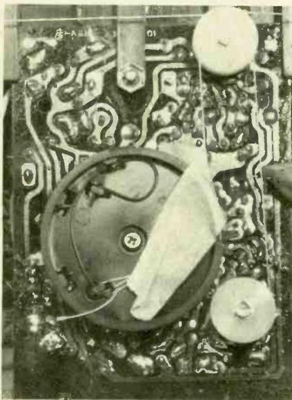
Fig. 7. If the dial drum must be moved during service, lock the cord onto the drum with tape to avoid unwinding the cord.
