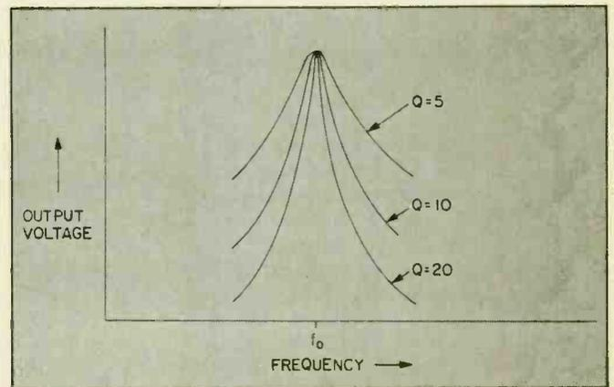
Fig. 2. The higher the "Q" value of the filter, the narrower the bandpass frequency width will be. Obviously, a filter with a "Q" value of 20 will exhibit a narrower width than one with a "Q" of 5.
