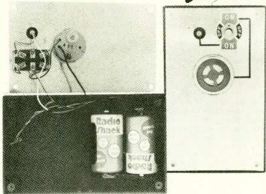
**Y**OU WON'T MISS any more phone calls when out of hearing range of your telephone, if you add this simple remote signalling unit which alerts you to incoming calls by means of either a buzzer or blinker light. The unit is self powered for easy placement in any room in your home, or even outdoors where there are no AC outlets.
