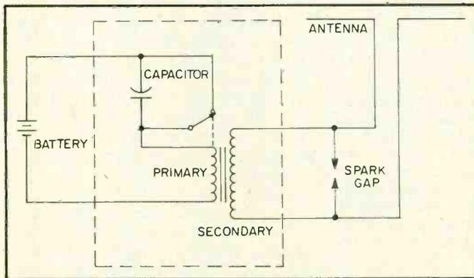
Fig. 1. This is the schematic of Hertz's original spark gap transmitter. There was no key, as it was set to oscillate continuously.
