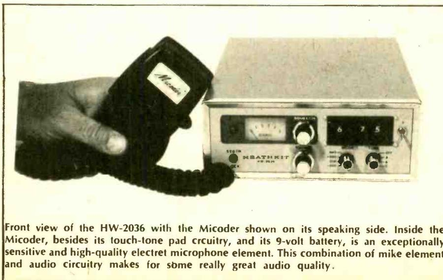
Front view of the HW-2036 with the Micoder shown on its speaking side. Inside the Micoder, besides its touch-tone pad circuitry, and its 9-volt battery, is an exceptionally sensitive and high-quality electret microphone element. This combination of mike element and audio circuitry makes for some really great audio quality.
