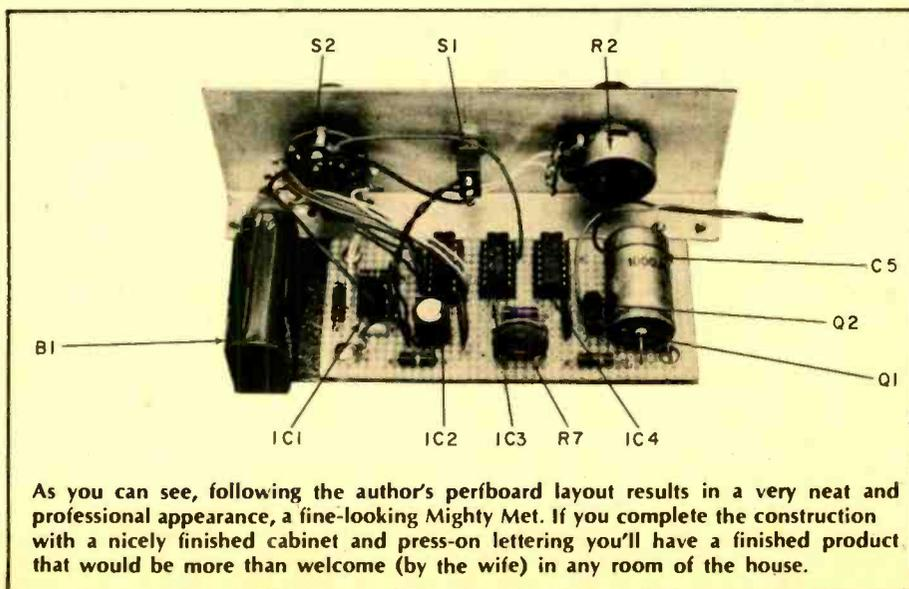
R3 is negligible). A different range may be had by changing the values of R1, R2, or C1. R1 determines the upper tempo limit, while R2 determines the lower limit. Changing C1 will affect the overall tempo range. The sound quality of the clicks can be changed by increasing or decreasing the value of R3, which changes the width of the pulse from IC1. Do not make R3 less than 200 ohms, however.
