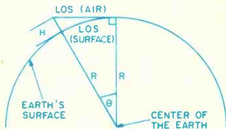
This figure illustrates the geometry on which the charts and diagrams are based. Note that  $r$  is measured from the center of the earth and  $H$  is the height of the antenna.
