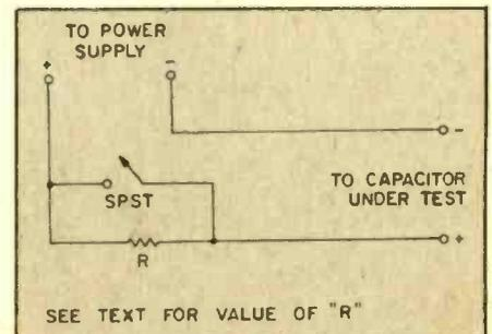
The resistor value R in this test circuit to find leakage is explained in the text.
