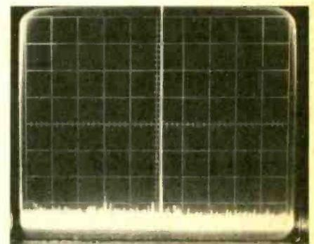
Is it clean? This 'scope trace off our spectrum analyzer shows only the signal, and the analyzer's noise as "grass" some 55 to 60 dB down. Each horizontal division is 5 MHz, so you're looking at 25 MHz either side of the carrier. We couldn't find any trace of a second harmonic in the "grass" so we're not showing a photo because there's nothing to show.
