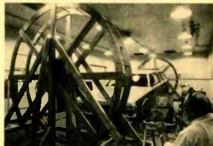
A new 1978 station wagon is tested for effects by outside power line radiation. GM also measures RF noise generated by auto.
