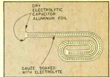
Cross section showing the internal construction of a "dry" electrolytic capacitor. Two sheets of aluminum foil are rolled up with a strip of electrolyte-saturated gauze between.
