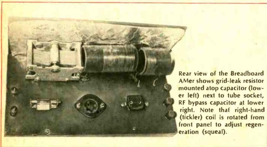
Rear view of the Breadboard AMer shows grid-leak resistor mounted atop capacitor (lower left) next to tube socket, RF bypass capacitor at lower right. Note that right-hand (tickler) coil is rotated from front panel to adjust regeneration (squeal).
