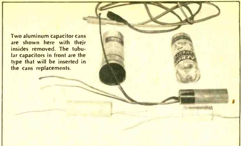
Two aluminum capacitor cans are shown here with their insides removed. The tubular capacitors in front are the type that will be inserted in the cans replacements.
