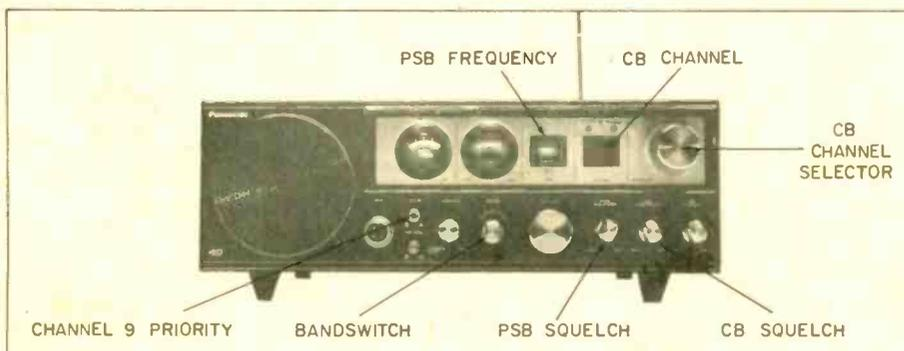
Though the Panasonic RJ-3660 combines an FM PSB receiver and an AM CB transceiver in the same cabinet, the front panel isn't cluttered or complicated. Major differences is a PSB tuning dial in addition to the digital CB channel indicator, and separate squelch controls for each receiver. You'll be sure to find the PSB receiver a useful addition, especially in time of emergency when your CB is most important. For more information circle No. 67 on the Reader Service Coupon.
