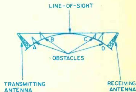
There are four possible ways obstacles may be positioned between a receiving and a transmitting antenna. Note that A and C are below line-of-sight between the antennas.
