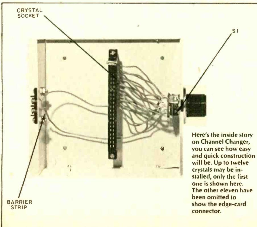
Here's the inside story on Channel Changer, you can see how easy and quick construction will be. Up to twelve crystals may be installed, only the first one is shown here. The other eleven have been omitted to show the edge-card connector.
