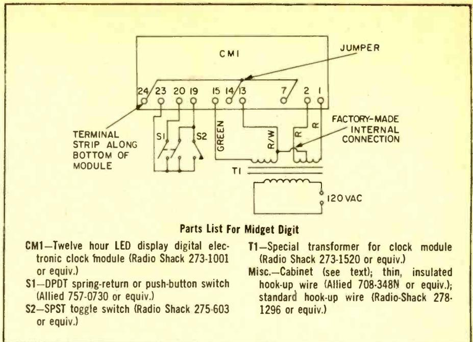
pressed (remaining depressed) the timer should hold. Releasing the switch should cause the timer count to resume without a reset to zero.
