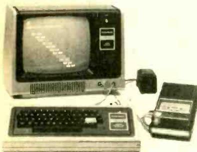
**Radio Shack System**—Radio Shack's TRS-80 microcomputer system consists of a 53-key professional type keyboard and microcomputer plus regulated power supply, a computer-controlled data cassette recorder and a 12-inch video display monitor. The complete system is priced at \$599.95 but the microcomputer alone is available for \$399.95. The microprocessor is an advanced Z-80 8-bit processor. The video display is memory mapped, all graphics and alphanumeric controlled by BASIC
