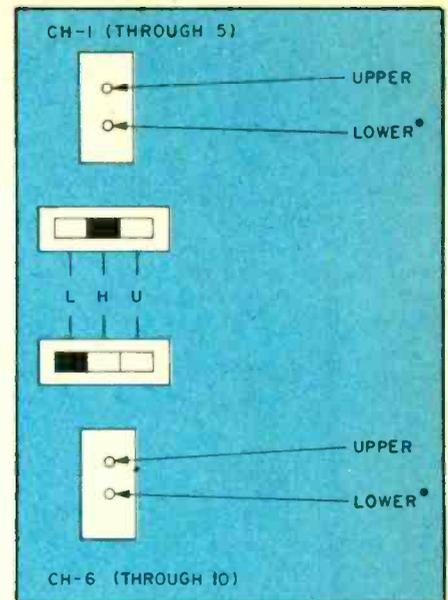
If you're interfacing Channel Changer on your scanner's channels 1 through 5 (inclusive) connect a wire from terminal one on the barrier strip to the lower pin in the socket. If to channels 6 through 10 (inclusive) then the wire goes from the terminal to the upper pin in the socket. Make certain you don't do it backwards.
