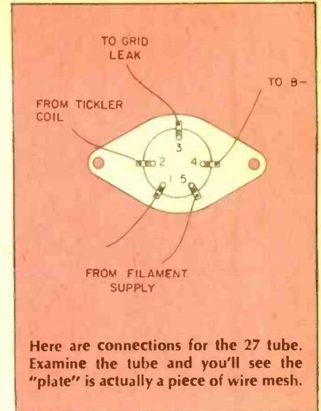
Here are connections for the 27 tube. Examine the tube and you'll see the "plate" is actually a piece of wire mesh.
