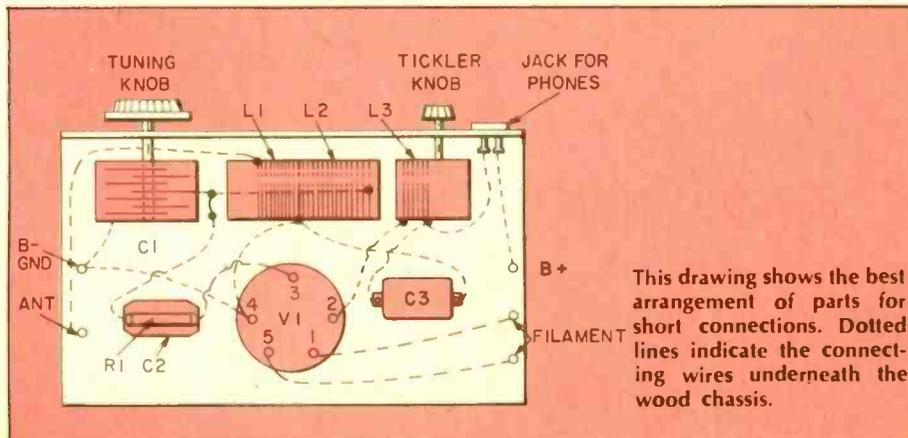
This drawing shows the best arrangement of parts for short connections. Dotted lines indicate the connecting wires underneath the wood chassis.
