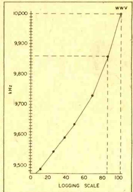
Note how WWV, 10,000 kHz, corresponds to 100 on the logging scale and a station known to operate at 9,850 kHz is found to correspond to 85. The points plotted on the middle and low sections help insure the graph's fidelity throughout its range.
