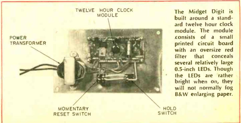
The Midget Digit is built around a standard twelve hour clock module. The module consists of a small printed circuit board with an oversize red filter that conceals several relatively large 0.5-inch LEDs. Though the LEDs are rather bright when on, they will not normally fog B&W enlarging paper.
