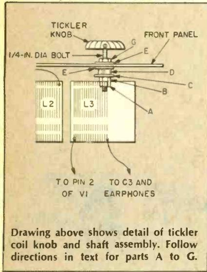
Drawing above shows detail of tickler coil knob and shaft assembly. Follow directions in text for parts A to G.
