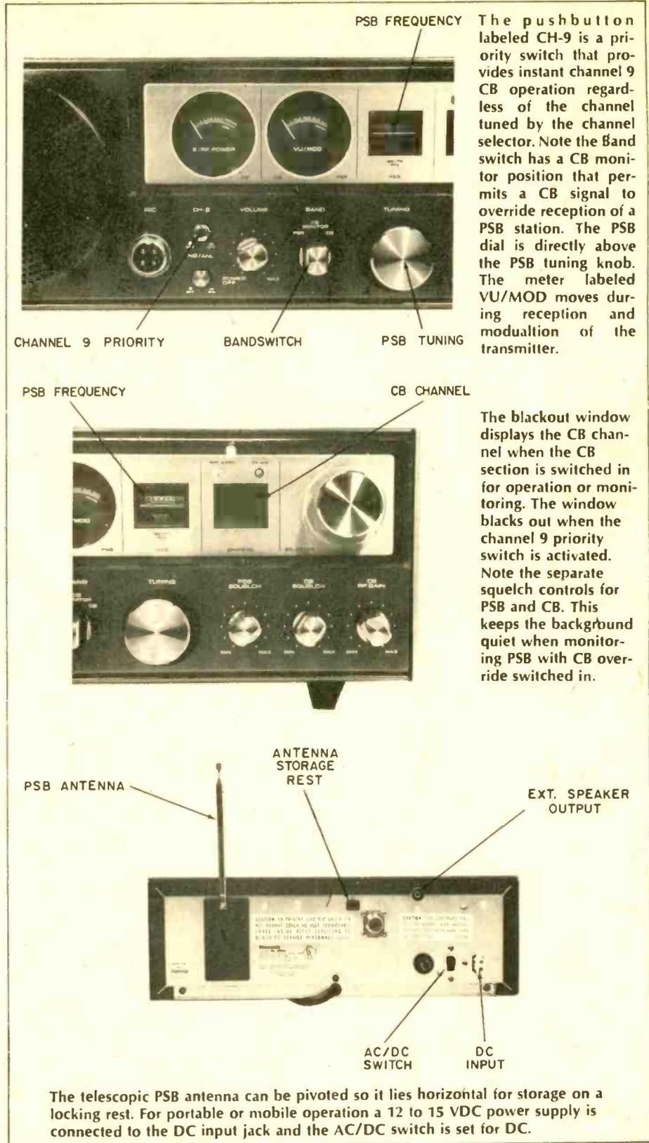
The pushbutton labeled CH-9 is a priority switch that provides instant channel 9 CB operation regardless of the channel tuned by the channel selector. Note the Band switch has a CB monitor position that permits a CB signal to override reception of a PSB station. The PSB dial is directly above the PSB tuning knob. The meter labeled VU/MOD moves during reception and modulation of the transmitter.
