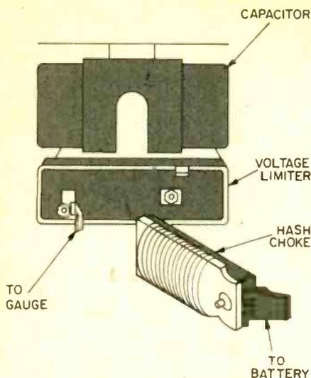
An erratic scraping noise may point to your vehicle's noise limiter. Try installing a hash filter in series with the limiter and battery; also install either a pigtail or a coaxial capacitor at the terminal.
