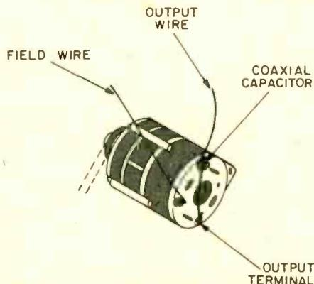
An alternator can often be stopped from whining by the installation of a coaxial capacitor at the alternator's output wire.
