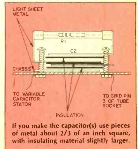
If you make the capacitor(s) use pieces of metal about 2/3 of an inch square, with insulating material slightly larger.
