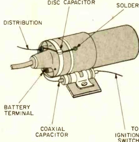
Those annoying popping sounds, which can be traced to the ignition system, can be readily cured. Install a coaxial capacitor at the coil's battery terminal and a .005-uF, 1,000 VDC, disc capacitor to distributor.
