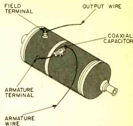
A generator's high whine can often be silenced by installing a coaxial capacitor at the armature terminal of the generator.
