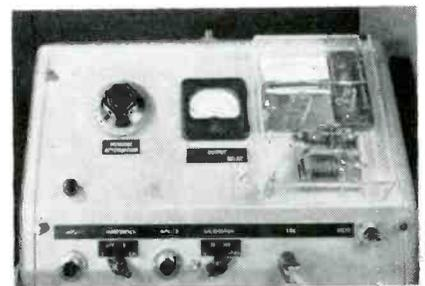
Front panel of respiration monitor with control relays mounted under plastic cover at upper right. System is fail-safe, switching to automatic operation if patient does not trigger breathing cycle
