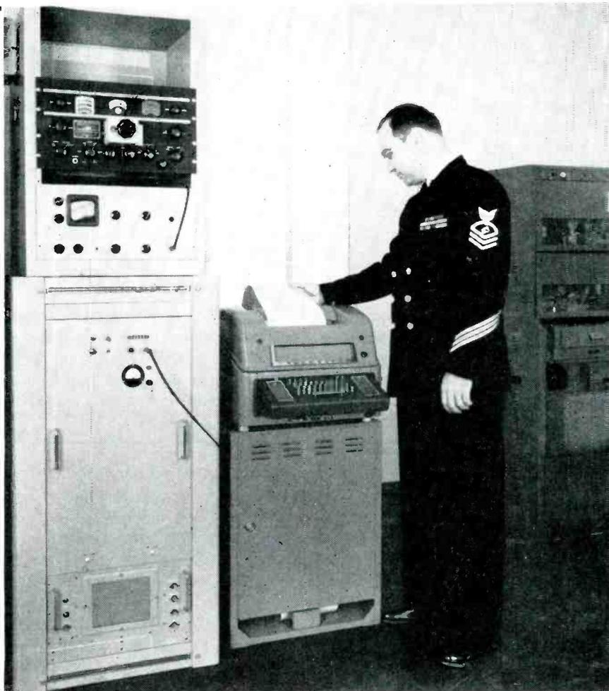
Trak model CMP-15 Morse-to-teleprinter code converter (lower left) installed for evaluation at U. S. Navy Radio Station, Cheltenham, Md., with station WWL being copied by interconnected Teletype machine at 100 words per minute. Radio receiver and static rejector are in rack above converter.—Official photograph, U. S. Navy
