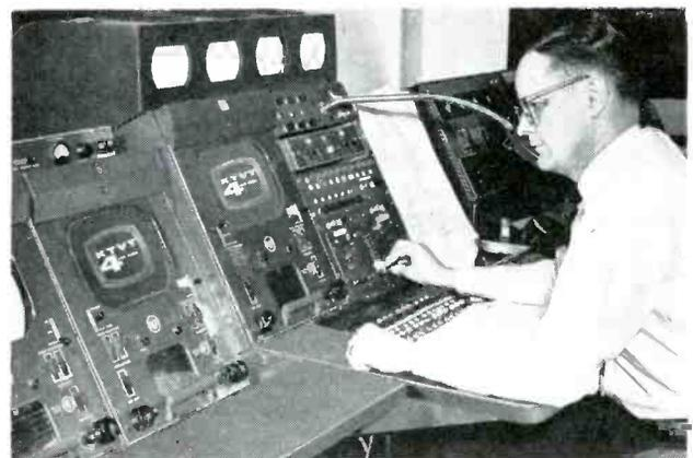
FIG. 3—Control circuit for use with RCA TK20-D iconoscope chain. Operator punches up call-letter slide on switching-mixing unit
