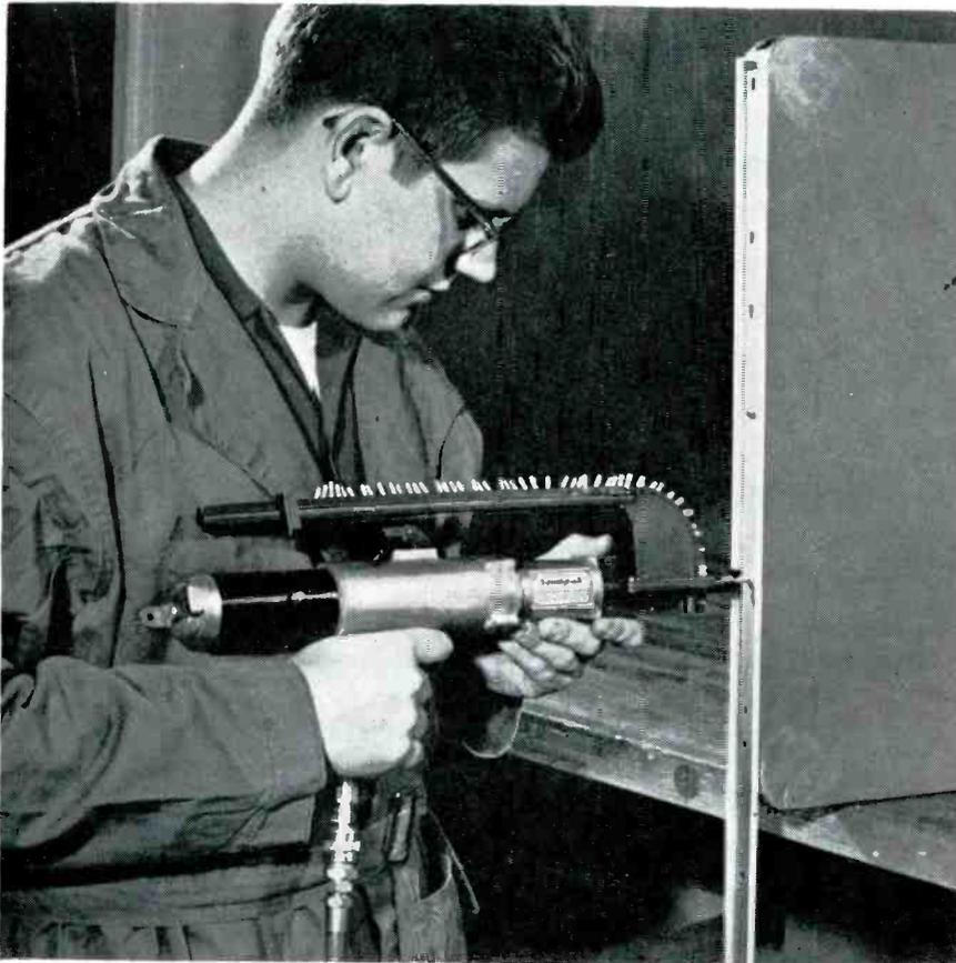
A COMPLETELY AUTOMATIC power screwdriver, developed for mass assembly operations by the Shakeproof Division of Illinois Tool Works, drives screws automatically at any angle as fast as the operator can pull the trigger. Weight is only 6½ lb.
