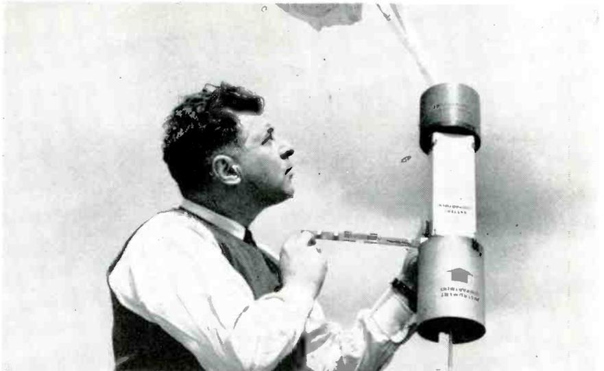
**ELECTRONIC** weather paratrooper, new type of high-altitude sonde, is checked in flight position by General Instrument engineer. The equipment is a . . .
