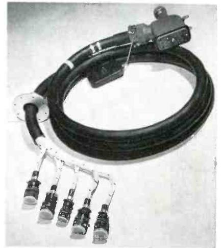
Example of special missile-launcher cable harness having neoprene jacket which remains flexible down to -65 F. Five connector fittings at lower left are anchored in waterproof junction box. Flange on cable provides seal to box
