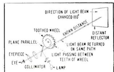
FIG. 1—Fizeau's toothed wheel for measuring speed of light
