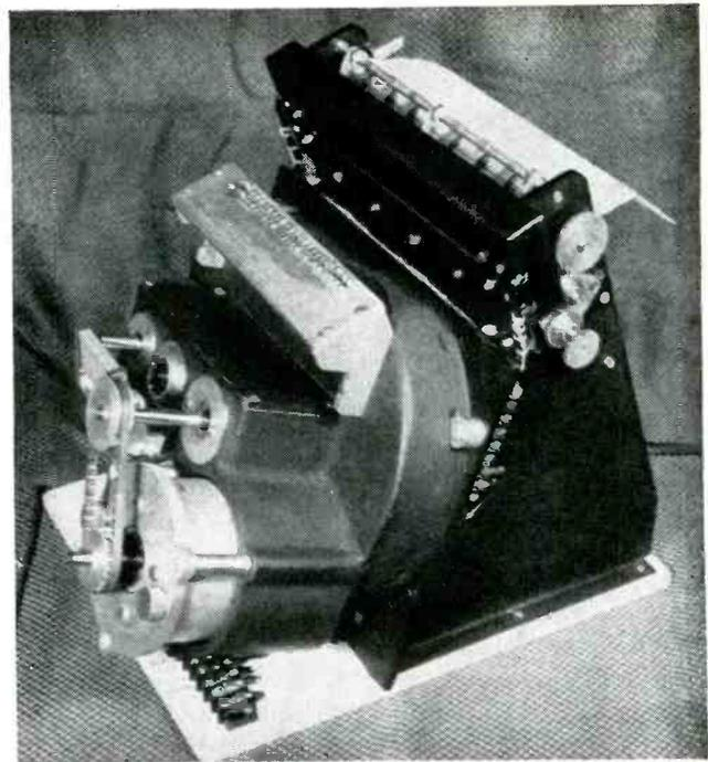
Transmitter-scanner must be solidly constructed to reduce vibration from high-speed operation. Continuous copy at upper right
