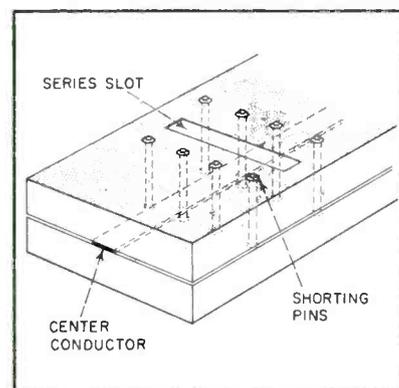
FIG. 2—Series-slot radiating element showing use of shorting pins
