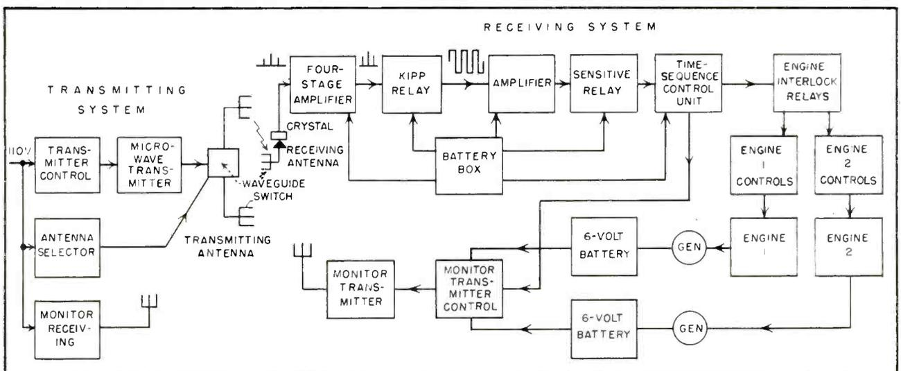
FIG. 1—Block diagram of microwave transmitting and receiving systems of remotely controlled fog alarm
