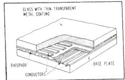
FIG. 2—Construction of phosphor screen
