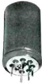
Airpax Series 300 choppers are available in three mounting styles. The popular plug-in style, Type 300, fits a 7-pin miniature tube socket. It can be locked in place by a tube shield.
