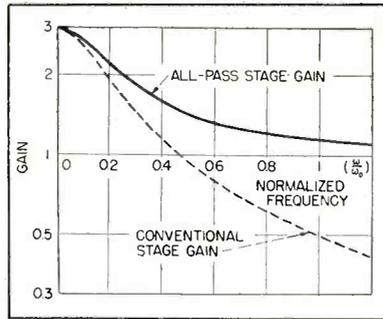
FIG. 2—Gain per stage of conventional amplifier compared with all-pass amplifier
