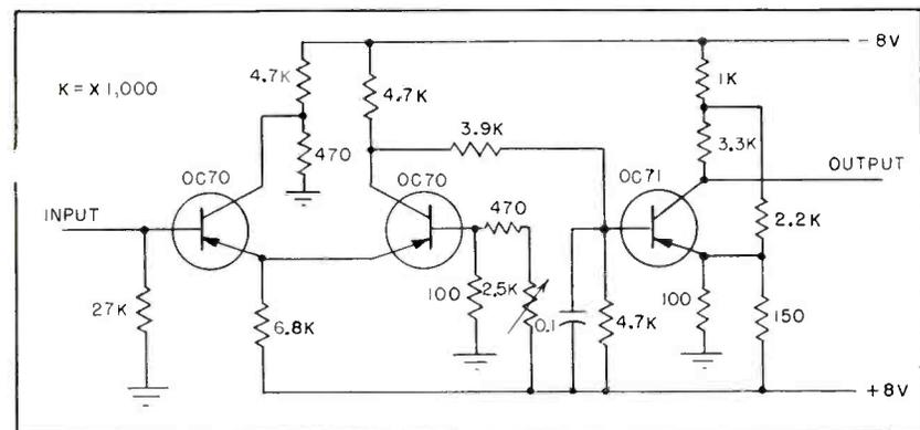
FIG. 2—Direct-coupled amplifier has gain of 500 and 30-kc bandwidth without feedback. Input impedance is approximately 50,000 ohms
