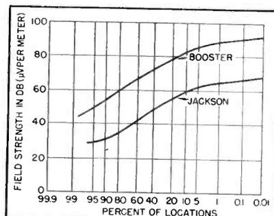
FIG. 3—Percentage of locations that have field strengths greater than or equal to the ordinate show usefulness of booster
