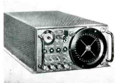
Compact indicator suitable for small airports tunes vhf aircraft radio bands and furnishes bearings even when voice signals are unintelligible. Built by Olympic Radio and Television, Inc., it was described in technical article on p 184 of June 1955 issue of this magazine but without company designation
