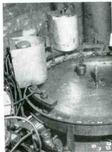
Air cylinders on top of turntable move the electrode banks up and down after turntable is advanced by air cylinder at lower left. First electrode bank is not in use here
