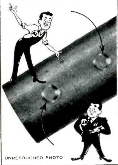
Loosen a set screw and look at the shaft it's pressing against. The set screw must make a full circle impression with no rough edges in order to give maximum holding power.
