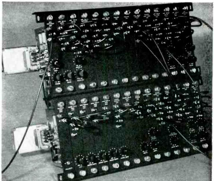
Rack-mounted group of simulator modulators. Unitized construction provides for testing wide variety of radar systems
