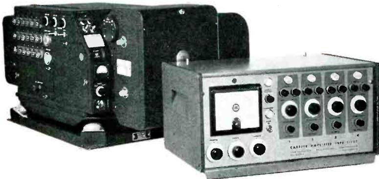
**5-114 RECORDING OSCILLOGRAPH...** most widely used, most versatile oscillograph in the world today. Either 18 or 26 traces on 7" paper or film. High-speed accessory magazine holds 250 ft. of paper and permits record speeds up to 500"/sec. SEND FOR CEC BULLETIN 1500C-X1.
