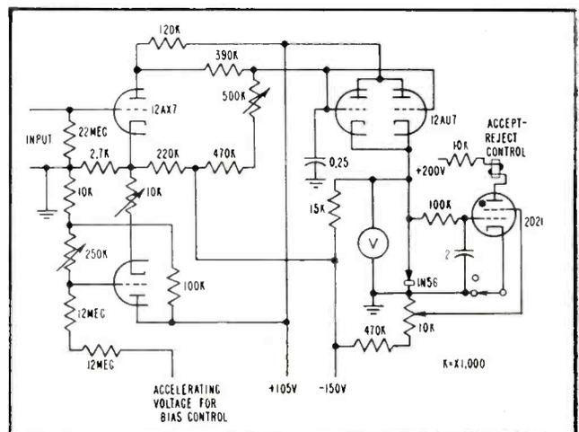
FIG. 4—Direct-coupled amplifier triggers thyratron to reject if ratio of phototube outputs is increased by presence of green rot
