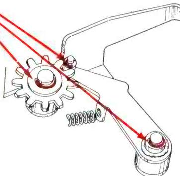
Truarc E-ring (Series 5133) eliminates use of tapped hole and shoulder screw, retains roller which prevents over-travel of gear. Assembly is rapid.
