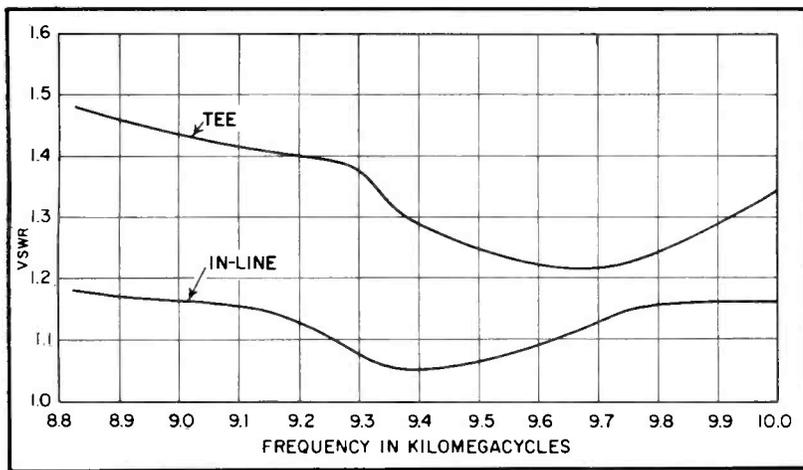
FIG. 5—Frequency versus vswr characteristics of in-line and T junctions
