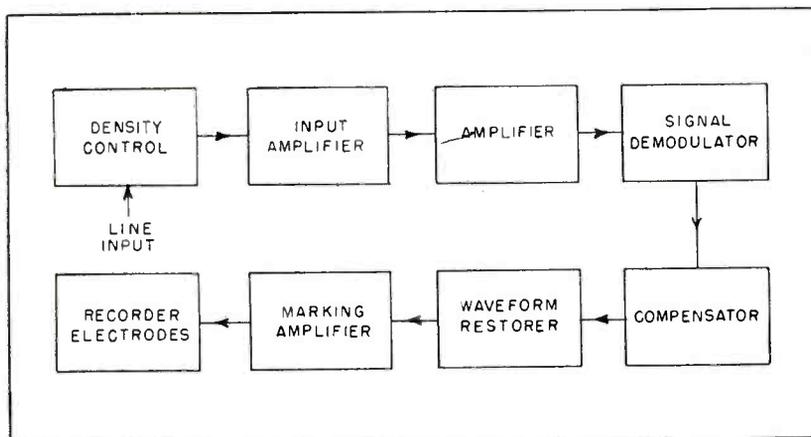
FIG. 2—Elementary facsimile receiver-recorder used on narrow-band lines
