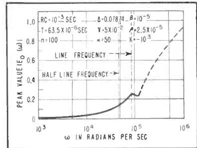
FIG. 3—Clamp circuit response to cosinusoidal signal after initial transient
