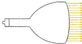
**MAGIC-MIRROR ALUMINIZED TUBE** — Aluminized reflector allows electron beam through. Blocks wasted light from backing up into tube. Reflects *all* the light into picture.
