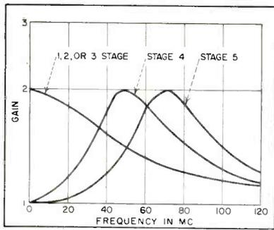
FIG. 5—Individual stage response of 10 to 70-mc all-pass amplifier
