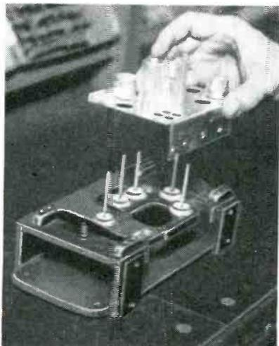
Placing chassis on jig after nuts of tuning elements have been set into recesses
