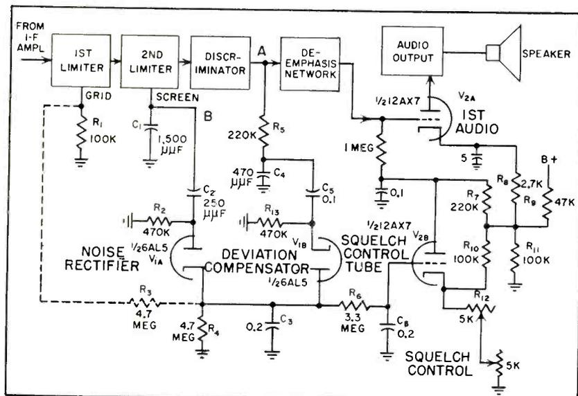
FIG. 2—Deviation-compensated squelch circuit uses audio output from discriminator to prevent muting during wide excursions of signal
