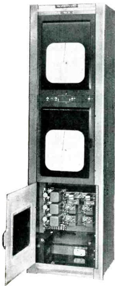
Central terminal equipment for control of remote operations and display of telemetered information.
