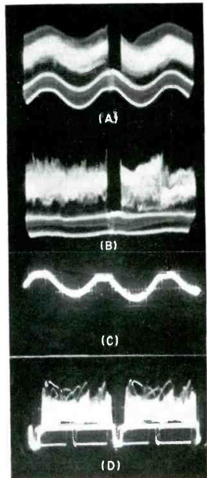
FIG. 7—Input (A) and output (B) signals for video signal with 20-percent sinusoidal voltage added. Error voltage (C) and waveform at 6AG7 cathode (D) are shown for the same condition
