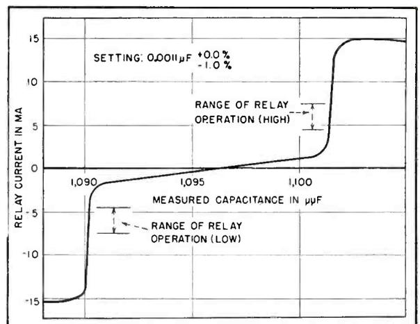
FIG. 5—Current in polar relay of 1-kc bridge when set for tolerance range of 1 percent at 0.0011  $\mu\mu\text{f}$
