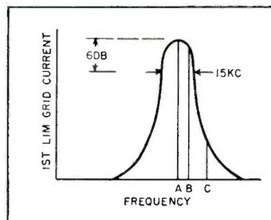
FIG. 3—Loss-of-signal effect encountered when un hindered deviation resulting from high modulation moves signal out of receiver passband
