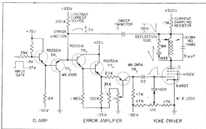
FIG. 4—Cathode-ray-tube deflection system employing transistors. Value of  $C$  in  $\mu\text{f}$  is equal to  $10 \times$  sweep duration in seconds
