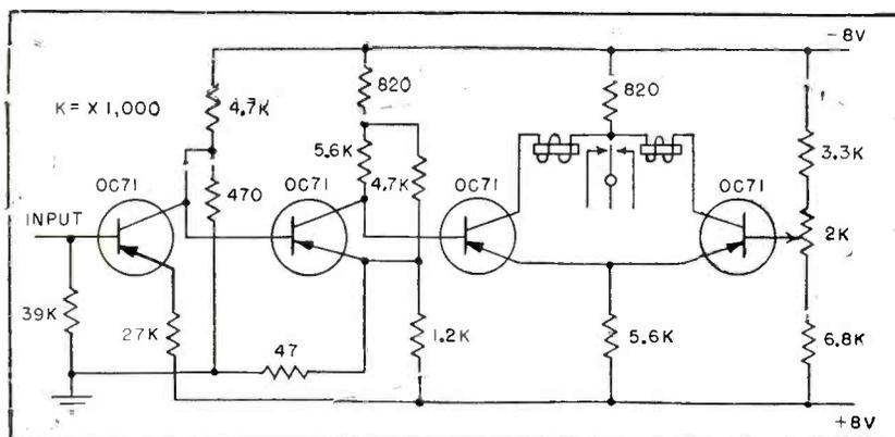
FIG. 1—Transistor servo amplifier with 0.11-watt power drain replaces vacuum-tube counterpart with 25-watt drain
