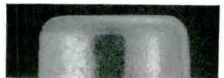
**Radius of Curvature** of edge of cap lessens the danger of high temperature "dishing" frequently experienced with large area, sharp edge cathodes. "Dishing" would affect cut-off voltage of tube, require use of more expensive variable resistor in grid circuit. A small flat surface is retained to provide a satisfactory source of emission current.
