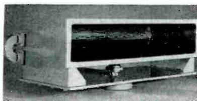
Vertically polarized receiving-antenna aperture has Vinylite-window weather seal for all weather operation
