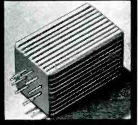
Here's a clamped flip-flop that can answer your need for subminiature plug-in binary elements in computer applications. Sprague's new Type 200C5 combines a proven circuit with a new concept of printed circuitry developed by Sprague.
