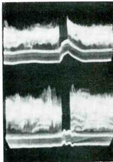
FIG. 6—Input and output signals for a video signal deficient in low frequencies
