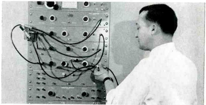
**2. 10-minute changeover.** Engineer simply connects one new delay unit into the system and sets up controls for new pulse sequence. Units are matched to each other; so no buffers are required. Units connect together through standard cables.
