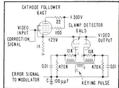
FIG. 1—Diode clamp detector operates from low-impedance source minimizing effect of unbalance between diodes
