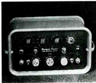
sec are provided; however, longer intervals are easily noted by watching the thousands decade, or through use of an auxiliary electro-mechanical register. The WE-210 can be used for timing high-speed electrical or mechanical devices such as: relays, actuators and camera shutters. The instrument also operates as an electronic counter having a maximum counting rate of 50,000 pps. One-kc and ten-kc front-panel outputs are provided for use as a frequency standard.
