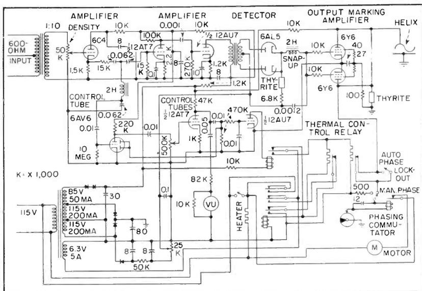
FIG. 4—Receiver-recorder employing special paper prints with output of marking amplifier
