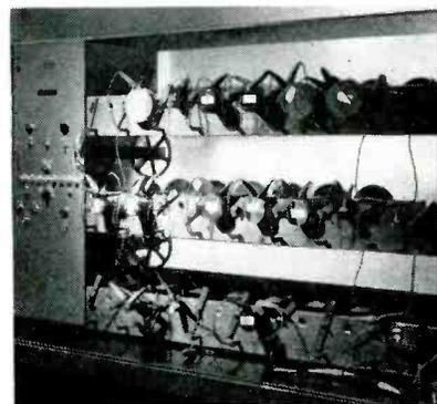
Gear-driven arrangement for testing 24 potentiometers at a time. Eight lamps combined with three-position selector switch permit quick determination of failed unit
