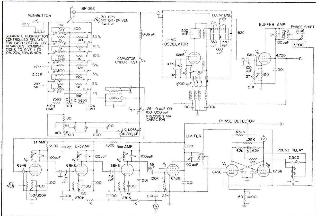
FIG. 3—Modified circuit using 1-mc signal source for sorting low-value capacitors
