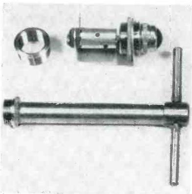
T-handled threaded mandrel used as ferrule wrench, with lamp socket assembly at upper right and the ferrule itself at upper left. Ferrule has flange that bears against front of panel when installed; knurled part of bezel on mandrel tool bears against this flange when tool is installed
