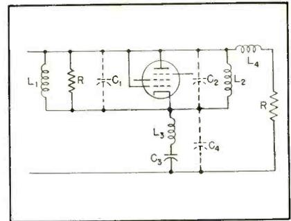
FIG. 3—All-pass amplifier stage, showing stray capacitance to ground with inductance  $L_1$  inserted in output
