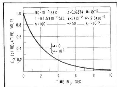
FIG. 2—Response of clamp circuit to cosinusoidal input
