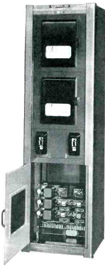
Remote terminal equipment. Operates in response to signals received from the central control point to perform ON-OFF and OPEN-CLOSE operations and returns metered data. Local control and indicating meters are also included.
