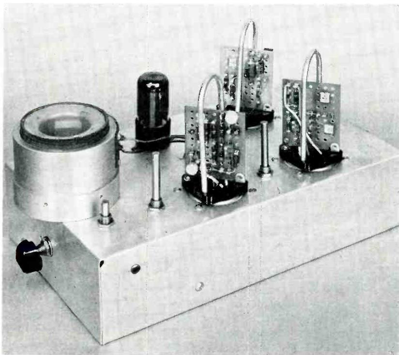
Complete transistor sweep system including yoke, yoke driver, error amplifier, clamp and gate circuits
