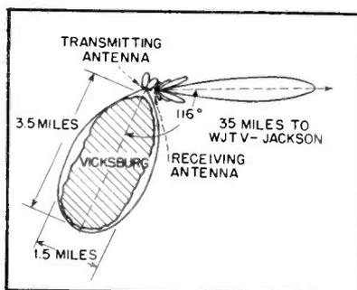
FIG. 2—Relative location of the booster, originating station and area to be served by it
