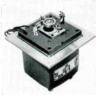
Closeup view of motor-driven switch that switches bridge from high-limit to low-limit standards at rate of 30 times per second to check tolerance
