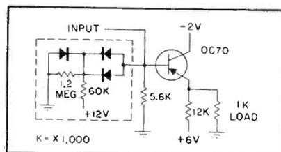
FIG. 7—Experimental temperature-compensating circuit uses germanium point-contact diodes
