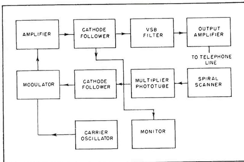
FIG. 1—Elements of the continuous-feed facsimile scanner-transmitter
