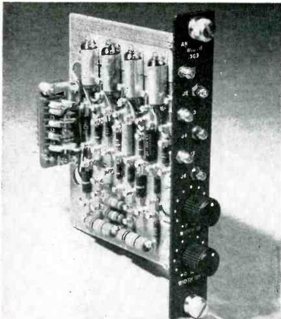
Terminal-board construction is used in modulators. Plug at rear connects unit into system
