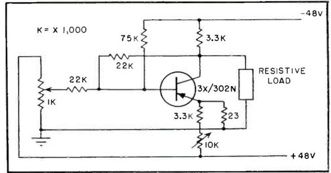
FIG. 5—Experimental high-output power amplifier uses 200-milliwatt pnp junction transistor
