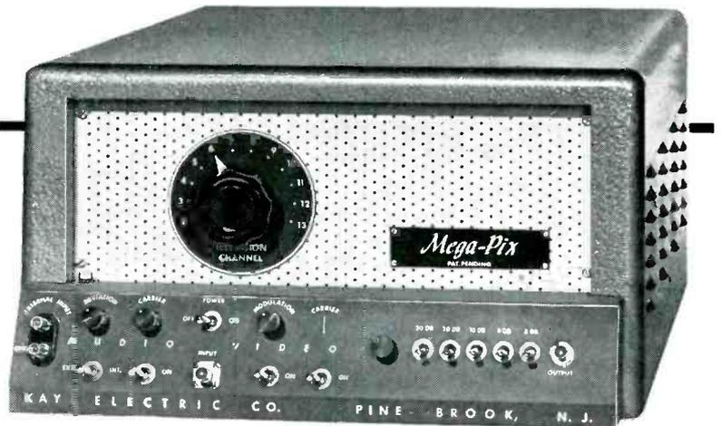
The Kay Mega-Pix provides two separate twelve-channel crystal controlled oscillators, frequency multipliers and output amplifiers to develop a crystal controlled RF picture and sound carrier on each TV channel.
