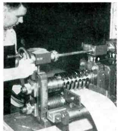
Input end of 12-inch rotary gang slitter as set up for cutting  $7\frac{3}{4}$  inch wide 0.012-inch silicon steel into  $\frac{1}{8}$ -inch strands
