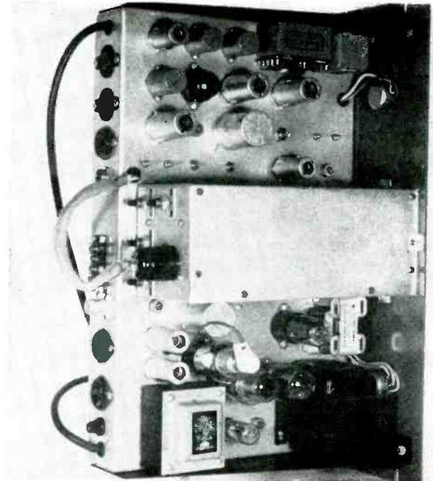
Compact scanner amplifier showing vestigial sideband filter (top) monitor oscilloscope (center) and power supply
