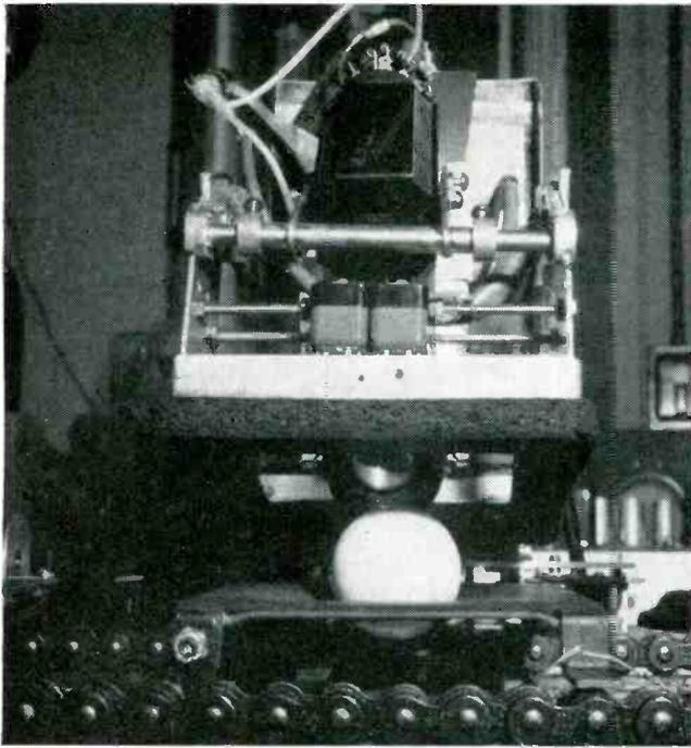
Phototube housing in raised position with cover removed to show placement of components
