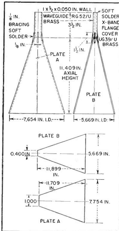
FIG. 2—Typical construction drawing for a gain-standard horn. Plates are made from 0.50 in. sheet brass
