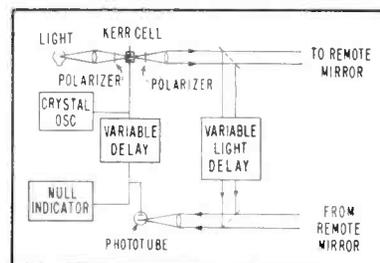
FIG. 2—Diagram shows use of the Kerr cell shutter and variable delay units
