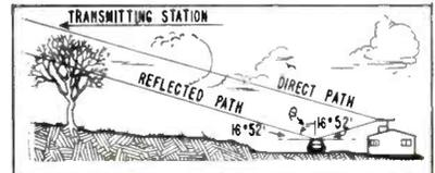
FIG. 1—Paths of direct and reflected television signals to receiving antenna
