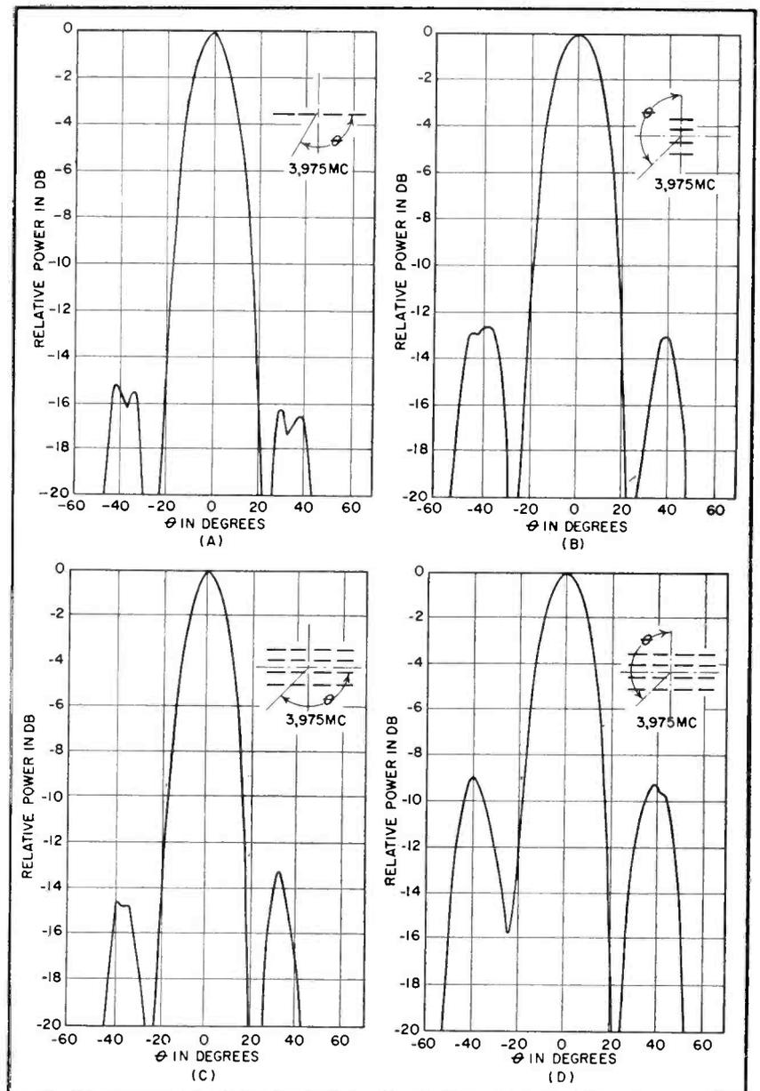
FIG. 10—Radiation patterns for H-plane array (A), E-plane array (B), E-plane pattern of composite array (C) and H-plane pattern of composite array (D)
