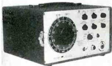
**RESISTANCE BRIDGE INDICATOR is self-balancing**
