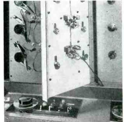
Door swung open to show eccentric slotted disks for each potentiometer. These mate with chain-driven slip clutches at right when door is closed
