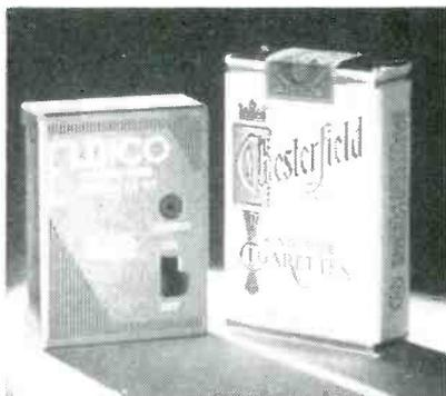
**FREQUENCY STANDARD is transistorized unit**
