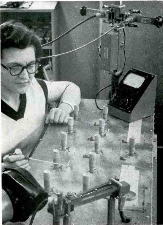
Using dental-type mirror to read each frequency meter in turn on mass-calibrating setup. Metal table is hinged and lifts up clear of meters for unloading and reloading after each batch is calibrated
