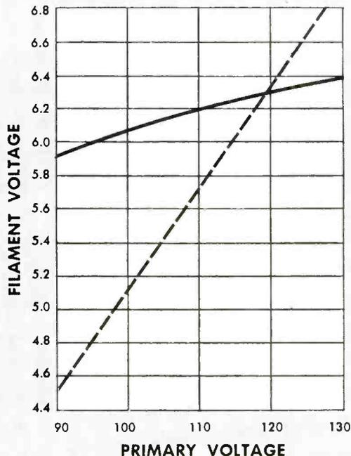
These curves contrast the plate and filament supply voltages obtained from a Sola and a conventional power transformer when line voltage is varied from 100v to 130v.
