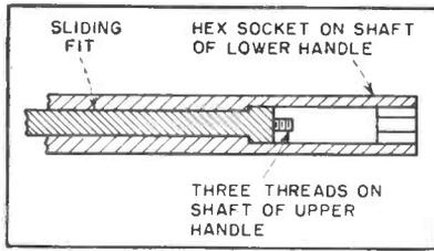
FIG. 1—Cross-section of two-handle starter for nuts
