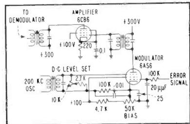
FIG. 4—Carrier-type modulator and amplifier used with clamp circuit
