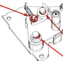
Three types of Waldes Truarc Retaining Rings are used in this assembly. One circular self-locking ring (Series 5105) retains pawl return spring. One external E-ring (Series 5133) retains roller used to prevent gear motion during transport cycle. One crescent ring (Series 5103) retains pawl which indexes gear. Second crescent ring retains sub-assembly. Truarc Rings speed assembly, cut rejects, eliminate parts.
