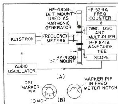
Calibrating setup (A), with waveforms seen on oscilloscope (B)
