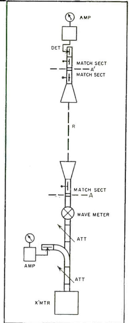
FIG. 3—Experimental setup for gain measurements
