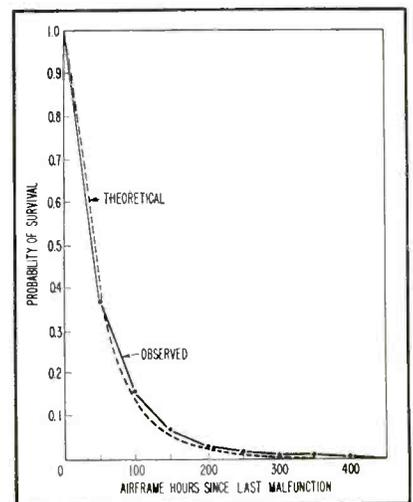
FIG. 1—Theoretical and observed reliability of airborne equipments
