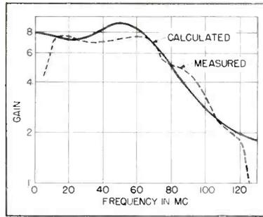
FIG. 6—Overall response characteristic of 10 to 70-mc all-pass amplifier
