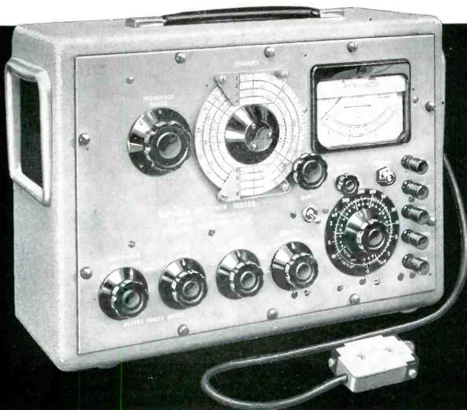
The Marconi Receiver Tester Type TF 888/3 combines a crystal-standardized cw/am signal generator, a tone source of variable level, and a 3-range audio power meter. Ideal for servicing, the instrument can be fitted with either an a.c. power pack or a dry-battery unit.
