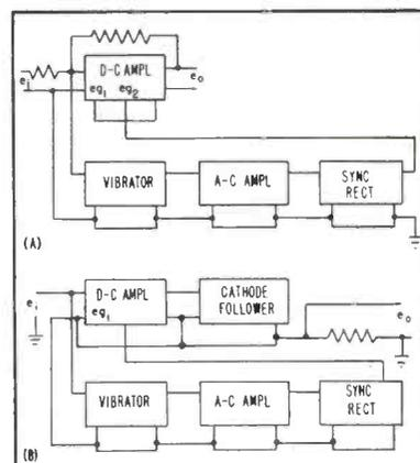
FIG. 5—Alternative stabilized d-c amplifier elements
