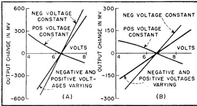
FIG. 4—Change in output of amplifier of Fig. 3 with variation of supply voltages for 68-db (A) and 78-db (B) feedback
