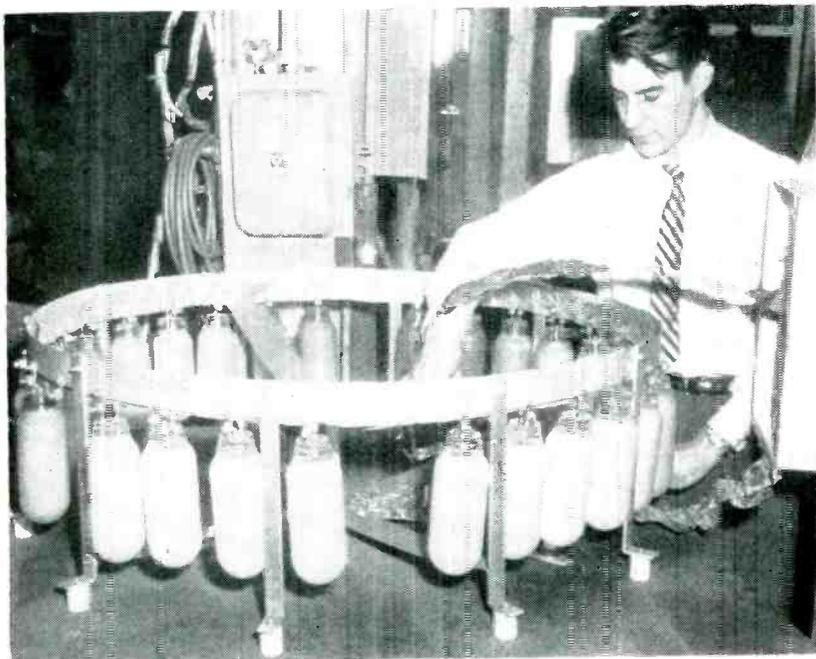
Connecting beacon lamp dummy load to 15-kw Thermatron r-f wood glueing generator operating at 6 mc
