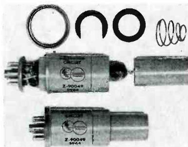
3.25 oz and is provided with a removable tube shield. It requires a peak-to-peak input signal of 25 v; +200 v d-c at 12 ma, -200 v d-c at 1 ma, and 6.3 v at 300 ma. The squaring circuit provides a 110-v peak-to-peak square or rectangular wave output up to 200 kc and 85 v at 1 mc. It has a negative-going rise time of 0.4 μsec or less and a positive-going decay time of 0.8 μsec or less. It has an output impedance of less than 10,000 ohms.
