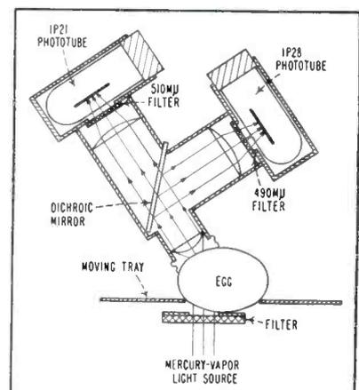
FIG. 2—Fluorescence from egg is split by dichroic mirror for transmission to two filtered phototubes
