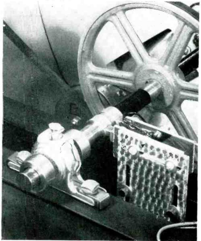
Audio signal is fed to rotating loudspeakers through coin-silver slip rings and silver graphite brushes
