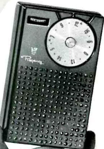
Here's a remarkable example of miniaturization . . . made possible mainly through the use of printed circuits and transistors. This diminutive radio weighs a scant 12 ounces, complete with battery. Yet, it has good tone, is selective, and delivers plenty of volume.
