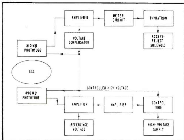
FIG. 3—Feedback from 490 m $\mu$  phototube is used to control accelerating voltage for both phototubes
