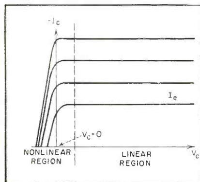
FIG. 1—Nonlinear and linear regions of junction-transistor characteristics
