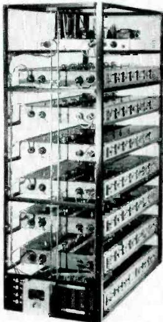
Rack-mounted tone generators can be placed up to 100 ft from console
