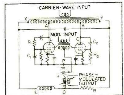
FIG. 10—Reactance-tube wide-angle phase modulator has low distortion
