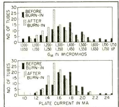
Effect of burn-in on range of mutual conductance and plate current for batch of 6BF7 tubes
