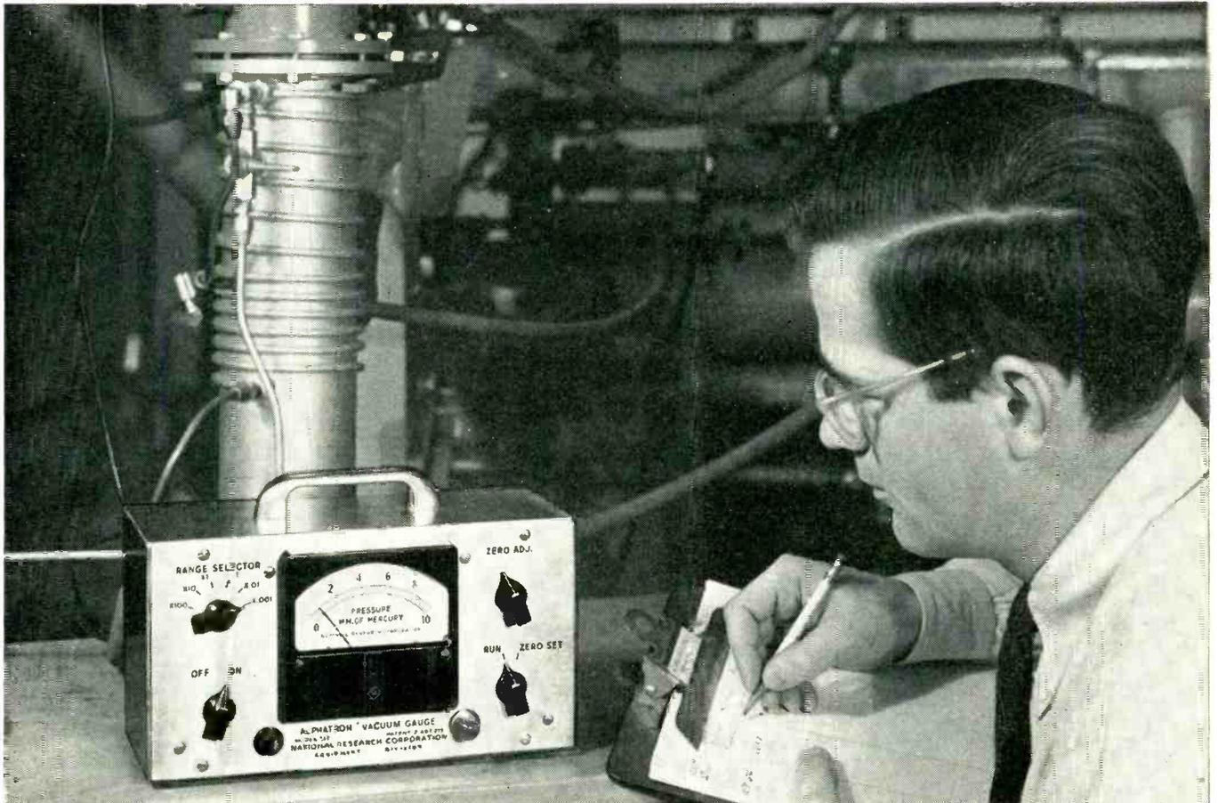
The AC-operated Model 517, newest of the Alpatron® Vacuum Gauges, with 6 ranges covering pressures from 1000 to .0001 mm. Hg. Price: \$425.
