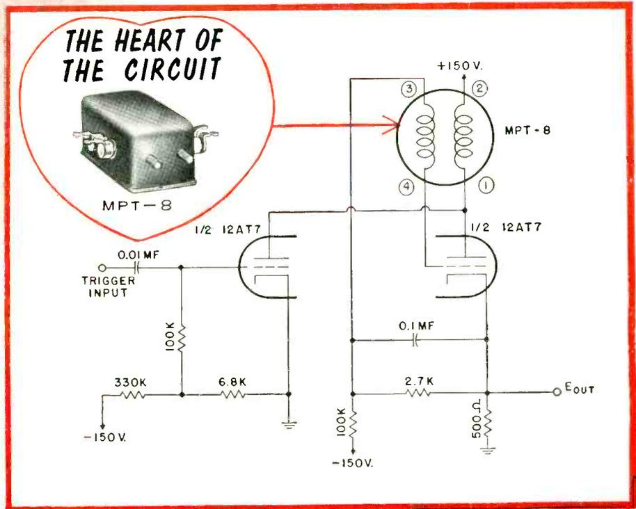
**HERMETICALLY SEALED PULSE TRANSFORMERS** for use in blocking oscillators, low level interstage coupling, and modulator outputs. Made in accordance with MIL-T-27 specifications. These pulse transformers are designed for maximum power, efficiency and optimum pulse performance. Balanced coil structures permit series or parallel connection of windings for turn ratios other than unity. Pulse characteristics, voltages and impedance levels will depend upon interconnections made.
