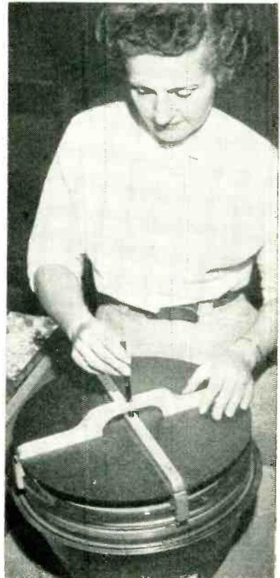
Marking center of picture tube by rotating crayon in centering fixture
