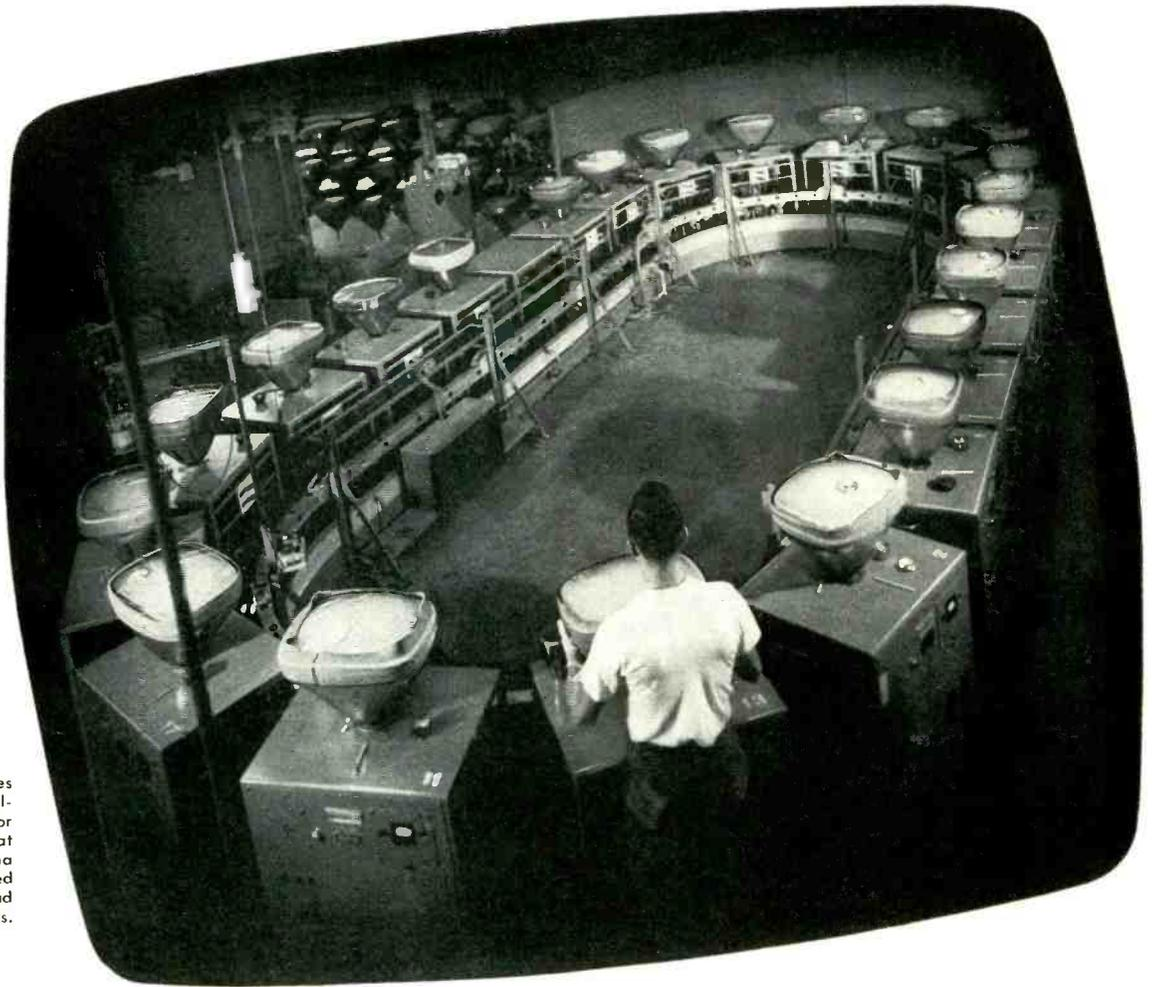
Overall view of Stokes continuous vacuum metalizing dolly system for aluminizing TV tubes at RCA's Marion, Indiana plant. Operator is required only to load and unload tubes from the 22 carts.
