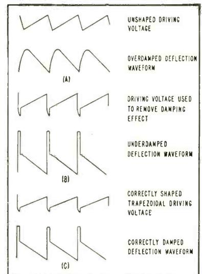
FIG. 2—Driving-voltage waveforms and deflection-voltage waveforms showing effects of overdamping (A), underdamping (B) and correct damping (C)
