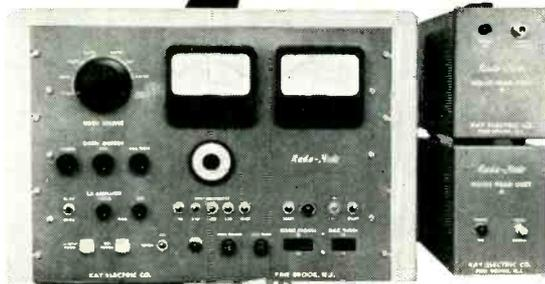
There's a Kay instrument to answer most needs in noise testing—with good measure! Each *Mega-Node* type affords accurate measurement of noise figure and receiver gain in a specific frequency range, while the *Rada-Node* can be obtained with all elements required for complete noise figure measurement, 5 mc to 26,500 mc, including power supplies. Thus you may trust your noise test work to one precision line of uniform high quality.
