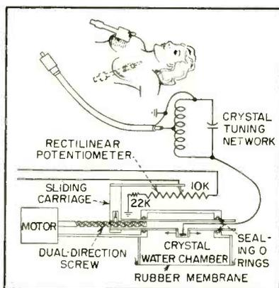
FIG. 1—Composite view of body-surface scanning crystal applicator. Sketch at top shows how the instrument is applied to the breast
