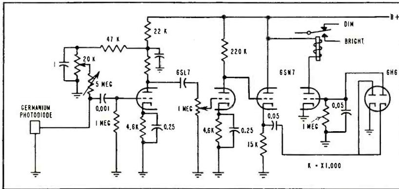
FIG. 7—Method of providing required amplification for photodiode
