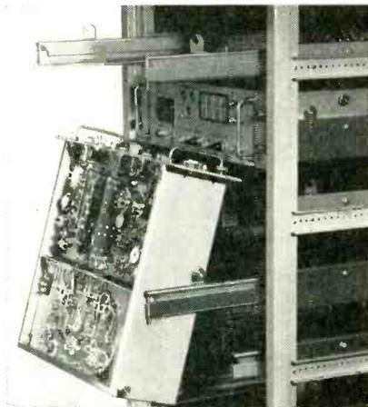
bronze rollers, stainless steel pins and nylon bushings. The finish on the steel parts is Iridite on cadmium per Federal Spec. QQ-P-416, Type H, Class C. Weight of the Slides and associated hardware is 6 pounds.
