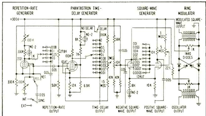
Target simulator combines repetition-rate, time-delay and square-wave generators in one unit. Neon lamps show if circuits are operating
