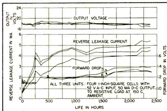
FIG. 3—Life test data on three developmental selenium rectifiers (Bradley Laboratories, Inc.)
