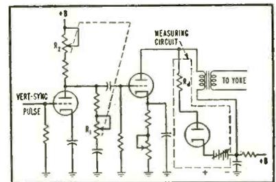
FIG 3—Circuit for automatic damping of vertical-deflection waveform. Diode circuit has been added for the purpose of making dynamic measurements
