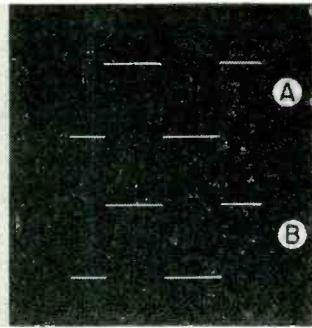
FIG. 6—Square wave of 15-kc frequency shows no impairment through amplifier
