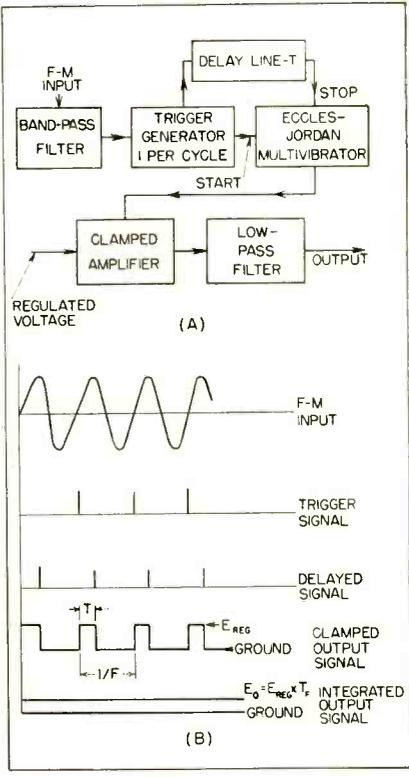
FIG. 3—Final form of f-m discriminator (A) using band-pass filter and trigger generator to start multivibrator. Pertinent waveforms at (B)
