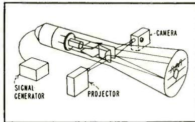
Optical images can be projected through the neck of a crt and reflected onto the inner surface of the tube face. One mirror can be used in photographing the resultant display
