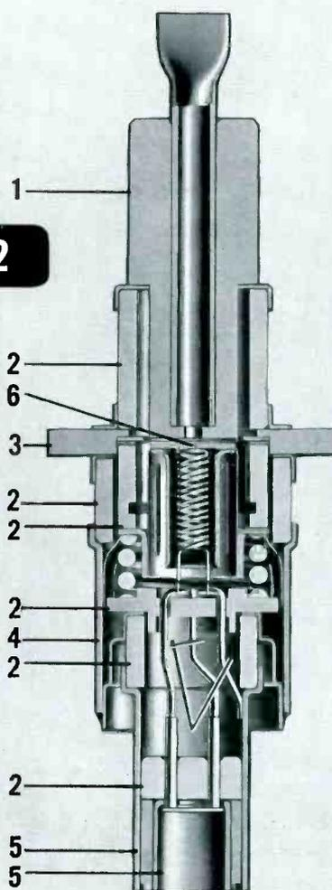
**1. PLATE TERMINAL** has exceptionally large area, for good electrical conduction and proper cooling. Extra length is a plus in the case of many tuning mechanisms. Surface is silver-plated—as are all GL-6442 terminals—for high conductivity.
