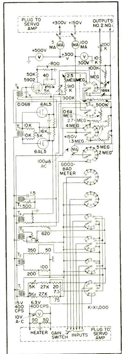
FIG. 2—When amplifier under test is plugged in, its terminals automatically make contact with plug terminals at top and bottom of circuit. Ten-deck, eleven-position selector switch is then swung through its positions while watching good-bad scale of microammeter
