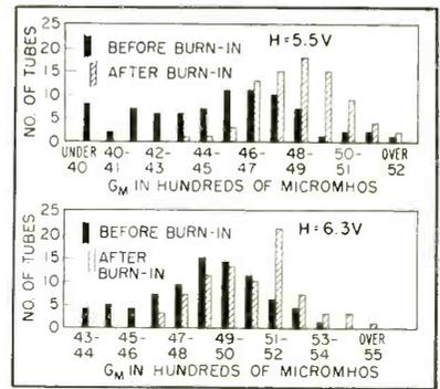
Effect of burn-in on two batches of type 5702WA tubes, using different heater voltages
