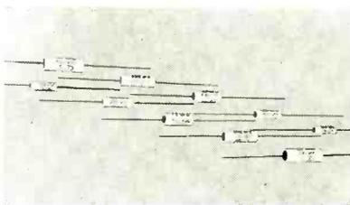
The new Midgets range in size from  $\frac{7}{32}$  in. in diameter and  $\frac{11}{16}$  in. in length to  $\frac{3}{8}$  in. diameter and  $1\frac{1}{8}$  in. length. Those rated up to 400 v d-c are impregnated in HT compound and have an operating temperature range from  $-40$  C to  $+90$  C while those rated at 600 v d-c are impregnated in Vikane and have an operating temperature from  $-55$  C to  $+100$  C.
