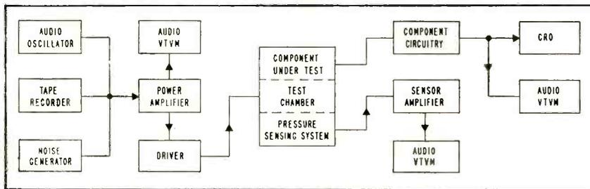
FIG. 2—High-intensity-sound test chamber and associated driving, sensing and monitoring equipment used for testing components
