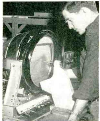
Centering picture tube on chassis by lining up crayon mark with centering plunger
