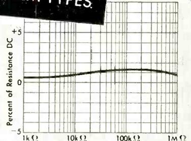
Load Life Test in MIL-R-11A allows maximum resistance change of 10%.
