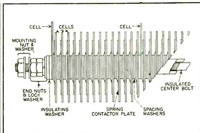
FIG. 4—Typical selenium rectifier assembly (Fansteel Metallurgical Corp.)
