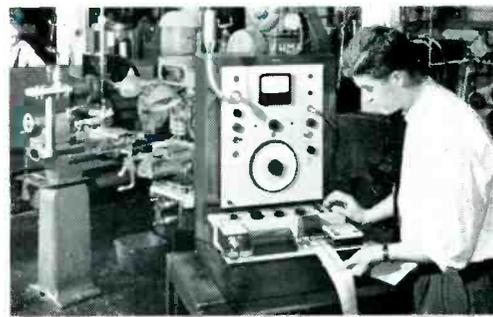
Third-Octave Spectrum Recorder provides a complete, self-contained system for noise analysis and recording—no extras to buy. Precision microphone and microphone calibration apparatus available. System automatically scans and plots sounds from 35 cycles to 18,000 cycles per second in  $\frac{1}{3}$  octave steps.
