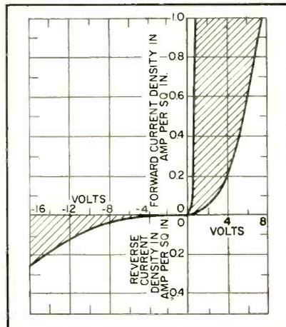
FIG. 14—Effect of temperature on titanium-dioxide cells. Shading shows range.
