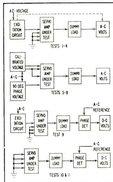
FIG. 1—Block diagrams of test circuits
