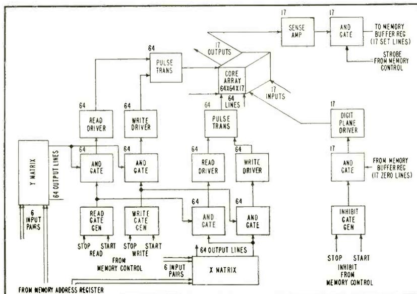
FIG. 1—Magnetic-core memory gives arbitrary or random access to any one of its registers every 6 microseconds
