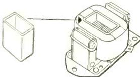
**Coil forms** for this solenoid have to operate at high temperature . . . an ideal application for Taylor Glass Melamine Laminate.
