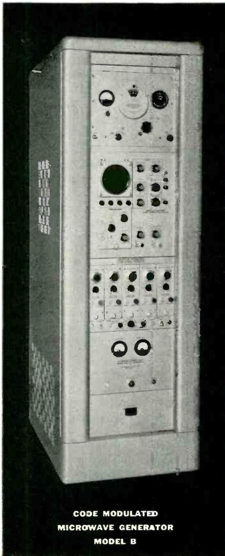
**Four Interchangeable Microwave Oscillator Units**—each with single control direct reading dial... cover the range 1000 to 10,750 mcs... constructed with precision power monitor circuit to maintain 1 mw power output reference level... keying circuit assures rapid rise time of modulated RF output... employs non-contacting chokes... built-in RF detector... can be modulated externally.
