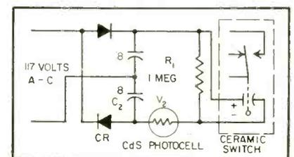
FIG. 1—Fast-acting photoelectric circuit requiring no amplification
