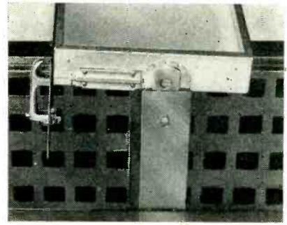
can be serviced while in the rack. Chassis-Trak is available in two variants: type CTD is provided with a tilt-lock detent mechanism locking at 30-deg intervals of rotation from -90 deg to +120 deg; type CTB tilts back to +120 deg for underside servicing. With either type the chassis may be easily released from the slides for removal by means of a finger-tip control.
