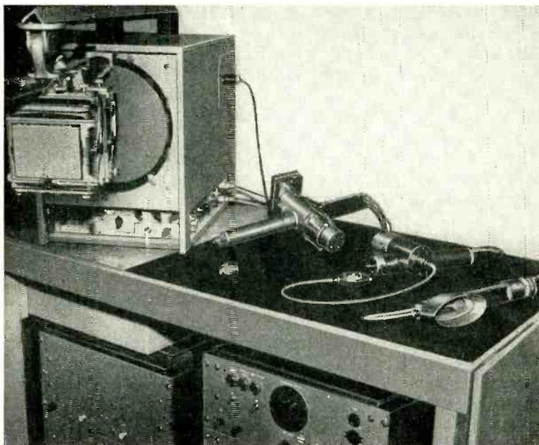
New electronic equipment used for cancer detection. Left to right: cathode-ray display unit and camera; vaginal sector-scanning crystal applicator with tip removed to show crystal mounting; ppi bowel-scanning crystal applicator; body surface scanning crystal applicator of type shown on the cover
