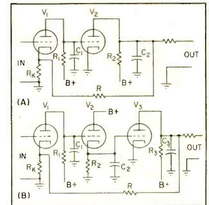
FIG. 1—Development of negative feedback amplifier with two low-pass sections (A) and three-section circuit (B)
