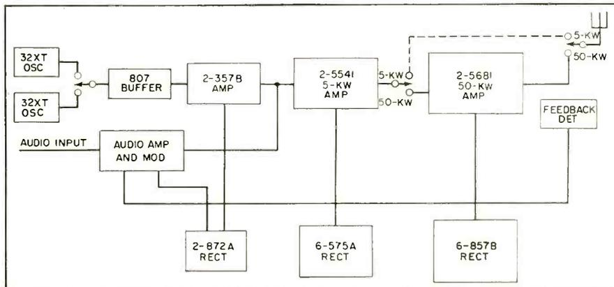
FIG. 2—Complete 50-kw transmitter, showing power switchover provisions for daytime and nighttime operation
