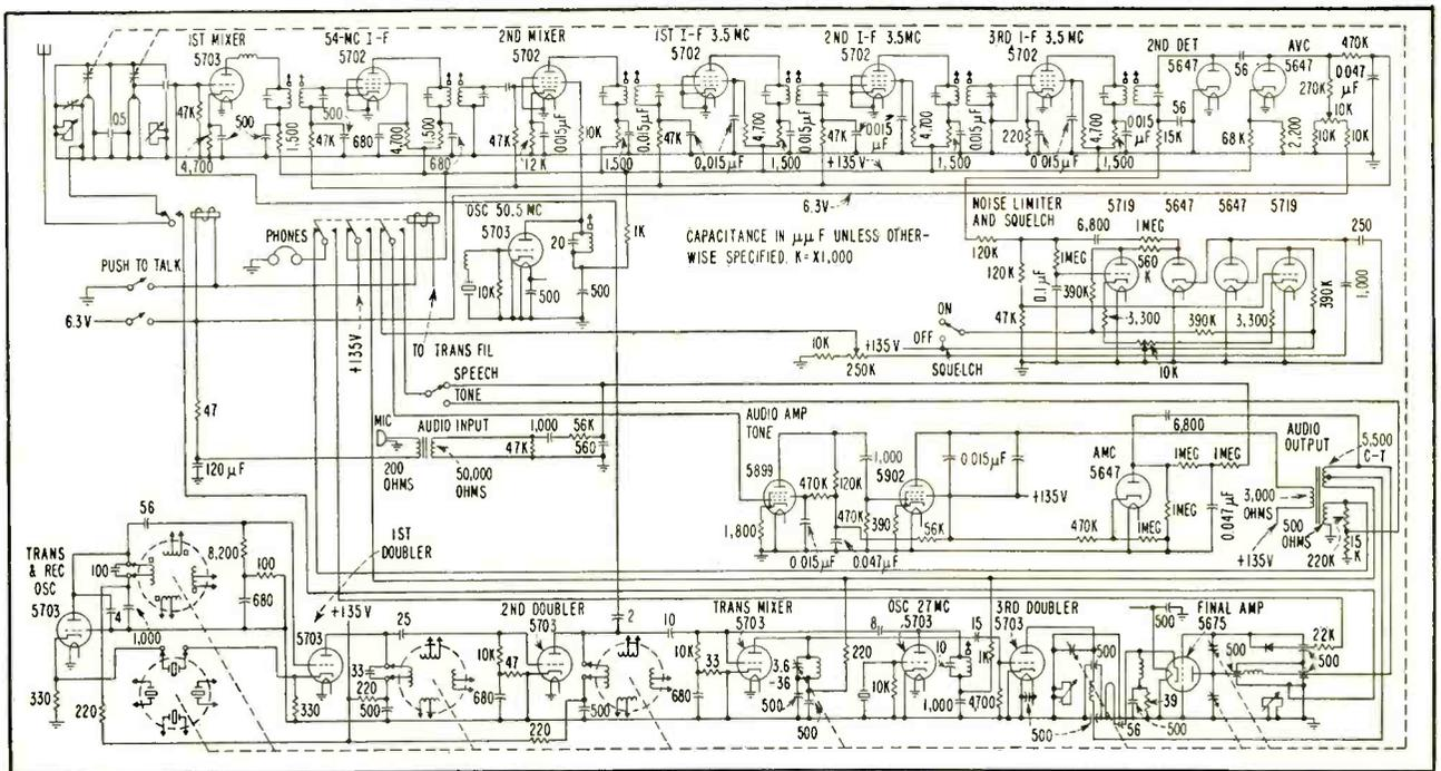
FIG. 2—Complete circuit, with plug-in connectors omitted for simplicity. Dashed lines connect all units mechanically ganged to crystal selector switch (lower left) for automatic tuning
