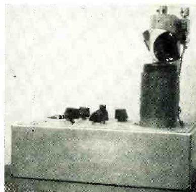
Experimental model of scanner-type dimmer using optical system of Fig. 1
