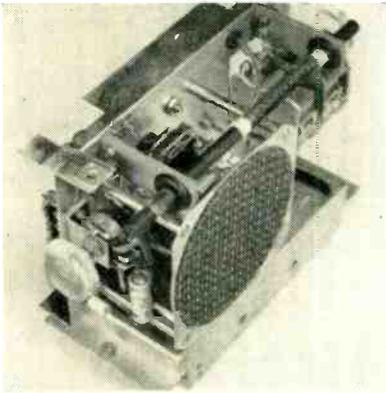
Top view of laboratory model showing ferrite rod antenna and output transformer, located behind loudspeaker
