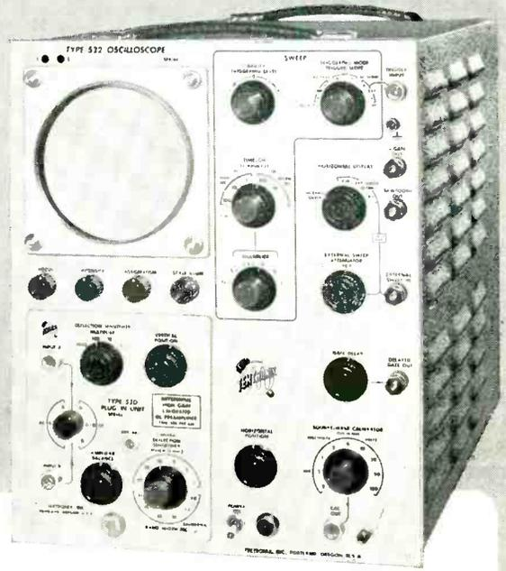
This new oscilloscope offers the advantages of all six Type 53 Plug-In Units now available — plus those yet to come. Only the wide-band units are limited by its dc-to-5 mc response. Wide sweep range (0.2  $\mu$ sec/cm to 12 sec/cm) and 4-kv accelerating potential complement the signal-handling versatility of the Type 532... resulting in performance characteristics desirable for a great many laboratory applications.
