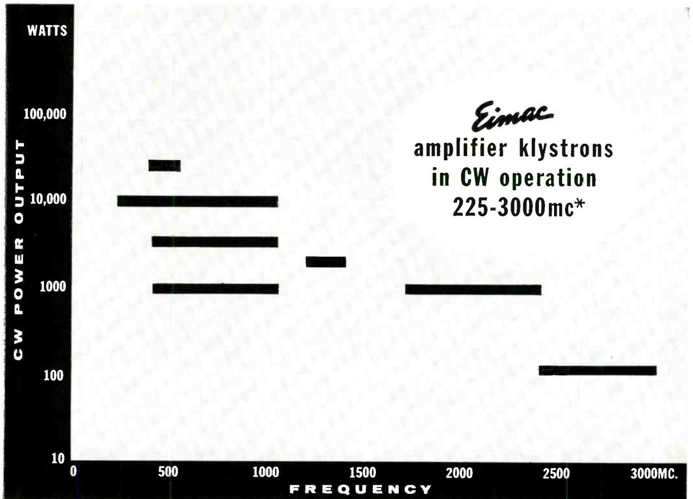
\*Pulse ratings many times CW ratings are available on most Eimac klystrons.
