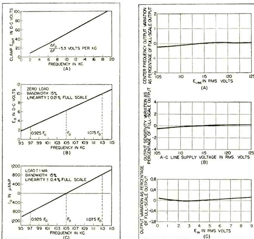
FIG. 4—Linearity characteristics for wide-band operation (A), telemetering band voltage output (B) and current output (C)
