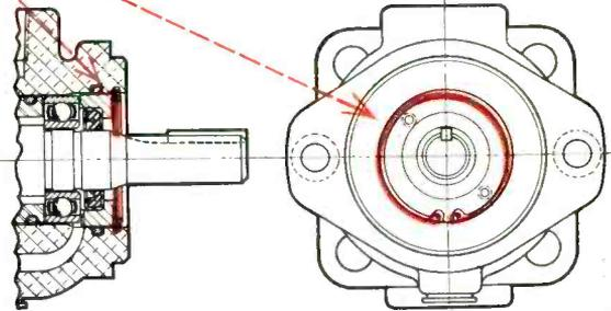
**Truarc Way:** Waldes Truarc beveled retaining ring (internal 5002) retains shaft and bearings, takes up accumulated tolerances rigidly, prevents leakage around shaft. Unit is one pound lighter. Assembly is quick and easy, more economical.
