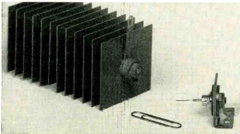
FIG. 13—Relative sizes of silicon junction rectifier (right) and conventional selenium rectifier having the same power-handling capacity
