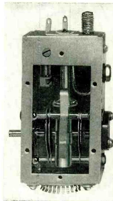
Transmitter tuning cavity, with pulley shaft projecting at left
