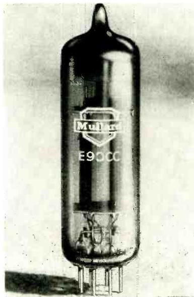
than 10 v. The E90CC is on a miniature all-glass base. It has a heater rating of 6.3 v, 0.4 ampere and an anode dissipation of 2 w per anode.
