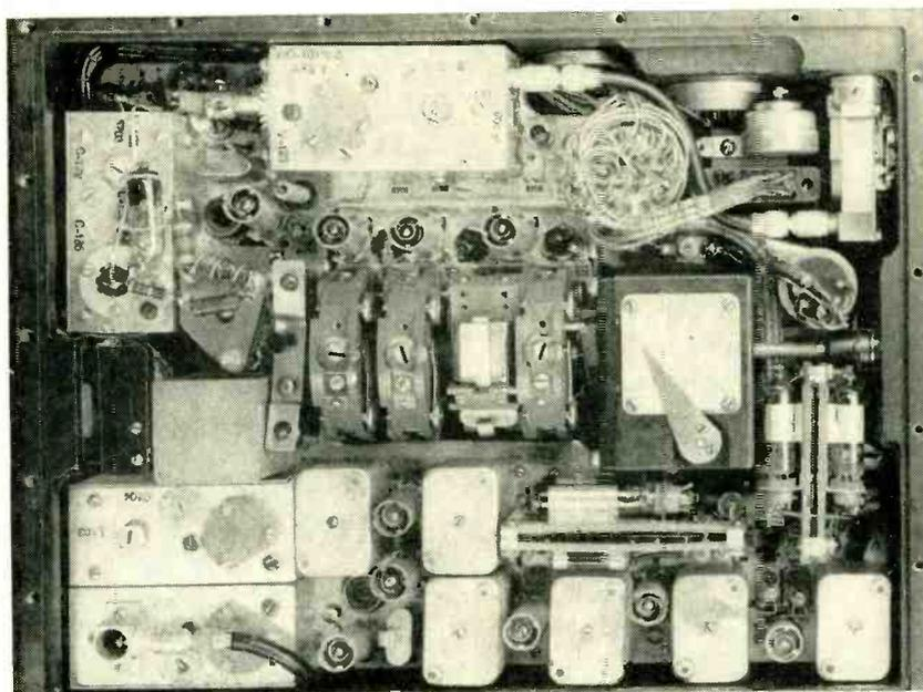
Interior of receiver-transmitter, showing coil and crystal turrets at center. Tuning cavities are at top and at lower left. Set has 23 tubes
