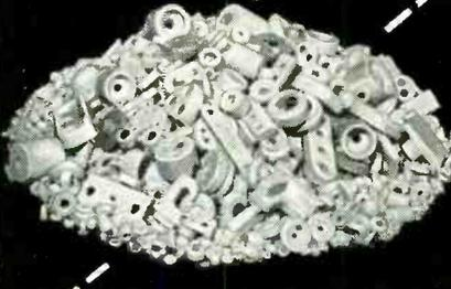
... about Star's fabricating facilities for producing small electrical porcelain parts. There is practically no limit to the variety of shapes we can turn out to meet your simple or intricate specifications precisely ... economically. More than 25 automatic presses, operating 24 hours a day are available to turn out millions of small parts. This means lower cost to you ... faster service. Write for the 26-page Star catalog describing this service, Star materials and engineering data.
