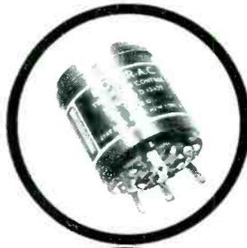
**D-13430 Motor-AC:** 2 phase control; 115 volts; 400 cycle single phase; no load speed 4800 rpm; stalled torque 1.45" oz; weight 8 oz; length 1 1/2"; OD 1 1/2"; Ke-toy Mfg. Corp. **\$22.50 each**
