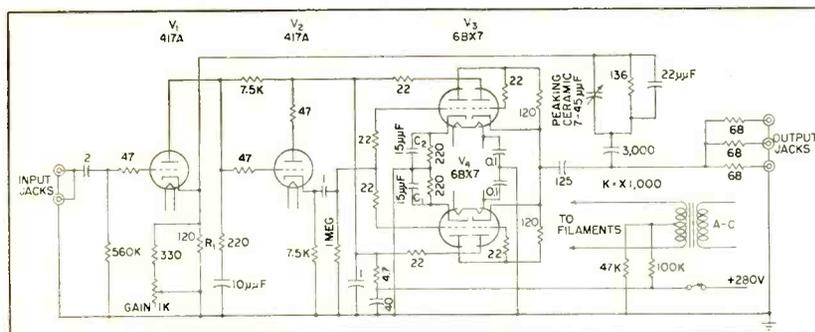
FIG. 2—Operating version of video distribution amplifier includes special bootstrap output stage further explained in Fig. 3
