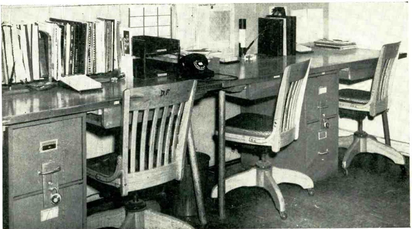
Inexpensive engineering-department desks made from doors, dowel rods and filing cabinets have added advantage of keeping confidential material within reach while meeting security requirements. Note use of simple metal plate and hasp for locking two-drawer files
