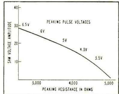
FIG. 6—Peaking resistance for optimum damping plotted against sawtooth amplitude
