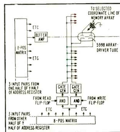
FIG. 8—Efficient  $8 \times 8$  rearrangement of the array-drivers for one coordinate
