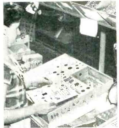
Placing subassembly chassis plate in position on main color receiver chassis resting in special wood pallet
