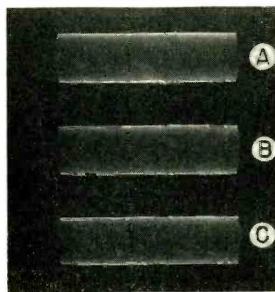
FIG. 10—Differential gain test signal through amplifier and high-pass filter at amplitude of 1.5 volt, peak-to-peak. Duty cycles of 10 (A) 50 (B) and 90 percent (C)
