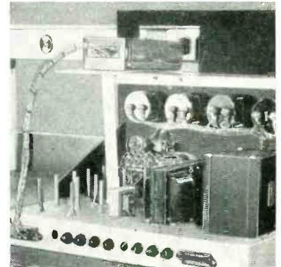
Rear of tester, showing plug and cable at upper left for making connections automatically to amplifier under test
