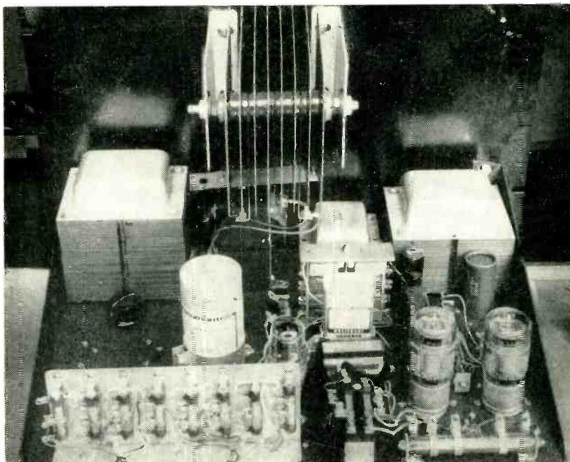
Prototype chassis for automatic program control of mass production machines. No error amplifier tubes are used because of the sensitivity of the phase-shifting circuit
