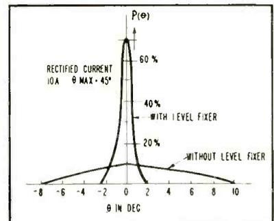
FIG. 3—Range of ignition phasing with and without level fixer
