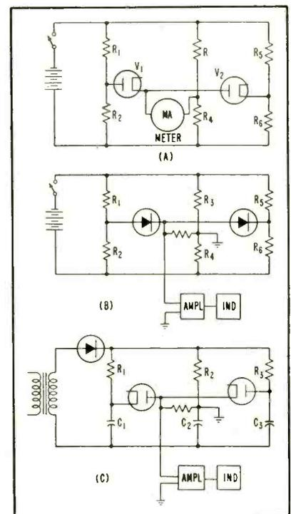
FIG. 3—Basic comparison circuit (A) and modifications (B) and (C)
