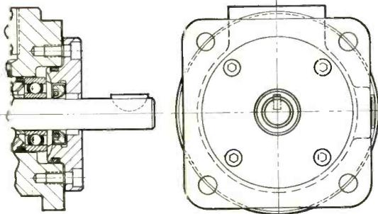
**Experimental Way:** One cast retainer plate plus four socket head cap screws hold unit together. Assembly requires skilled labor, machinery, time-consuming careful adjustment.
