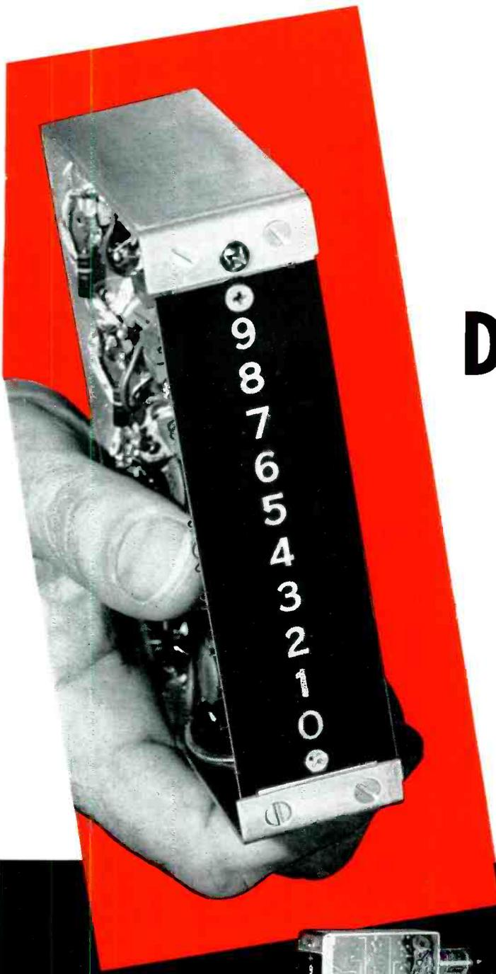
Counter with new printed circuit designs is compact, requires only 1.2 watts. Counter generates one output pulse for each ten input pulses.
