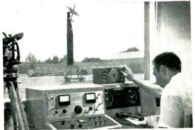
**Electronics Research Engineer Irving Aine** records radiation antenna patterns. Twenty-two foot plastic tower in background eliminates ground reflections, approximates free space. Tower is of Lockheed design, as are pattern integrator, high gain amplifier, square root amplifier, logarithmic amplifier.
