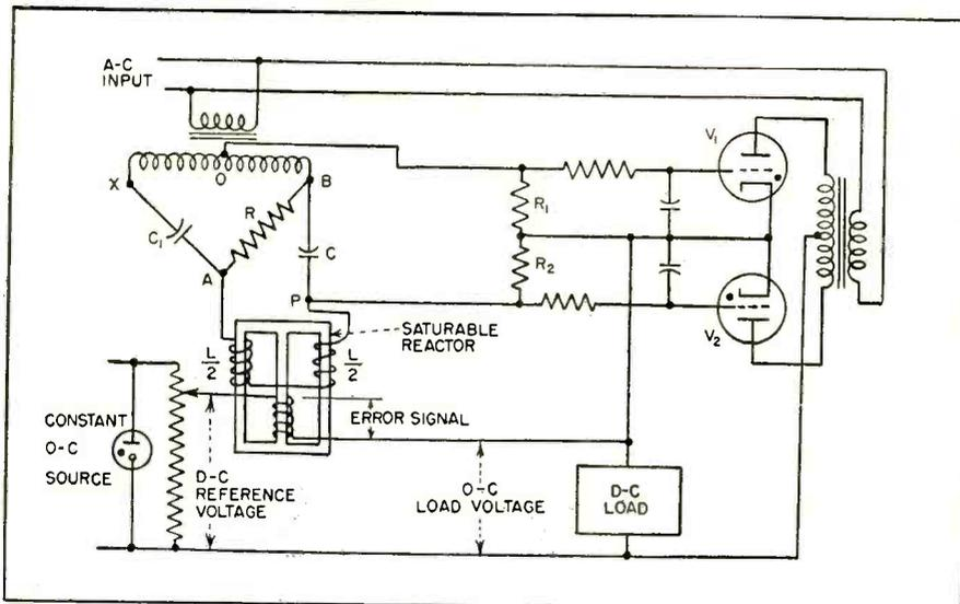
FIG. 7—Negative-feedback circuit delivers constant voltage to d-c load from full-wave thyatron rectifier
