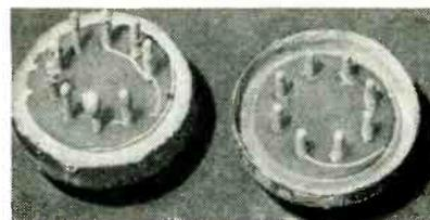
Headers with similar crack patterns on both surfaces. Note lack of coincidence
