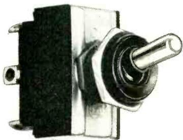
SEALNUTS serve dual function of mounting and sealing electrical switches. Twelve stock styles fit most toggle, rotary and push-button types. They provide rigid, metal-to-metal contact with panel for secure mounting, while Silicone sleeve and O-ring seal against external pressures to 200 lbs./in<sup>2</sup>, stay flexible at -65°C, meet requirements of MIL-B-5423.
