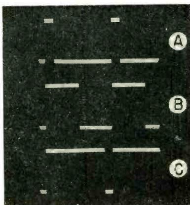
FIG. 8—Differential gain with 10-percent duty cycle (A) 50 percent (B) and 90 percent (C)
