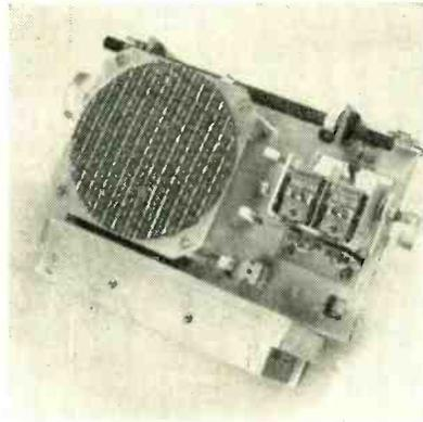
Front of set. Transistors are mounted on chassis between loudspeaker and tuning capacitor
