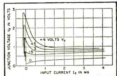
FIG. 2—Input characteristic of a double-base diode
