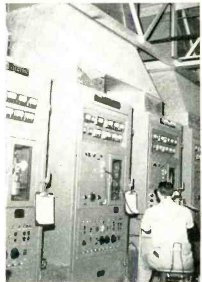
Four of the 64 hydrogen thyratron test sets from which hot exhaust air is ducted into building's heating system
