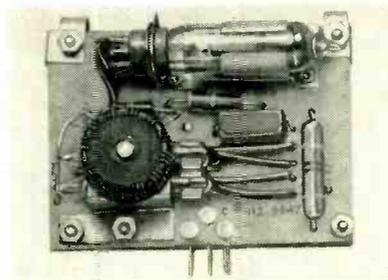
Plug-in panels produced by dip-soldering for squelch circuit (left) and a-f amplifier
