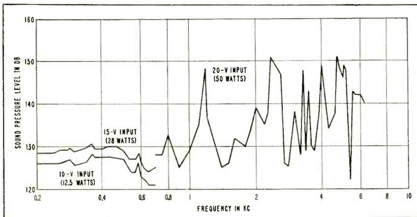
FIG. 3—Sound pressure levels in test chamber at different frequencies for constant voltage inputs. Reference level of 0-db is taken at  $2 \times 10^{-4}$  dynes per sq cm
