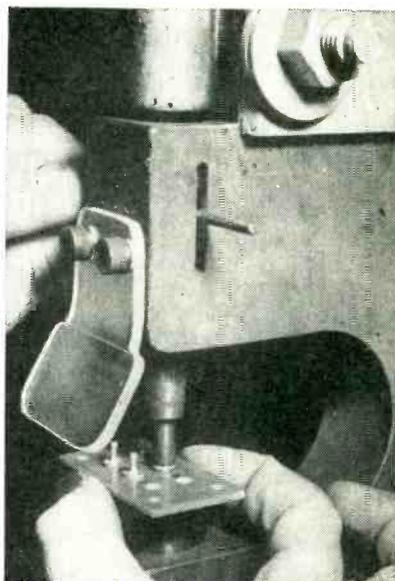
Operating the manual riveter. Protruding rod moves upper die down against light spring action. Operator inserts terminal in board, brings board into upper jaw as shown, then pulls down jaw with left hand to insure that terminal seats perfectly. Pressing foot pedal then pulls down cable attached to actuating air valve of riveter
