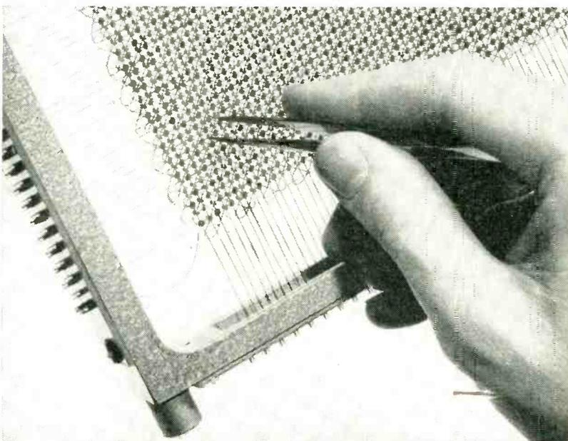
Closeup view of the plane. Four lines pass through each core, one each for  $x$ ,  $y$ , digit (parallel to  $x$ ) and sense (diagonal)
