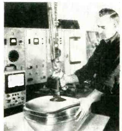
Lowering picture tube into shipping carton after completion of final tests
