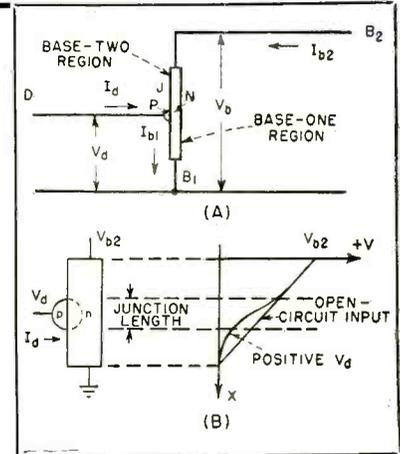
FIG. 1—Double-base diode construction (A) and potential through bar (B)
