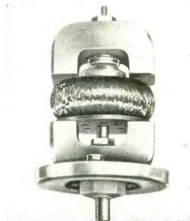
range for any individual Rotoroid is from 50 to 150 percent of the nominal value. Inductance variation in the Rotoroid is obtained by the rotation of one of a pair of permanent magnets placed on apposite sides of the winding. As a result, no external d-c power is required for biasing, the inductance variation with rotation of the control knob is nearly linear, and high Q and low harmonic distortion are preserved even with extreme variation of inductance.
