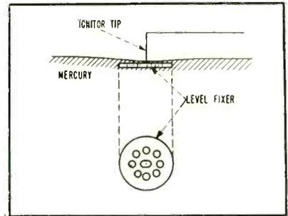
FIG. 2—Level fixing unit in mercury pool eliminates timing changes resulting from variation in mercury level
