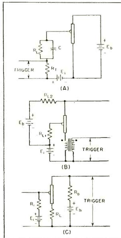
FIG. 8—Variations of double-base diode switching circuits showing junction-triggered type (A) base-one triggered (B) and base-two triggered (C)
