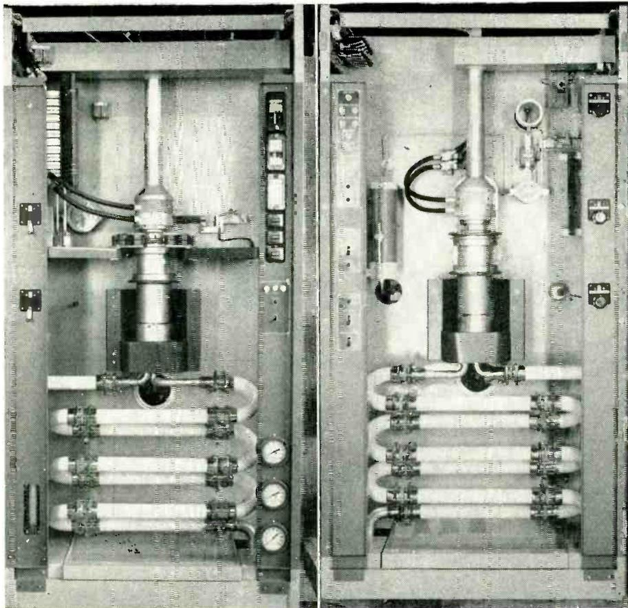
Fifty-kilowatt final amplifier. Closeup view of carrier amplifier shows grounded-grid arrangement (left). Peak amplifier is shown at right
