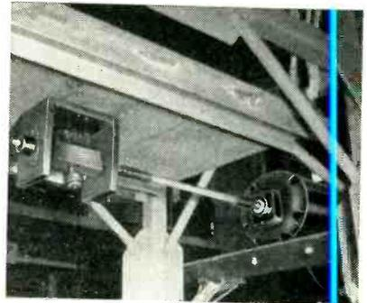
Bottom view of shake table, showing bearing supports for eccentric weight and method of extending motor shaft to drive the weight
