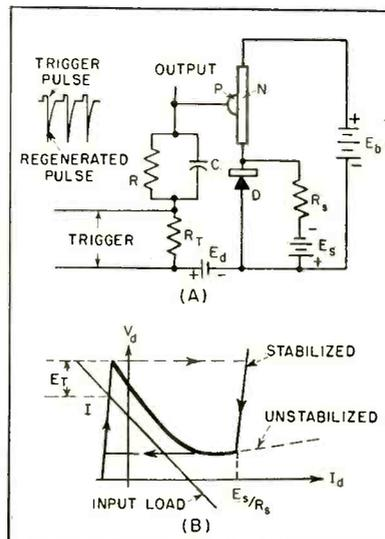
FIG. 5—Regenerative-pulse amplifier circuit (A) and input characteristic of amplifier (B)
