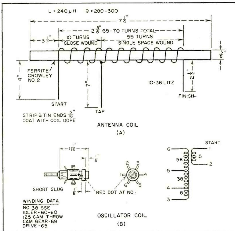
FIG. 2—Winding data for antenna (A) and oscillator (B) coils. Other components are available commercially
