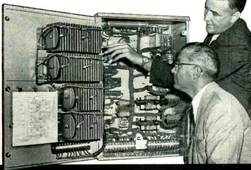
*Mr. Dornhoefer (upper right) inspects current production of magnetic amplifier regulator with Mr. J. F. Hysler. Rating of the motor generator set it regulates:*
