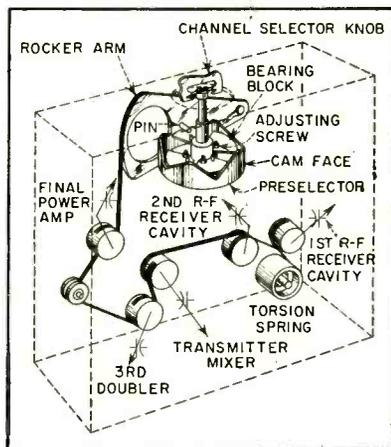
FIG. 4—Method of linking all tunable controls with the four-position channel selector knob for automatic tuning
