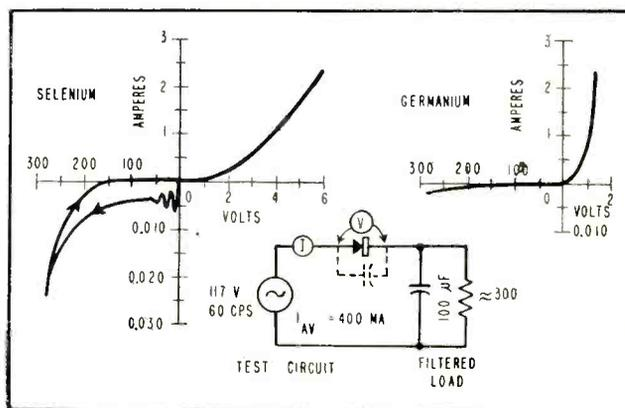
FIG. 11—Volt-ampere characteristics of selenium rectifier and equivalent germanium rectifier (Transistor Products, Inc.)
