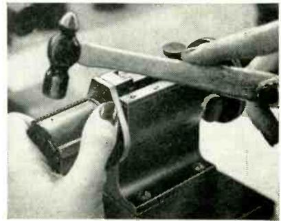
Tapping first drive pin into housing to anchor far end of coil
