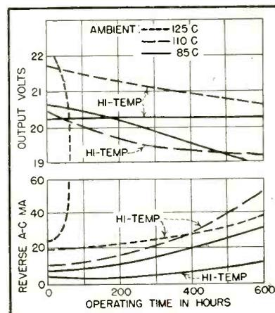
FIG. 5—Comparison of conventional selenium rectifier (unlabeled curves) and high-temperature selenium rectifier in single-phase bridge circuit with 26 v rms input and 1 ampere d-c output (Radio Receptor Co.)
