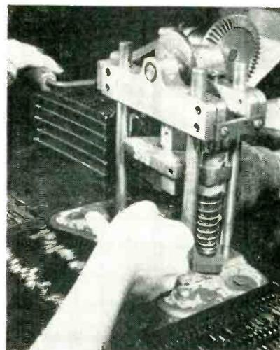
Forming anvil containing grid is held in position on bed of press with right hand while operator brings down crank with left hand
