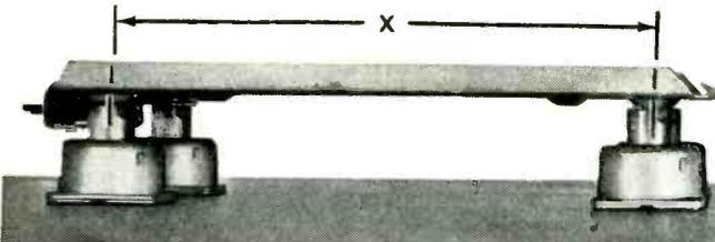
*Excessive height required. Unit mount bulk imposes reduced spacing (X) between support centers, resulting in impaired stability (critical in lateral direction). Greater sway space required.*
