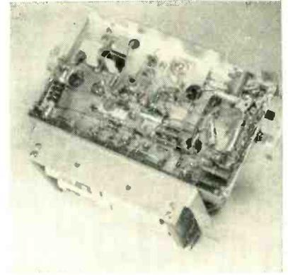
Rear of chassis showing interconnecting wiring. Flashlight batteries are mounted below case
