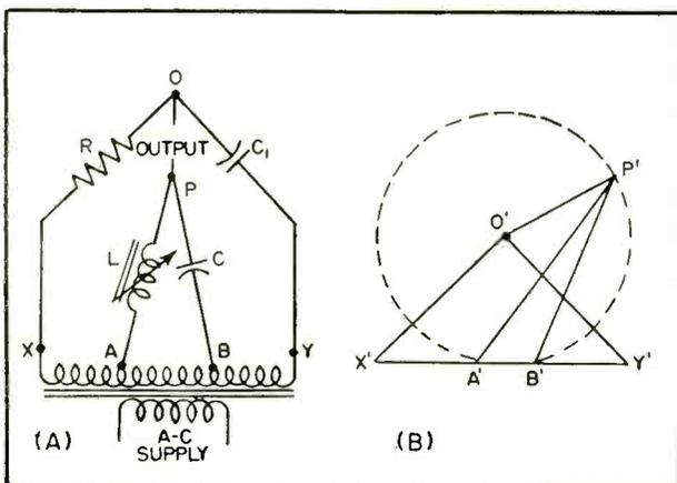
**FIG. 3—Circuit for transmitter phase-modulator applications**
