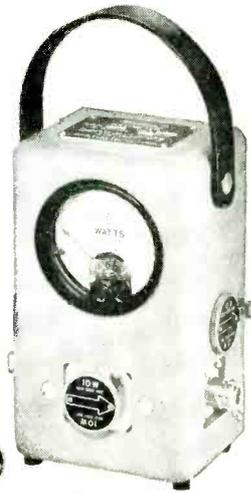
Model 43 with front element in operating position. Dimensions: 7" x 4" x 3" Weight, 4 pounds. SO239 jacks for PL259 plugs available.
