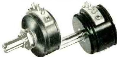
Four watts continuous at 80° C. Resistances 10 to 100,000 ohms. Diameter 1-1/8 in., depth 1/2 in. Weight is less than 3/4 ounce.
