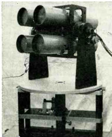
Multiple photoelectric photometer used to measure and record night airglow. Colored filters in each telescope allow various light frequencies to be observed
