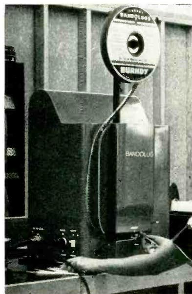
minals. The reel may be changed in seconds and the Bandolug belt rapidly guided into the universal die set. The operator merely depresses the single control and feeds stripped wire into the lug barrel. As fast as the machine is fed, an electrical device activates the compression dies and a complete terminal installation is made.
