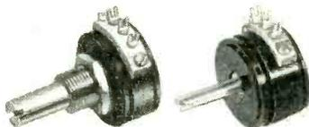
Precision wire-wound construction. Three watts continuous at 80° C. Resistances 10 to 50,000 ohms. Diameter 7/8 in., depth is 3/8 in. Weight is only 1/2 ounce. Independent linearity 3% standard.
