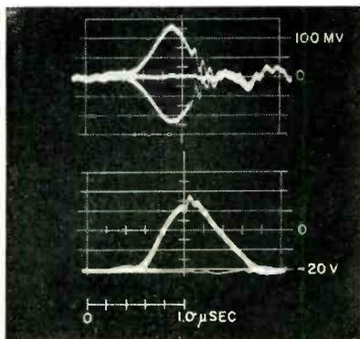
FIG. 5—Digit-plane output (upper), and pulse fed into gate tube after amplification and rectification (lower)
