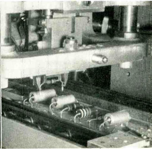
Resistor-inserting position, showing how conical sleeves on leads are pushed into panel holes (Continued on page 10)
