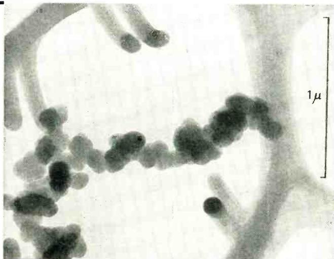
Holes in collodion film and attached smoke particles at a magnification of 22,000 times ( $1\mu$  equals 2.5 inch in original half-tone)
