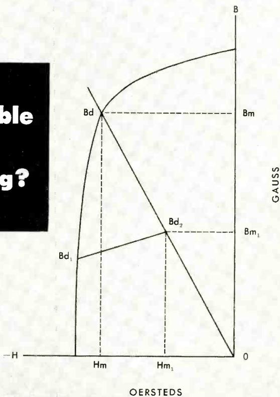
A closed circuit magnet exists when the magnet is magnetized in its assembly of soft iron or other magnetic materials and is not removed later. Normally, there is a specified air gap. The chart illustrates the demagnetization curve for Alnico permanent magnet material.
