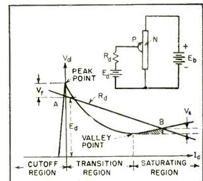
FIG. 3—Three regions are obtained from experimental input characteristic
