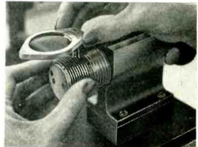
As first step, coil is threaded onto drum while gate is held out of way
