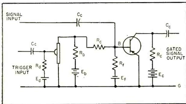
FIG. 9—Gating circuit employs double-base diode to gate transistors
