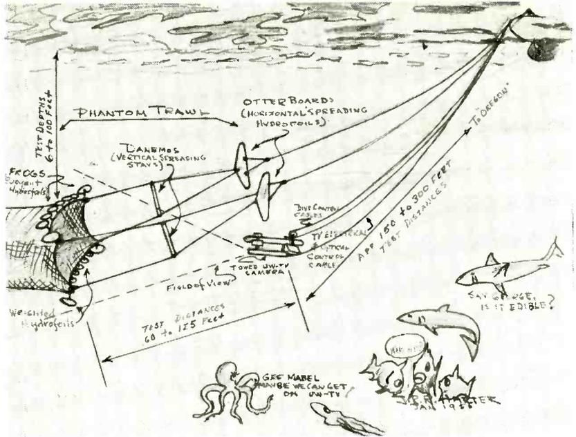
Electronics and Experimental Diving Groups at BuShips used tv and fishing equipment shown above for rating nets (see p 26). We have added "frogs", "danemos" and "otter boards" to our lexicon
