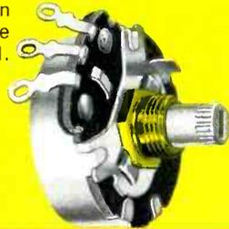
Concentric shaft tandem control with conventional bushing mounting. Designed for front panel dual knob applications, such as contrast and volume. Available in various combinations of composition or wirewound front and rear sections with or without on-off switch attached to rear section. CTS type GC-C252-45 with wirewound front section, composition rear section and on-off switch illustrated.
