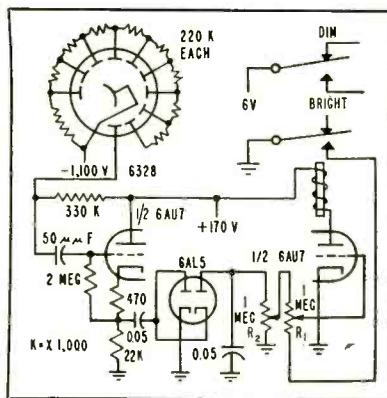
FIG. 2—Circuit uses special automotive type multiplier phototube
