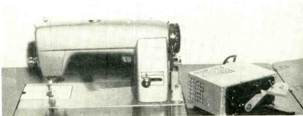
New phase-shifting circuit reduces size of motor control circuit (in box) used to vary speed of sewing machine. Control circuit uses inductance-capacitance combination instead of conventional carbon pile
