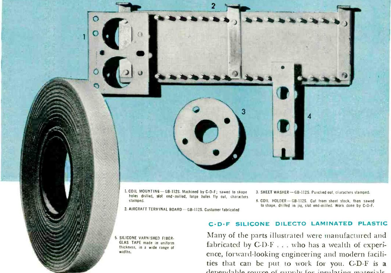
1. COIL MOUNTING—GB-112S. Machined by C-D-F; sawed to shape holes drilled, slot end-milled, large holes fly cut, characters stamped.
