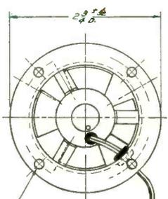
(4) 5/32" DIA. HOLES EQUALLY SPACED ON 2-3/8" DIA.
