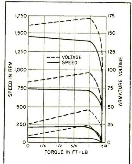
FIG. 8—Regulation curves for shunt-motor controlled by circuit of Fig. 7
