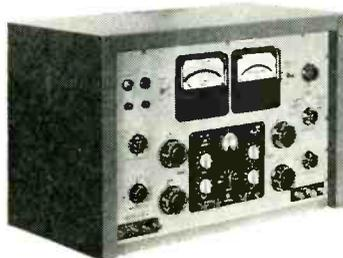
Compact cabinet contains power supply, standard meters, Wheatstone Bridge and all circuits for quick, convenient instrument calibration to 0.5% accuracy by non-technical personnel.
