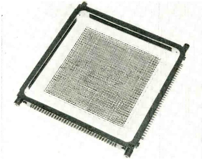
Completed core-memory digit plane with the 4,096 cores spaced on 0.1-inch centers. Overall dimensions of the plane are about  $10 \times 10 \times \frac{3}{4}$  inches. Memory employs simultaneous excitation of  $x$  and  $y$  coordinates, a 2-beat cycle and the principle of sampling of the output signal
