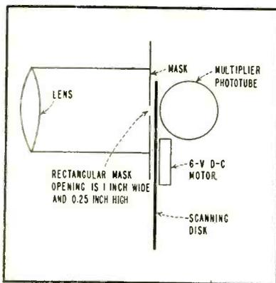
FIG. 1—Simplest optical arrangement of scanner-type dimmer
