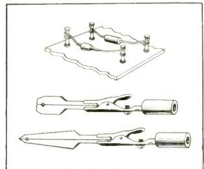
GERMANIUM and silicon crystal diodes often require special care in assembly to prevent damage to sensitive elements. When soldering is required, allow extra lead length for strain relief, and use heat-dissipating clamps on leads to prevent
