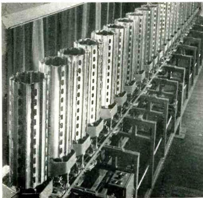
Autofab 24-head machine delivers complete panels at lower left, ready for dip-soldering
