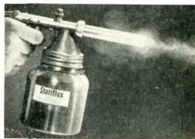
Positively charged powder being blown from special gun
