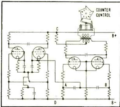
FIG. 4—High-speed counting and collecting device uses make-and-break contact as shown
