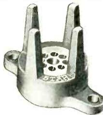
Stainless steel #303 insert permits close tolerances between holes of pin circle and angular spacings. Holes counter bored for easy insertion of tube pins, minimizing strain on glass tube button.
