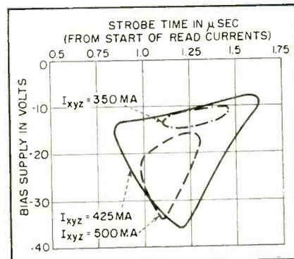
FIG. 7—Failure bias bounds in sense gates as a function of the sample or strobe time
