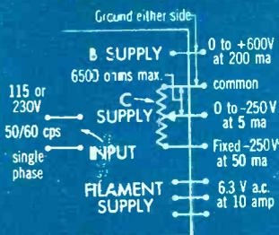
Flexible ground permits stacking of supplies to provide up to  $-600V$ . cathode voltage and an additional C to  $-250V$ . for the reflector of low voltage klystrons.
