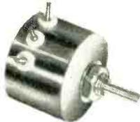
Designed for high-temperature use. Dissipates one watt at 200° C. Dissipates five watts at 80° C. Resistances 1,000 to 25,000 ohms. Stainless steel case, one inch dia. by 1 1/16 in. depth behind panel. Teflon-insulated terminals.
