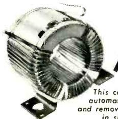
*This coil is set-up, automatically wound, and removed from machine in six minutes.*
