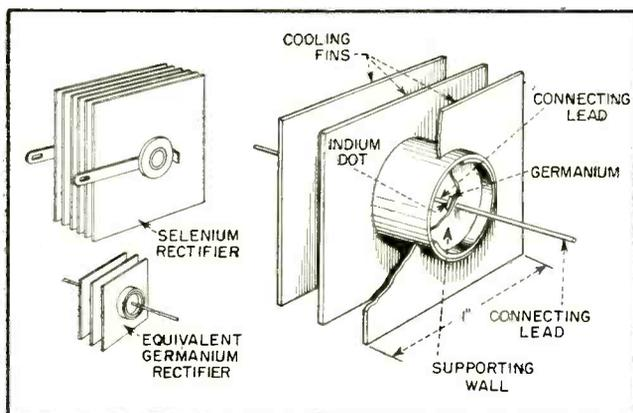
FIG. 10—Construction of germanium power rectifier (Transistor Products, Inc.) and comparison with equivalent selenium unit
