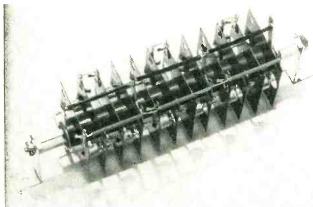
FIG. 7—Stacked germanium rectifiers on radiating fins, rated 70 v rms input per cell and 0.5 amp d-c output to resistive load
