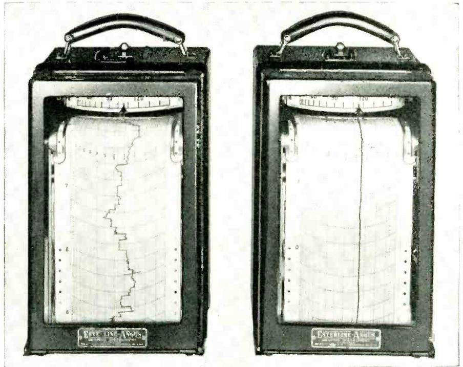
**TYPICAL EXAMPLE OF SOLA VOLTAGE REGULATING ACTION.** The recording on the left represents a fairly common condition of voltage fluctuation on a 115v line. The chart on the right
