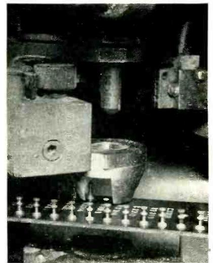
Riveting head in position. Terminal was previously dropped into conical lower member where it is held by spring in upright position until die descends
