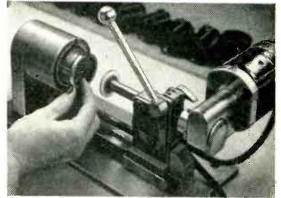
Motor-driven fixture uses grooved nylon wheel to press turns of coil outward for firm seating in internal spiral grooves of housing
