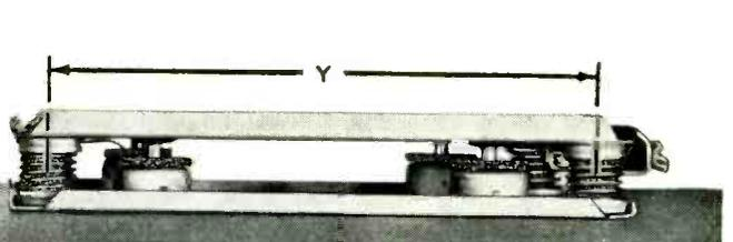
*Note reduction in mounting height. Important space saved. Maximum spacing (Y) of resilient elements at extreme corners provides stability. Less sway space required.*
