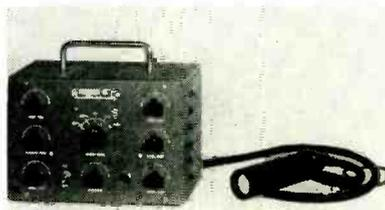
complete scopes on the market. It measures 6 in. high, 9 in. long, 5 in. deep, taking up less than half a sq ft on the bench and weighs only 7½ lb. The Probe-Scope has a 1-in. Mumetal shielded crt incorporated into a probe small enough to be held in the palm of a hand, yet the waveform is even sharper and clearer than on larger oscilloscopes.
