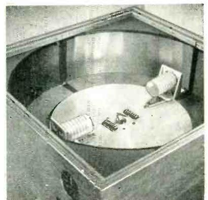
Method of mounting two eight-potentiometer units on turntable
