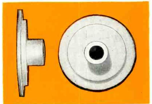
As operating temperatures rise, melamine laminated plastics can satisfy many requirements for component parts. Glass base melamine grades of Dilecto resist elevated temperatures — up to 300° F. continuously, 350° F. intermittently. They have extremely high impact strength; excellent arc resistance and self-extinguishing properties. C-D-F melamine Dilecto grades are usually specified for many electrical applications requiring high arc resistance, mechanical strength, flame and heat resistance.
