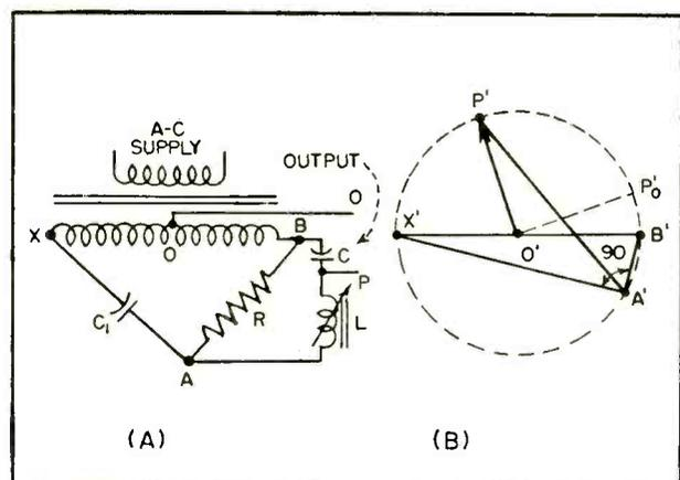
**FIG. 4—Thyatron control circuit is fail-safe**
