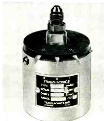
The Trans-Sonics® Baroresistor is a rugged pressure actuated potentiometer designed and field tested for use in operational aircraft. This pressure transmitter provides a simple and reliable means of varying fire control equipment and autopilot performance as a function of pressure (altitude).
