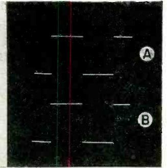
FIG. 7—Sixty-cycle square wave has minor tilt (oscilloscope is reversed)
