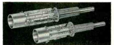
Size Comparison of Color TV Guns. Note how much more compact gun can be with miniature disc cathodes. Permits more slender tube neck.
