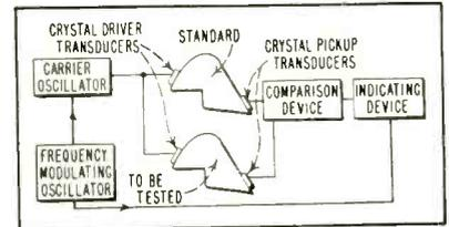
FIG. 1—Standard and part tested are excited by ultrasonic signal and reflected characteristics compared
