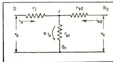
FIG. 6—Equivalent a-c small-signal circuit of double-base diode
