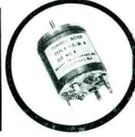
**Type R-110-2A-B Control Motor:** 115 volts; 400 cycle; OD 1.437; length 1 1/2"; speed at maximum power output 2800 rpm; Kearfott Company Inc. **\$22.50 each**
