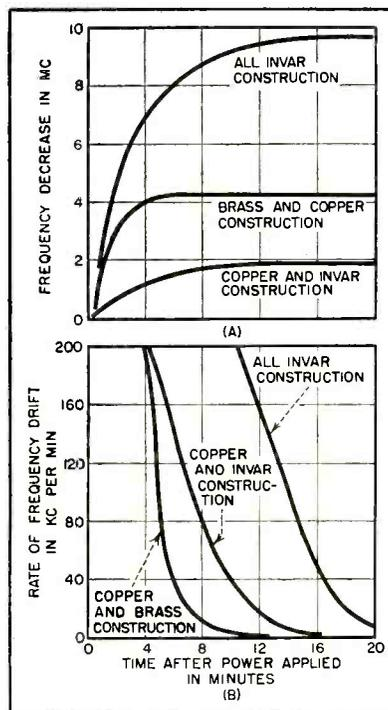
FIG. 3—Poor thermal conductivity of Invar, in one oscillator design, overshadows its dimensional stability
