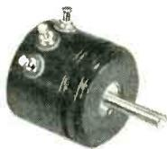
Designed for minimum-torque uses. Minimum torque is 0.01 inch-ounce. Dissipates one watt at 80° C. Resistances — 100 to 100,000 ohms. Weight is only 1/2 ounce. Ganging to 6 decks, internal clamps hold 7/8 in. diameter.
