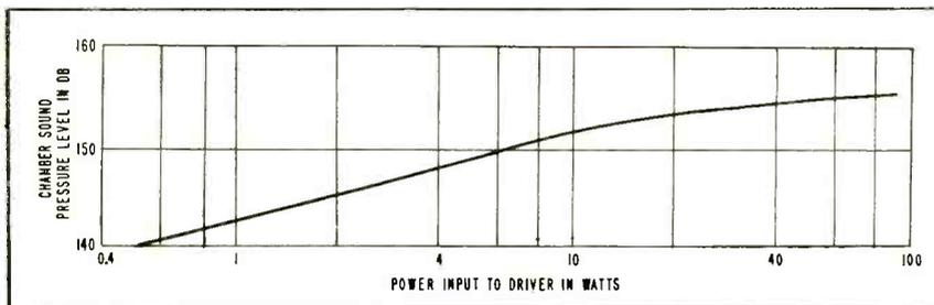
FIG. 4—Sound pressure level in test chamber at test chamber resonance of 2,300 cps. Reference level is same as that in Fig. 3
