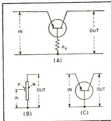
FIG. 7—Point-contact transistor switch (A) double-base diode switch (B) and driven junction transistor switch (C)
