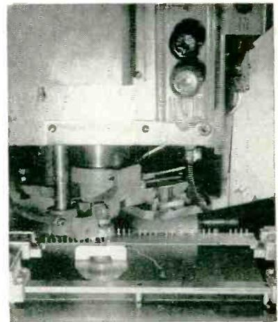
After putting in terminals on one side of board, the machine automatically shifts the board over and starts installing the other row of terminals. Air cylinders are used for actuation
