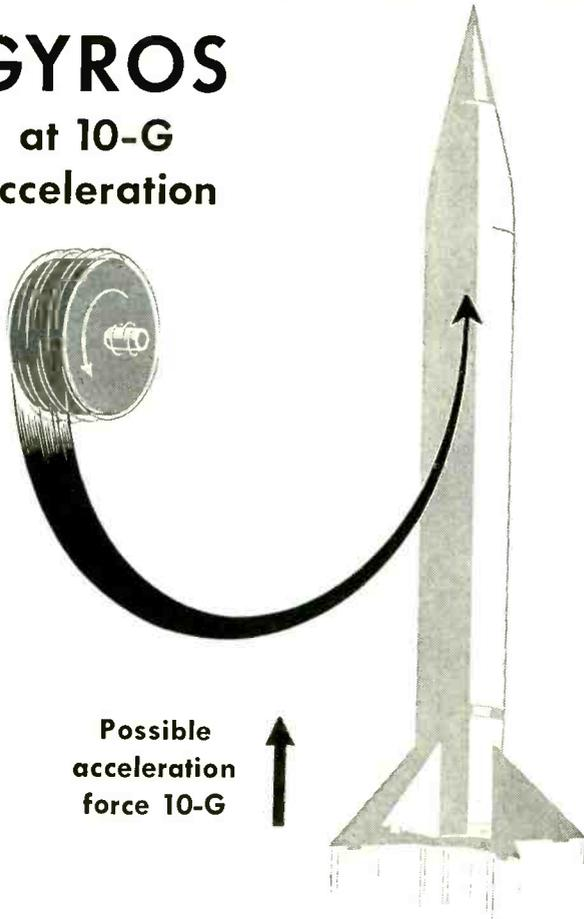
The gyroscope in a missile guidance system must be able to withstand acceleration forces up to 10 G's in any direction. This gyroscope, designed and developed by the Guided Missile Development Division of the U. S. Army and the Ford Instrument Company, will function under this acceleration. Tests have shown these gyros to be accurate to  $1/50^\circ$  per hour drift, or better.
