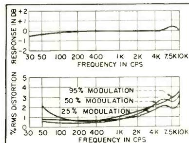
FIG. 3—Performance of transmitter, showing frequency response (top) and distortion (bottom)
