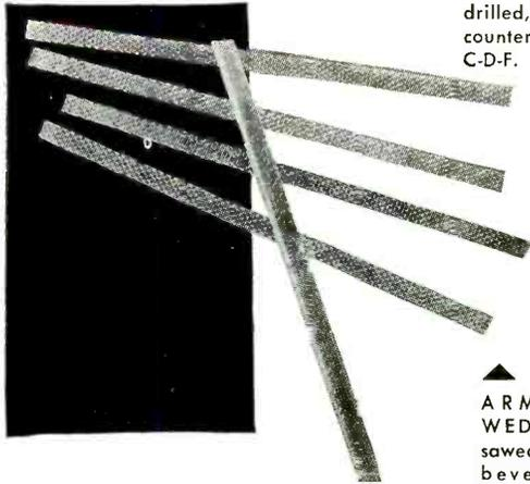
▲ ARMATURE SLOT WEDGES — GB-28M, sawed into strips, then beveled edges were broached to angle of 21° 23', and strips were cut to exact length. Machined by C-D-F.
