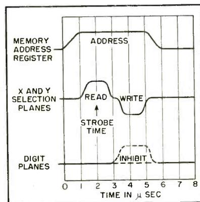
FIG. 2—Timing diagram of the currents in the core-memory array lines
