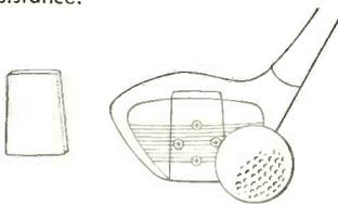
**Insert** in face of golf club, made of Taylor Vulcanized Fibre, withstands severe impact . . . gives long-lasting, long-hitting surface.
