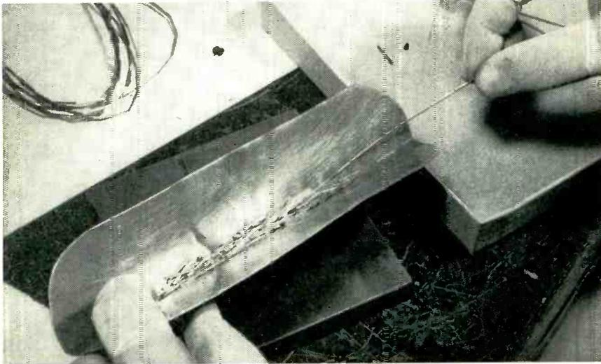
Method of loading cathodes for reliable type tubes on conductive wire in preparation for electropolishing before spraying with electron-emitting coating
