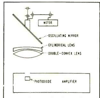
FIG. 6—Oscillating mirror scanner
