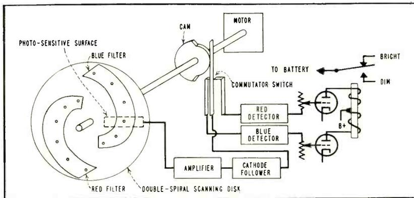
FIG. 5—Dual-channel circuit gives high sensitivity for taillights
