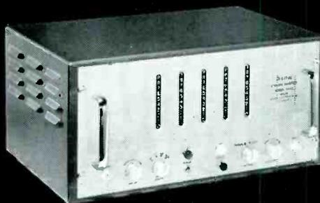
This Digital Cycling Counter, incorporating the *Countess*, is used for counting events, measuring frequency, RPM, etc.
