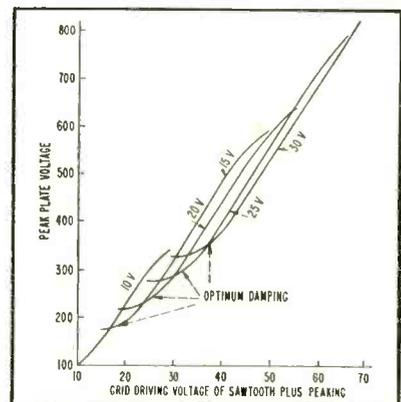
FIG. 5—Sawtooth-plus-peaking values for various levels of sawtooth input
