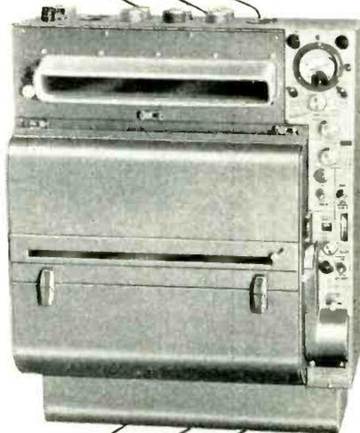
Separate light-tight record drums permit easy daylight loading; access to drive gears permits instant selection of record speed ranges.
