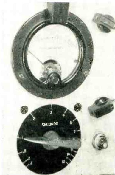
Time control and pilot lights are mounted below the photometer
