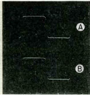
FIG. 5—Square wave (1 mc) displayed directly (A) and via amplifier (B)
