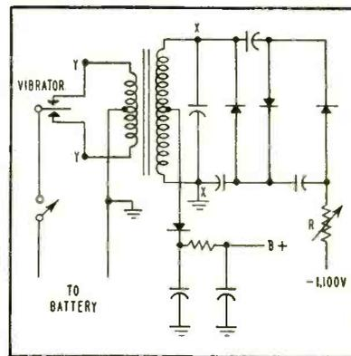
FIG. 3—Selenium-rectifier voltage tripler for phototube dynodes
