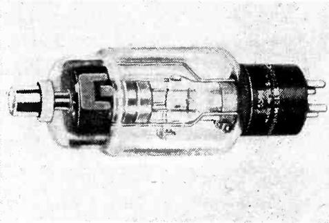
ambient temperature range of from -50 to +90 C. Maximum ratings: peak forward anode voltage, 2,500 v; peak inverse anode voltage, 5,000 v; average anode current, 0.5 amp; peak anode current, 2.0 amp; filament voltage, 2.5 v; filament current, 5.0 amp.
