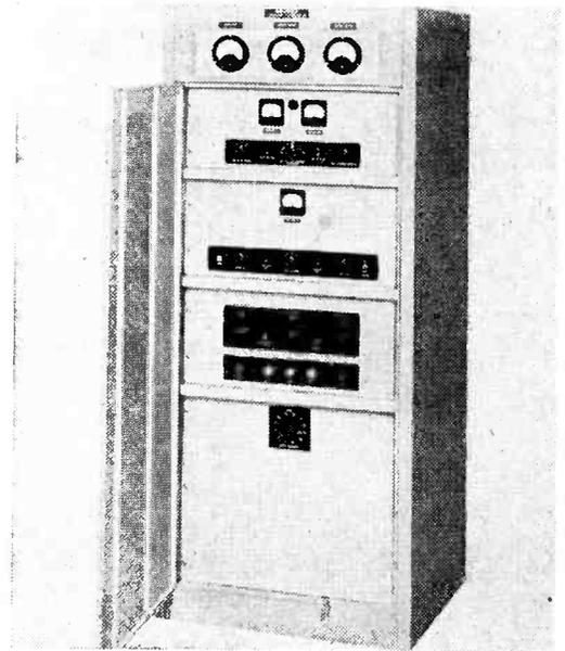
gan Ave., Chicago 11, Ill. A series of 1,000-watt audio amplifiers has been designed for vibration testing. Hum level has been held 48 db below full output. A final stage to deliver 2,500 watts is available for higher power vibrating equipment.
