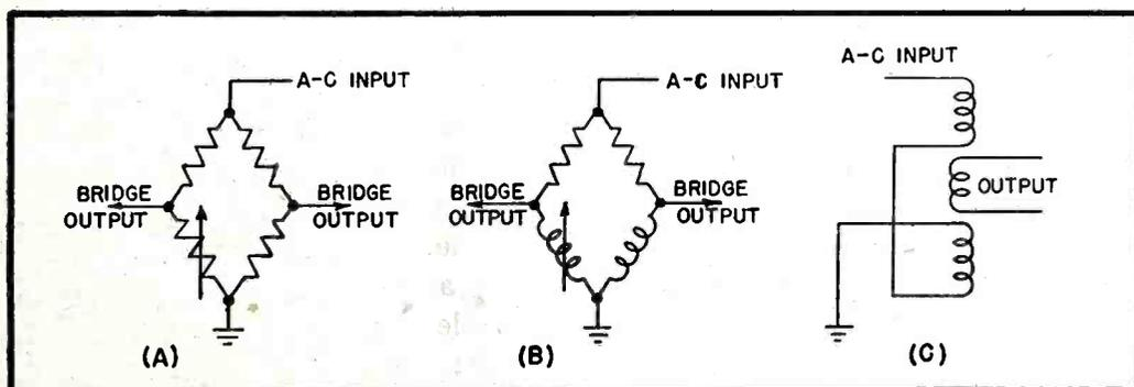
FIG. 1—Typical input circuits used with carrier-type amplifier
