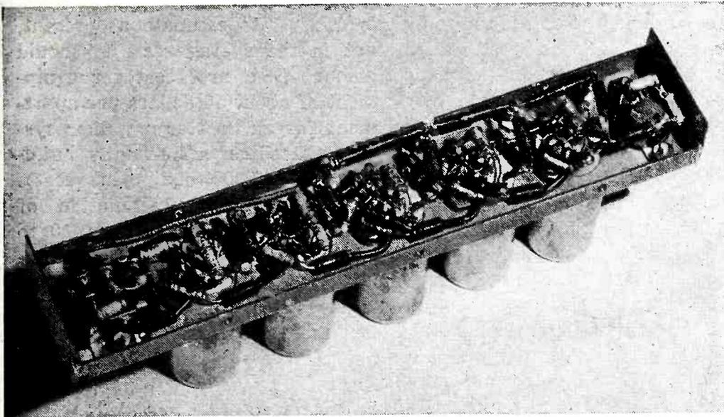
FIG. 2—Internal construction of channel amplifier shown in Fig. 1. Single-tuned staggered circuits are employed to secure flat response on each channel, high attenuation outside
