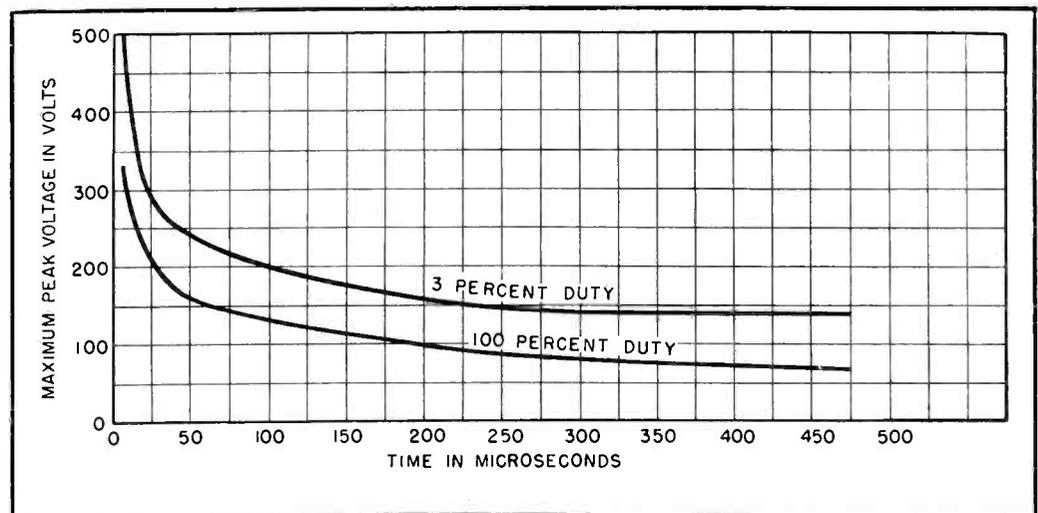
FIG. 10—Ignitor firing voltage as a function of linear buildup of voltage on ignitor of welding type ignitrons shows higher firing voltages at fast buildup
