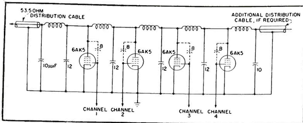
FIG. 7—Low-pass filter (cutoff 300 mc) used as a common load impedance for the final stages of channel amplifiers (four shown)
