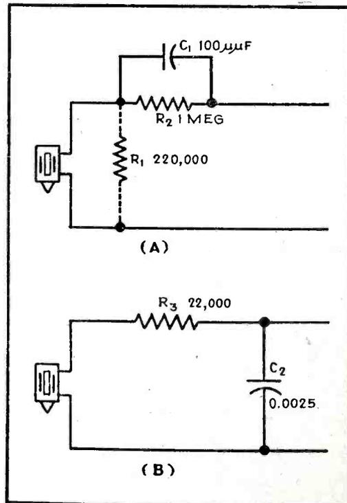
FIG. 2—Tone compensation circuits for use with a crystal pickup
