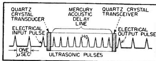
Diagram illustrating action of mercury memory storage tank unit used in EDVAC electronic computer now under construction at University of Pennsylvania
