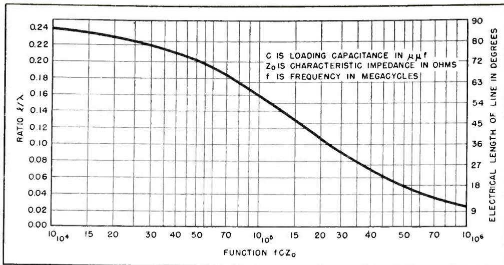
FIG. 2—Length of line relative to resonant wavelength is a function of the capacitance loading and characteristic impedance
