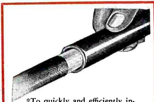
\*To quickly and efficiently insulate winding connections on the motor illustrated above, the manufacturer draws a sleeve of tough, flexible, heat resisting Fibron #5373 tubing over the connections. The windings are then impregnated with insulating varnish and baked; every connection is uniformly sealed and insulated.
