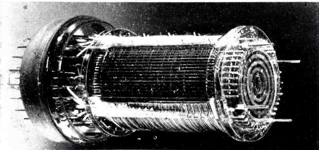
Two views of memory tube in which a multiplicity of images may be stored for later release as, for example, in a calculating machine (RCA)
