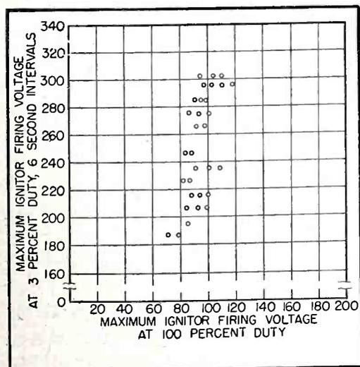
FIG. 3—Influence of intermittent duty on firing voltage of the ignitor
