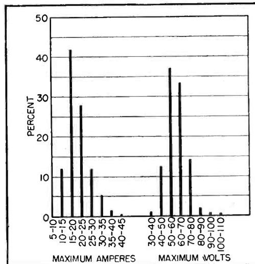
FIG. 5—Distribution of firing characteristics of welder ignitrons at full duty
