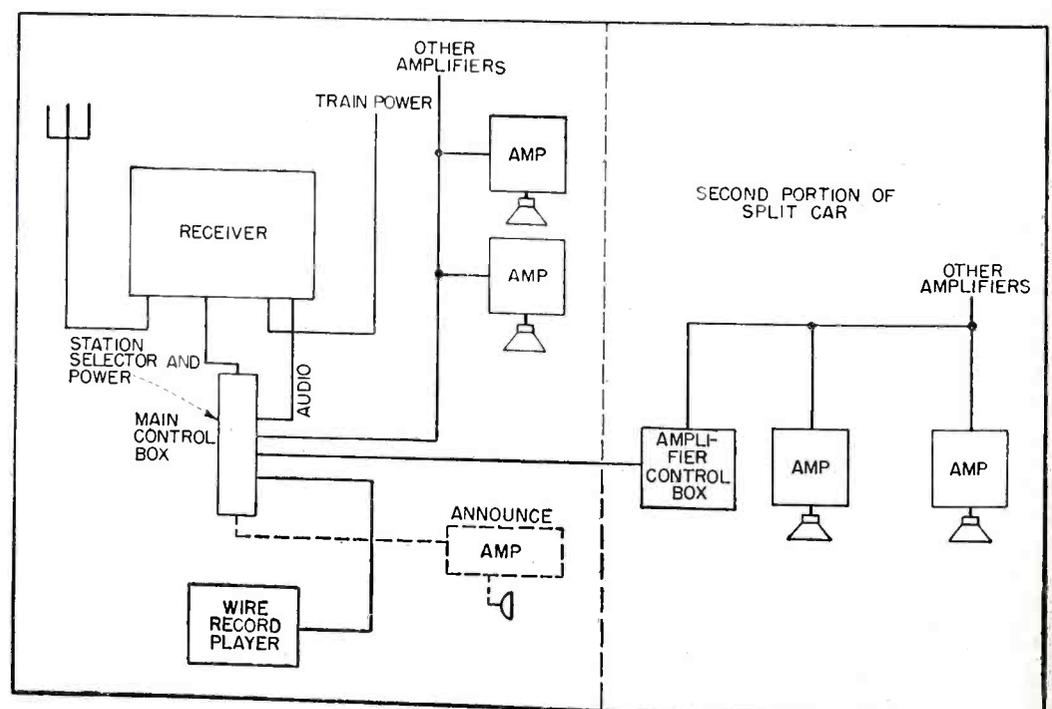
Block diagram of the equipment installed in one railroad car
