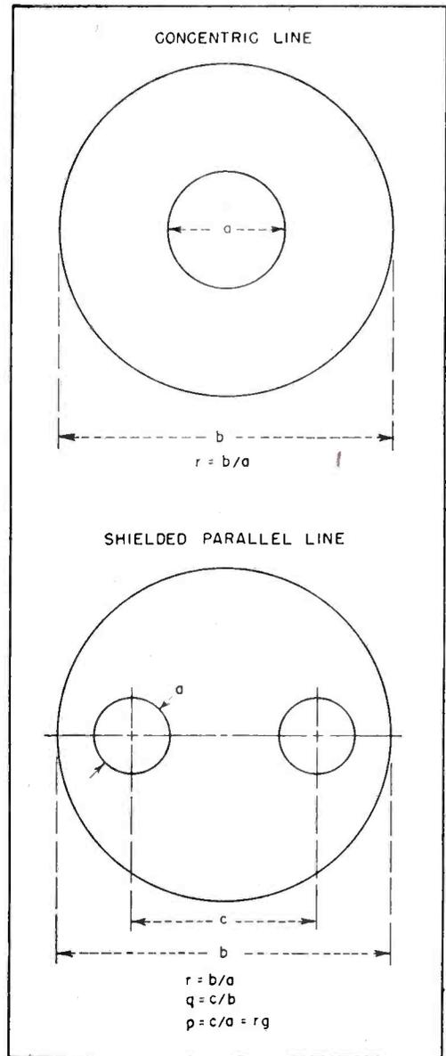
FIG. 1—(A) Size of concentric line is expressed by dimensionless ratio. (B) Size of shielded parallel line is expressed by two dimensionless ratios
