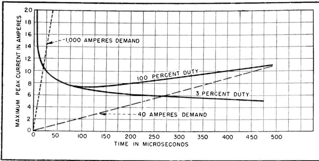
FIG. 11—Ignitor firing current varies as a function of time of linear buildup of ignitor current in welder type ignitrons, showing a minimum for full duty operation
