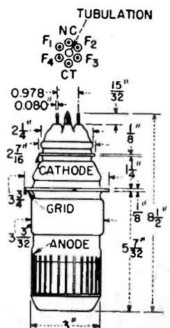
As a plate modulated Class-C pulse
