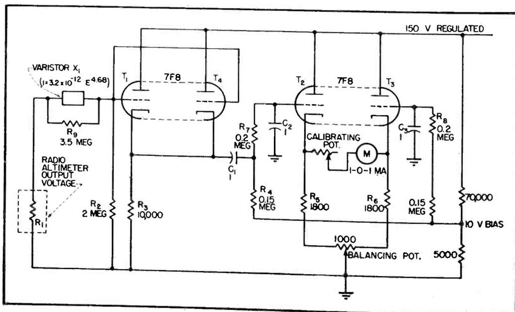
FIG. 1—Vertical velocity meter circuit
