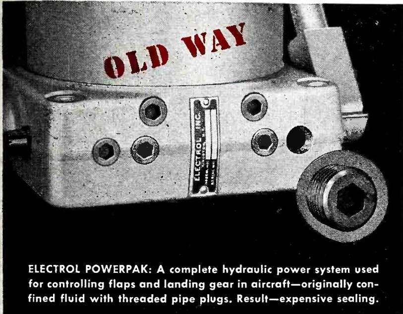
**ELECTROL POWERPAK:** A complete hydraulic power system used for controlling flaps and landing gear in aircraft—originally confined fluid with threaded pipe plugs. Result—expensive sealing.
