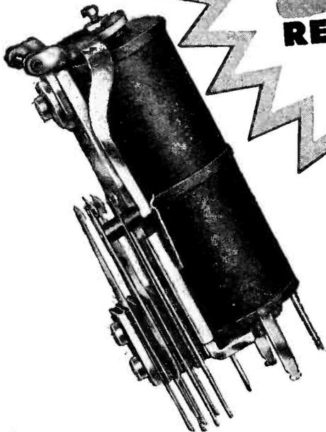
Clarostat telephone type relay. Great flexibility because of large variety of contact arrangements. Long life—many millions of operations. High sensitivity. Coil values up to 11,300 ohms. Available in long and short types.
