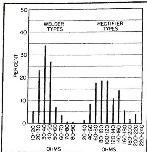
FIG. 7—Typical distribution of cold resistance of ignitrons of ignitron tubes
