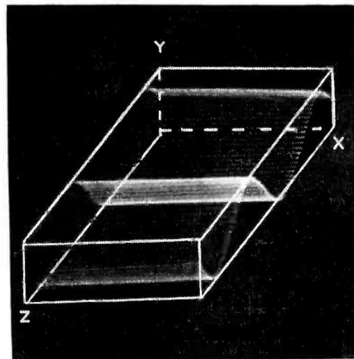
Three-dimensional cathode-ray tube portrayal of a sinusoidal wave traveling down a waveguide, with the lines simulating the waveguide formed by an auxiliary lantern-slide projector
