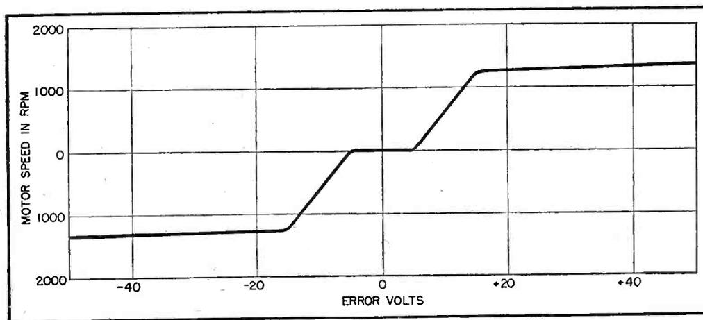
FIG. 6—Motor speed as a function of error voltage applied to d-c amplifier
