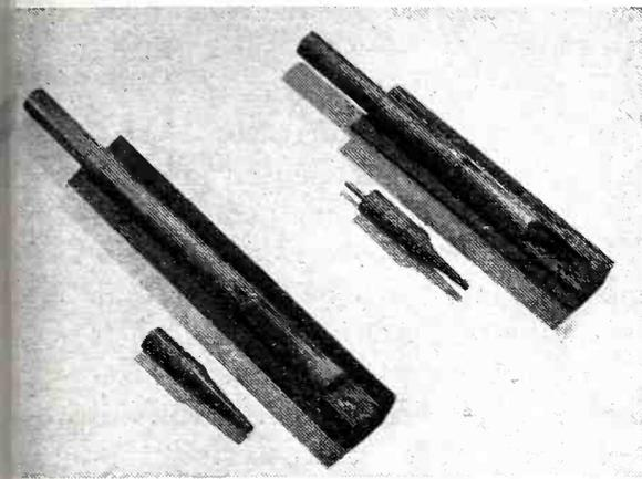
Finished ignitors and the blanks from which they are ground; left, for rectifier service; right, for welder service
