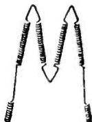
**CALLITE'S "M" SHAPED FILAMENTS** for high-power projection lamps. Employing a tungsten wire of .010" diameter wound on a .035 molybdenum mandrel for 55 turns per inch, its faster crystal growth produces interlacing crystals whose structure maintains the stability and non-warping property of the coil, thus withstanding elevated temperatures. Used for vacuum and incandescent lamps of high wattage and heat dissipation.
