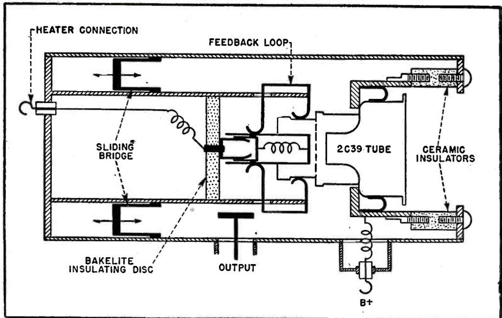
FIG. 2—Cross-section of 1,000-mc oscillator assembly using series capacitance method of stabilization
