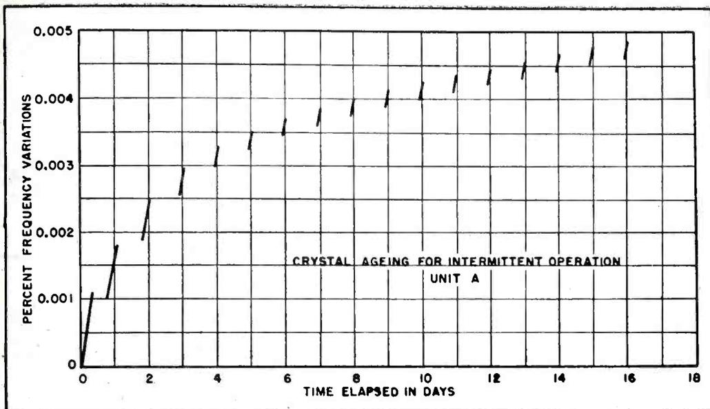
FIG. 4—A typical crystal and oven assembly can be expected to have this ageing characteristic for intermittent operation during its first few weeks of operation
