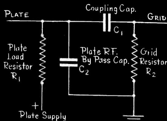
**2** First commercial application of the "printed circuit", and now available for the first time, Centralab's new *Couplate* is a complete interstage coupling circuit which combines into one unit the plate load resistor, the grid resistor, the plate by-pass capacitor and the coupling capacitor.
