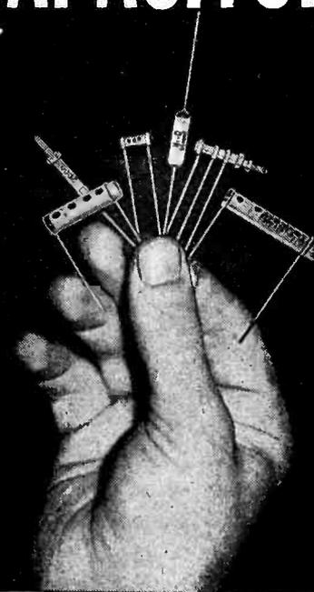
● Hi-Q Ceramic Capacitors are manufactured of titanium dioxide (for temperature compensating types). Electrodes are of pure silver, precision coated. They are individually tested for accuracy of physical dimension, temperature coefficient, power factor and dielectric strength. Available in C. I. type (axial leads) and C. N. type (parallel leads) also S. I. type Durez coated for fullest protection against extremes of fungus and climatic conditions.
