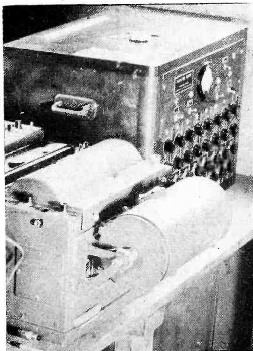
Amplifier bank alongside recording galvanometer
