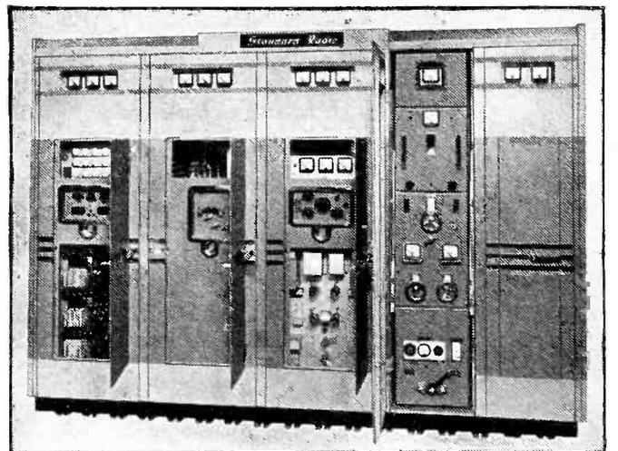
*Standard Radio* Type D.S.10 5kW Transmitter—first of its kind to use air-blast cooling of valves. It has a frequency range of 2.5 to 25 Mc/s and operates on up to three C.W. channels with independent keying; or on two C.W. channels with common keying or one C.W. and one PHONE channel with simultaneous transmission on two different frequencies. The equipment is remarkably compact and is designed for tropical conditions.
