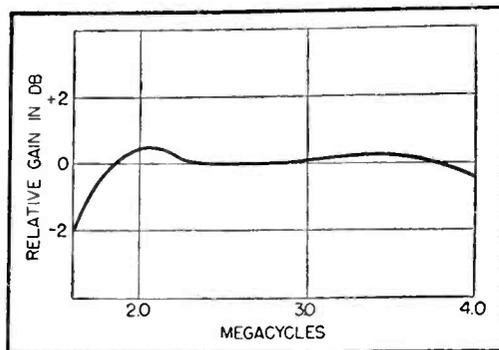
FIG. 3—Receiver gain as a function of desired frequency
