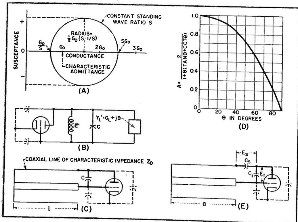
FIG. 1—(A) Locus of all possible admittances looking into transmission line; (B) simplified equivalent lumped circuit of Colpitts oscillator; (C) equivalent tank circuit of coaxial line oscillator, in which resonance occurs when reactance of  $C$  is equal to the inductive reactance of the section of closed coaxial transmission line; (D) variation of factor  $A$  with electrical length  $\theta$  of coaxial line; (E) circuit of series-capacitance method of stabilization
