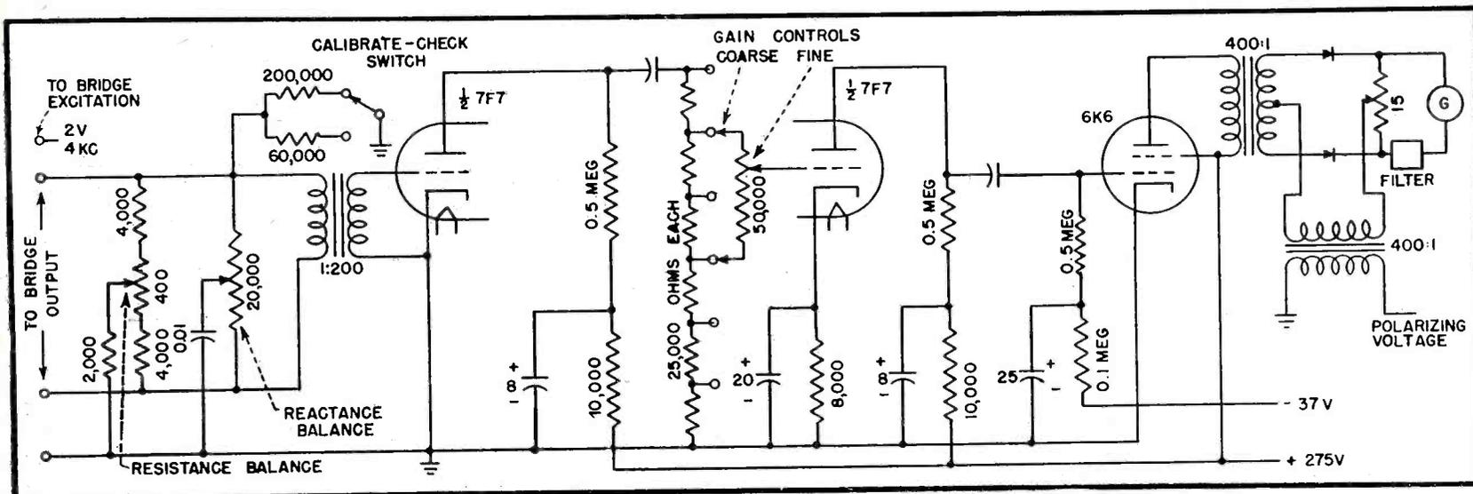
FIG. 3—Simplified schematic of amplifier, showing connections to demodulating circuit. Switching circuits have been omitted
