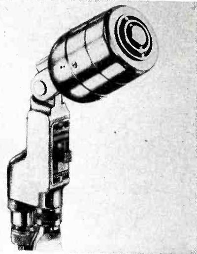
crophone now provides frequency response that is substantially flat from 40 to 9,000 cps. Output level is 53 db below 1 volt per dyne per sq cm, open circuit. The new Acoustalloy diaphragm withstands high humidity, extremes of temperature, corrosive effects of salt air, and severe mechanical shocks. Complete information is given in Catalog No. 101.
