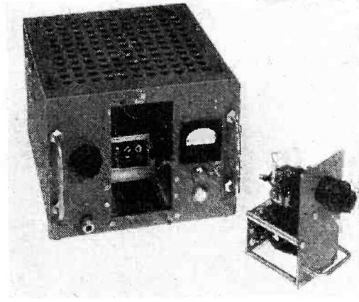
Oscillator with plug-in klystron unit
