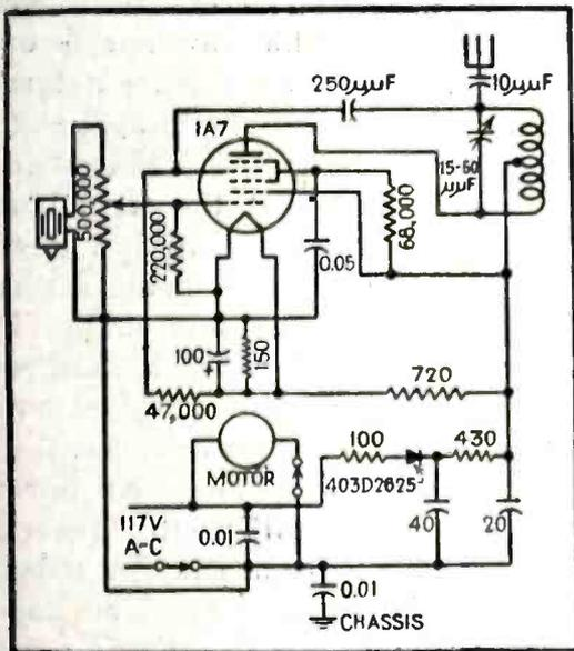
FIG. 3—Use of a filament-type tube permits instantaneous operation when the switch is thrown
