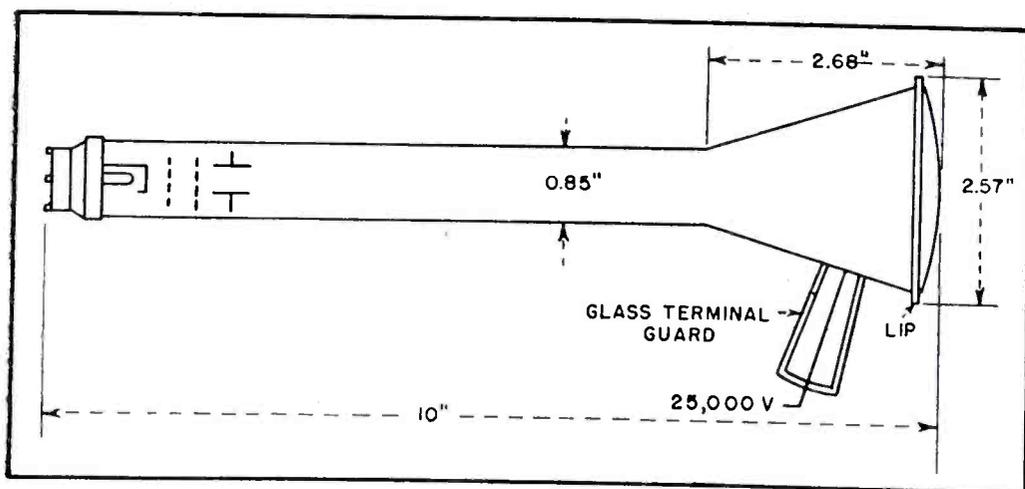
Extremely compact cathode-ray tube designed for projection television receivers. Maximum diameter of the tube is just a little over 2½ inches, but it is capable of projecting a 12 by 16-inch picture (Philips)
