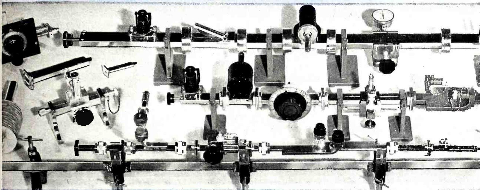
The complete line of De Mornay-Budd standard test equipment covers the frequency range from 4,000 mcs. to 27,000 mcs. It provides all R. F. waveguide units necessary for delicate, precision test work requiring extremely high accuracy in attenuation measurements, impedance measurements, impedance matching, calibration of directional couplers, VSWR frequency measurements, etc.
