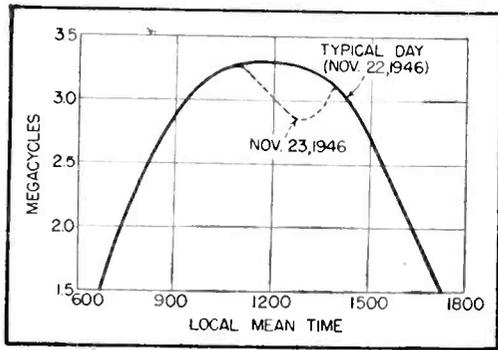
FIG. 1—Variation of E-layer critical frequency with time
