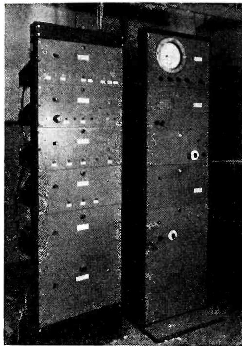
The central control unit contains a shading signal generator, mixing amplifier, RMA signal generator, synch generator, and power supplies at left. The video and audio monitors and channel-selector circuits are at right
