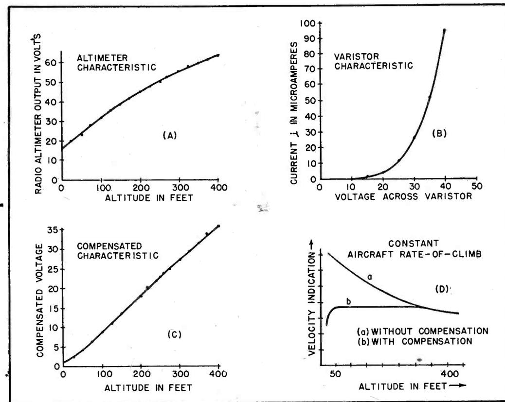
FIG. 2—(A) Nonlinear voltage output of radio altimeter. (B) Varistor characteristic. (C) Varistor-compensated altimeter characteristic. (D) Comparison of rate-of-climb indications of uncompensated and compensated altimeter
