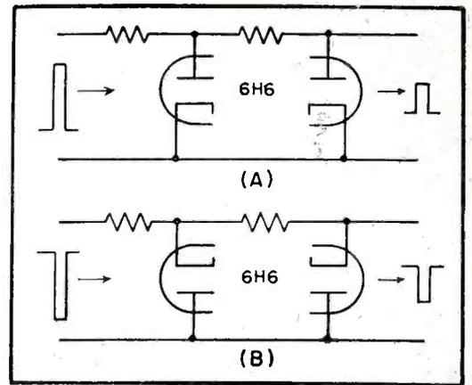
FIG. 3—Shunt diodes can be used in a nonlinear compression circuit
