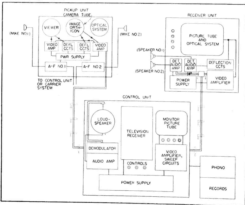
FIG. 2—Breakdown of electronic circuits. The central control unit normally handles several camera pickups and receiver units
