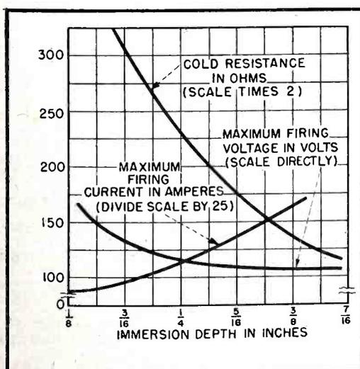
FIG. 9—Typical variation of ignitor characteristics with immersion of ignitor
