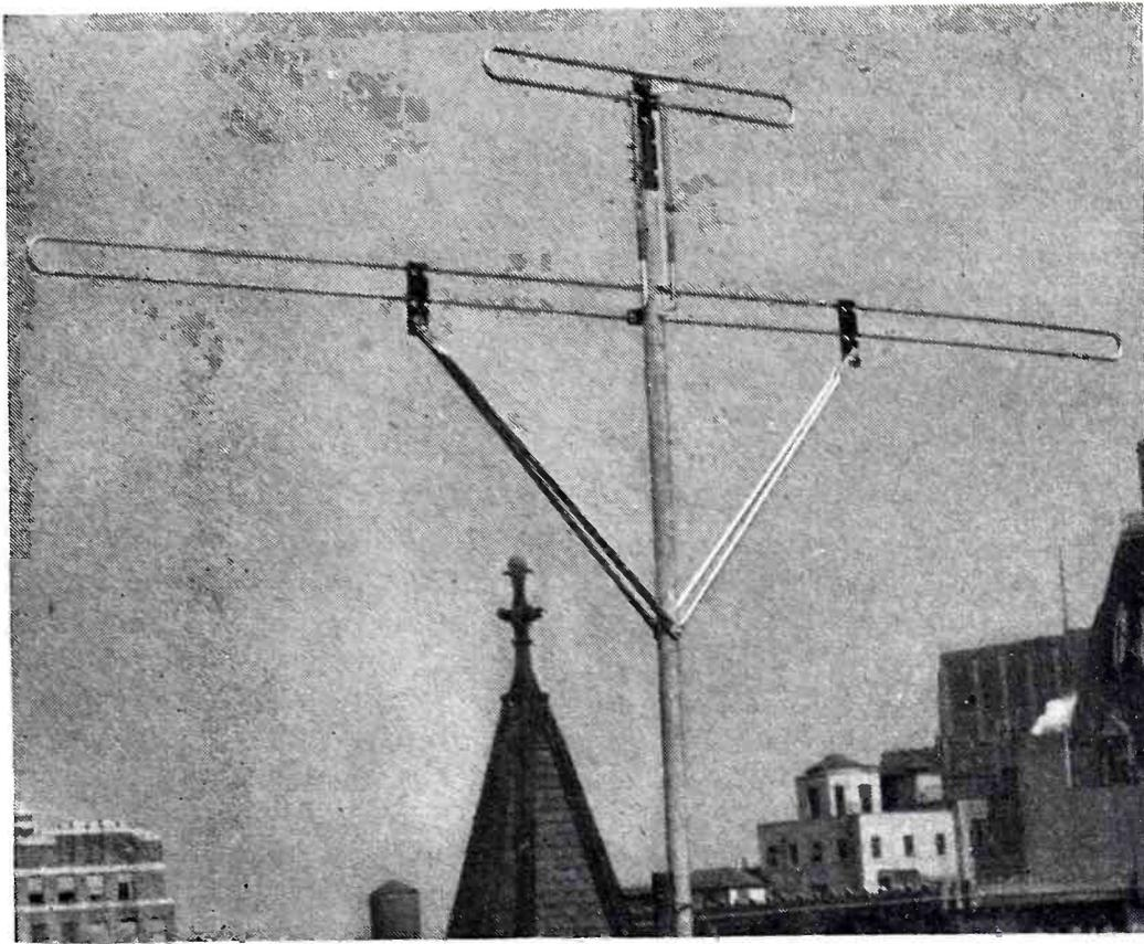
FIG. 5—Double folded-dipole antenna designed by Amy, Aceves and King to cover low and high frequency regions. The upper dipole is 28 inches long, the lower 94 inches long. An anti-resonant circuit prevents third harmonic operation of the lower element on the high frequencies, preserving the figure-eight reception pattern shown in Fig. 6
