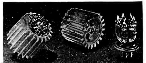
The voltage regulator unit consists of 7 subminiature gaseous voltage regulator tubes uniquely assembled in one unit as illustrated. Particularly adaptable where regulation requires a flat top (130 volts) with close accuracy and space conservation.
