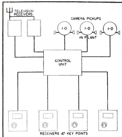
FIG. 1—Basic units of television system for monitoring manufacturing operations in a factory
