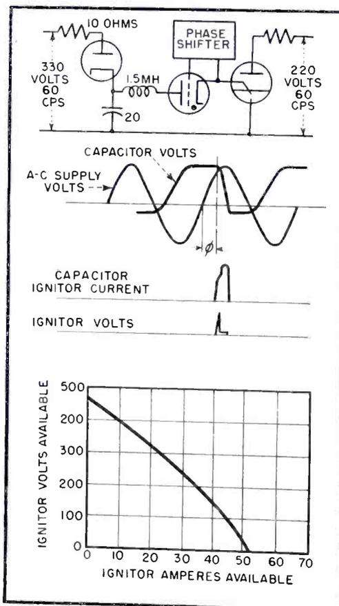
FIG. 13—Typical ignitor firing circuit uses charge stored on capacitor to fire ignitor
