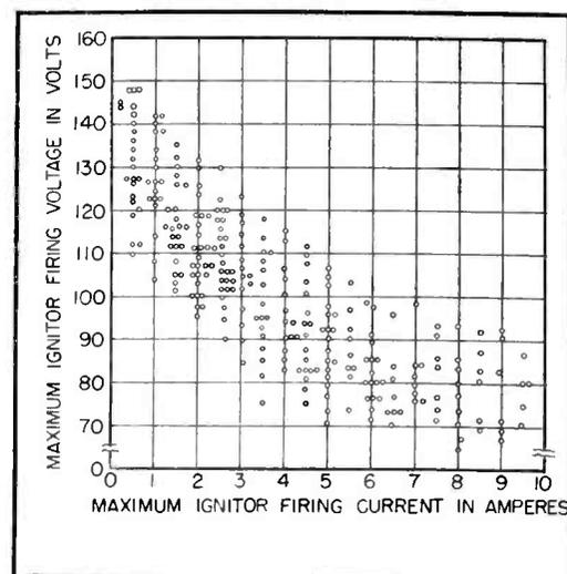
FIG. 8—Distribution of maximum firing voltage against maximum firing current
