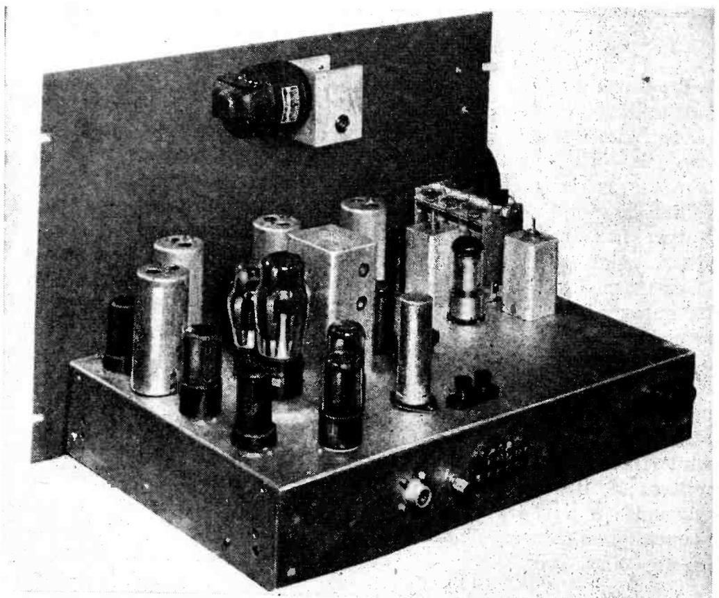
Rear view of receiver chassis showing motor and gear reduction box. The discriminator circuit is contained in the center shield can
