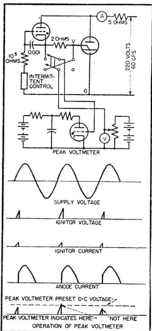
FIG. 1—Test circuit for studying ignitron characteristics, and typical wave shapes
