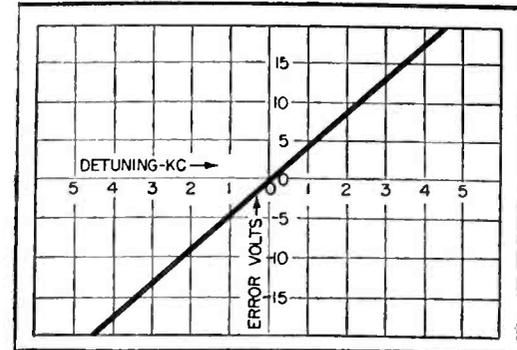
FIG. 4—Discriminator output characteristics with 100-microvolt signal at antenna
