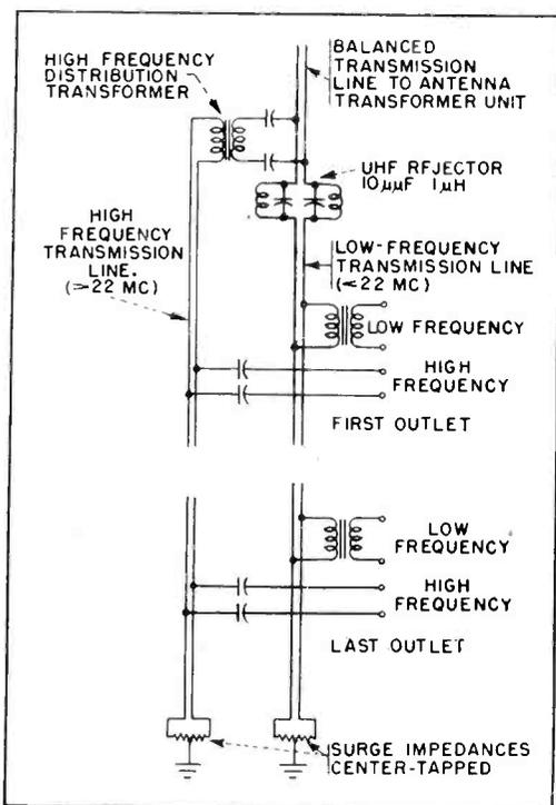
FIG. 4—Pre-war distribution system, employing a rejector filter and transformers to separate low from high frequencies
