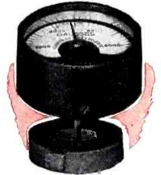
A tiny SILMANAL cylinder magnetized along a diameter is the heart of the G-E gauss meter. When the probe is placed in the field of a permanent magnet or a d-c electromagnet, the SILMANAL magnet on the shaft tends to line up with the flux. Flux density is measured by rotating the instrument until the pointer reaches its highest reading. This occurs when the probe-magnet flux is at right angles to the flux being investigated. The pointer when at zero scale position indicates flux direction.
