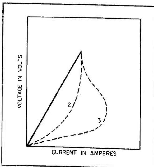
FIG. 2—Oscilloscopic traces of arc transfer show high currents for slow transfers
