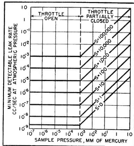
FIG. 4—Sensitivity of General Electric leak detector depends on speed of auxiliary pumping equipment S in liters per second
