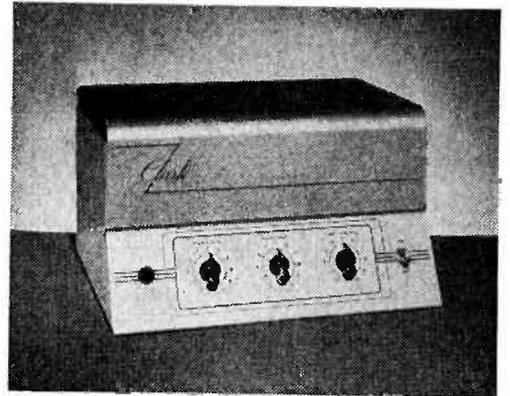
cycles and less than 3 percent harmonic distortion at maximum power. Hum is 60 db down. Two half-megohm inputs are provided. Output is tapped for 4, 8, 16, and 500 ohms impedance. Further information is given in Bulletin 134.
