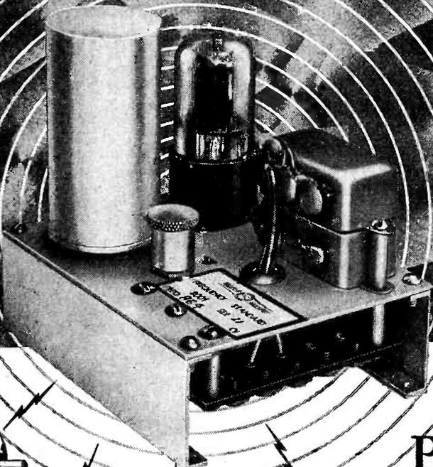
Pictured here is a tuning-fork frequency standard with accuracy guaranteed to one part per million per degree Centigrade. The fork is temperature-compensated and hermetically sealed against variations of barometric pressure. This standard, when combined with basic equipment, facilitates accurate speed and time control by mechanical, electrical, acoustical or optical means.
