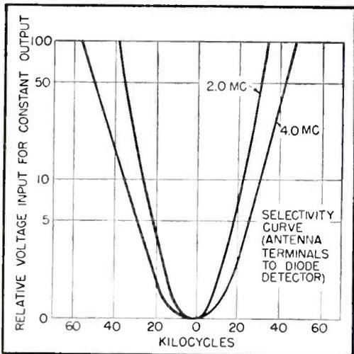
FIG. 2—Overall bandwidth of receiver
