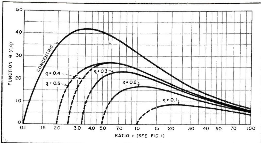
FIG. 6—Selectivity function (see Eq. 8) indicates optimum relative line dimensions for any application. If design is begun with this graph, optimum tank efficiency can be obtained
