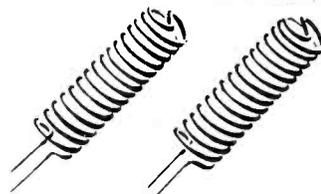
**CALLITE'S MINIATURE DOUBLE HELICAL HEATER** for radar and microwave transmitting tubes. This molybdenum-tungsten alloy filament, .0048" in diameter and 133 mm. in length, is coated with aluminum. Evenly wound, of high tensile strength, good ductility and uniform resistance, this filament is particularly adaptable for high and ultra-high frequencies in restricted spaces.
