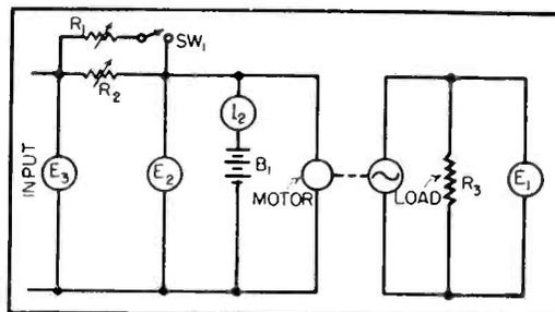
FIG. 1—Basic charging circuit in which a manually operated switch is used for illustration
