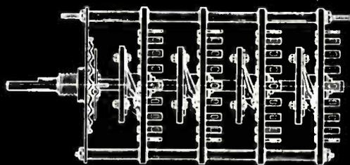
**I** Specially designed for transmitters, power supply converters, and a broad new range of industrial and electronic uses, Centralab's medium-duty power switches give you efficient performance up to 20 megacycles. Tests prove that these switches have a mini-
