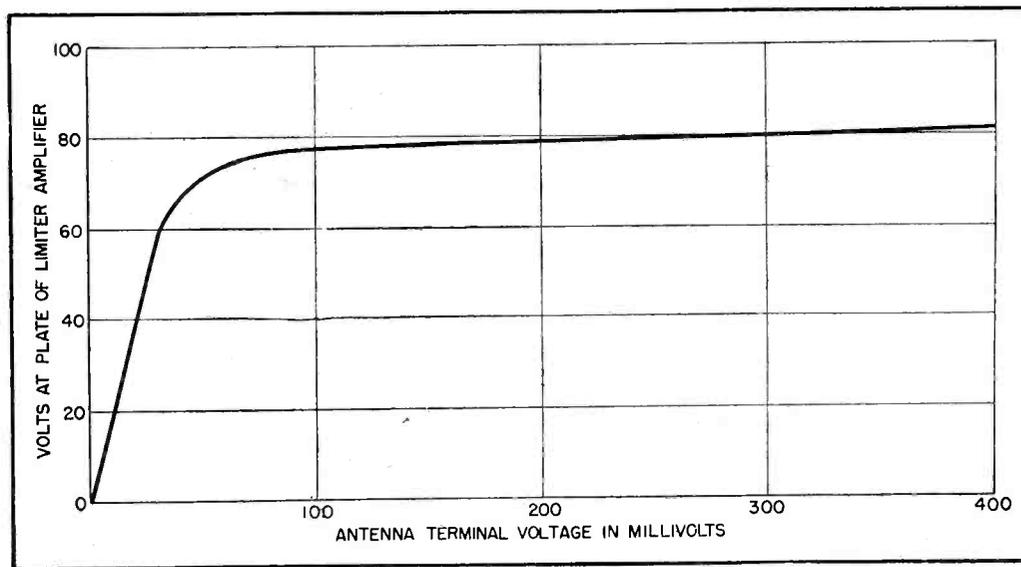
FIG. 5—Linearity characteristics from antenna terminals to discriminator input
