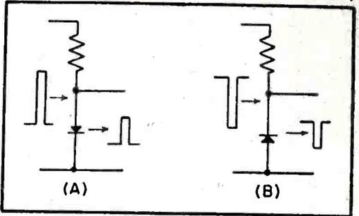
FIG. 1—Nonlinear compression circuits use crystal rectifiers
