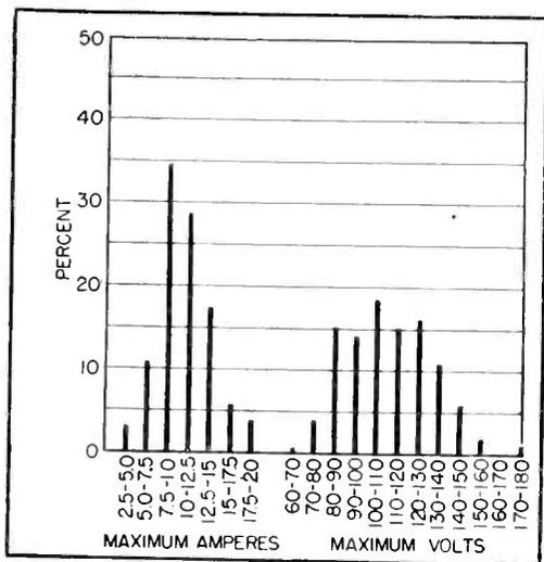
FIG. 6—Distribution of firing characteristics of rectifier ignitrons at full duty
