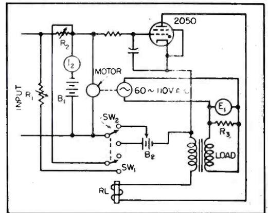
FIG. 2—Electronic charging control circuit with battery  $B_2$  supplying a reference voltage
