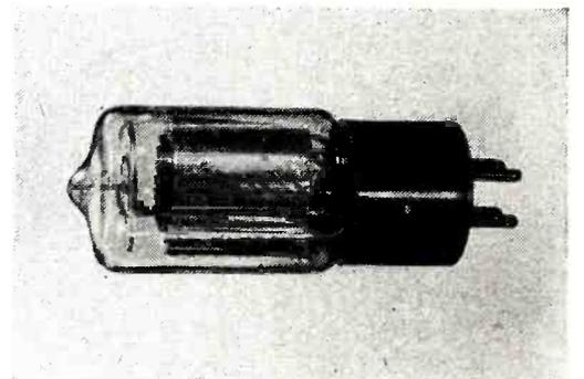
anode current, 1.0 amp; peak anode current, 8.0 amp; maximum peak inverse voltage 700 v; and filament voltage, 2.5 v. The tube has been designed for motor-control, servo-amplifier, high-speed counting and similar circuits.
