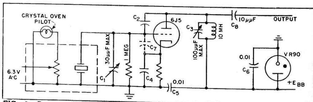
FIG. 3—Conventional crystal oscillator circuit used in the secondary frequency standard
