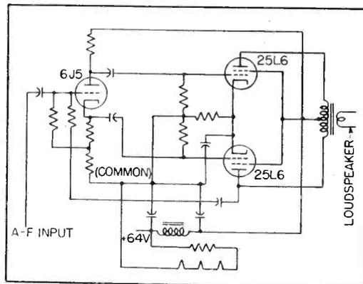
Circuit of a loudspeaker amplifier
