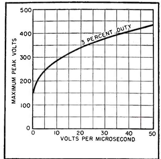
FIG. 12—Ignitor firing voltage versus rate of rise of applied voltage
