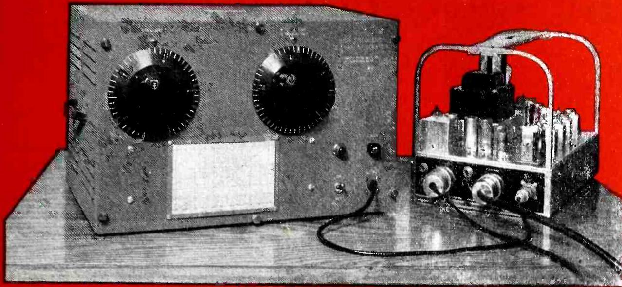
Model 196TS High Frequency Signal Generator being used to align a Harvey 152-162 Mc. Mobile Receiver.
