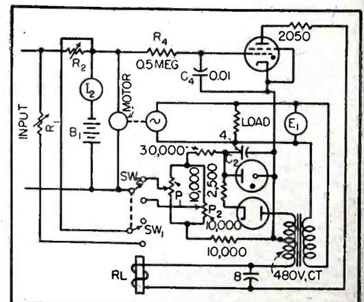
FIG. 3—Stabilized voltage source replaces the reference battery in the final circuit
