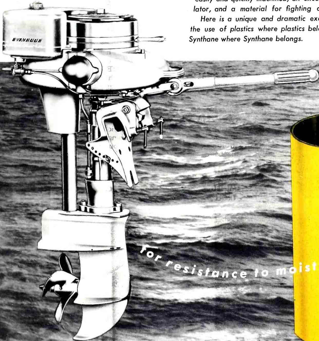
*This outboard motor pivot bearing (above) requires no lubrication...resists both salt and fresh water, wears long and well... it's Synthane.*
