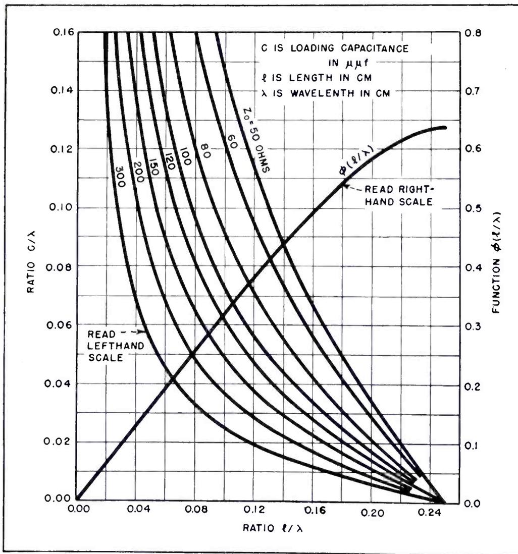
FIG. 3—Left hand scale gives ratio of loading capacitance to wavelength as a function for line length (see Fig. 2) for various characteristic impedances (see Fig. 4). Right hand scale gives unloaded impedance length parameter (see Eq. 6)
