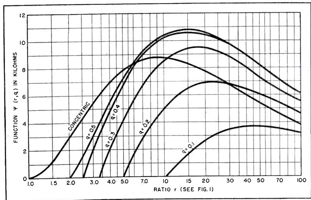
FIG. 5—Unloaded tank impedance cross-section parameter (see Eq. 7) is given as a function of the dimensionless ratios of line size
