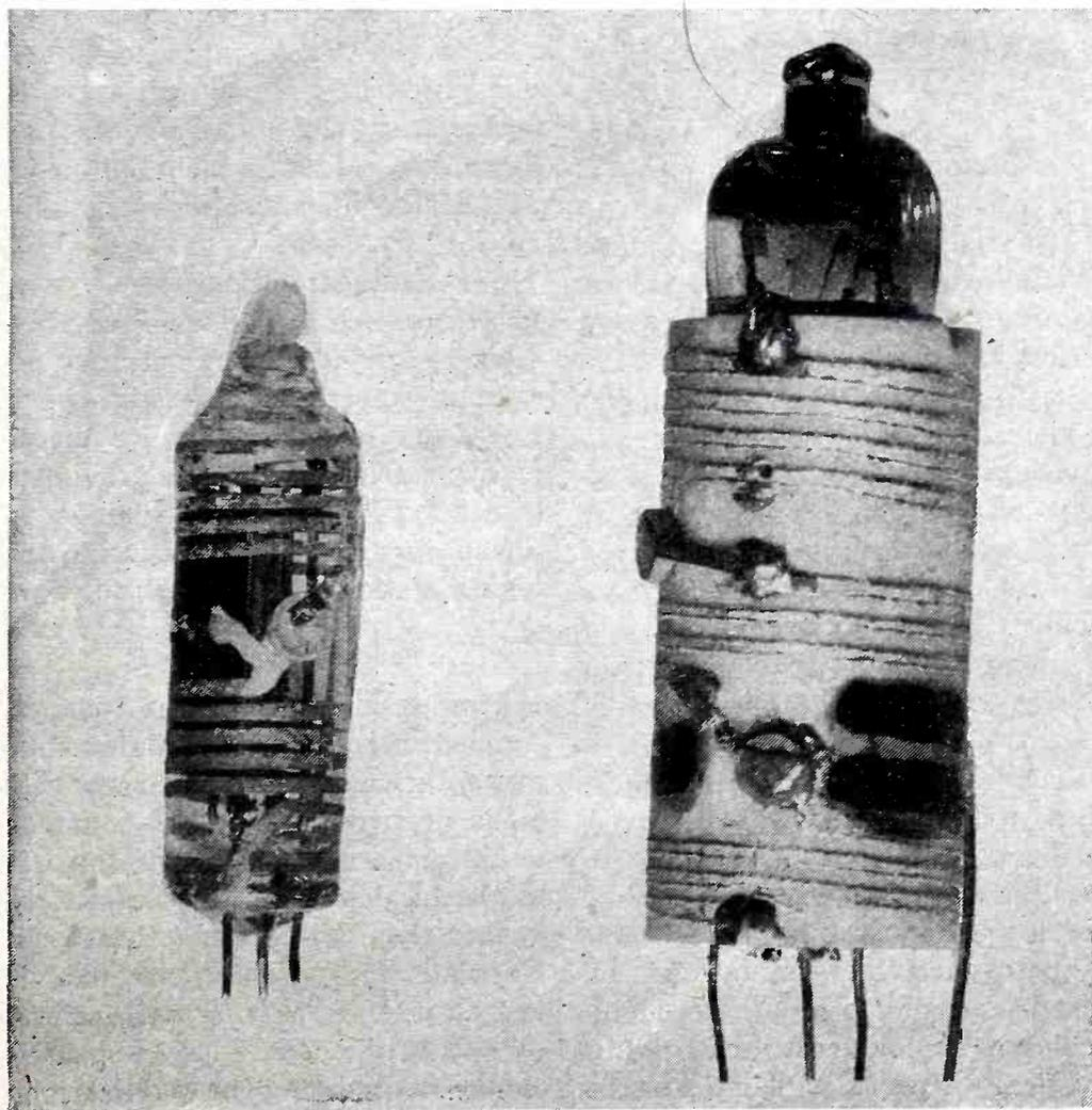
Two versions of a 2-meter transmitter, complete except for microphone and batteries, utilizing printed circuits. In one case wiring and components are placed right on the inch-long tube envelope, while in the other they are printed on a ceramic sleeve (NBS)
