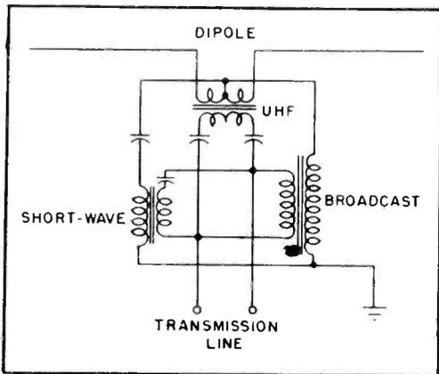
FIG. 3—Antenna coupling unit for non-amplifier system designed to abstract broadcast, shortwave and television signals from a single vhf dipole
