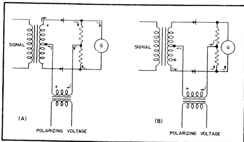
FIG. 2—Directions of current flow in bridge-type demodulating circuit
