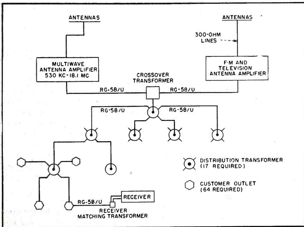
FIG. 9—Antennaplex distribution diagram for 64 outlets, providing broadcast, shortwave, television and f-m signals over a single cable with transformers to multiple branch points. This system can be extended to 256 outlets without additional amplifier equipment
