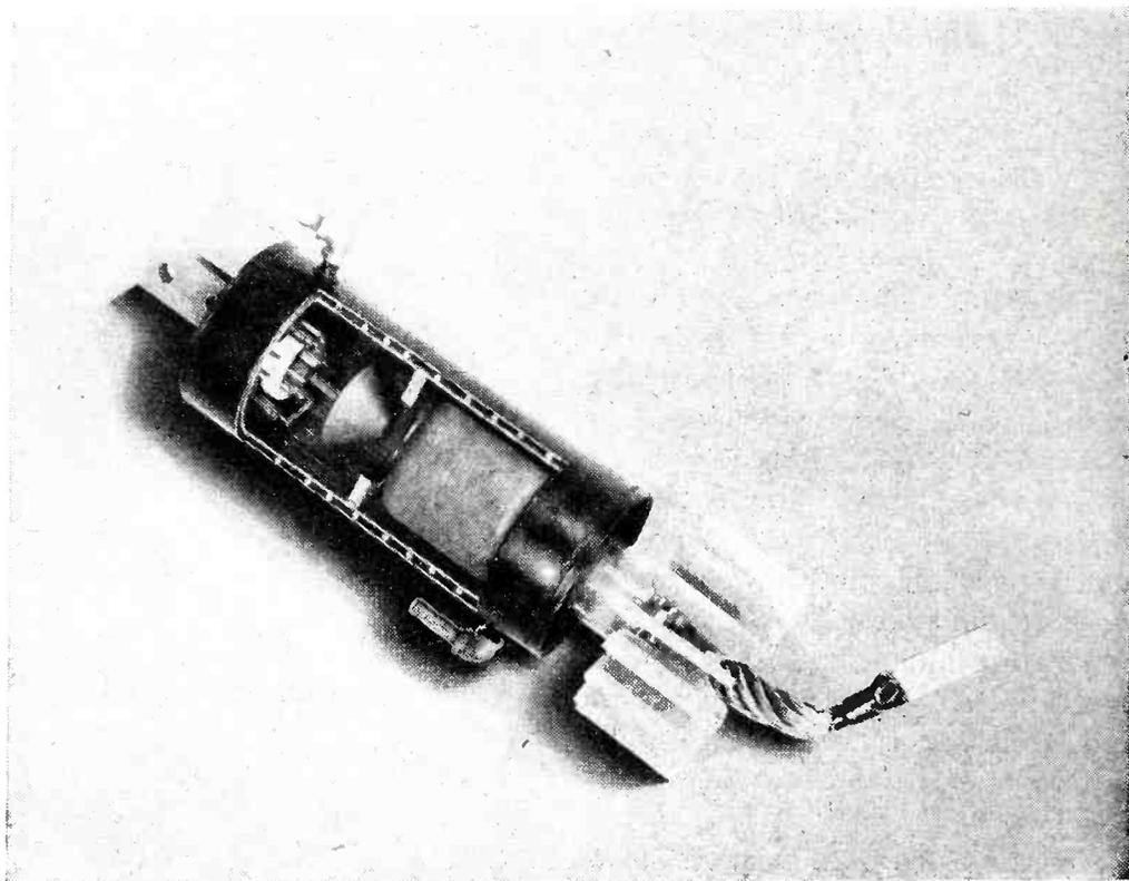
Cutaway of rectifier type ignitron
