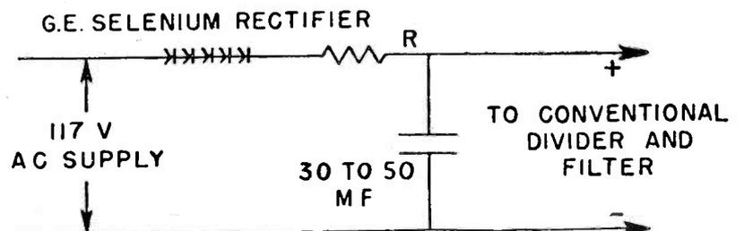
*Typical diagram for radio receivers using the new G-E selenium rectifier. A ballast resistor "R" is usually provided to limit the output voltage of the rectifier to that required by the particular circuit. The value of "R" is usually between 25 and 50 ohms, but may be modified to meet any particular circuit requirements.*
