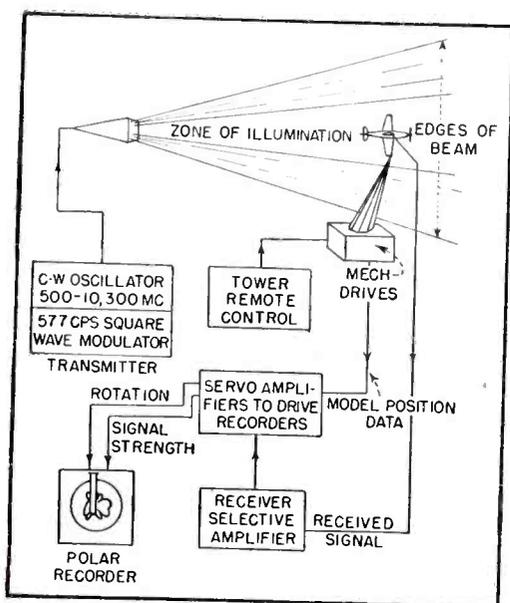
FIG. 1—Block diagram of complete system for measuring aircraft antenna radiation patterns in miniature
