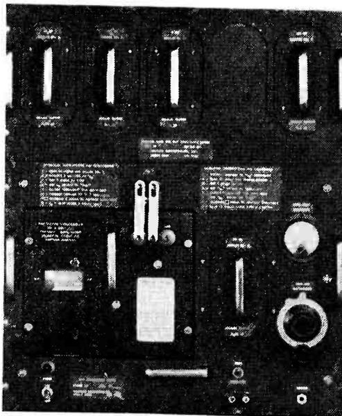
meter has been designed for use in the region between that served by the conventional 1,000-cycle bridge and the array of equipment usually employed at radio frequencies. In five decades it covers continuously the ranges of 1 microhenry to 100 millihenrys. The instrument can also be used for direct measurement of small capacitance up to 1,000 micromicrofarads, or for indirect measurement of larger capacitance. The equipment is rack mounted.
