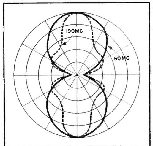
FIG. 6—Horizontal coverage diagrams of antenna shown in Fig. 5, taken at typical frequencies in the low and high frequency regions of the television band
