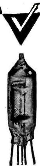
The VX series of subminiature vacuum tubes are especially adaptable to electrometer applications in fine instrumentation and for circuits used in radiation measurement. Feature 10 ma. filament current, grid resistance of  $10^{15}$  ohms. Unusually stable.
