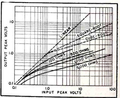
FIG. 2—Compression characteristic of germanium crystal divider varies with series resistance
