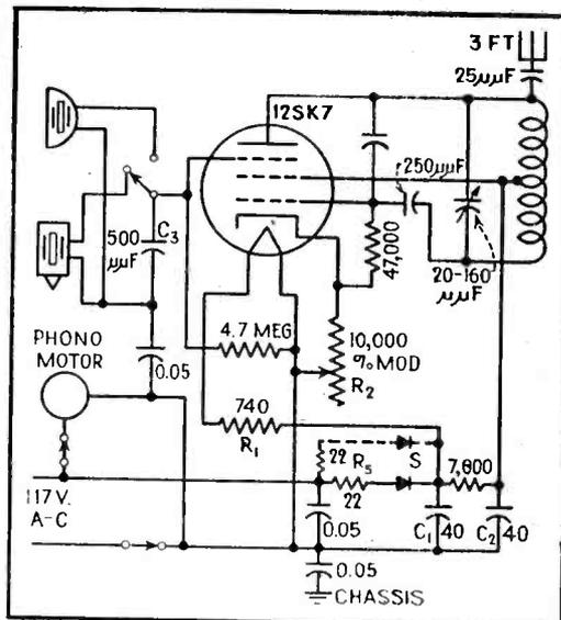
FIG. 1—Circuit of versatile phonograph oscillator using a selenium rectifier
