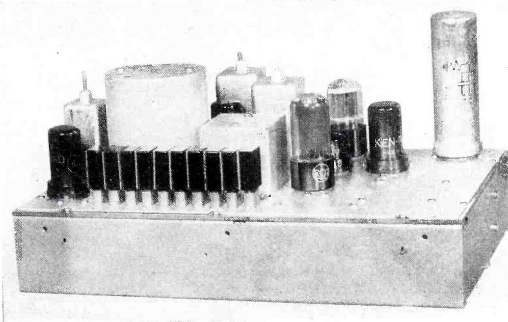
Crystal mountings and components on top of chassis
