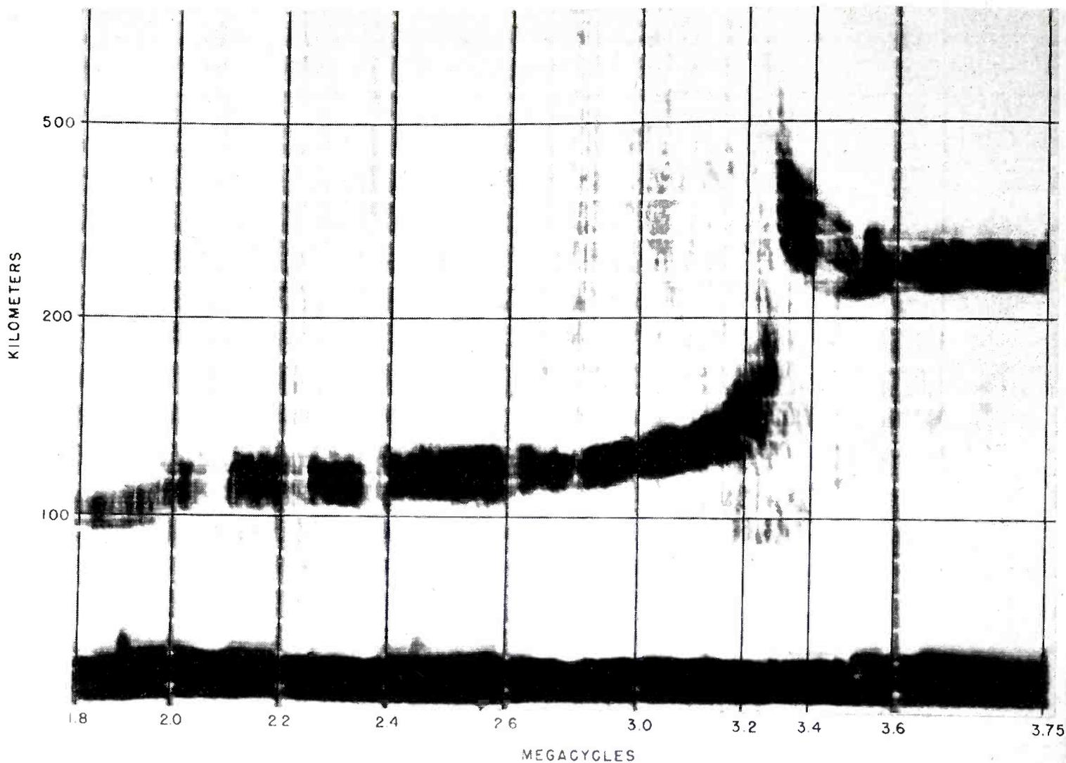
FIG. 7—Sweep-frequency record of November 24, 1946, at 1222 local mean time, showing the E-layer critical frequency at 3.3 megacycles (vertical incidence). This control data was taken the day after the eclipse
