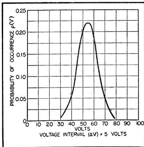
FIG. 4—Probability of occurrence of ignitor firing at a given voltage in 656 cycles
