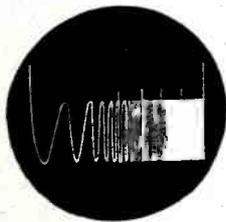
CLARKSTAN brings you Sweep Frequency Film (a Wayne R. Johnson development) for testing motion picture sound equipment. The CLARKSTAN Sweep Frequency Film and
