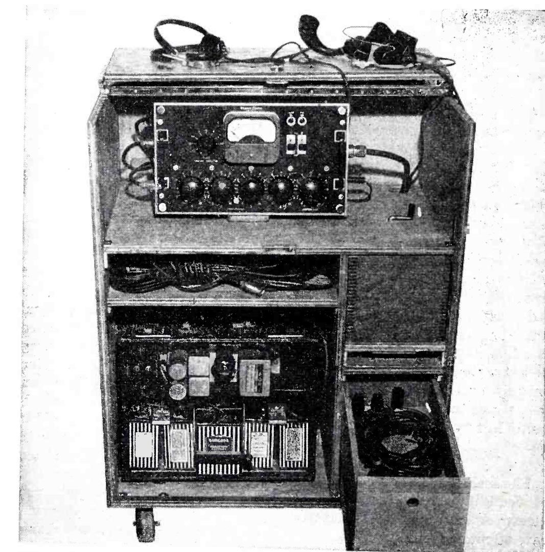
FIG. 1—Remote pickup equipment for scheduled broadcasts includes mixer-amplifier, telephone equipment, a-c and battery power supplies mounted in cabinet with spares
