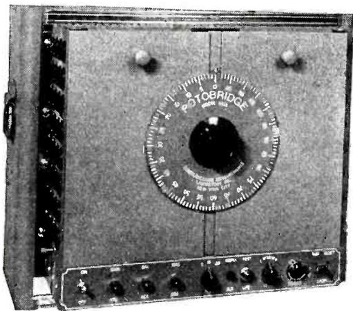
This new ROTOBIDGE is designed for radio and electronic manufacturers who require quick-shift inspection equipment on the production lines to test relatively short runs of varied products. It is capable of testing up to 120 circuits for wiring errors, continuity, and proper resistance values by bridge-type measurements. Indicates and isolates defective circuits by number. Acceptance or rejection is automatic on a "go" or "no go" basis against established inspection standards.
