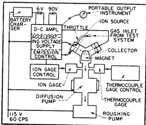
FIG. 3—Block diagram shows essential components of spectrometer leak detector
