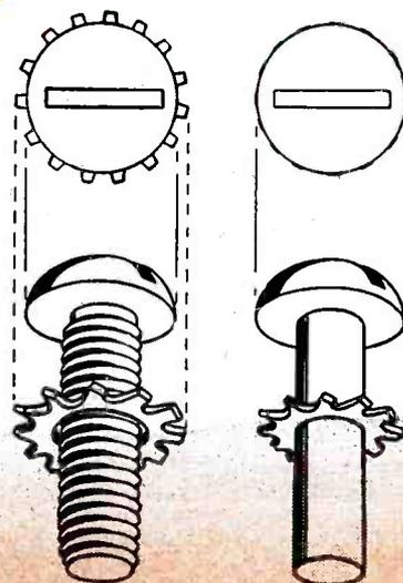
The illustrations above show the difference between hand assembly of separate washers and screws and the mechanical pre-assembly of SEMS by Shakeproof. Note the smaller internal diameter with the teeth pulled in beneath the screw head when the lock washer is placed on the screw blank before the thread is rolled. Also, note how the teeth of the hand-assembled combination protrude out from under the screw head.
