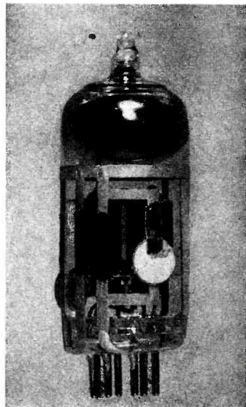
FIG. 1—Resistors and conductors are printed onto glass envelope; capacitors use high dielectric constant insulators to obtain high capacitance in small volume
