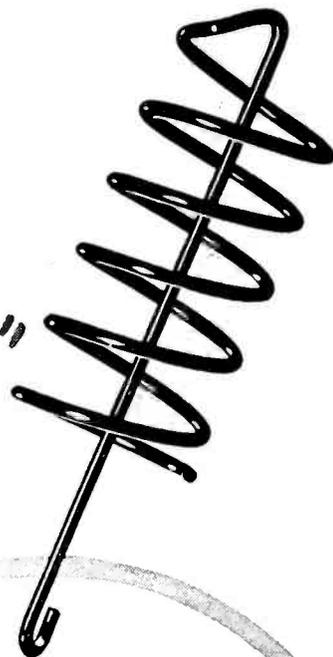
**CALLITE'S CONE-SHAPED TUNGSTEN FILAMENT.** This heater wire, .020" in diameter, is specially designed to produce lamp filaments that will maintain a constant lumen output because it permits very little distortion of the coils (despite their unusual pattern) during the life of the lamp. Used for special types of incandescent and gas filled lamps.
