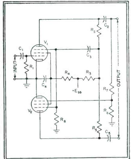
FIG. 1—Duplex feedback preserves balance of inverter
