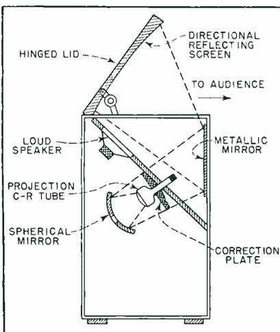
FIG. 2—Projection system of new Philco receiver, shown at Princeton for first time. The directional reflector confines light to eye level, thus increasing brightness and contrast four times over comparable projection units
