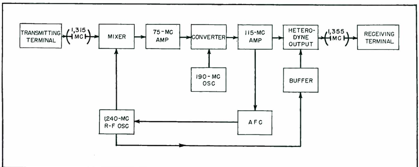
FIG. 2—Diagram of 1,315-mc television relay system. Transmitting terminal block at the left and receiving terminal block at the right are similar to the units in the studio-transmitter equipment diagrammed in Fig. 1
