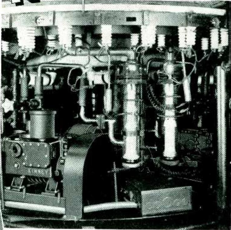
Compact installation of Kinney Compound High Vacuum Pumps used to back diffusion pumps in the manufacture of ultra high frequency tubes at Raytheon Mfg. Co., Waltham, Mass.
