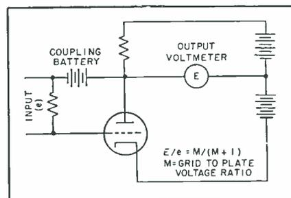
FIG. 1—Degenerative coupling from plate to grid, through a battery to preserve the required operating potentials on grid and plate, stabilizes the tube circuit
