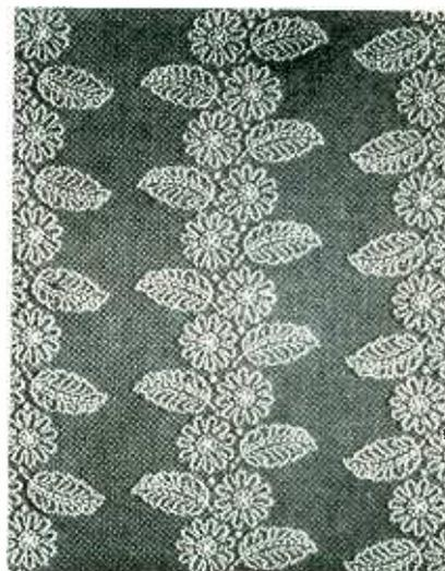
By applying adhesive through a stencil prior to electrostatic treatment, a tufted material having a design such as shown above is formed
