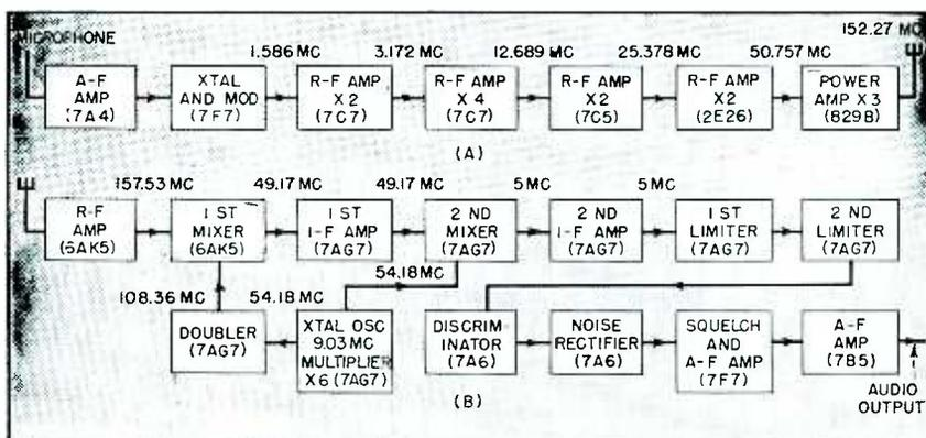
FIG. 1—Block diagram of Hackensack system circuit elements used in both fixed and mobile transmitters (A) and receivers (B). A single crystal furnishes conversion frequencies for the double-detection superheterodyne receiver
