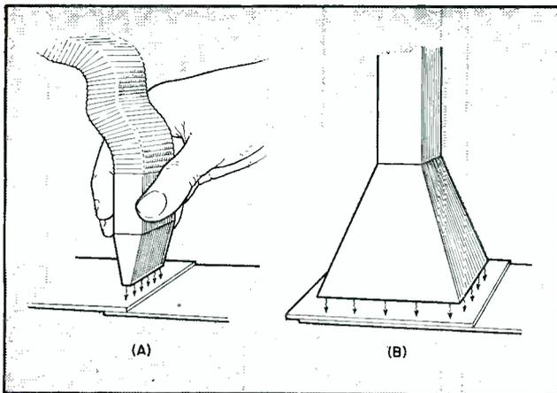
FIG. 5—A method of concentrating microwave energy at a narrow joint by means of a flexible waveguide is illustrated at A, and use of a divergent taper at the waveguide aperture for spreading the heating energy is shown at B
