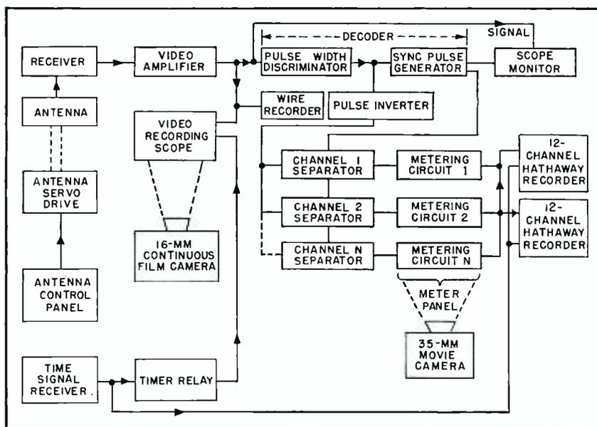
FIG. 2—Block diagram of equipment located in trailer serving as ground station for V-2 telemetering system
