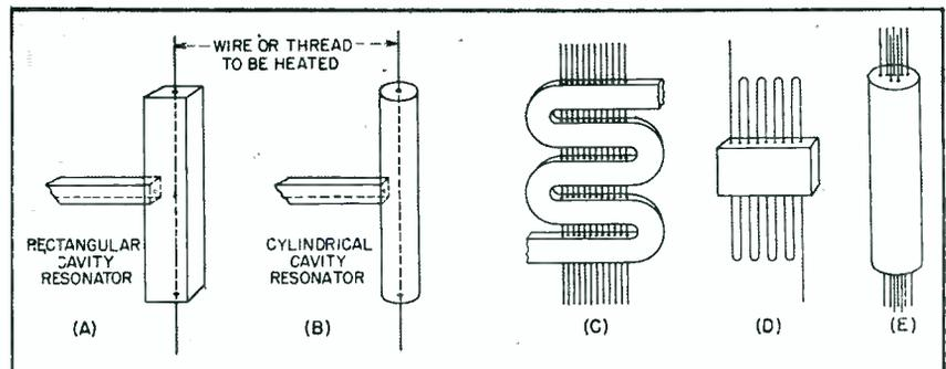
FIG. 2—Five methods to transferring microwave energy from a waveguide to a wire or thread for dielectric heating
