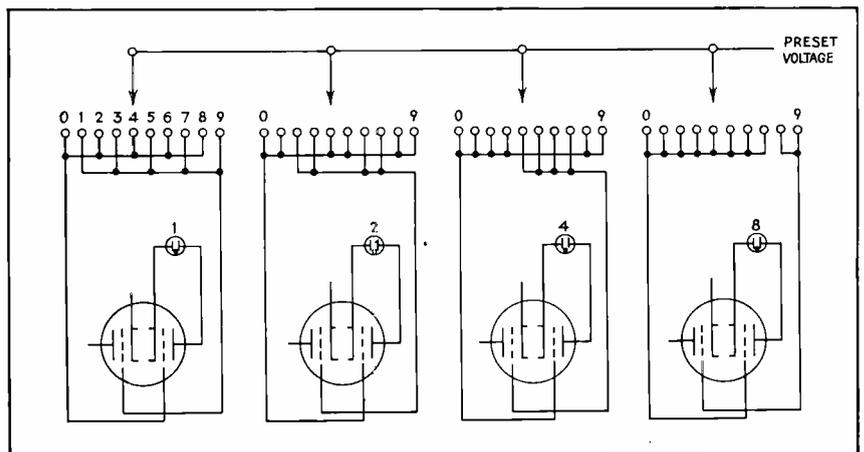
FIG. 3—Switching circuit used for selection of predetermined count on one decade
