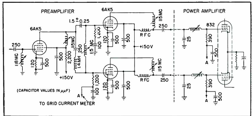
FIG. 4—Preamplifier output, and power amplifier input connections
