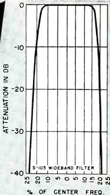
Actual measurements taken on Toroidal Coil Filter manufactured by Burnell & Co.
