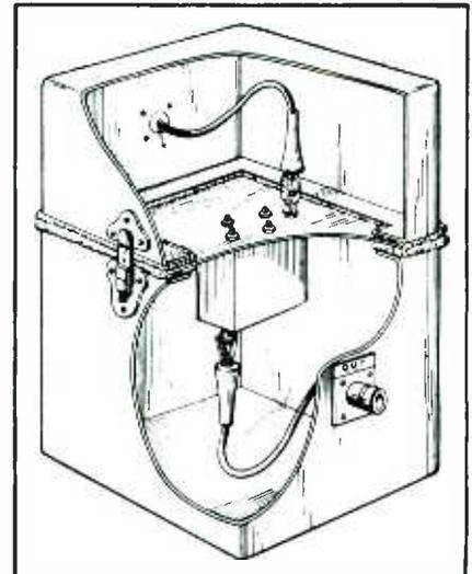
FIG. 2—Filter is mounted on plate inside shield box
