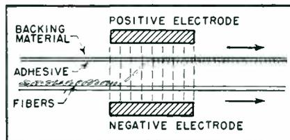
Arrangement of electrodes for electrostatic deposition of fibers to form a pile fabric
