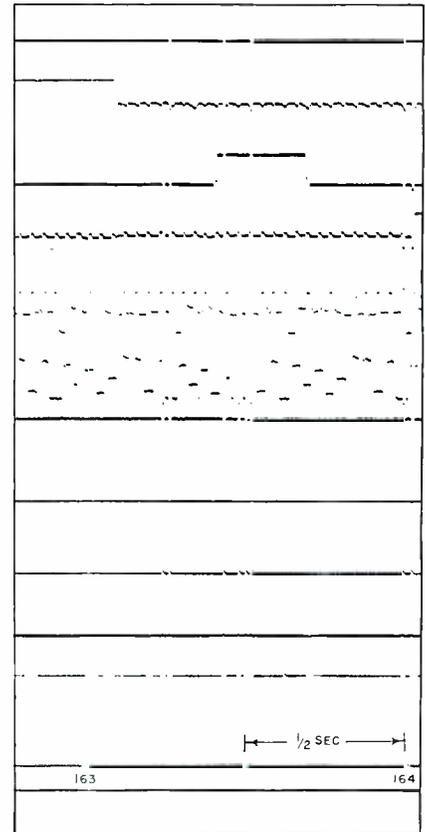
Section of typical telemetering record. Numbers on time reference trace (second from bottom) indicate elapsed time in seconds since takeoff. Time reference pulses are a half second apart
