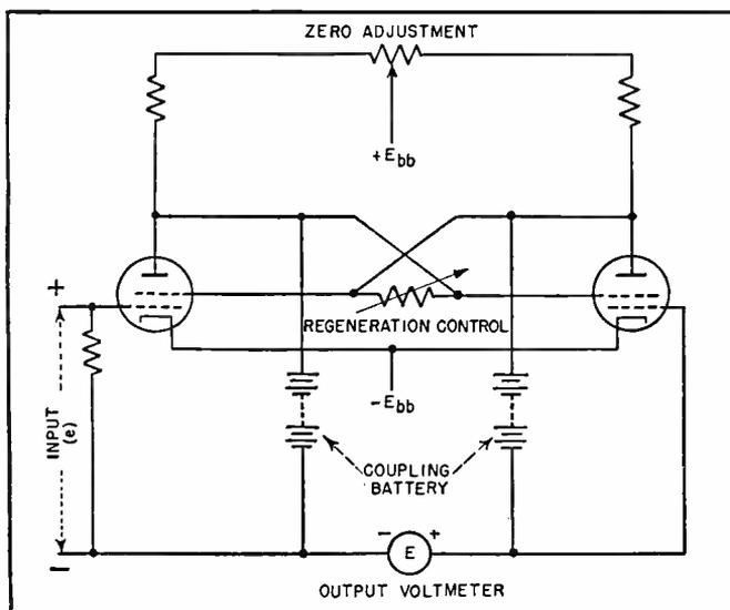
FIG. 2—Regenerative feedback to auxiliary grids increases amplification. Balanced circuit is used to obtain necessary phase reversals
