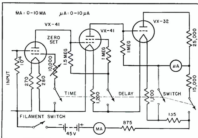
FIG. 3—Circuit of portable instrument for indicating intensity of low-level radiation
