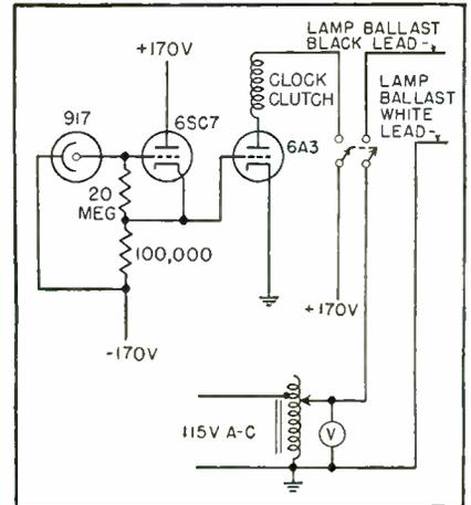
Circuit of phototube relay for time lag measurement
