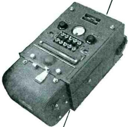
Hathaway Type S12-A 12-element Portable Oscillograph
