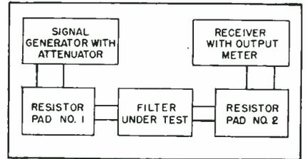
FIG. 1—Basic method of measuring insertion loss of filters is to determine generator output necessary to give same reading of output meter at receiver with and without filter in circuit. Unless complete shielding is used results are not reliable
