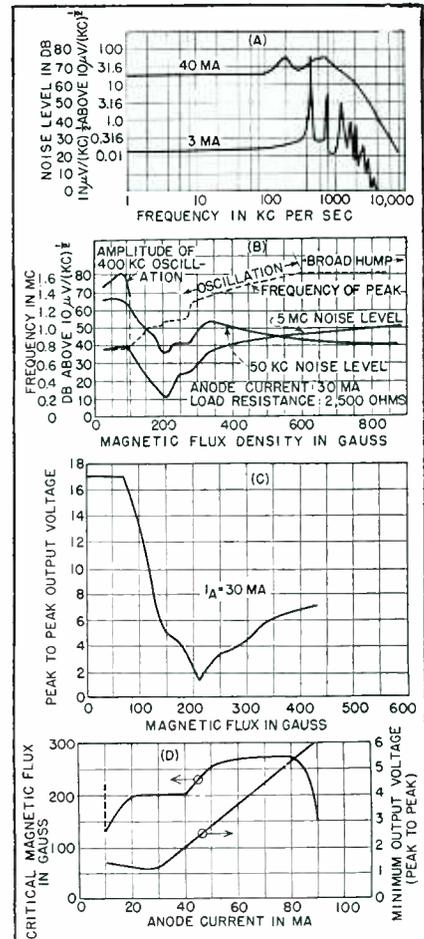
FIG. 1—Noise characteristics of 884 for various operating conditions
