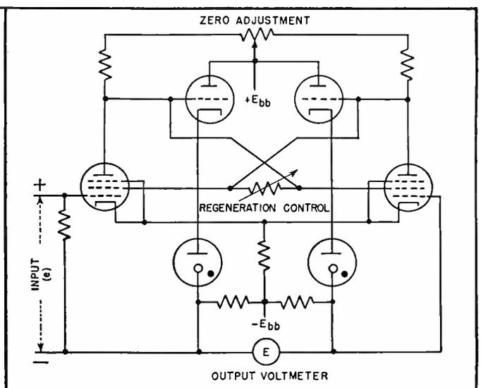
FIG. 3—Practical circuit incorporates cathode-coupled isolation tubes and gas tubes in place of batteries for maintaining proper biases
