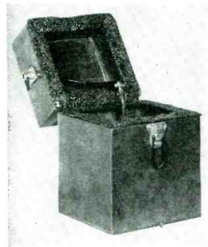
Filter to be measured is placed inside metal shield can
