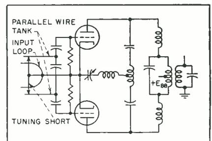
FIG. 2—Triode mixer has balanced input and output and a symmetrical, self-sustaining heterodyning loop
