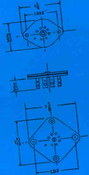
57 A 11 and 57 A 12 Miniature Laminated Sockets have spring type contacts that GRIP and hold the tube securely without the need for locking devices. These contacts, being longer and spaced wider apart, permit greater ease in soldering thus lower production costs. 57 A 12 is interchangeable with Octal Sockets of like mounting center enabling chassis design for use with either.
