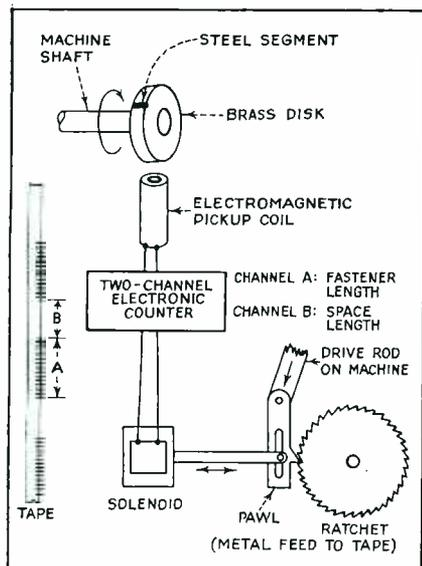
FIG. 4—Arrangement for automatic control of slide fastener machine, using one predetermined channel to control the number of elements inserted in the fastener tape and using the second predetermined channel to control the spacing between sections on the tape
