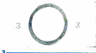
**4. SILMANAL.** High in coercive force, this alloy of silver, manganese, and aluminum is most useful in instruments where service in strong electrical fields is necessary. The Silmanal magnets in illustration 4 were rolled, punched, and machined from the ingot shown. For more information about these magnetic materials, write for Bulletin GES-3337.
