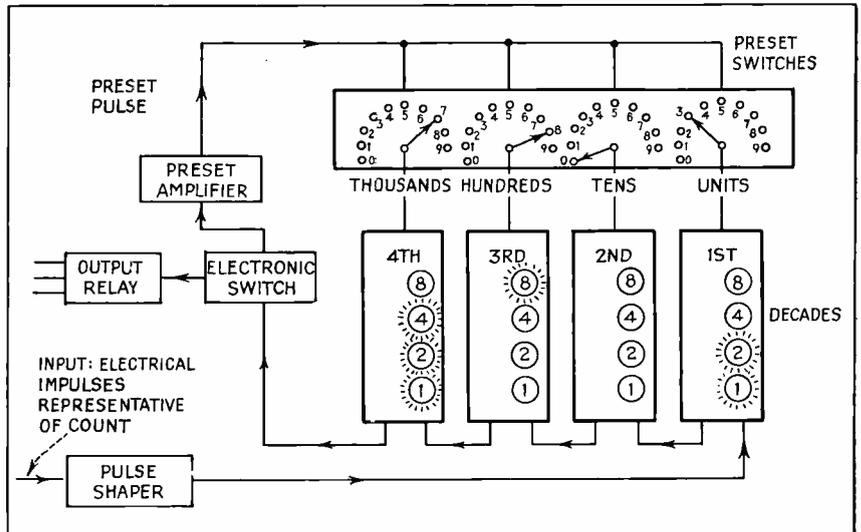
FIG. 2—Block diagram of four-decade single predetermined counter, showing switches and lamps set for starting count of 7803 as required for batching of 2197 units
