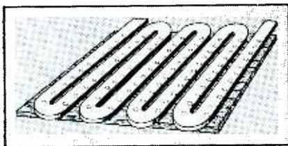
FIG. 3—Arrangement of waveguide with radiating holes for spot-tacking of glue line simultaneously at many points in edge-glued lumber
