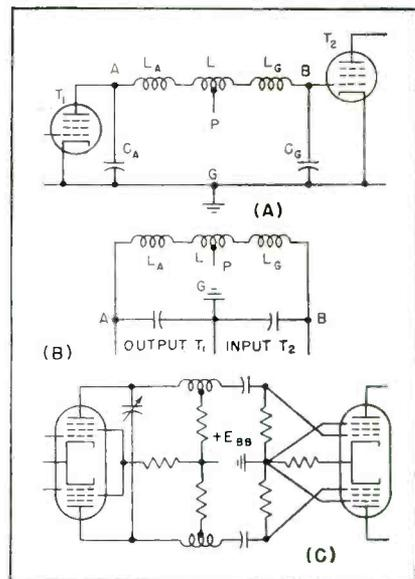
FIG. 1—UHF amplifier coupling network utilizes stray reactances
