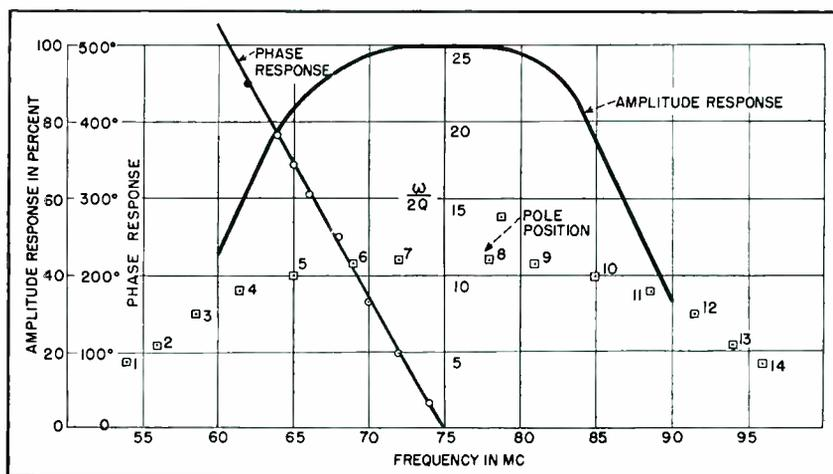
FIG. 8—Receiver i-f amplifier response curve
