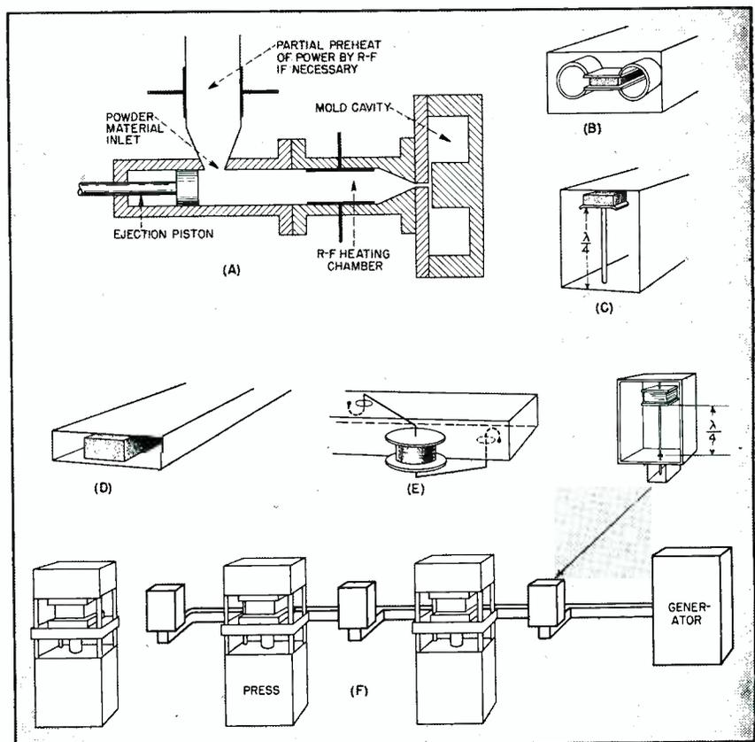
FIG. 4—Suggested methods of utilizing microwave energy in molding of plastics
