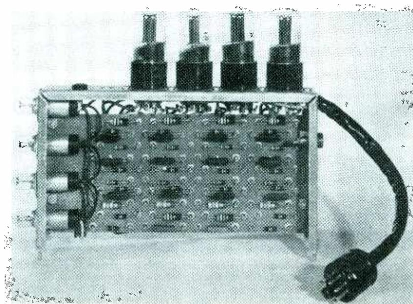
Complete four-tube counter decade, which delivers one output pulse for every ten input pulses
