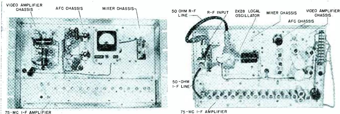
Front (left) and back views of a typical relay receiver chassis
