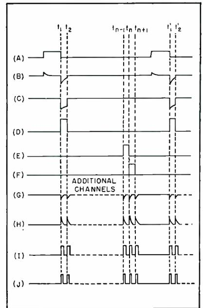
FIG. 4—Waveforms at various points in airborne telemetering circuit of Fig. 3
