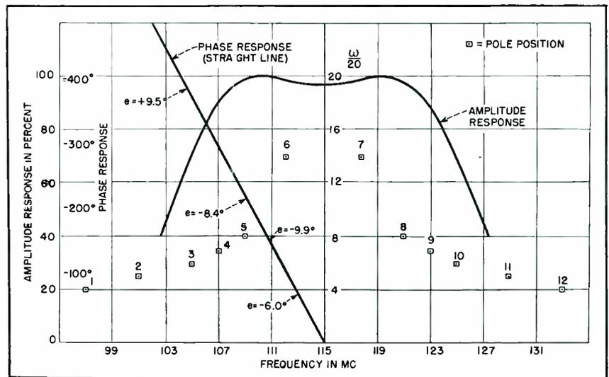
FIG. 5—Transmitter i-f amplifier response curve
