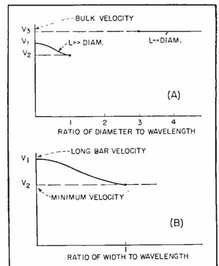
FIG. 1—Variation of velocity of sound with dimensional ratios of solids
