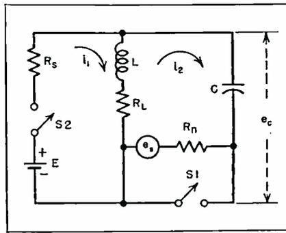
FIG. 4—Equivalent circuit of pulsed oscillator
