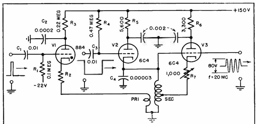
FIG. 2—Circuit of a pulsed oscillator that delivers pulses of high, uniform amplitude
