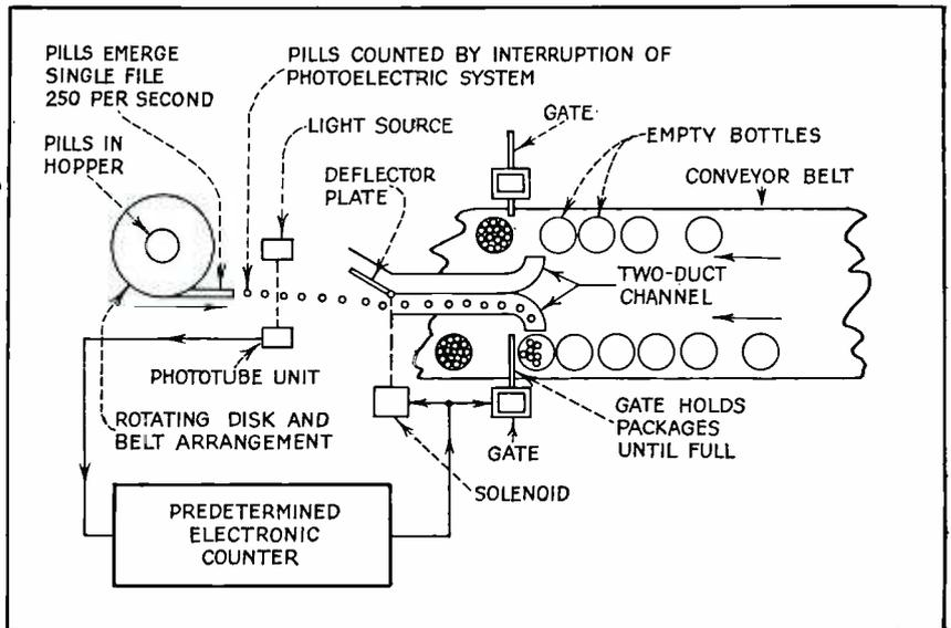
FIG. 1—Method of using single predetermined electronic counter for counting pills at rate of 15,000 per minute and placing exactly the correct number automatically in each bottle on the conveyor belt
