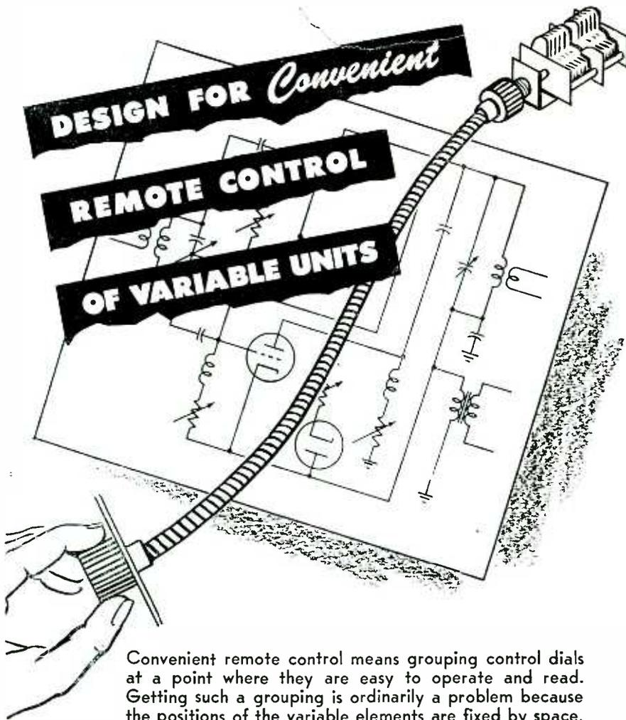
Convenient remote control means grouping control dials at a point where they are easy to operate and read. Getting such a grouping is ordinarily a problem because the positions of the variable elements are fixed by space, circuit, or wiring requirements.
