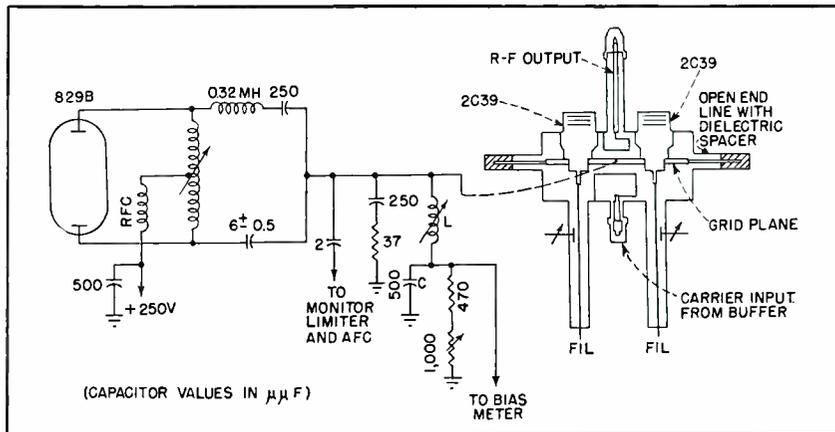
FIG. 7—Heterodyne r-f output stage of the television relay equipment, including part of the preceding i-f amplifier
