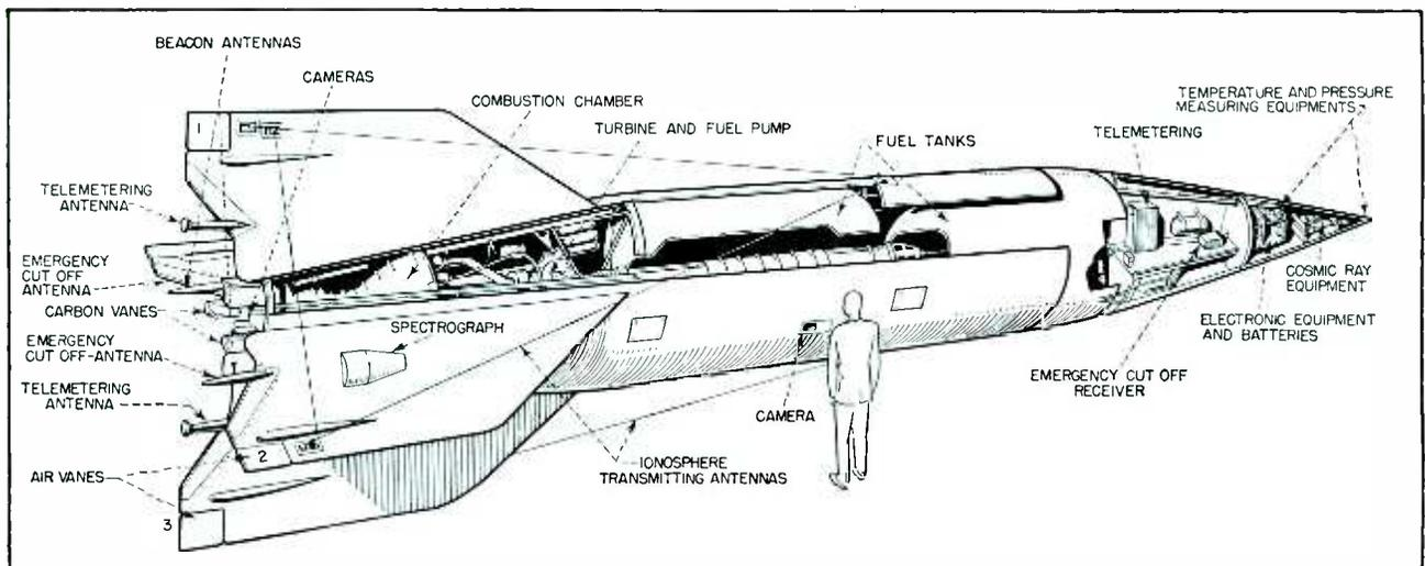
Sketch of V-2 rocket equipped for study of ionosphere, showing location of telemetering unit in nose and telemetering antennas behind tail fins. In the first successful flight made for this purpose, all instruments recorded continuously until the huge missile landed 13 miles away after reaching an altitude of 83.5 miles
