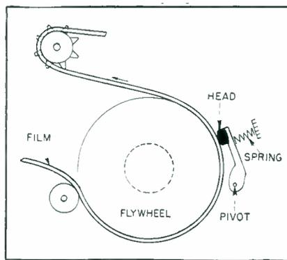
Mounting arrangement for the magnetic pickup head. The pressure against the coating is on the order of 0.0001 ounce
