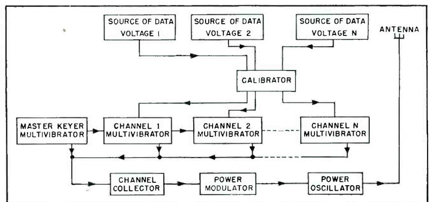
FIG. 1—Block diagram of airborne telemetering unit used in V-2 rockets
