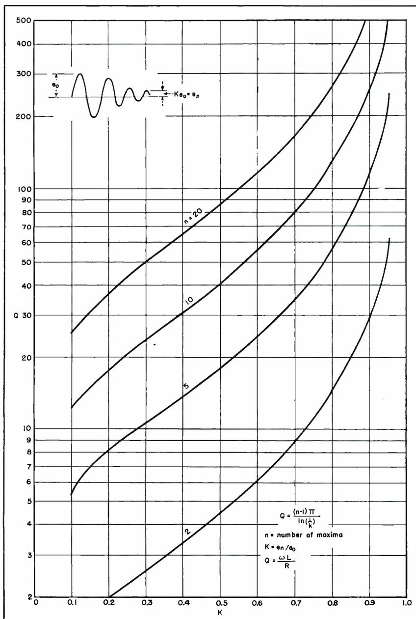
FIG. 5—Graph shows the quality (Q) of a resonant circuit if the oscillations initiated by shock are to decay to a particular fraction (K) of their initial value in a given number (n) of cycles
