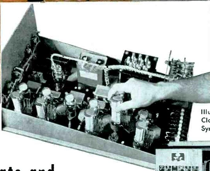
Illustration shows use of Clare Relays in Raytheon Synchronous Control Cabinet
