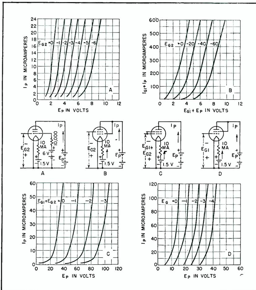
FIG. 2—Transfer characteristics obtained with tube connections shown
