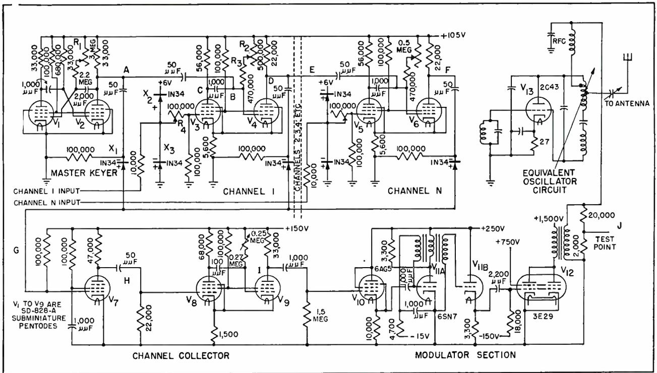
FIG. 3—Circuit of airborne telemetering unit. First and last channels are shown, others being identical
