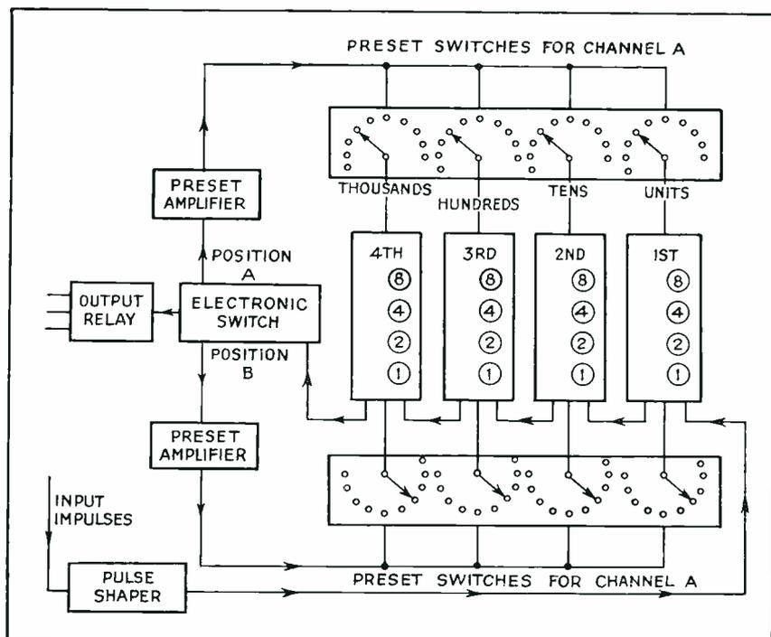
FIG. 5—Block diagram of dual predetermined counter used for high-speed control of two different operations that occur in sequence and recycle continuously
