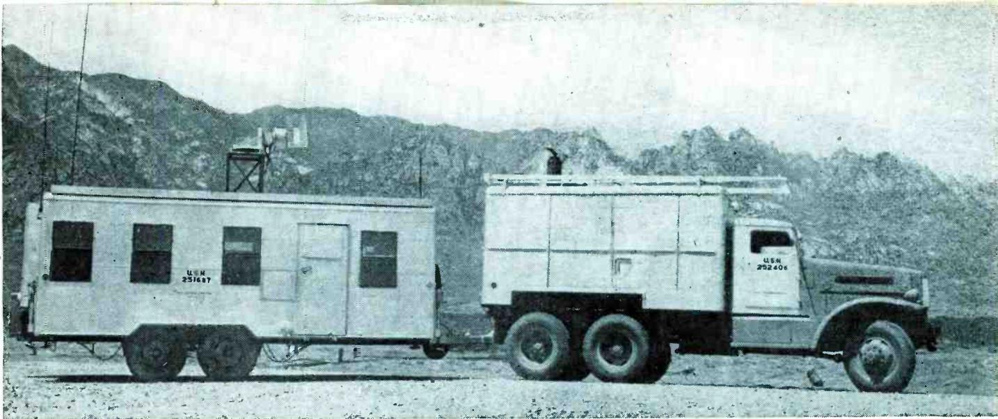
Mobile telemetering ground station. The trailer carries a 1,000-mc receiver, a decoder, recording equipment, monitoring and test equipment, communication receivers and transmitters, and timing mechanisms, while truck contains 25-kw power generator
