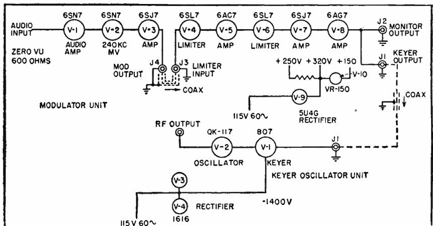
Block diagram of the microwave transmitter. Jacks permit operation as repeater or terminal equipment and allow monitoring of circuits
