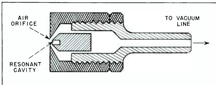
FIG. 2—Cross-section of ultrasonic generator used on automobile. Air gap between orifice and resonant cavity is adjusted for high signal intensity and entire assembly is then locked and soldered
