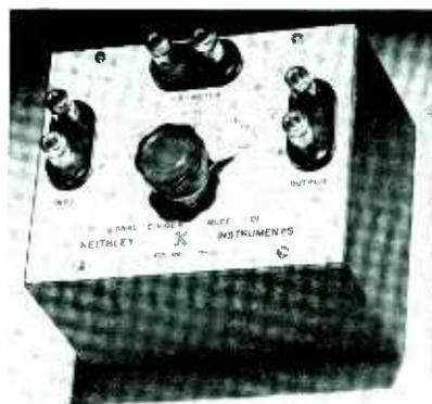
plifiers. Since most laboratory oscillators can be controlled from 0.1 volt to 15 volts, the divider extends the range down to about 10 microvolts. Frequency range is 0 to 200,000 cps and input admittance is approximately 11,000 ohms. Further details are available in bulletins issued by the manufacturer.
