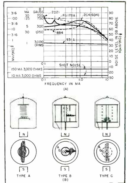
FIG. 2—Characteristic noise from several types of gas tubes
