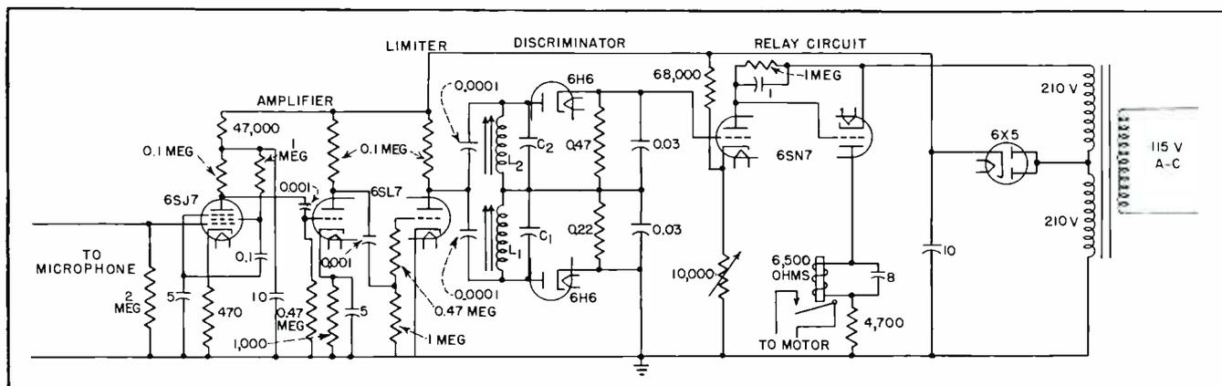
FIG. 1—Complete circuit of amplifier used in supersonic door-opening system
