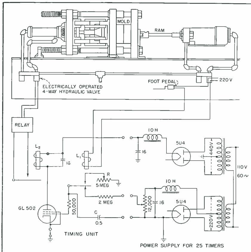
Circuit of one timing unit and the common power supply
