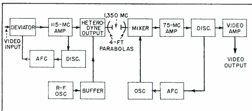
FIG. 1—Block diagram of studio-to-transmitter link equipment, showing video transmitter, at the left, receiver at the right, and the radio path between them
