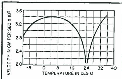
FIG. 2—Variation of longitudinal velocity in 45-degree X-cut Rochelle-salt crystal with temperature
