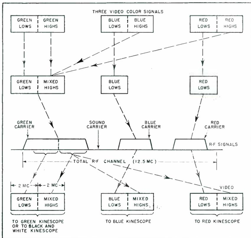
FIG. 1—By transmitting all fine detail of the image through the green channel, RCA mixed-highs system reduces bandwidth requirements of simultaneous system by 2mc. achieves effect of black plate in color printing.
