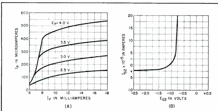
FIG.1—(A) Diode characteristics with both grids connected to plate indicate cathode emission characteristic. (B) With 10 milliamperes filament heating current, 250 microamperes first (space charge) grid current, and 10 microamperes plate current, this second (control) grid input characteristic is obtained
