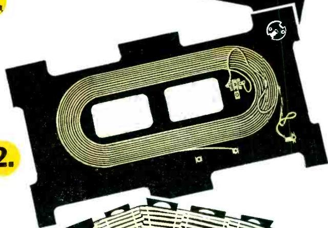
**1.** Multi-band combination loop Antenna and Radio Back.
