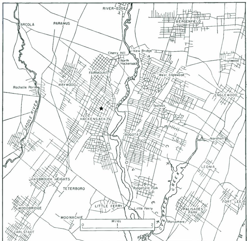
Map showing area of taxi operations covered by 15-watt transmitters. Location of fixed station transmitting and receiving antenna about 90 feet above sea level is indicated by star. Some areas served are behind elevations exceeding that of this antenna
