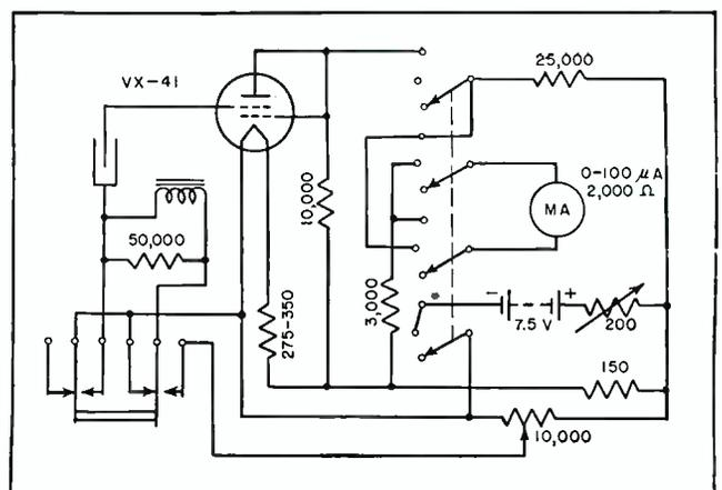
FIG. 4—Cumulative x-ray radiation is indicated by this direct reading integrating meter
