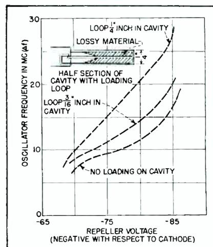
FIG. 3—Typical reflex klystron oscillator tuning response with various degrees of loading
