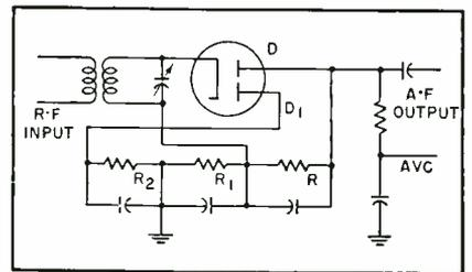
Second anode of detector diode is used to develop noise suppression voltage
