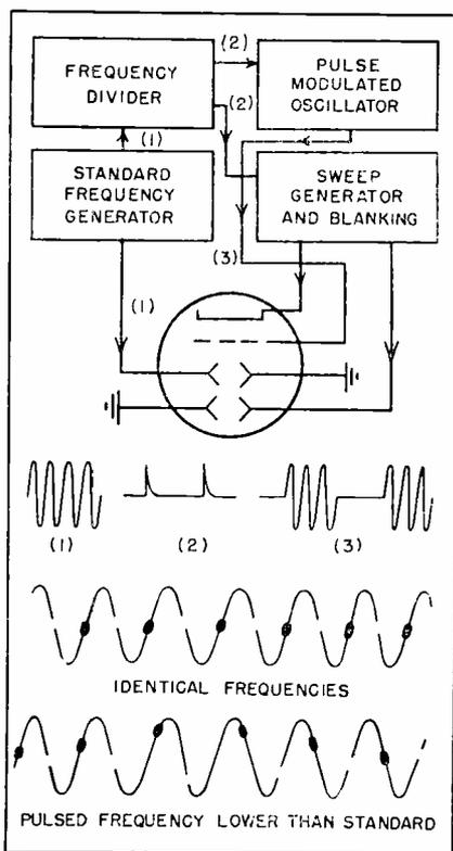
FIG. 3—Using the method shown at the top, the patterns shown below are obtained to indicate the frequency of the pulsed oscillator
