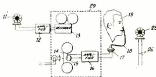
chanically applying vibrations of audible frequencies to the skin of a human in the region of the throat, to cause the air within the vocal cavities to vibrate. Oct. 10, 1938 and March. 27, 1939.
