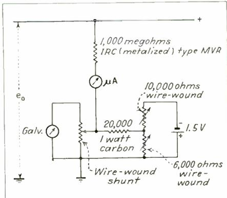
Fig. 3—Galvanometer circuit for measuring small changes in the output voltage
