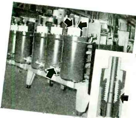
**FOR MERCURY-ARC RECTIFIERS**—The cut-away inset is a mercury-arc rectifier seal using compression-molded G-E mycalex. Metal can be cast around this insulator without softening, blistering, or otherwise affecting its structure.
