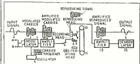
Fig. 2—Block diagram of the recorder and reproducer showing the functions of the various parts
