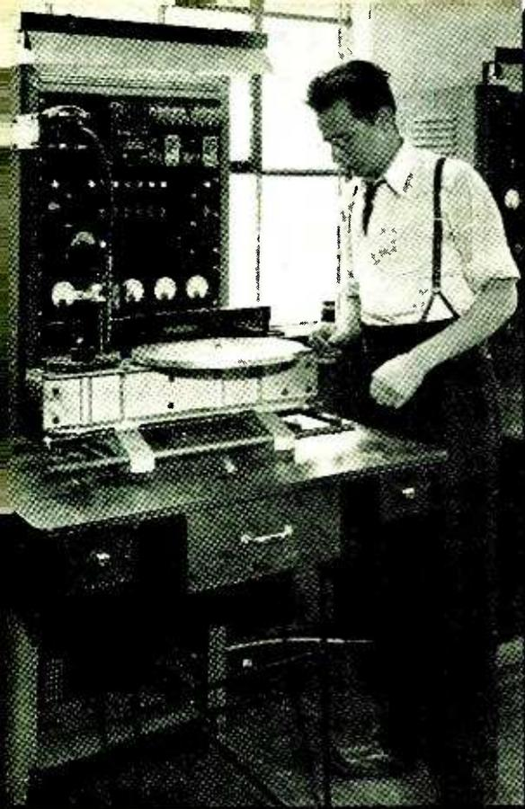
The Fluxgraph in use. The turntable carrying the coil under test may be seen at the left. A paper disc is in place on the turntable at the right
