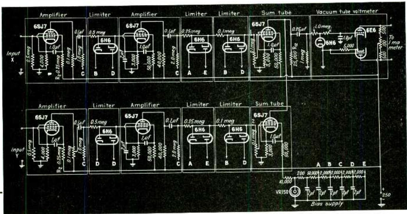
Fig. 3—Circuit diagram of the electronic phase-angle meter. Each sine-wave signal is fed into an amplifier and limiter channel and the outputs of the final limiters have a common load
