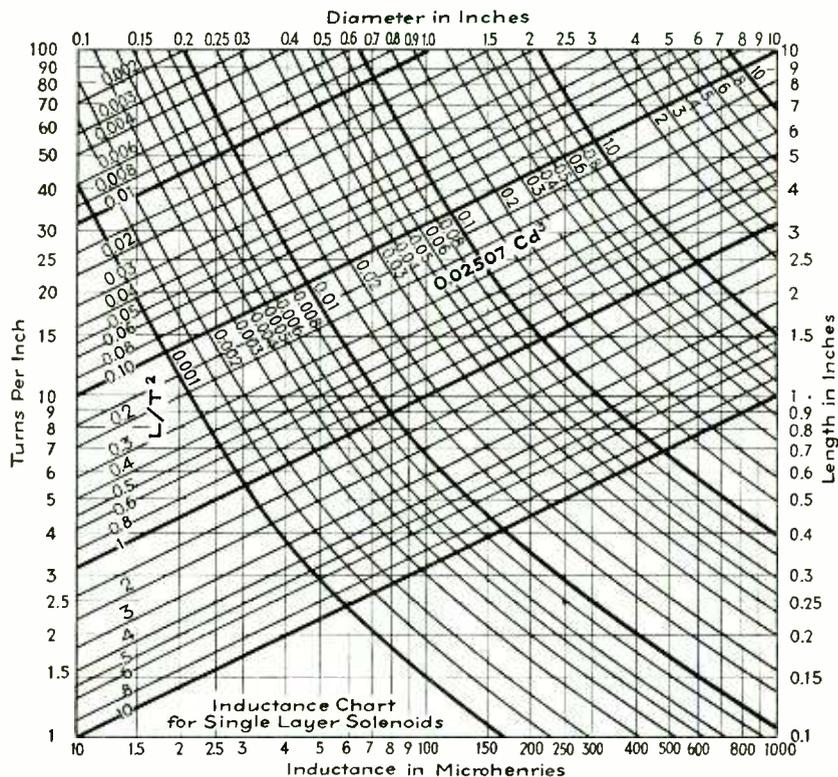
Graphical plot connecting all inductance factors for single layer coils and sufficiently accurate for most purposes
