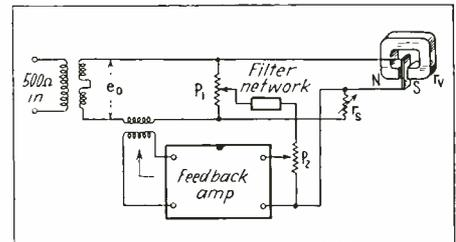
Fig. 2—Feedback applied to a light-valve circuit
