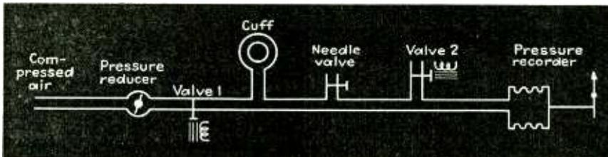
Fig. 3—Diagram of the air pressure system. Valves 1 and 2 are electronically controlled
