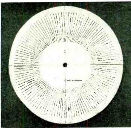
FIG. 1—Plot of typical test coil when using pencil lead as a Fluxgraph recording stylus
