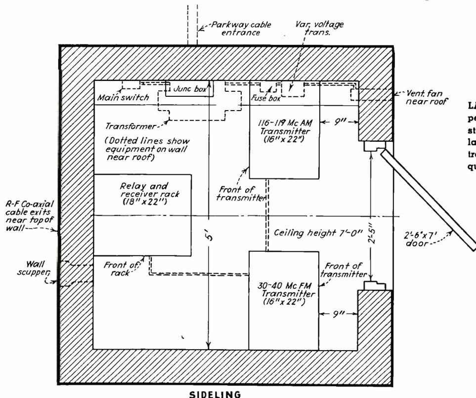
**LAYOUT**—Plan view of typical hilltop repeater equipment house. All six repeater stations have 116-119 Mc amplitude modulated transmitters and combination control receiver and relay racks. The frequency modulated transmitter is omitted at Tuscarora and Ray's
