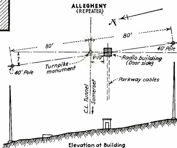
**PLAN AND ELEVATION**—Allegheny Mountain's repeater station equipment house is located high on the hilltop, as near the turnpike's right-of-way center line as terrain permitted. Antenna poles are set up near the north and south right-of-way borders. Note east-west line showing tunnel far below. Poles are placed broadside to the paths followed by repeater signals
