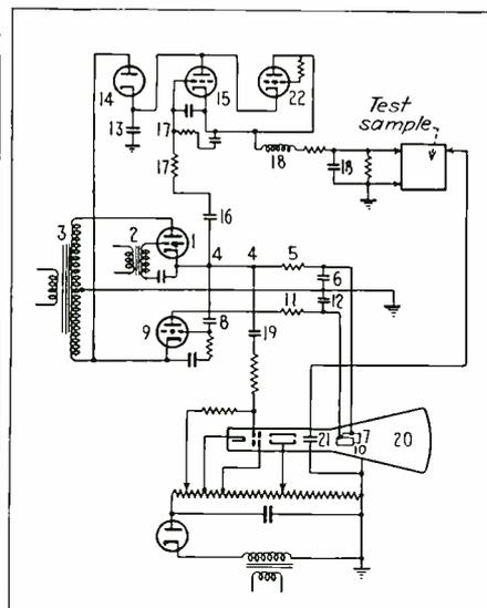
Fig. 1—Diagram of the surge generator, sweep circuit, and cathode-ray oscillograph
