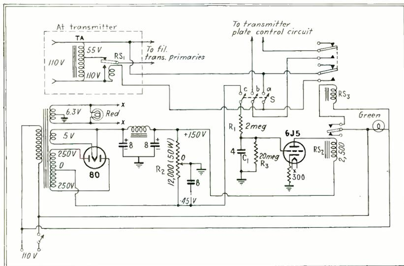
Circuit of automatic filament control device. Condenser *C*<sub>1</sub> should have low leakage and in the WQOC unit is oil filled
