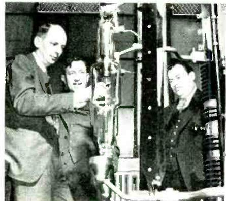
Millionth of a second x-ray pictures through one inch of steel armor plate are made possible by this twin tube unit operating at 300,000 volts and 2,000 amperes in the Frankford Arsenal. Dr. C. M. Slack of Westinghouse explains its operation to Dr. Herschel Smith, civilian aide at the Arsenal, and an assistant
