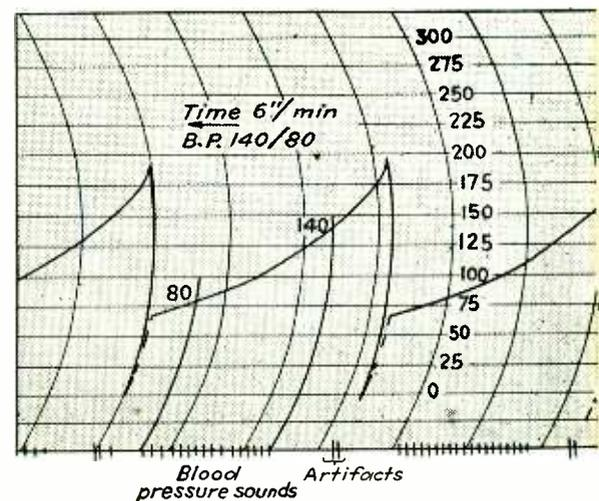
Fig. 2—A celluloid arc is required for reading the pressure record by the method illustrated here
