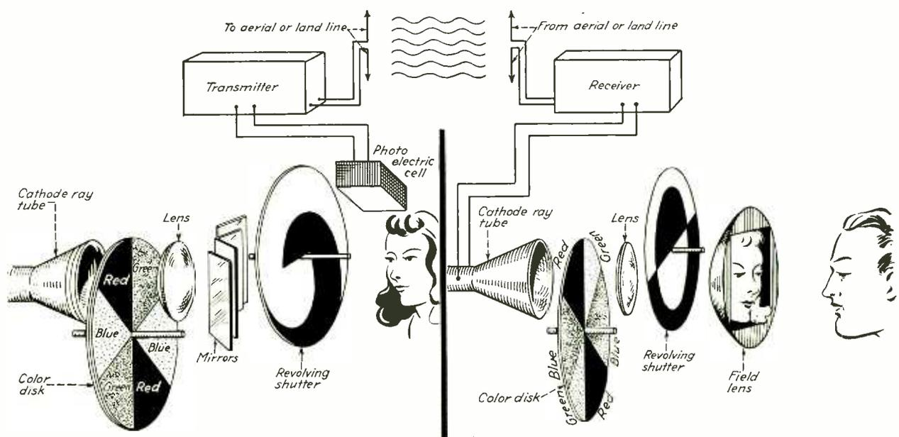
Schematic pictorial diagram of the elements of the stereoscopic color television system developed in England by Mr. Baird
