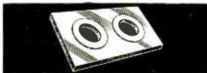
Spring insulators are made from special heat treated Bakelite that permits punching without cracks or checks and possesses minimum cold flow and low moisture absorption properties. Each Type K Relay is given a 1000 volt a. c. insulation breakdown test.
