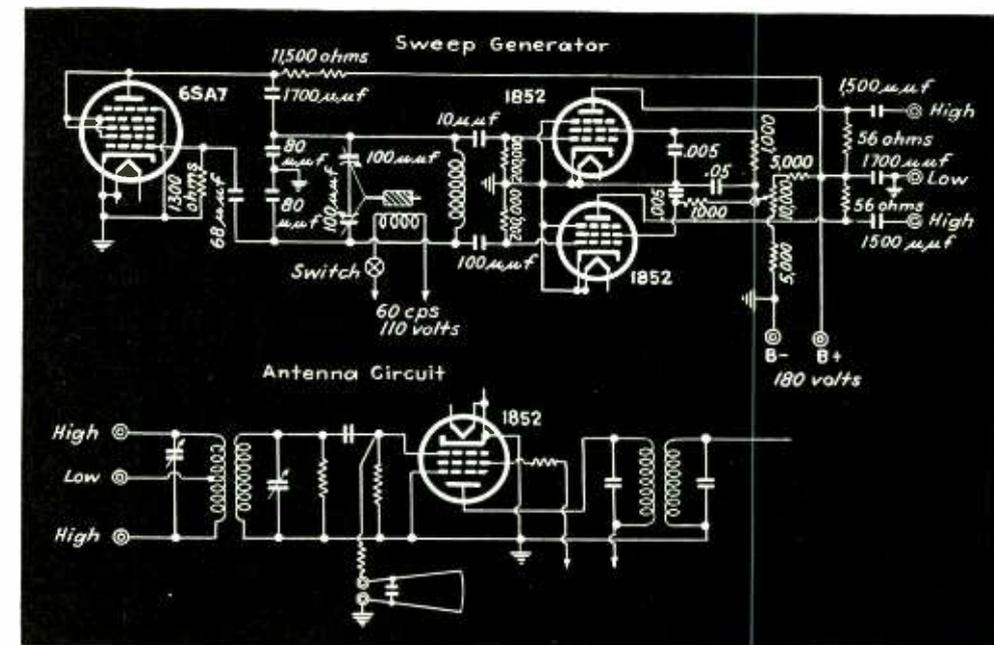
Fig 1. Circuit diagram of the sweep generator together with typical band pass amplifier tested by its means
