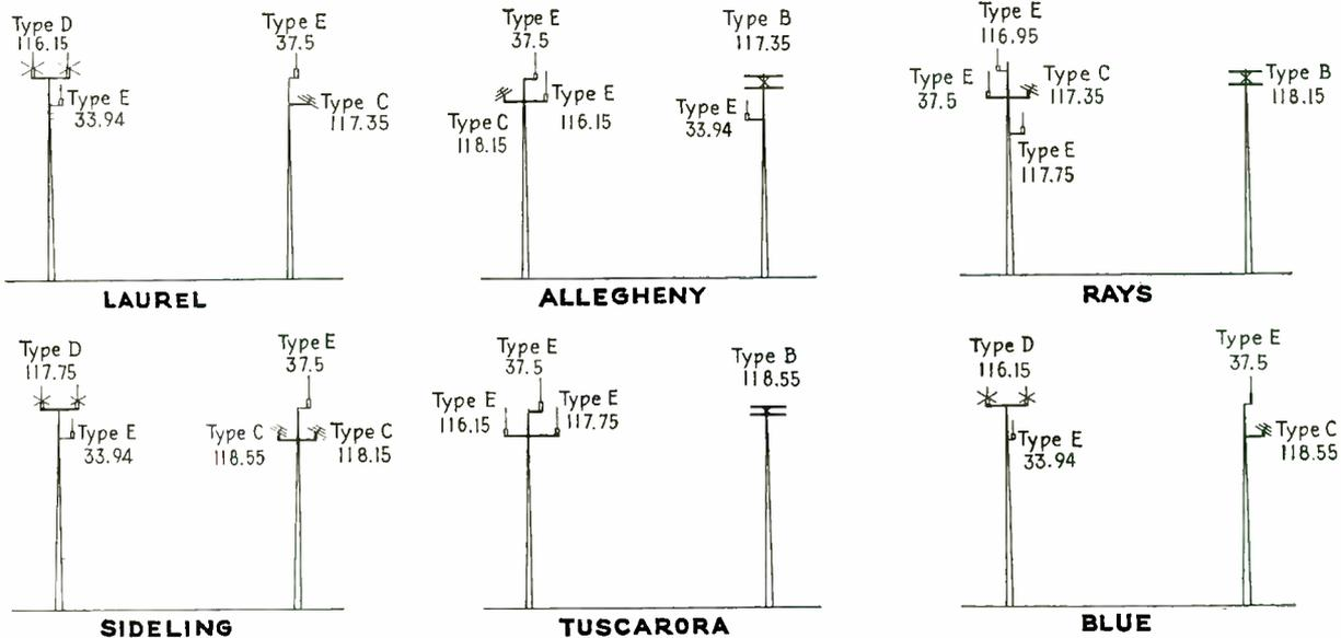
**REPEATERS**—The six hilltop stations have two 40 ft. poles apiece, with 116-119 Mc relay receiving and transmitting antennas on the separated poles to minimize interaction. Antennas feeding 37.5 Mc amplitude modulated repeater control receivers and
