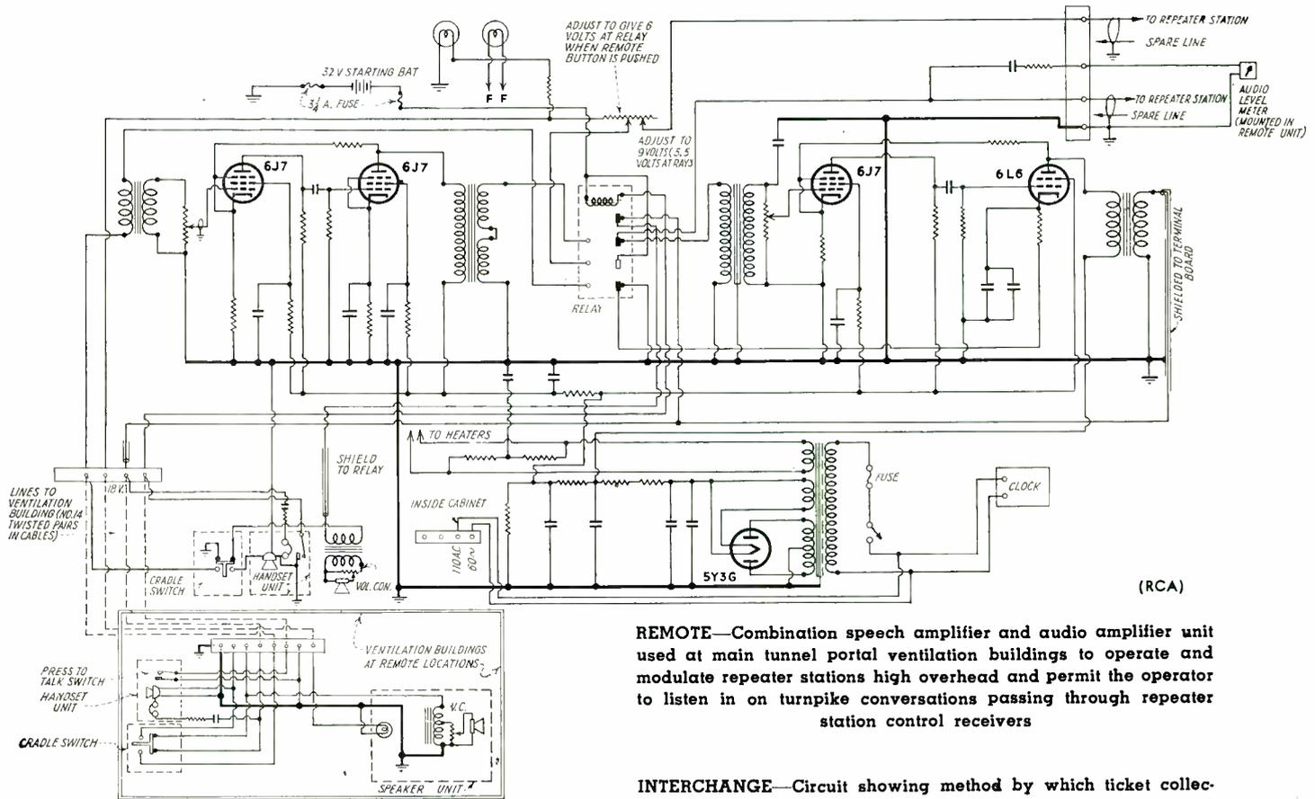
**REMOTE**—Combination speech amplifier and audio amplifier unit used at main tunnel portal ventilation buildings to operate and modulate repeater stations high overhead and permit the operator to listen in on turnpike conversations passing through repeater station control receivers
