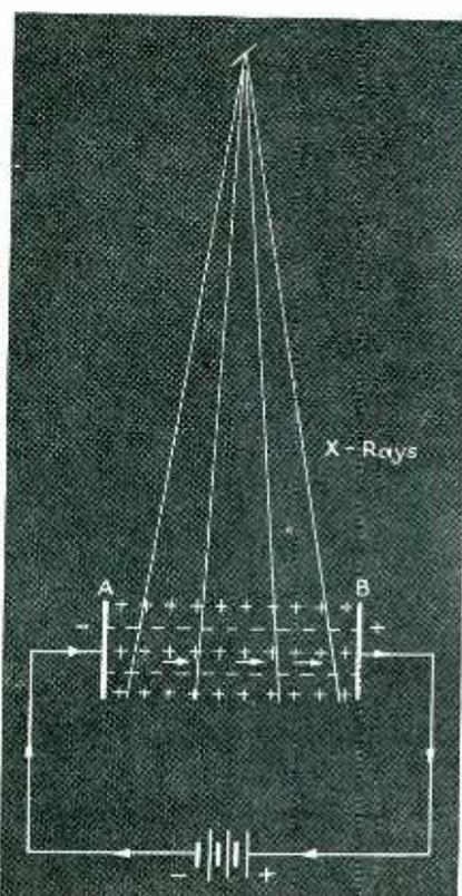
Fig. 4—Diagram showing the presence of positive ions and negative ions (direction shown by arrows) in the chamber
