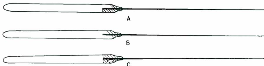
Fig. 2—Typical imperfect joints in the knives. The presence of less than the normal amount of solder causes the knife to be rejected
