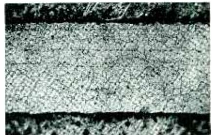
Fig. 4—Section after drawing into wire form
