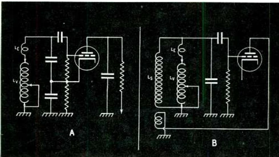
Fig. 10—Two basic oscillator circuits suitable for inductive tuning. *A*, the Colpitts circuit is a two terminal oscillator to which the feedback ratio is dependent only upon the capacitance ratio. *B*, the tickler feedback circuit uses a shunt inductor which may also be used as the parallel tracking coil
