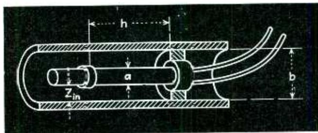
Fig. 4—Structure of the "coaxial" water-cooling assembly. The water enters and leaves the assembly at ground potential
