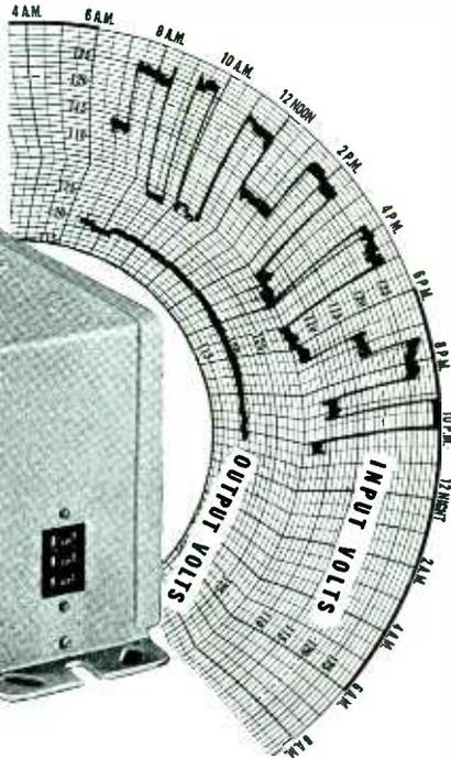
son Automatic Voltage Regulators write for Catalog SD-422. Above chart shows actual line voltage fluctuations over 14 hour period and corresponding regulated output delivered by a Thordarson Automatic Voltage Regulator.
