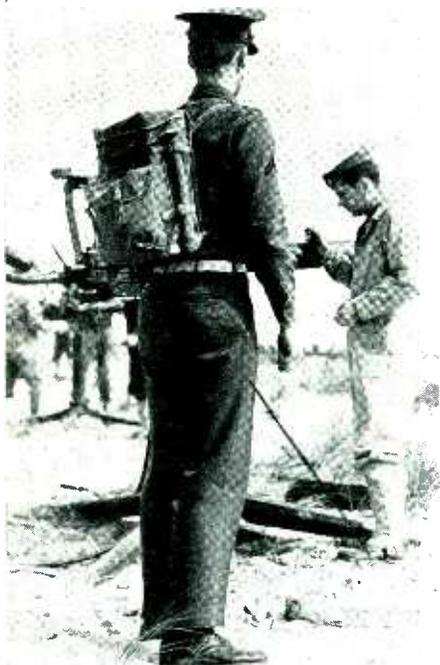
Soldier carrying Walkie-Talkie radio apparatus, used by the 62nd Coast Artillery during fire practice at Fort Tilden, N. Y., in which 50-calibre guns were used. By means of this portable equipment, two-way voice conversation can be carried on between observer on the ground and a plane which tows an aerial "sleeve" target for gun fire
