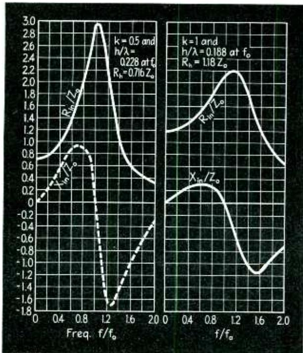
Fig. 12—Left, impedance variation as a function of frequency, based on the specified values of  $k$  and relative length. The impedance is critical near the resonant frequency. Fig. 13—Right, impedance variation curve for other parameter values, showing flatter characteristic, that is, less reactive effects
