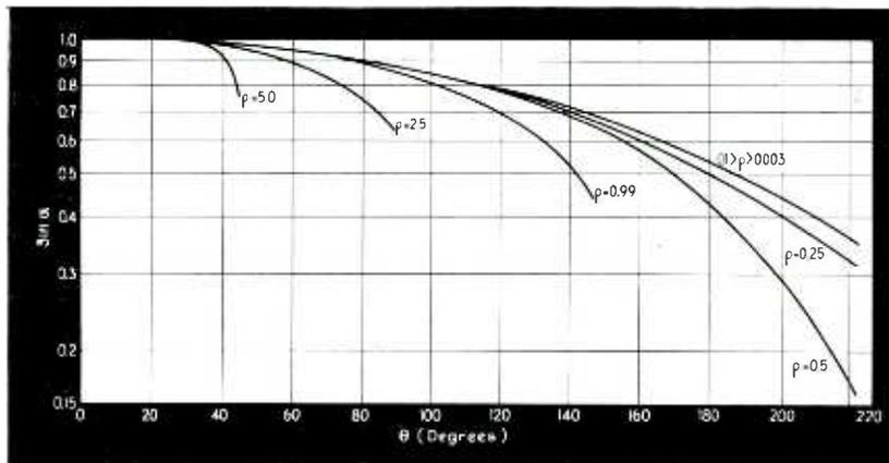
Fig. 5—The sine of the starting angle versus conduction angle
