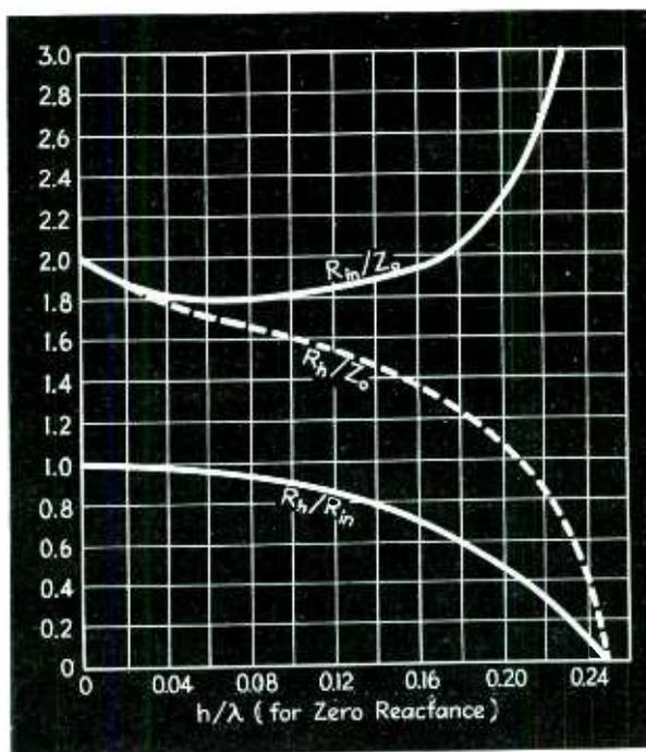
Fig. 5—Graphical data for designing a resistor to have zero reactance at a given frequency
