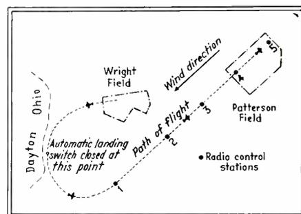
Fig. 3—Path of flight during an automatic landing
