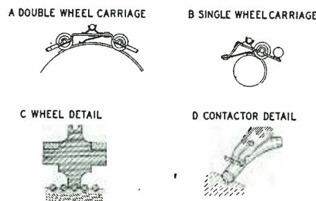
Fig. 2—Details of the method of making contact. The single wheel carriage has the advantage over the double wheel unit of approaching much closer to the high frequency end of the coil
