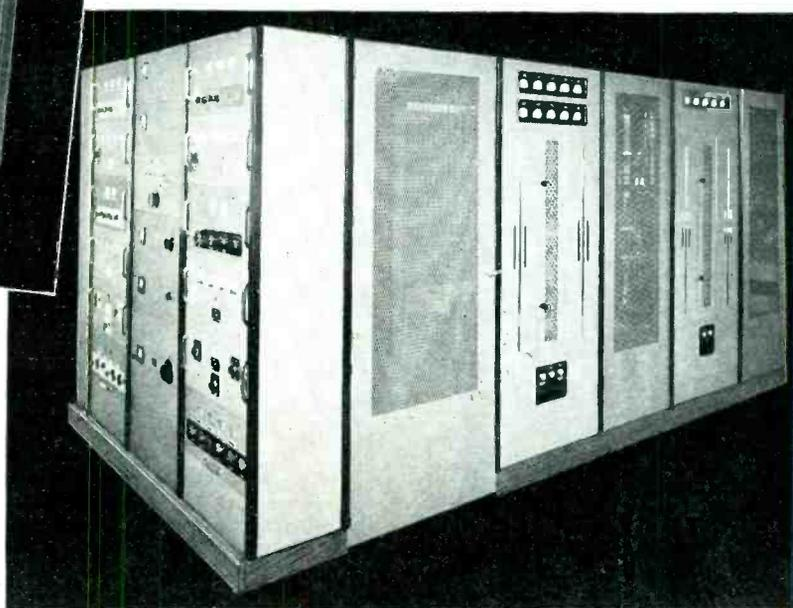
The first F-M relay transmitter (250 watts at 156 Mc) in the World, installed by R.E.L. for the Yankee Network in Boston, Mass., relaying to Paxton, Mass. (45 miles, airline) and in operation 16 hours daily since May, 1939.
