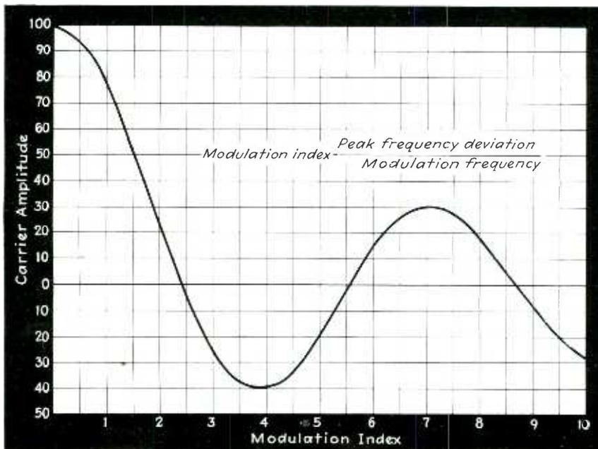
Fig. 2—Method of calibrating the frequency deviation scale of the instrument. The carrier voltage goes to zero periodically, as the modulation level and frequency deviation are increased (after Crosby)
