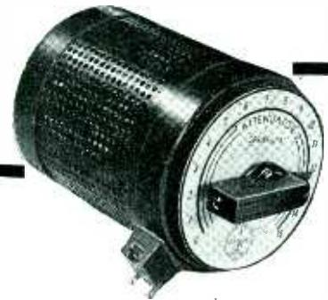
For distortionless control of loud-speaker volume, Clarostat offers its Series CIA constant-impedance output attenuator. 25-watt dissipation at any setting. Linear up to 45 DB in 3 DB steps. Constant input and output impedance because of compensated ladder-type network. Infinite attenuation at end position. With or without power switch. Also available in CIB series; 10 watt dissipation; smaller size.
