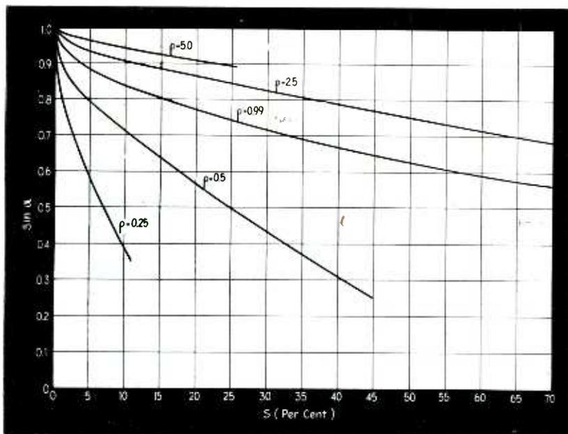
Fig. 4—Chart of the sine of the starting angle versus ripple voltage for large ripple voltages
