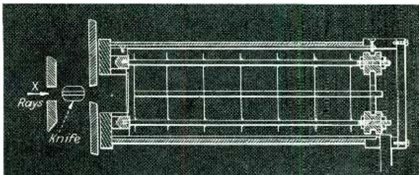
Fig. 7—Cross section of the ionization chamber showing the knife in place for inspection. The metal plates in the interior of the chamber increase the number of ions available to operate the relay
