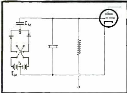
Fig. 1—Diagram of the basic circuit of the variable resistance crystal oscillator
