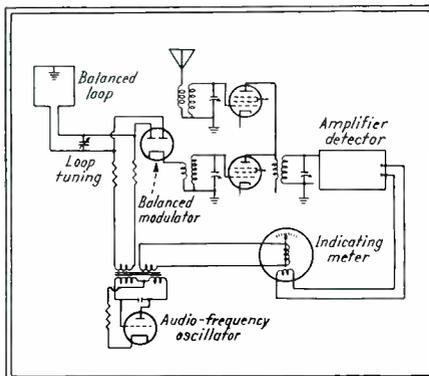
Fig. 2—Simplified circuit diagram of the radio compass
