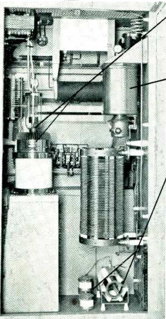
★ **THE 892-R POWER** amplifier tube, air-cooled, is easily reached when the rear door of the radio frequency power amplifier cubicle is opened.
