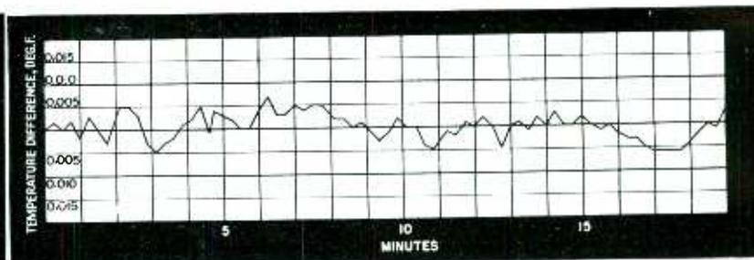
Fig. 4—Temperature stability curve of the Resistotherm regulator. The temperature is maintained well within 0.10 degree F
