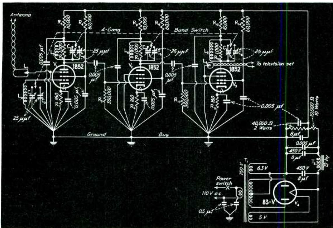
Fig. 2—The circuit diagram of the amplifier. By varying the values of the resistors shunting the tuned circuits, the gain may be varied approximately inversely as the bandwidth covered
