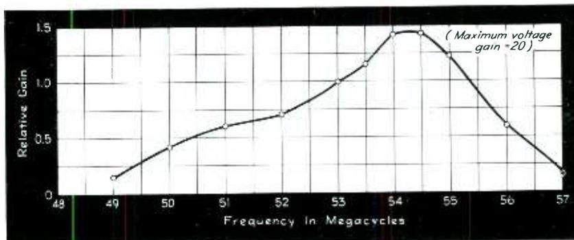
Fig. 4—Overall response characteristic of the television preamplifier, using damping resistors of ohms. Over the picture sideband, the gain varies about plus or minus 3 db, with a maximum gain of 20
