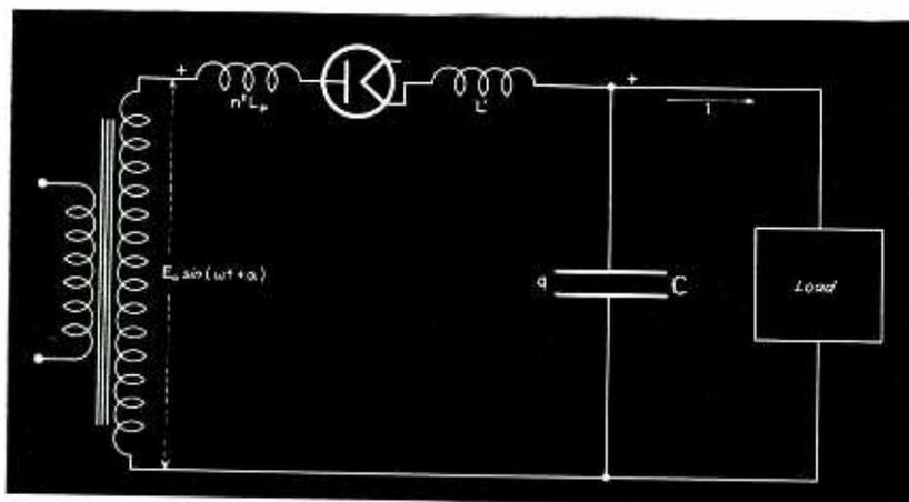
Fig. 1—Single-phase half-wave rectifier circuit on which the solution is based
