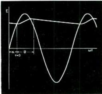
Fig. 2—Left, input and output voltages of the rectifier, showing starting phase angle and conduction angle. The series choke prolongs the condenser charge
