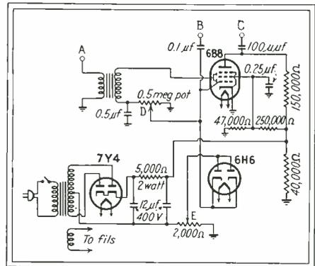
Circuit of a simple electronic attenuator
