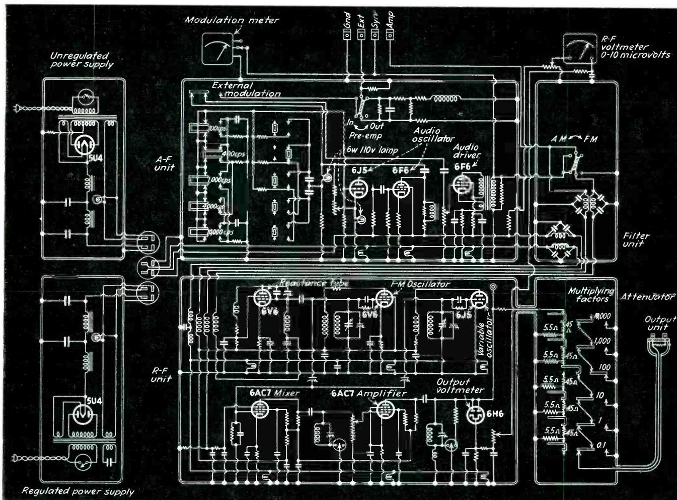
Fig. 4—Circuit diagram of the signal generator. Two alternative power supplies are shown, one (the lower) incorporating a voltage regulation power transformer
