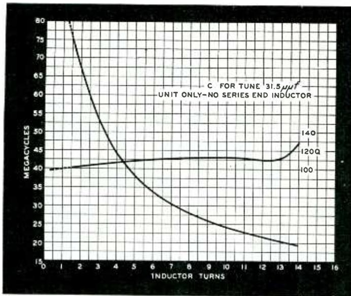
Fig. 7—Curve showing the Q of the Inductuner. Except for the portion of the curve between 13 and 14 turns the Q varies less than 10 per cent
