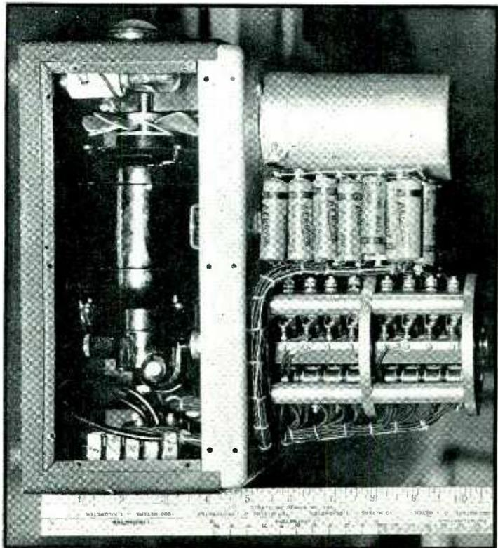
Fig. 6—Contactor unit of the timing source. The amplifier supplies power to the synchronous motor which drives the contactor
