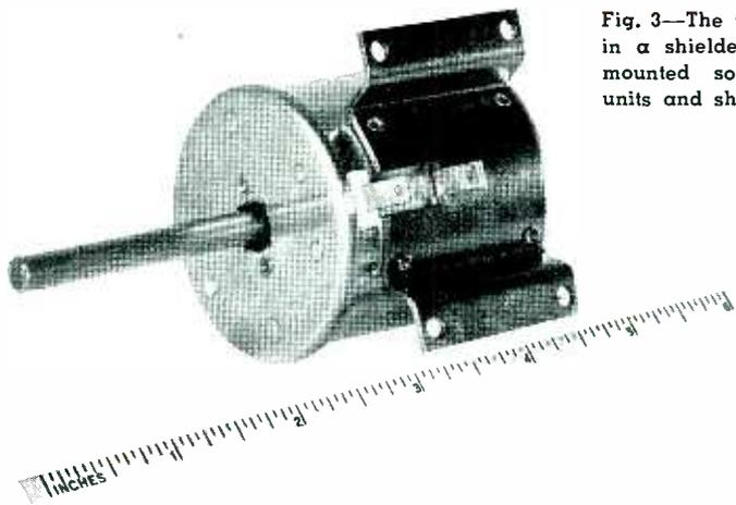
Fig. 3—The tuning unit is contained in a shielded unit which may be mounted so that closely spaced units and short leads may be used
