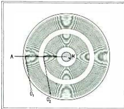
Fig. 1—Stereophonic record showing two sound tracks
