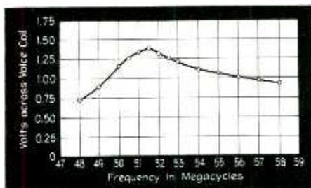
Fig. 3—Calibration curve of the communications receiver used to determine the overall gain of the television preamplifier
