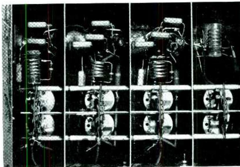
Fig. 5—Tuned circuits and shielding construction. The parts are mounted as near the tube bases as possible
