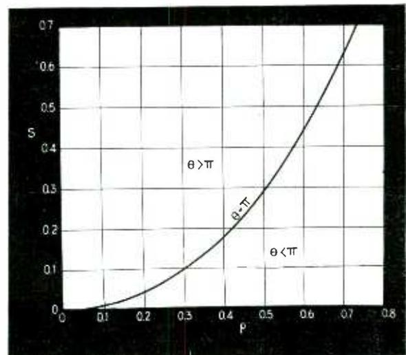
from these figures the angles  $\alpha$  and  $\theta$  can be read directly as functions of arbitrary design parameters.
