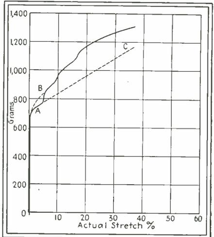
Fig. 1—Per cent stretch measured in terms of stretching force
