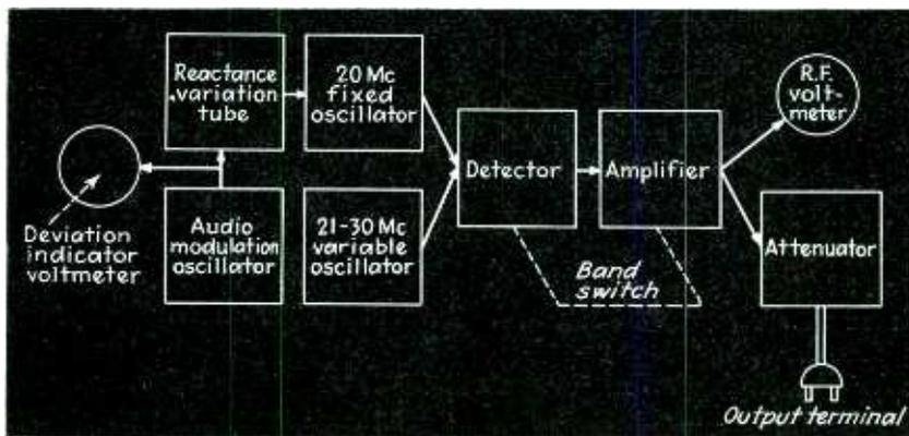
Fig. 1—Block diagram of the signal generator, showing the method of combining two oscillator outputs, one of which is frequency modulated
