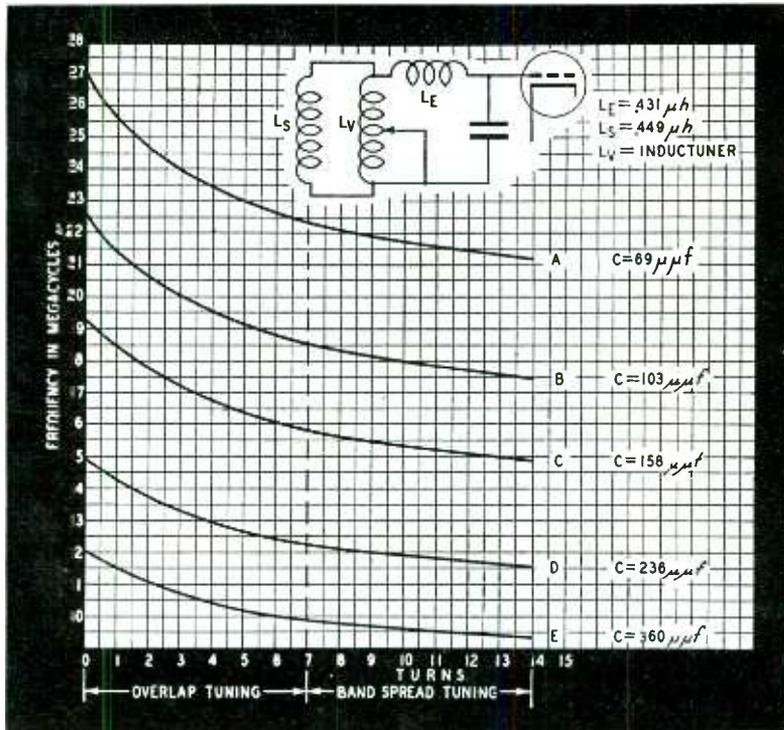
Fig. 11—Circuit which allows expanded band spread tuning. The constants chosen so that a number of short wave bands are covered using one half of the tuning motion and the other half is used to overlap the adjacent band
