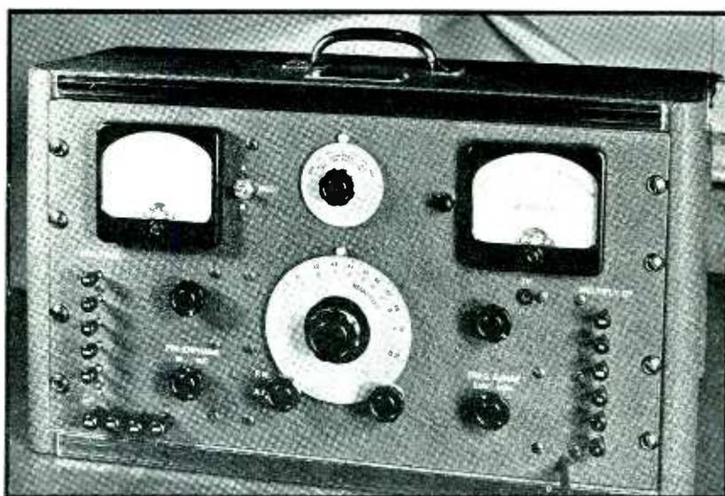
External appearance of the generator. Push button selection of the audio modulation frequency and output voltage level is provided
