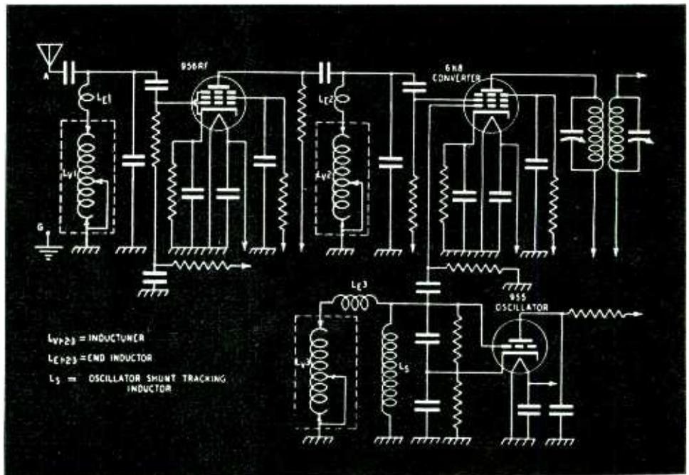
Fig. 9—Typical receiver circuit using inductance tuning units with the oscillator frequency on the high side of the signal frequency
