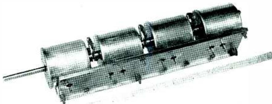
Fig. 5—A four gang unit with insulated couplings. It is necessary to use insulated couplings to avoid undesirable circuit coupling at ultrahigh frequencies
