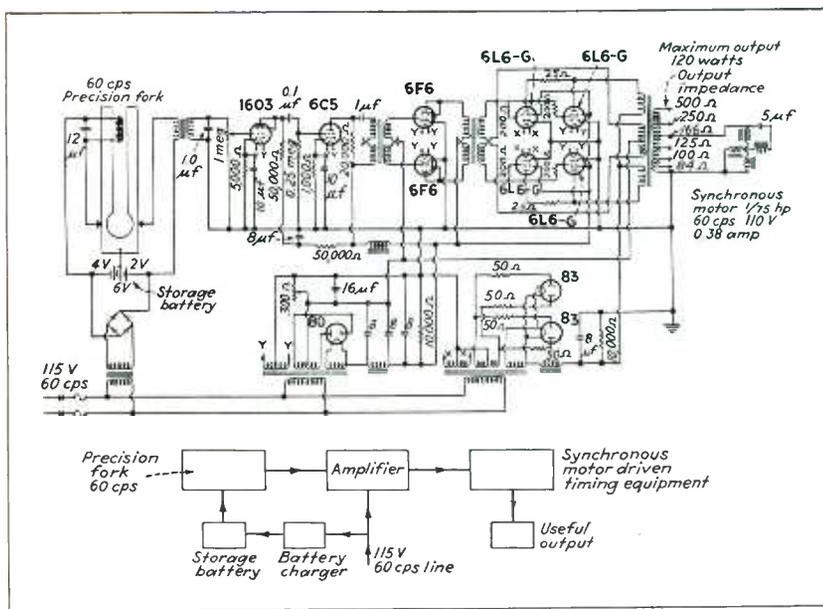
Fig. 5—Circuit diagram of the precision timing source for 60 cycles per second current. This unit is capable of driving 48 magnetic counters calibrated in seconds and tenths of seconds
