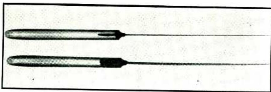
Fig. 3—Radiographs of two knives, one with a proper lead solder joint and the other with an imperfect joint
