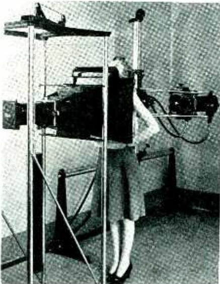
The newest type of rotating anode x-ray tube is used in this radiographic method of examining large areas of the body. An x-ray photograph of the girl's chest is made on a small film at the extreme right. The film need not be life size as was formerly the practice
