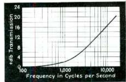
Fig. 3—The standard pre-emphasis characteristic incorporated in the generator is removable by means of a selector switch, whenever overall "flat" measurements are to be made
