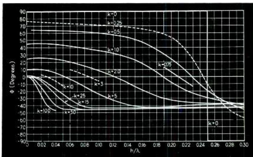
Fig. 10—Phase angle of the input impedance, for various values of the parameter  $k$  (compare with Fig. 9)
