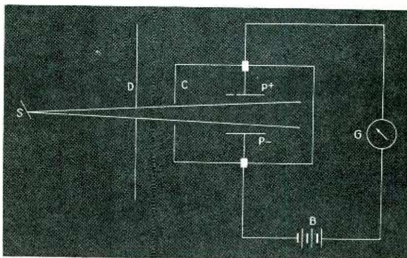
Fig. 5—Rough setup for measuring intensity of x-ray ionization. The x-rays flow through the opening in the lead sheet *D* into the chamber *C* where ions are formed. The ions migrate to the charged plates to cause a current flow which is measured by the galvanometer *G*
