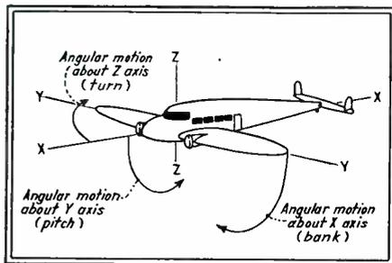
Fig. 1—An airplane has freedom of motion about three axes and is controllable by remote means in each of them
