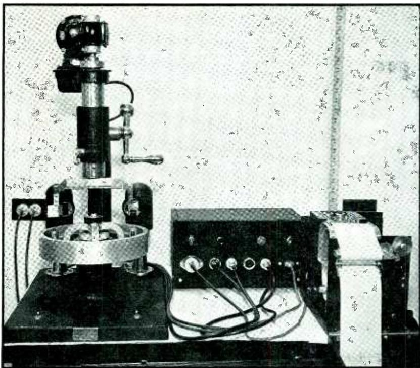
Fig. 8—Apparatus whose circuit is shown in Fig. 7. A light source and phototube are mounted so that light is reflected from a decagonal mirror on the flywheel shaft into the phototube
