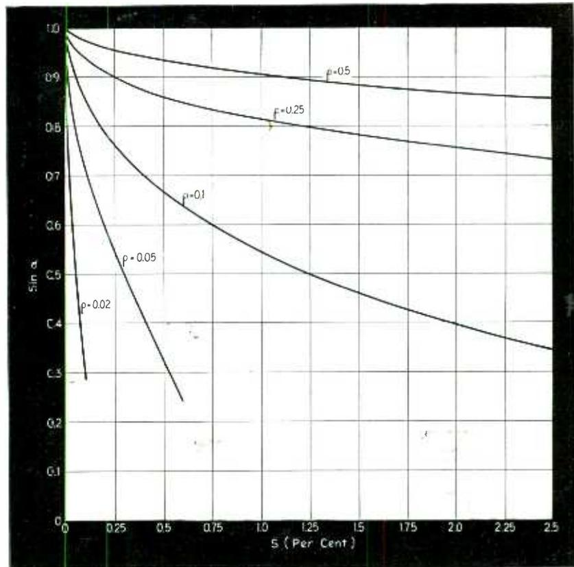
Fig. 3—Chart of the sine of the starting angle versus twice the fractional ripple voltage for low ripple voltages
