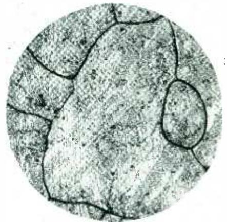
Fig. 3—Section B showing structure of alloy after thorough annealing
