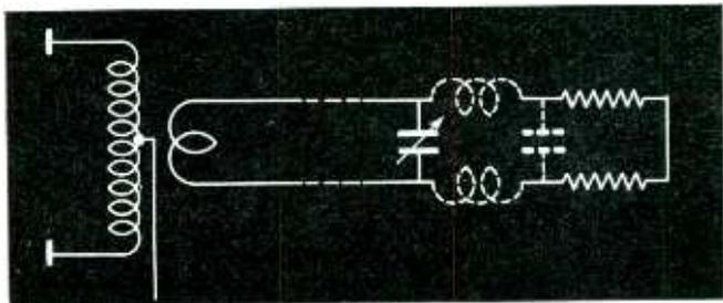
Fig. 3—Typical dummy antenna circuit, of the transmission-line type, used as a basis for the resistor design
