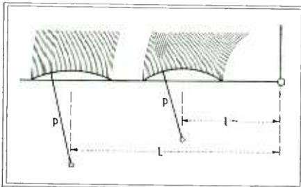
Fig. 2—The pickup arm of the inside sound track is shorter than the other
