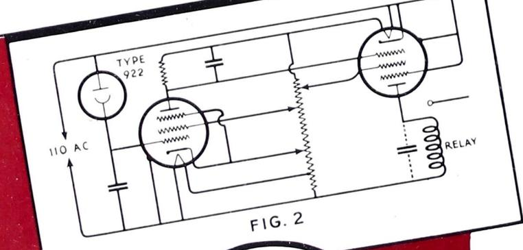
**RCA-2050**—Used to control up to 650 volts peak and will handle a peak current of 500 ma. and an average current of 100 ma.
