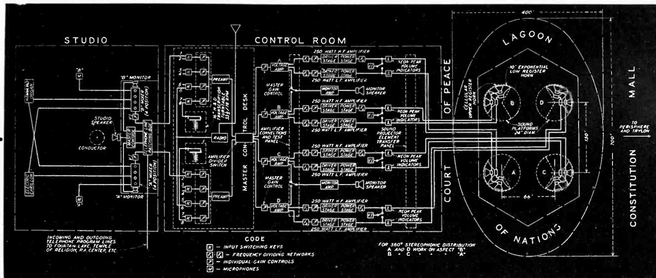
Block diagram of complete system. Stereophonic perspective is provided by two complete and separate sound systems, one for each aspect of the orchestra
