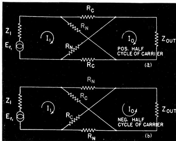
Fig. 12—Equivalent circuits for the ring modulator
