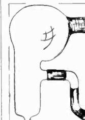
**EVACUATED DEVICES:** Shields, guard rings, "cat's whisker" contacts, conductive cements, and special electrodes or contacts are formed conveniently with "dag" dispersions.
