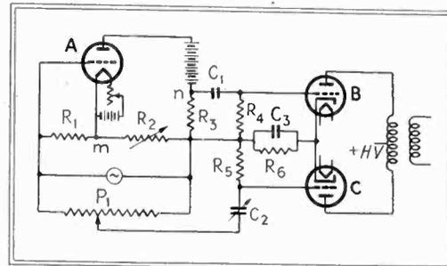
Fig. 2—Improved circuit, used to measure  $\mu$  of tube A
