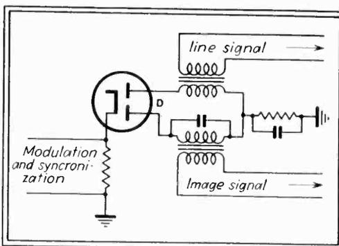
Fig 2—Double diode impulse detector circuit
