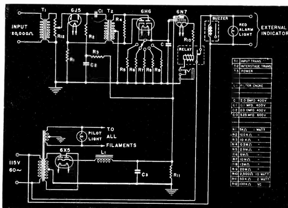
Circuit diagram of program failure alarm. Variation in the time delay before the alarm operates is provided by the adjustable diode load resistor and condenser
