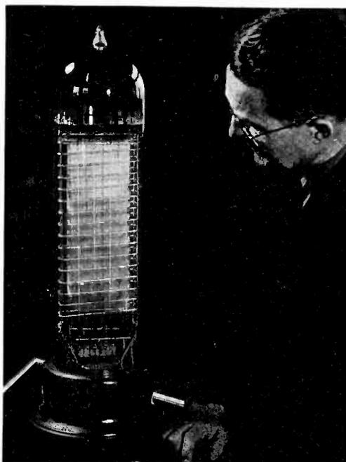
A three electrode vacuum tube of giant dimensions is specially constructed with filaments on the outside and plate on the inside. The plate is coated with fluorescent materials so that the operation of the tube can be determined visually
