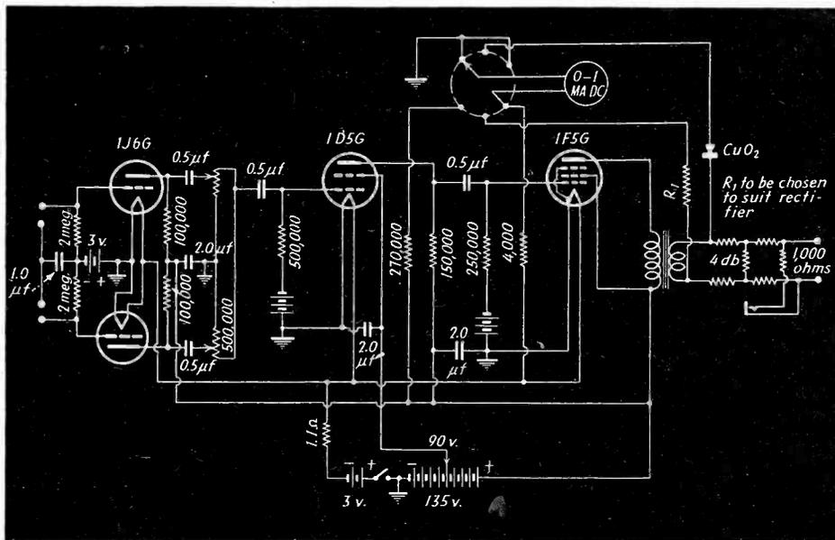
By the use of a 0-1 milliammeter with a CuO rectifier and a three-way position switch (top, above), it is possible to check the output level, the A voltage or the B voltage at any time
