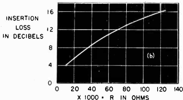
Fig. 14—A variable-loss network using double rectifiers (See reference 10)
