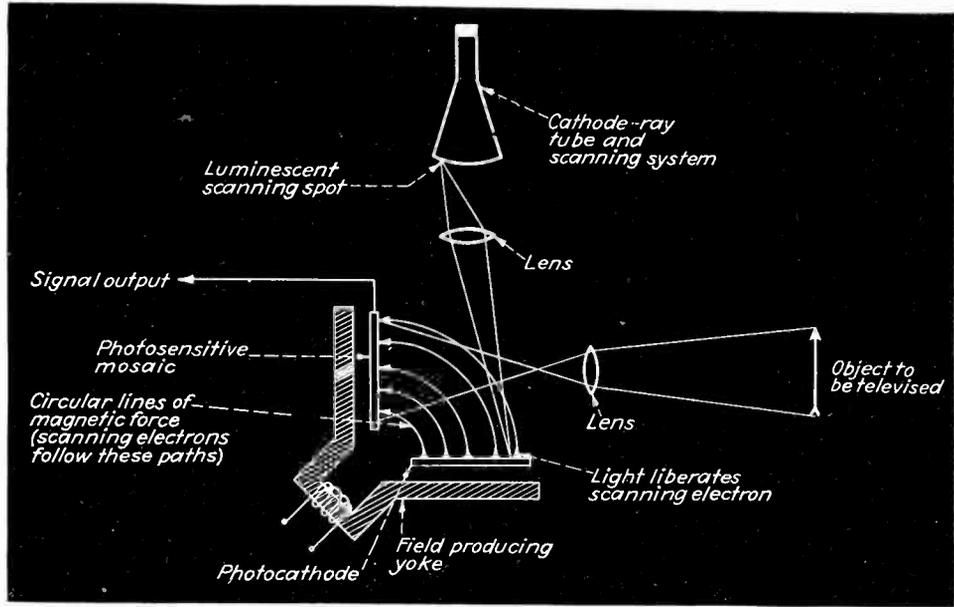
Fig. 5—An early system for obtaining perpendicular scanning employed a flying light spot focussed on a photocathode which liberated the scanning electrons
