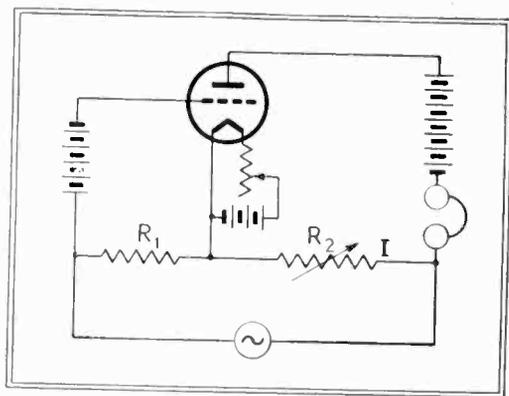
Fig. 1—The conventional measuring circuit
