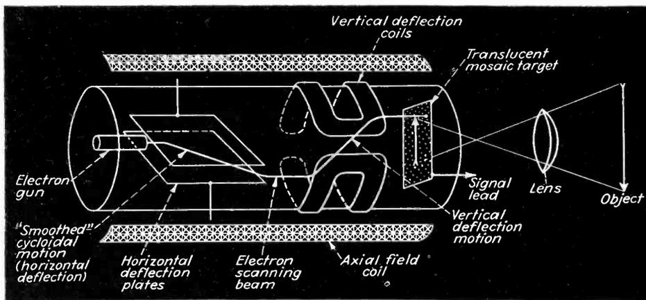
Fig. 10—The Orthicon in complete form. The deflection systems are shown in detail in Figs. 8 and 9. Note that the scanning beam hits the translucent mosaic at right angles
