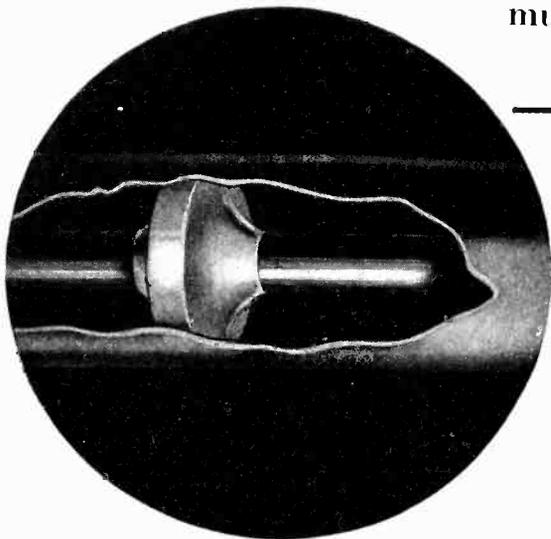
Fig. 1—Section of Isolantite coaxial cable. The shape of the insulator serves to distribute the lines of force uniformly over its surface
