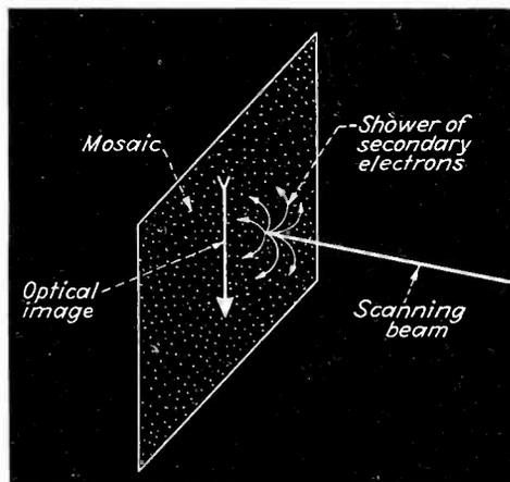
Fig. 2—When the high-velocity scanning beam hits the mosaic it generates a shower of secondary electrons which fall back on the mosaic, producing a spurious signal
