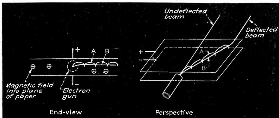
Fig. 9—Vertical deflection is obtained with a transverse magnetic field supplied by coils at right angles to tube axis
