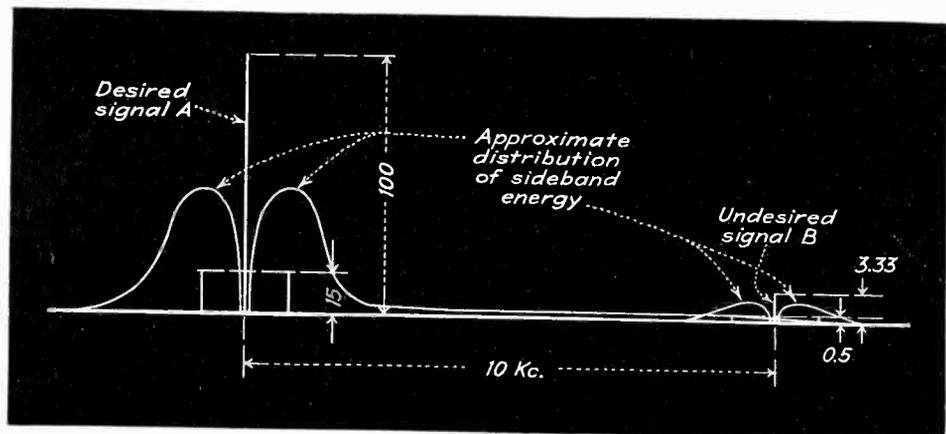
Representation of the relative strengths of the desired and undesired signals and their sidebands. The energy of the sidebands is concentrated in the region between 100 and 2000 cps
