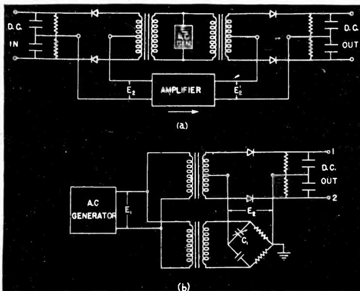
Fig. 9—Typical applications of CuO rectifiers to modulation in telephone service: (a) bridge circuit and (b) ring modulator
