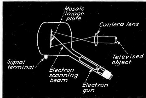
Fig. 1—Arrangement of the conventional iconoscope, now widely used as a pick-up camera tube
