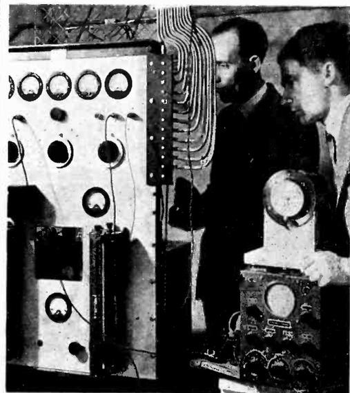
The Greenwich Observatory outside of London is making use of piezo-electric quartz plates in its new super clock which, it is expected, will keep time to within 1/1000th of a second
