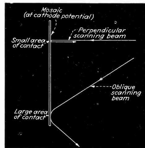
Fig. 3—When low-velocity electrons are used for scanning, defocusing occurs unless the scanning beam hits the mosaic perpendicularly
