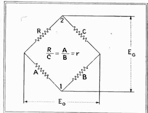
Fig. 1—Basic bridge circuit
