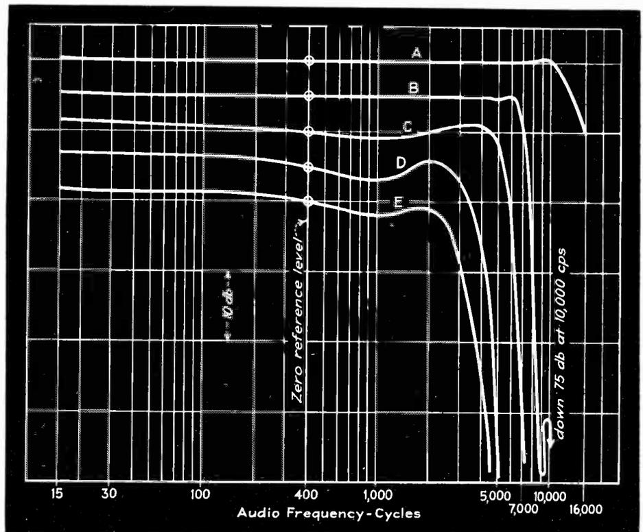
Audio response curves measured from antenna input to voice coil. Curve A is the wide-band response, curve B is the response with the variable i-f transformers and low-pass audio filter adjusted to eliminate a moderate amount of interference. Curves C, D and E are the curves for increasing amounts of interference
