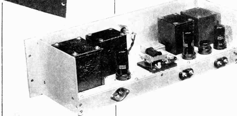
The unit is designed to operate on lines which carry a level of eight vu or higher. It is self-monitoring and a failure within itself will cause an alarm
