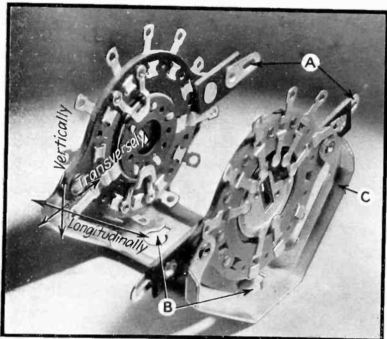
*Bracket and switch assembly. Rigidity in three dimensions as indicated. A. Lugs for supporting resistors and bypass condensers. B. Dowel hole with key slot for locking assembly and for alignment. C. Bracket of pressed steel*
