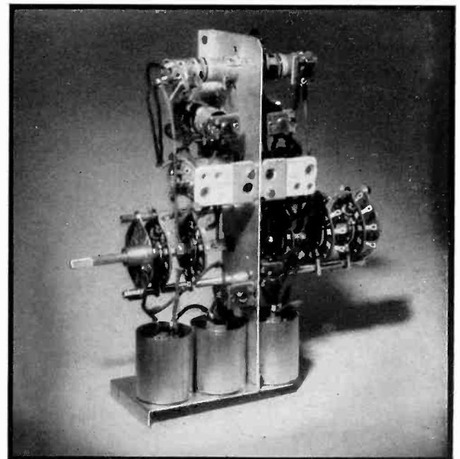
*Predecessor of the Centromatic unit. A complete coil and switch assembly as used in the Bosch radio receivers, model 480. This was followed by the unit described here*
