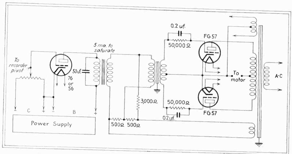
Circuit for turn-table speed control, using grid-controlled rectifiers
