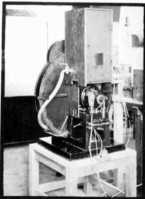
Television transmitter and receiver built by T. Sone of Tokyo. The disc method is used
