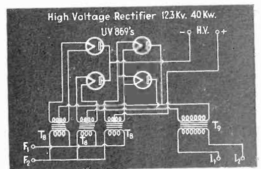
High voltage power supply for h-f generator
