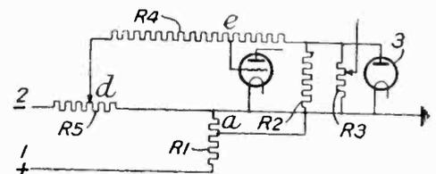
ent on the strength of the rectified current in the resistance *R3* and on the position of the slider *d* which is ganged to the tuning control of the amplifier. The anode of the diode never becomes negative whatever the position of the slider *d*. Philips. No. 424,735.
