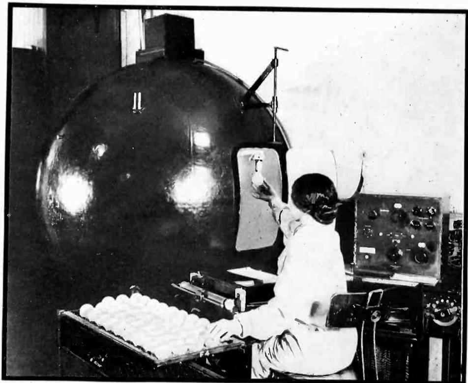
This integrating sphere directs the entire light output of a sample lamp, taken from the production line, into a phototube mounted on top, which in turn measures the light output in lumens
