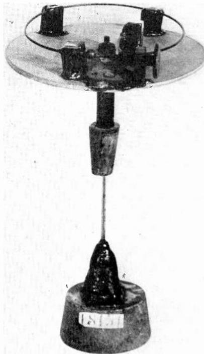
Photographs of two resonators used by Heinrich Hertz in his demonstration of the existence of electric waves
