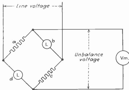
Fig. 1—Bridge circuit composed of resistances and lamps
