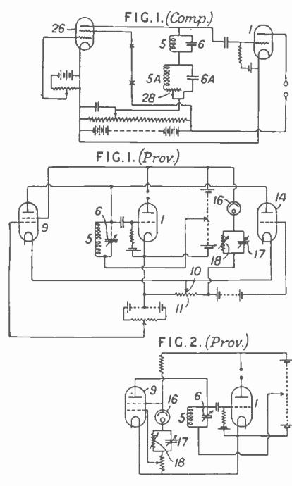
**Phase modulation.** Two components of the same carrier wave phase displaced by 90 deg. are radiated simultaneously from separate aerials after being modulated by signal currents in phase opposition. For reception it is necessary to supply a local oscillation of the same frequency, but de-phased from the incoming carrier so that the signals cause minimum interference with any normal type of receiver. G. W. Walton, London. No. 400,273.
