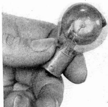
known as the FJ-114 is made in an automobile headlamp bulb and therefore is much smaller than the average tube. The active surface is caesium deposited on oxidized silver, enhanced by other special treatments which not only contribute to the high sensitivity (35 microamperes per lumen) but produces a high sensitivity in the infra-red.
