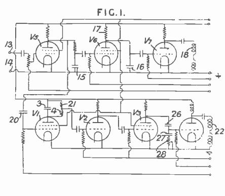
**Automatic tone control.** Combining manual tone compensation applied to the low-frequency stages of a receiver in combination with automatic volume control applied to the high-frequency stages, with the object of correcting the natural tendency of the ear to accentuate the middle frequencies as compared with the higher and lower notes, particularly at a low level of sound-output. L. E. Barton, Marconi Co. No. 397,763.
