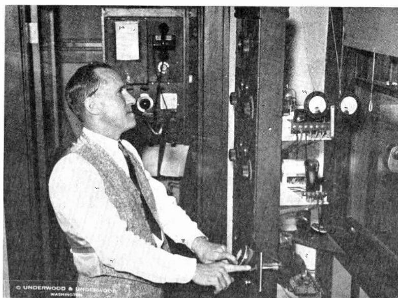
A new method of remotely controlling radio beacons by wavelengths of the order of 5 meters has been developed by engineers of the Department of Commerce. The apparatus here is under control of G. Muehl, who simply dials to stop or start the Washington beacon.
