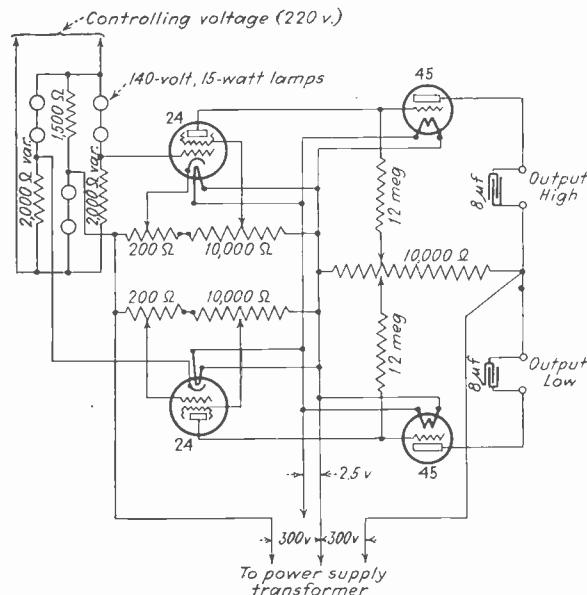
Fig. 6—Double-acting electronic voltage relay
