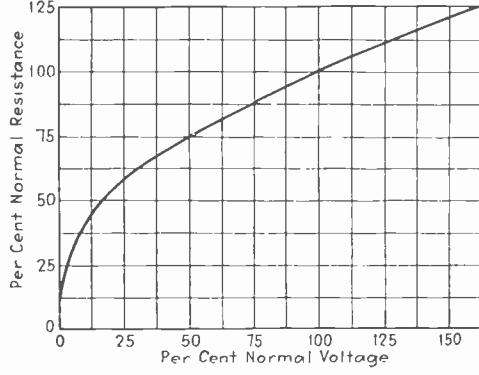
Fig. 2—Voltage-resistance curve—25 watt tungsten lamps
