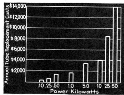
● One of the largest markets for vacuum tubes and rectifiers of power size is the broadcast station; and the chart shown here portrays the average expenditures of stations in various power brackets. Thus it is seen that the cost of tube replacement, which is by far the largest item in the maintenance budget, runs from a few hundred dollars annually for the small station to an expenditure of
