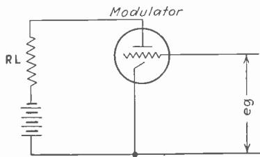
Fig. 2—Equivalent circuit of modulation circuit
