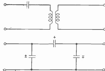
Fig. 6—Design steps for transforming at each end the impedance of the filter diagrammed in Fig. 2 by the artifice shown in Fig. 5
