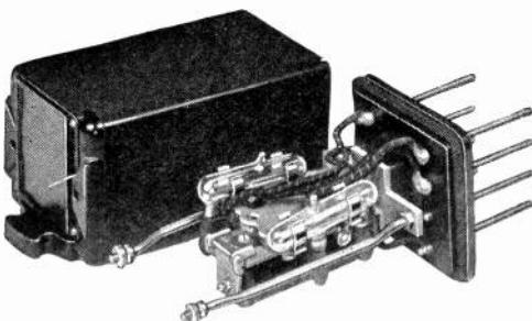
This mercury contact relay handles comparatively heavy currents with minimum relay current consumption. It is quick-acting, non-chattering, and can be equipped with one or two mercury contacts, easily adjustable for either make or break operation. Supplied either with angle bracket or on Bakelite base with cover, and for a variety of voltages and frequencies. (D.C. relay shown in illustration.)
