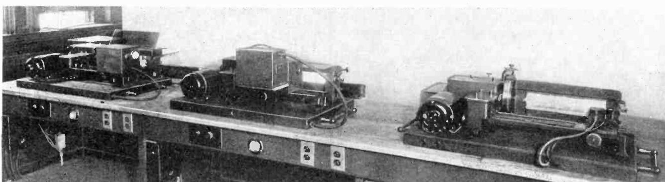
Facsimile apparatus at Radio Central of RCA-Communications, New York. At the left are two transmitters, with box-like housings for the photo-cell scanners. The right-hand machine is a spray-type ink-paper receiver, which operates in ordinary light using ordinary paper. The ink-paper and photographic receivers are operated in parallel, and are now in service from London, Berlin, Buenos Aires and San Francisco
