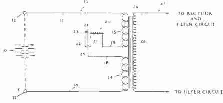
**Phase shifting device.** An electron tube method of continuously shifting the phase of an alternating current. W. A. Morrison, B. T. L., Inc. No. 1,942,483.
