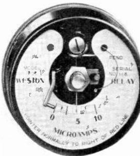
The relay will make contact on values down to three microamperes or one millivolt and its contacts are capable of handling five watts at 110 volts.
