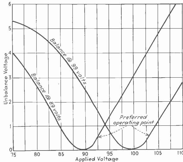
Fig. 5—Response of electronic voltage relay
