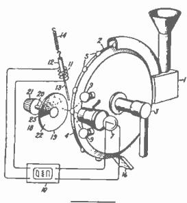
**Light control.** Photoelectric system for regulating the amount of illumination in a given area contributed by several light sources. F. W. Lyle, W. E. & M. Co. No. 1,944,751.
