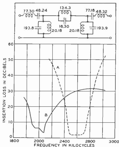
Fig. 4—(left) Modification of L and C of Fig. 2, so that the resonance frequencies are the same as before, changes the characteristics of the filter from A to B.
