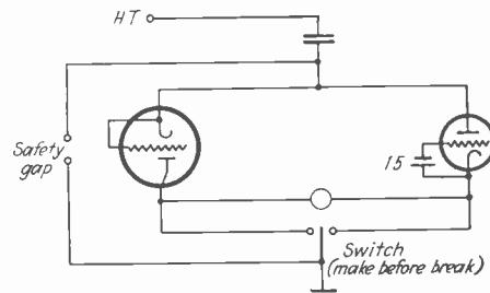
heated type. In one tube the grid is connected to the cathode while in the other a grid-bias of about minus 1.5 volt is used, although 1.1 volt would be sufficient to interrupt the flow of current. The over-biased voltmeter will read accurately from 2,000 to 500,000 volts with a condenser of 246  $\mu\text{f}$ . With 2,000 volts the galvanometer reads 70  $\mu\text{a}$ . (r.m.s.) and the voltage across the diodes about 15.—*Proc. Phys. Soc. London*, 49: 35-46, Jan., 1934.
