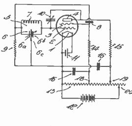
**Copper oxide rectifier.** Circuits for use in radio receivers. W. P. Place, assigned to Union Switch and Signal Co. No. 1,937,783 to 1,937,785, inclusive.
