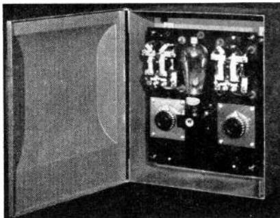
adjustable from 1/10 second to 45 seconds. It can be applied to any spot or projection welding machine now in service which is equipped with a magnetic main contactor. The electronic timer is unusually rugged, as the industrial grid glow tube is designed for sturdiness and long life and operates the contactor directly without delicate intermediate relays. The grid glow tube is free from any effects of wide temperature changes.
