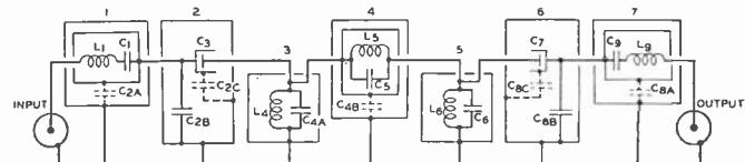
Fig. 8—Final filter circuit with desired characteristics
