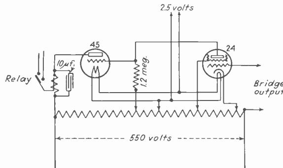
Fig. 4—Elementary diagram of voltage relay
