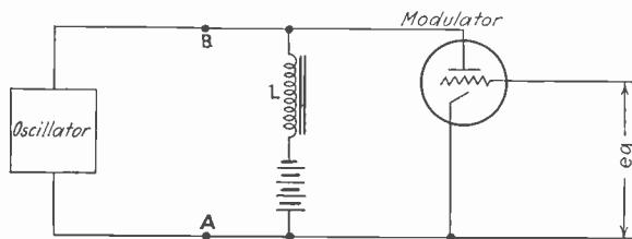
Fig. 1—Block diagram of constant current modulation system
