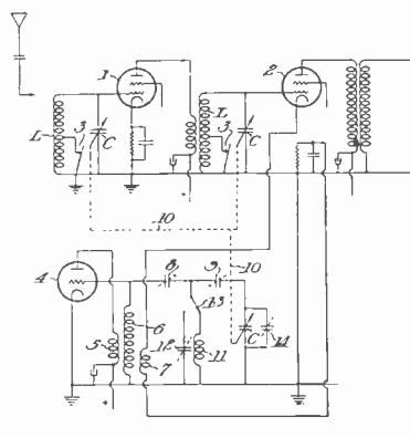
**Navigation system.** A radio system comprised of two co-planar coil antennas connected in series, an independent coil connected at right angles, electron tubes, etc. J. A. Willoughby, Washington, D. C. No. 1,942,526.
