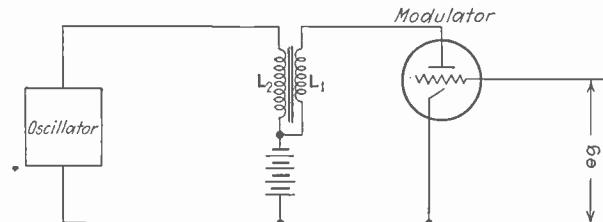
Fig. 3—Modified constant current system
