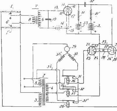
**Dual band system.** An amplifier system adapted for operation in more than one band of frequencies. C. J. Franks, assigned to R. F. L. No. 1,943,790.
