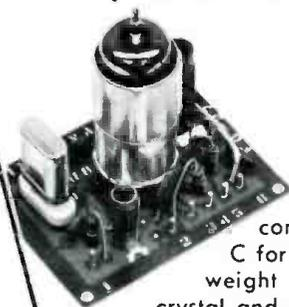
**D** Transmitter Unit (prewired and tuned) Oscillator and amplifier. Crystal controlled. Requires Unit C for modulation. Shipping weight 2 lbs. Complete with crystal and tube certified .005% tolerance. \$14.50.
