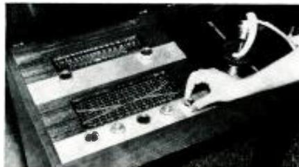
cabinet stereophonic consoles, shows visually, on a movable graph, the bass and treble decibel setting for each sound channel. By making a note of the desired ratings for each record, listeners can preset the controls when the record is replayed, without having to walk back and forth from their listening positions to make adjustments.
