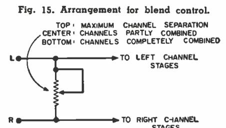
Fig. 15. Arrangement for blend control.
