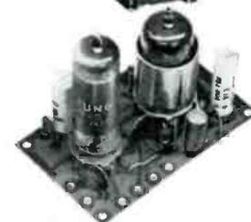
**C** Audio Unit (printed circuit prewired), speech amplifier for crystal or carbon microphone, first audio for receiver and power amplifier/modulator stage. Designed to follow unit B. Includes output transformer but not speaker. Shipping weight 2 lbs. \$13.50
