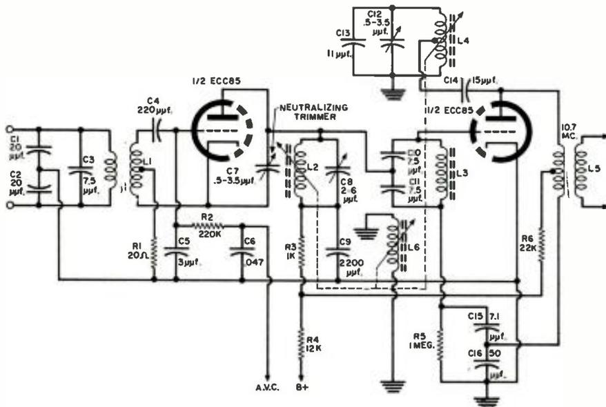
▲ Fig. 1. Specific circuit of the autodyne front end as used in the Telefunken "Jubilee" and other FM receivers.
