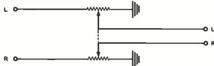
Fig. 5. A typical basic master gain control.
