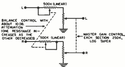
Fig. 7. Combined balance and master gain.
