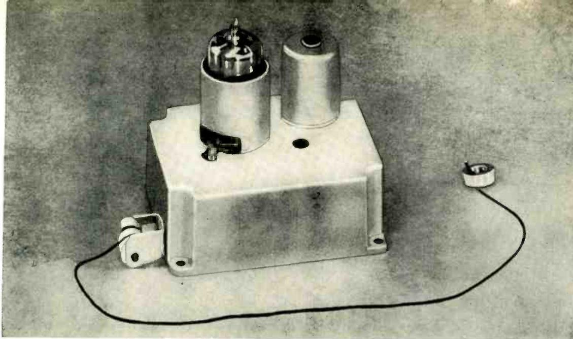
This subchassis, integrating an r.f. and converter circuit, is made by General Instrument Corp. and used by manufacturers of FM tuners and receivers. Other units using this general type of circuit are imported from West Germany.
