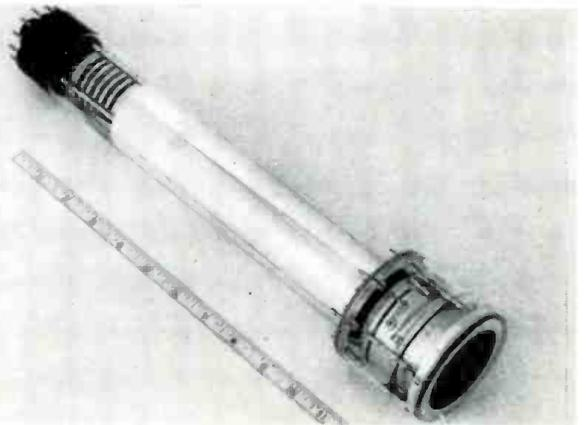
The new tube is identical to standard broadcast orthicons with respect to size, configuration, and socket connections, and can be used in existing equipment without changes. However, the tube is up to 100 times more sensitive when used in a special TV camera.
