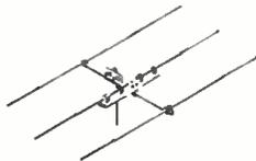
MODEL A-311, Three Element Beam for best point-to-point communication.
