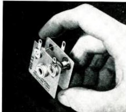
power circuits. This single TV-502 silicon stack will also replace two selenium rectifier stacks in all black-and-white TV sets that use twin selenium stacks in a doubler circuit.
