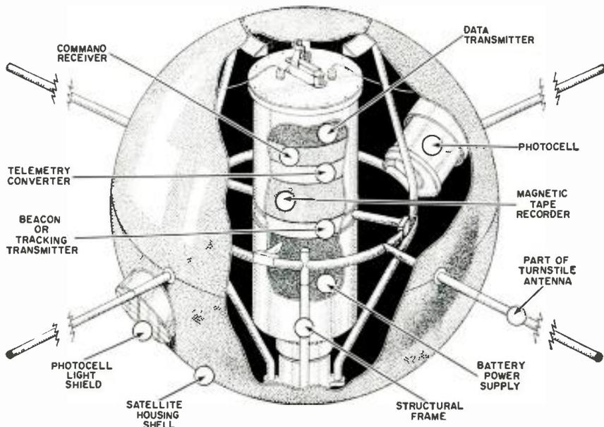
Fig. 2. Here is a photo of the package of electronics gear used in "Vanguard II."
