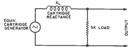
Fig. 2. Equivalent circuit of typical magnetic cartridge.
