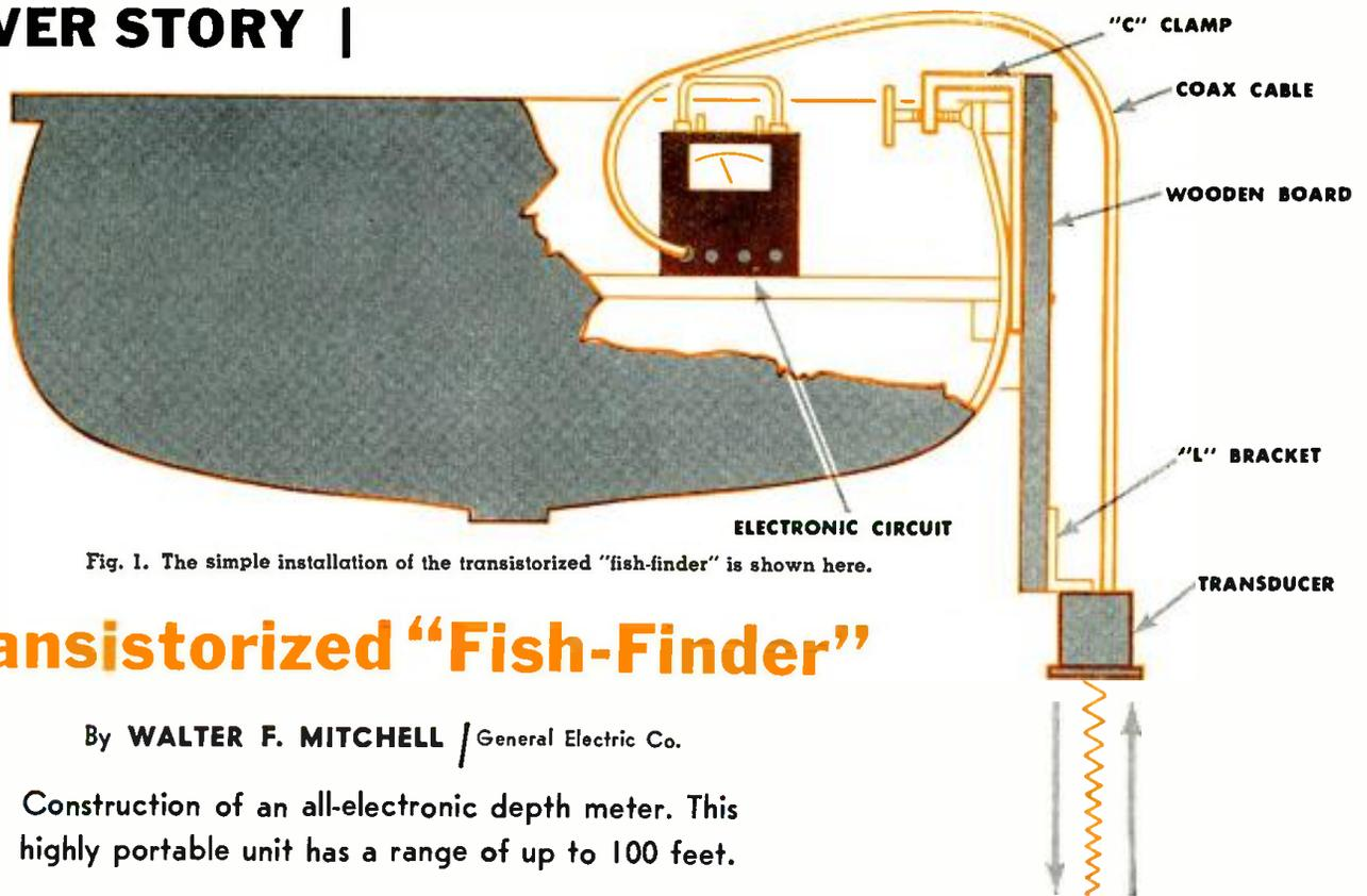
Fig. 1. The simple installation of the transistorized "fish-finder" is shown here.
