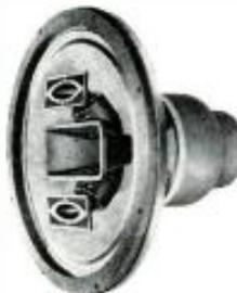
The "Tetraxioms" are 15" units featuring the "Rigidflex" cone, a completely flexible, free-floating cone rim, and completely rigid cone center to provide pure piston action. The speakers have high power capacity and smooth response from 20 to 20,000 cps with usable response to 35,000 cps. They are composed of four independent, concentrically placed radiators, each designed for maximum performance and efficiency within their portion of the spectrum.
