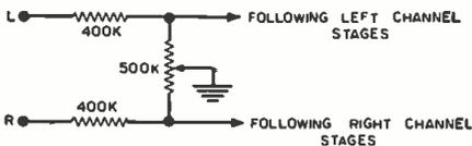
Fig. 2. Single control for balancing.
