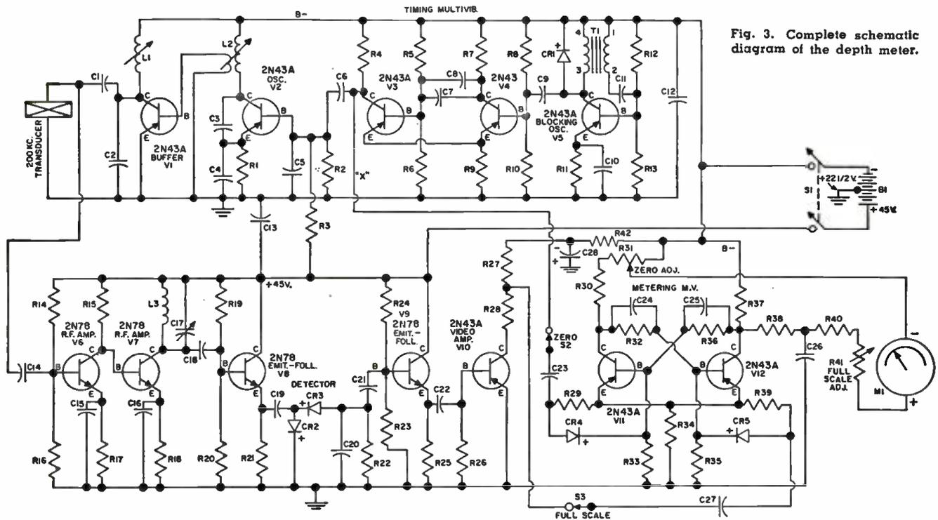
Fig. 3. Complete schematic diagram of the depth meter.
