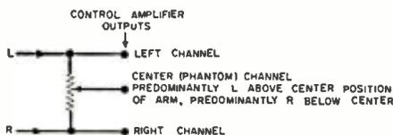
Fig. 17. Phantom channel with mixing.
