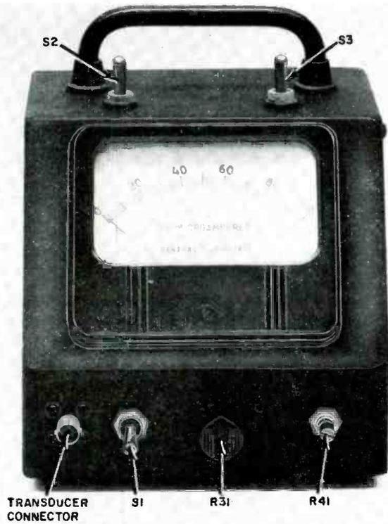
Front view of electronics unit of depth meter. Depths, in feet, are read directly on the microammeter's 0-100  $\mu$ a. dial scale.
