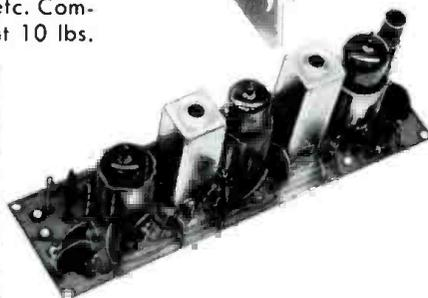
**B** IF Unit (printed circuit prewired) consists of mixer and tunable local oscillator feeding 262 KC IF stage. Includes noise-limiter and squelch circuits. Designed to work with units A and C. Makes dual conversion receiver. Shipping weight 2 lbs. \$16.00.
