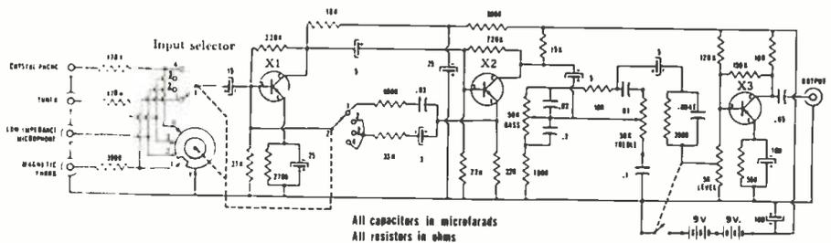
Fig. 1. Diagram of the Regency preamplifier. Apparently the company uses several different sources of supply for the transistors since they were not identifiable.
