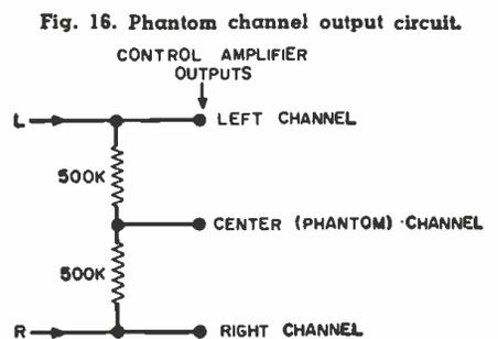
Fig. 16. Phantom channel output circuit.
