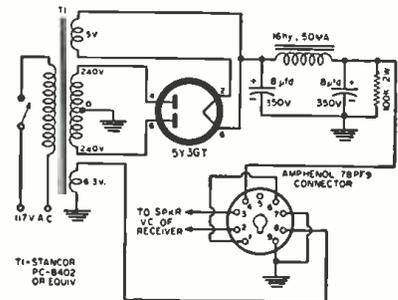
Fig. 5. Small power supply suitable for use with transmitter at fixed location.
