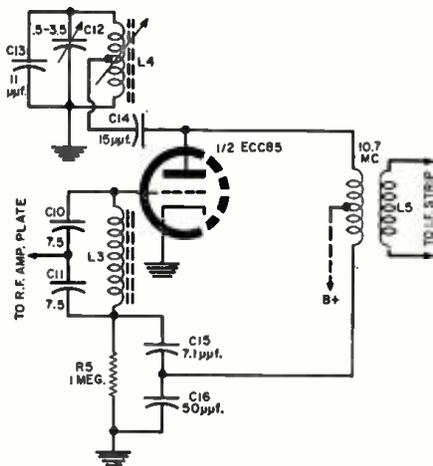
say that this was worked out first and that C<sub>11</sub> was added to provide bucking action, as some r.f. signal applied to the grid might otherwise sneak away down coil L<sub>2</sub>.
