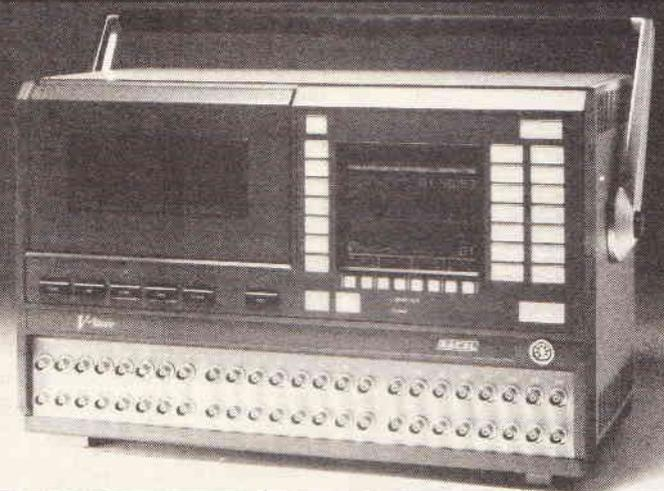
Racal Recorders in Southampton has produced a highly advanced instrumentation recorder that uses standard VHS video cassettes for data storage.
