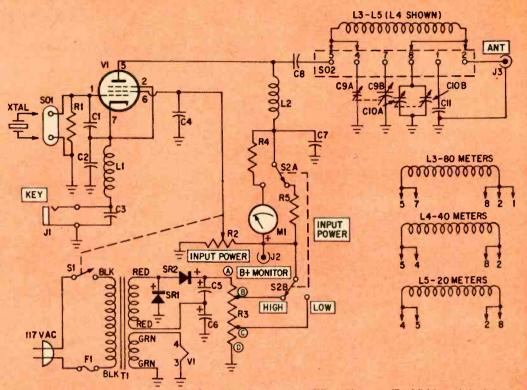
Fig. 2—Transmitter schematic. S2 determines input power. When it's set to "high" (shown), high B+ is supplied to V1 from tap "B" on R3. When S2 is set to "low." lower B+ is supplied to V1 from tap "C." R2, which establishes VI's screen voltage, is used to vary the input power continuously in both ranges. 80-meter coil, L3, is 33 turns. 40-meter coil, L4, is 171/2 turns. 20-meter coil, L5, is 81/2 turns. (See Fig. 4.)
