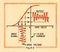
produces no change in the quantity, no matter what opposing values are added. And therein lies the explanation as to why average plate current of an RF or IF amplifier in a receiver remains the same whether no signal, an unmodulated carrier or a modulated signal is applied to its grid.
