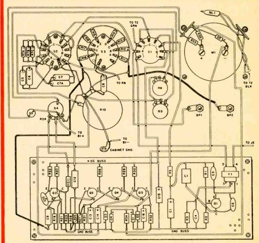
Fig. 2—Circuit board and front-panel wiring. Perforated board is  $8\frac{1}{2} \times 3\frac{1}{2}$  in. To prevent oscillator output from getting to amplifier, put oscillator at right of board and amplifier input at extreme left. Note that shield on wires from BP2 to R11 and from C9 to R18 is grounded at R11 and R18 ends only.
