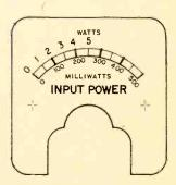
Fig. 6—Meter is calibrated in milliamperes, but if you paste this scale over its scale, you'll be able to read the rig's input power directly.
