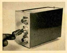
Output side of Center. Scrape away the paint on Minibox under connectors to make sure there is good contact between connectors and the cabinet.
