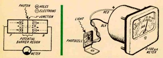
Fig. 3—In diagram of photovoltaic cell at left, holesand electrons are caused by light to cross potential barrier region and combine. Minority carriers which are created pass through the junction and are actually the current developed by the cell. Diagram at the right is of photovoltaic-cell light-level meter.
