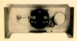
Fig. 6—FSM remote is built in a 21/4 x 21/4 x 5-in. Minibox. Parts placement is not critical. Connect it to Tester with RG174/U coax cable.
