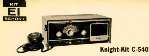
THE Knight-Kit C-540 transceiver is a compromise design. That is, it combines the ease-of-operation and price advantages of a single-channel transceiver with the multichannel flexibility of more expensive rigs. Although it has a single-channel transmitter, the crystal socket is mounted on the front panel. This permits you to change the transmitting frequency conveniently by plugging in another crystal.
