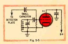
the carrier reaches the detector. To do this we mix the received signal with one generated by a local oscillator called a beat-frequency oscillator (BFO). If the BFO is tuned only a few hundred cycles away from the carrier frequency, it modulates the carrier with a difference frequency falling in the audio range.
