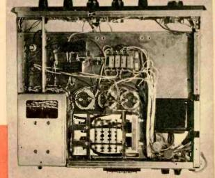
Underside of LK-60 is exceptionally clean. Preamps are enclosed in shielded compartment in lower left corner. Input selector switch also is located in compartment and is coupled to the unit's front-panel knob with the extra-long shaft.
