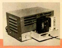
Model GW-12D transceiver includes vibrator power supply for 6 or 12 VDC operation. Supply is bolted to rear of chassis but can be removed.
