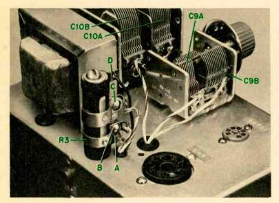
Fig. 3-Closeup of top of chassis shows mounting of B+ voltage-divider power resistor R3. Mount R3 with a 1/4-20 x 2½-in. screw. Slider contact "C" is home brew since only one slider is supplied. Make a cover of perforated aluminum to fit over R3 so you don't touch it. If you did you'd get a nasty shock and burn. Both sections of C10 (top) are connected in parallel. C9A is the smaller section of C9.
