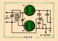
between the IF and the BFO frequency. This modulation will be detected in the normal manner and will produce a a 1500-cycle tone in the detector output. If desired, the frequency of the BFO can be altered slightly to adjust the pitch of the dots and dashes to suit individual taste.
