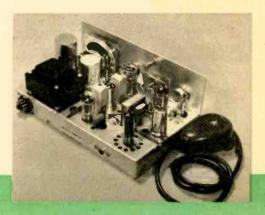
Vibrator on Universal model C-540 is between transformer and speaker. Circuit includes six tubes and has solid-state doubler power supply.
