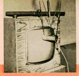
Among most dramatic tests conducted at UL's Melville, N.Y., facility is that for implosion of a TV picture tube. Technician (at left) was forced
