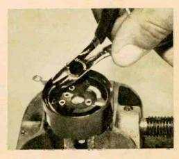
To add off position to R2, cut wire where it connects to left lug. Then remove a few turns so wiper doesn't touch wire when turned all way to left.
