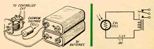
Fig. 5—Schematic of photoconductive-cell control device. Sixteen volts is required to provide current to cause relay contacts to close. Clairex cell we specify (not shown above) can handle up to 300 V and can, therefore, be used with AC relay in line-operated circuits. Cell handles up to 75 milliwatts.
