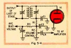
during positive half-cycles move down through the IF transformer and R1 and R2 to return to the cathode through the common-ground circuit. And in doing so, they create a pulsing, DC diode current through the resistors with accompanying voltage drops.
