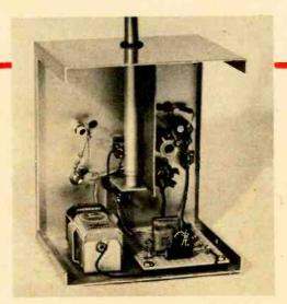
Fig. 2—Antenna hole is 1% in. back from front of cabinet. Put grommets between board and bottom of cabinet. Put tape on cabinet under board.
