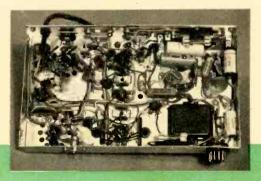
Though it looks crowded, there's room to spare in the underside of the C-540. 117-VAC or 12-VDC power cord fits on connector at lower right.
