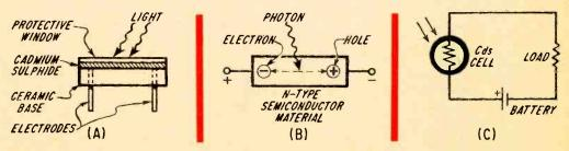
Fig. 1—Diagram A shows photoconductive cell construction. In B, activity of free electrons is increased by light which causes them to be attracted by positive external voltage. Holes left behind are attracted by negative side. This results In a current flow whose magnitude is determined by light intensity.
