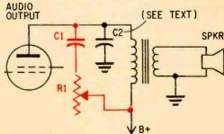
Fig. 2—Simple tone control consisting of Cl and Rl improves audio quality, helps in DX work.
