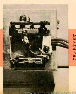
Adjustable wirewound resistor and fuse holder should be mounted on back of chassis. Because resistor will be difficult to get to after unit is mounted, measure the dropped voltage with recorder operating before installing chassis under the dash. Fuse should be a .15 A type 3AG.
