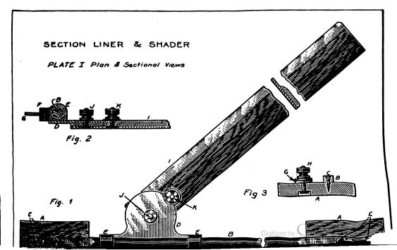
any sort of wood, hardwood preferably. The rod B carrying the runner can be made of brass, iron or steel. As can be seen, it is flattened at both ends, so that it can be more easily fastened to the bases A with screws C.
