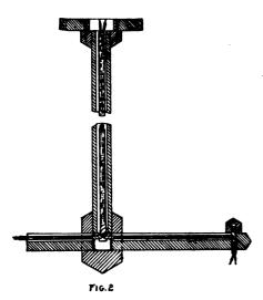
cally, No. 18 wire may be used in the branches, one side of each branch all being joined to No. 14 wire which extends up through the vertical part. If the mechanic is not familiar with this method, it would, perhaps, be better to let the small wires extend up the entire length, making one side of the circuit so that the number of wires may be properly divided and secured at the terminal of the rosette.
