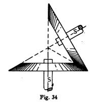
angle. In this arrangement the wheel P must be smaller than the other, as it is a pinion working inside an annular wheel.
