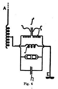
in the condenser circuit, the two circuits were brought into electrical resonance, a condition which I first pointed out as being essential in order to obtain efficient radiation and good tuning.
