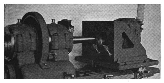
an average of nine thousandths of an inch to be removed by grinding. Heald Cylinder Grinding Machines are largely used which employ the high speed abrasive wheels and put the finishing touch to the "heart" of the motor car, as it can truthfully be called.
