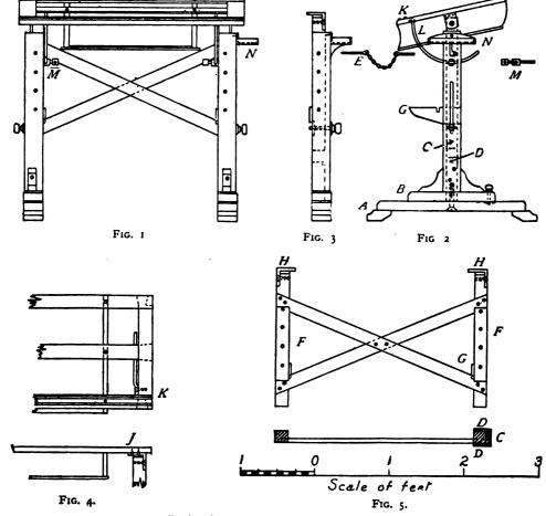
Design for a Portable Drawing Frame
