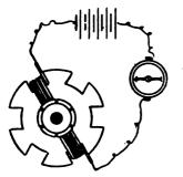
Fig. 1. Testing Armature Winding
