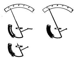
with melted lead or rosin, and, when hard, bend it so that it will lay along the arc of the larger circle. The center of the tube when laid on the drawing should about line up with the inner circle. Melt the lead or rosin out of the tube, fit heads of wood or hard rubber 1 in. in diameter, cover the tube with several layers of paper and wind full of No. 22 magnet wire, bringing the two ends out for terminals.
