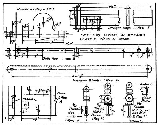
seen from the drawing that the wood Iunder D has been filed to admit the latter. Thus the washer under K lies flat. If desired, the straight-edge I need not be filed, but then a small piece of wood or metal must be placed under part of the washer, to make it lie flat; otherwise it will not satisfactorily clamp I to D.
