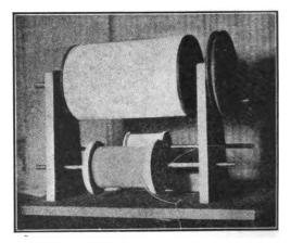
Fig. 2. Showing Method of Winding the Secondary
