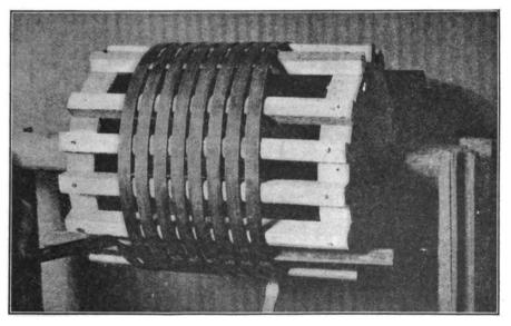
Fig. 1. Showing Method of Building Up the Primary
