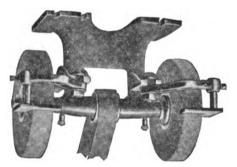
With the 308 the driving pulley is at one side and the sharpening wheel at the other. The belt can come from above, from the side or from directly beneath. All bearings are extremely long, wide and heavy. The manufacturers are willing to guarantee all the parts of the machine for many years.
