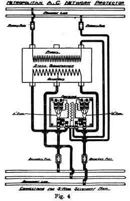
The terminal of the secondary of the commercial transformer are connected each through its own coil C and  $C_1$ , on the current transformer. These latter coils connected to the middle point of the looped fuses D and  $D_1$ . One side of the fuses is connected from E and  $E_1$ , to the outer conductors of the three-wire network. The fuses D and  $D_1$  act as a short-circuit connection on coils F and  $F_1$ .
