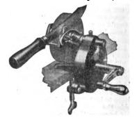
viates any danger of the knife's being jammed between the guide and the wheel, as the wheel continually lifts the knife. Sharpening it on the side face of the wheel gives a finer, smoother edge than could be otherwise attained. It leaves it also with no graining, especially if the knife is moved forward and back while being sharpened.
