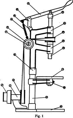
can be purchased at almost any price -\$3.00 to \$5.00. Get one capacity of  $0-\frac{1}{4}$  in. While this range,  $0-\frac{1}{4}$  in., is not the drill's maximum, it is well not to go beyond it, as the speed that the press requires for the smaller drills would prove disastrous for larger ones.
