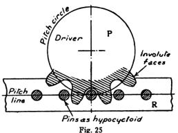
The faces of the pinion teeth, however, should not be an epicycloid curve, because they should be produced by the generating circle which has produced the so-called radial flanks of the rack. But this circle is one of infinite radius—in fact, it is a straight line. Therefore, the faces of the pinion teeth should be curves produced by rolling a straight line upon the circumference of the pitch circle; the curve should thus be an involute of the pitch circle of the pinion, Fig. 23.
