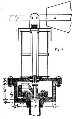
General Arrangement of Electric Wind Vane
