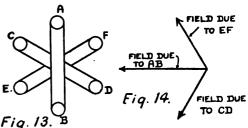
1,500 revolutions per minute. We could by increasing the number of poles still further reduce the field speed; therefore, the rotor speed. For instance, a six-pole field would give 1,000 revolutions per minute, and an eight-pole field 750 revolutions per minute, and so on; this is, of course, reckoning on a supply of 50 periods per second.
