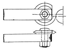
Fig. 15-Circular Threading Tool
