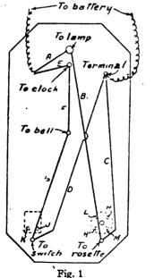
Fig. 1 Fig. 2 Front and Back Views, Showing Connections
