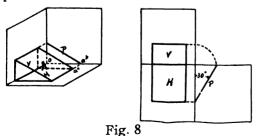
angle of 30 degrees, and which is perpendicular to PP. It will be seen that the plane cuts HP and VP in straight lines, and these straight lines are called the horizontal and vertical traces of the
