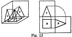
its true size and shape, but as all of its faces are inclined to VP and PP, these faces will not appear in their true size and shape in either the VP projection or the PP projection.
