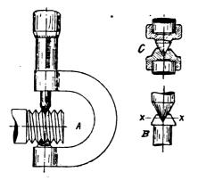
Fig. 13-Measuring Angular Diameter of Screw
