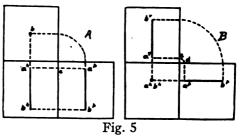
will project upon VP as a point and the distance  $ca^p$  will be the actual height of the line above HP, while the distance  $ca^h$  will be the actual distance which the line is in front of PP.
