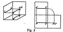
Since both VP and PP are perpendicular to HP, it is evident that  $cA^{P}$  must equal  $bA^{*}$ .
