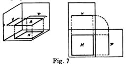
Fig. 7 shows the projections of the plane A which is parallel to HP and perpendicular to the other two reference planes. As in the case of Fig. 6, the plane projects in its true size and shape upon the plane to which it is parallel, while its profile and vertical projections are but straight lines. For the sake of simplicity all lettering which can, has been omitted, and the projections of the plane A are designated simply by means of the letters V, H and P.
