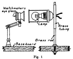
cut in the end to fix it to the lamp-holder, which is one such as is used for ordinary electric lamps. To the connecting-posts inside the holder, connect two pieces of copper wire, which are then connected to a 4-volt 4 c.p. Osmi lamp, Fig. 1. A small hole about  $\frac{3}{8}$  in. in diameter is now cut in the lid of the tin to allow the light to shine on the mirror. Between the lamp and the coil a watch-maker's eyeglass is fixed, Fig. 1, which can be
