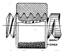
Fig. 11—Showing Clearance at Bottom of Spaces in Ring Gauges to clear Flat Tops of Work Threads
