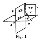
to each other and intersect in a line called the ground line. While these two planes will in some cases be sufficient to properly and clearly represent the object, yet there are many times when a third plane, called a profile plane, is needed. This third plane is taken perpendicular to the other two planes.
