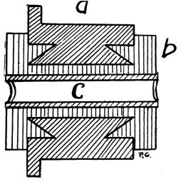
An invention that will in all probability revolutionize the manufacture of small commutators and cause the passing of the present taper ring method of conplacing the bars (with mica between) in a circle and putting a circular clamp around them is followed in this invention. and if necessary this combination is put into a lathe and the tapered recesses "trued up."
