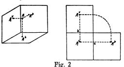
When a third view of the object is needed it is shown on the profile plane PP, and this view of the object is called a side view or side elevation. It is important to notice that the different views of the object derive their names simply from the plane on which they are shown and not from the face of the object represented.
