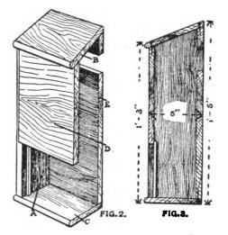
and back of the box, after which the sides, top and bottom may be finally fixed together. The overhanging front and end edges of the top and bottom should be rounded, as shown in the illustrations, and the joints when finally fixed together should be secured with glue.
