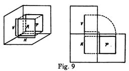
show the true size and shape of the plane A, although the projection upon PP shows the true length of the plane, and the horizontal and vertical traces show the true width of the plane.
