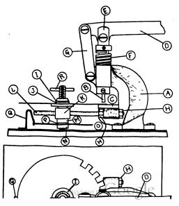
oil and then into water to harden it after it has been wound, or the spring may be cut from any old spring which may be available.
