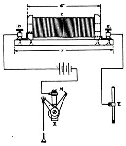
when three dry cells of the high amperage or ignition type are connected in series with it.
