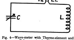
Galvanometer in Circuit
