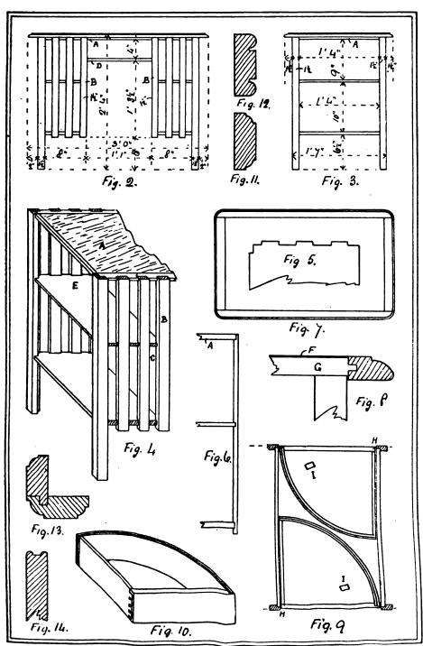
Novel Writing-Table and Book-Case julitzed by GOOG C Fig. 2.—Front elevation of table. Fig. 3.—End elevation of table. Fig. 4.—Isometrical sketch of half framing. Fig. 5.—End of shelf cut to take bars and legs. Fig. 6.—Vertical section chowing
