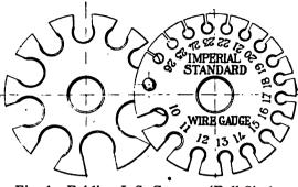
Fig. 1—Folding I. S. Gauge—(Full Size)
