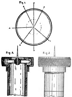
block till needle enters hole A, then the tailstock-spindle is parallel to bed.
