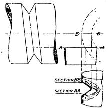
Fig. 9—Showing Effect of Setting Cutting Edge Below Center
