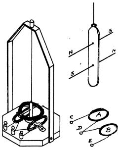
An Astatic Galvanometer
