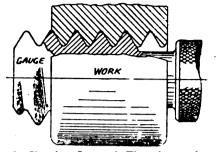
Fig. 3—Showing Internal Thread cut deeper than Standard
