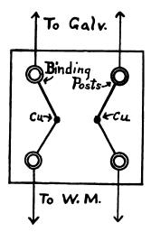
Fig. 2-Connections of Thermo-element
