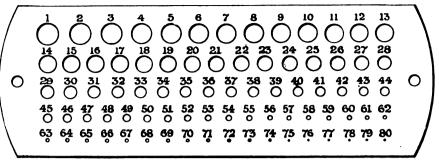
Fig. 2-Stubb's Gauge Plate-(Full Size)
