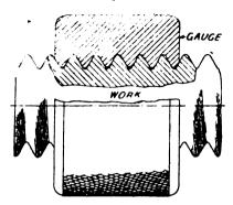
Fig. 2—Showing Example 1 Thread cut deeper than Standard
