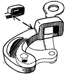
In the illustration the dotted lines show the solid steel forgings, and the makers broach a hole and pass the slip-neck through the forging, thereby making it practically an impossibility to break it. During the life of the patent on the oldstyle tool, it was never made in this way, and the Smith & Hemenway Co. announce that they have met with wonderful success with this new
