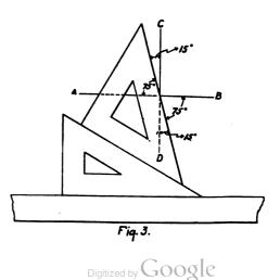
tal make (90-X) degrees with the vertical, the edge of the triangle makes an angle of (90-75) degrees or 15 degrees with the vertical. In Fig. 4, the edges of the 45 degree triangle make angles of 15 degrees with the horizontal and 75 degrees with the vertical.
