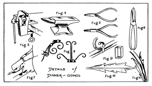
parts merely holding the article together, and making a complete and serviceable article. The making is so straightforward and simple that the veriest amateur may fetch out his tool-box without the least fear, for success in the act of forming curves in thin strip-iron comes easily after a little practice.
