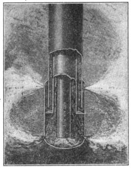
Section through Bottom of Pipe
