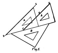
dicular to AB at point K. First place one of the short edges of triangle E along the line AB and place one of the long edges of triangle F along the long edge of triangle E. Now hold F firmly in place and slide E to position E'. When in this position, the other short edge of E is perpendicular to AB at point Kand the line CD may now be drawn.
