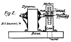
to within  $\frac{1}{4}$  in. of the bearing. This is done so that the wheel may be clamped between two nuts. See Fig. 2. The wheel should be painted with red lead so as to prevent rusting.
