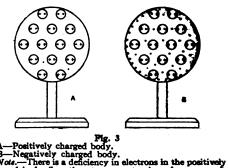
Note.—There is a deficiency in electrons in the positive charged body (less than two per atom), and an excess the negatively charged body (more than two per atom).
