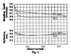
than circular. (The difference between the maximum and minimum diameter, however, rarely exceeded 10 percent). In reducing the results of the cross-bending tests to a common basis, the diameter of the filament was therefore taken as the mean of two diameters at right angles in order to reduce the error due to possible deviation from a circular section.
