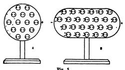
Fig. 5 A—Positively charged body. B—Neutral insulator brought near the charged body. Note.—In this case the electrons are held to the atoms by restraining bonds. If the body be cut in two and the charged body A be then removed, no trace of charge can be found on either half (showing that electrons did not leave their places to pile upon the end).
