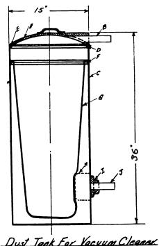
The dust tank is made from heavy sheet iron, with the seams either welded or soldered together. All the joints around the seams and rivets should be filled with iron cement or putty. Give the tank two coats of black shellac, soaking it in well around the joints.
