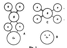
Fig. 7 A-Neutral molecule of copper sulphate (CuSO<sub>4</sub>). B-Copper ion (Cu + +). C-Sulphuric ion (SO<sub>4</sub> - -). Note.—The approximate size of the different atoms and of the electrons is correct. The actual arrangement of the atoms and electrons in the molecule is probably far different from that in the drawing from that in the drawing.
