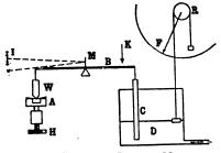
FIG. 1 - FILAMENT TESTING MACHINF.
