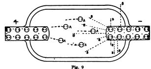
Fig. 9 Electric current flowing through vacuum tube (with metal electrodes.). A—Copper atoms (acting as ions) crossing vacuum to deposit themselves on legative electrode. B—Electrons, shot off at right angles to surface of electrode.
