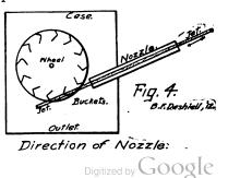
nozzle is connected to a faucet by means of a hose. All connections should be very tight, as there is a high pressure in the hose and nozzle. The water motor ought to be provided with a front cover so that the interior may be readily inspected. The whole should have a coat of red lead on the outside and inside.
