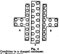
A-Positive plate. B-Negative plate. C-Dielectric. Note.-There is excess of electrons at negative plate, and deficiency at positive; also, dielectric is under electrical strain.
