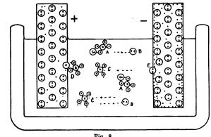
Fig. 8 Electric current flowing through CuSO<sub>4</sub> solution. A-Undissociated molecules of CuSO<sub>4</sub>.
