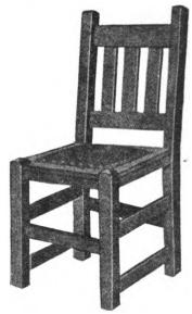
are fitted neatly to the proper size and doweled firmly together. After the cane is put in the opening it is covered over and upholstered with leather.
