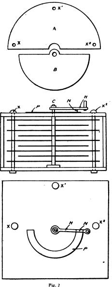
Showing Construction of Condenser
