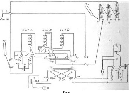
Fig. 4 Diagram of Connections
