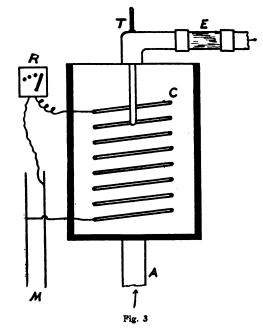
condition of the exit steam. For instance, if the steam is wet the glass will become moist, while if the steam is dry, no moisture will be present to fog the glass. Now, knowing the heat added to make the steam dry saturated and the amount of steam flowing through, you can compute the quality of the steam.
