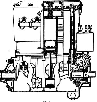
'Fig. 1 Reynolds' Rotary Plate Valve Motor
