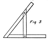
enough to go through the base and bolt up dead square, missing the center, which will be required to carry a socket capable of being revolved to adjust to the correct orientation last. If a casting, when filed up true and square to the angle, the same drilling, tapping and studding, will be required.
