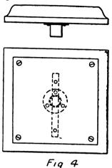
wood by flush countersunk screws of brass, and the holes drilled on a center line to take the studs right through the wood (Fig. 4). The gnomon being temporarily bolted in place, and its base filed till it stands square on each side, the whole affair must be leaned against a well, with the point of the gnomon resting on the table in such manner that the top face of gnomon, tried with a square, is perfectly vertical to the face of the table (Fig. 5).
