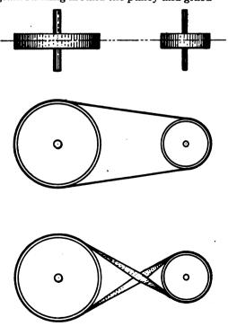
Fig. 9. Open and Crossed Belt Arrangement
