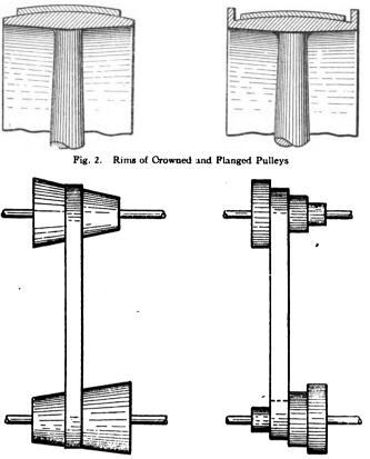
Fig. 3. Cone and Step Pulleys
