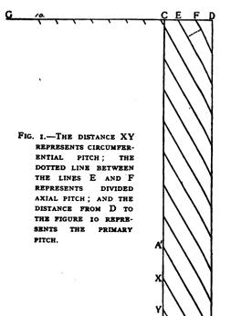
from D, step off ten points along the line DCG, the tenth point will show where the thread which started at D re-appears on the same axis of advance. In other words, it is the pitch of the screw, a small section of which we wish to cut. This measure was so nearly  $4\frac{1}{2}$  in. that again I felt justified in assuming that the skew gear had been cut to a "primary pitch" of  $4\frac{1}{2}$  in.
