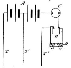
The wires TT'' lead to the gas jet. A buzzer B is placed in series with the coil as indicated., This buzzer alone, however, is not sufficient to produce the result desired, for it will be found that on attempting to light the gas, that the buzzer only will ring and the spark for lighting will be at the buzzer rather than at the jet.
