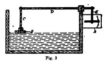
gauge registering at all times an amount corresponding to the depth. The reading is taken directly from the scale, as the gauge is calibrated in feet (or gallons) instead of volts. A few dry cells are sufficient to operate same, as they are only used the short time during which the reading is being taken.
