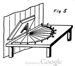
into quarters (Fig. 5). Adjust this on the table in a shady time of day or place, putting a piece of candle, lit, on the center line of the paper at its curved edge, shifting the paper round till the shadow of top part of gnomon falls exactly centrally on the dial. This is the 12 o'clock line, and will be  $\frac{1}{2}$  in. wide, and a slight
