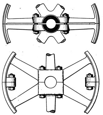
Fig. 1. Two Forms of Split Pulleys
