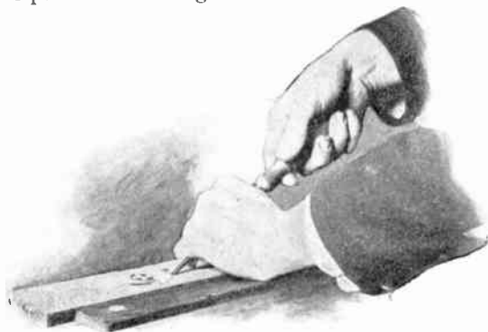
Fig. 10 Manner of holding the flat gouge for "grounding-out"
