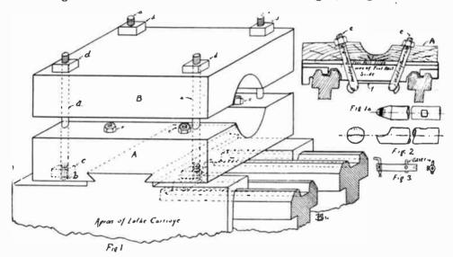
are screwed through the nuts c which are set into the wood flush with their face, to prevent their turning. As will be perceived these bolts in addition to holding down the clamp B, act to steady the whole attachment by giving a firm support at each corner and by reacting against the U bolts.
