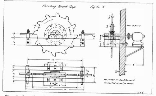
The wheel consists of a disc of  $\frac{1}{4}$  in. aluminum, the perimeter of which is divided into twelve equal parts. The diameter of the disc is 12 in. and the teeth are cut 1 in. deep. Each tooth is spaced 30 degrees from the next tooth, and is rounded off on one side and cut square on the other, thus allowing it to gradually approach the zinc electrodes and abruptly leave them. In the centre of the disc, a 4 in. hole is made, as shown by the dotted circle in the elevation in the drawing.
