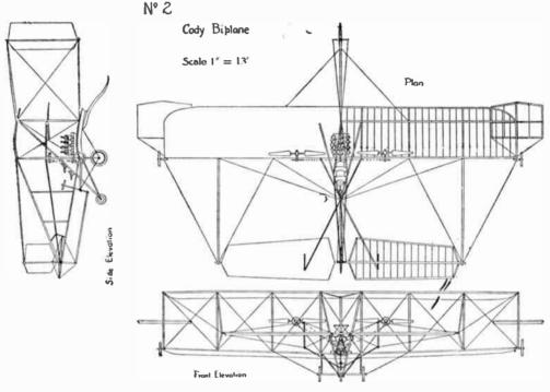
of the main cell. The lower seat is for the aviator, while the other was designed for the use of an observer in war time to take sketches of the enemy's position, etc. (*The Mounting* consists of a large pair of wheels, which carry most of the weight, a small wheel in front of them, and a skid in the rear. Wheels are also fixed on each end of the lower plane to carry the machine easily over the ground if it should alight on one end.
