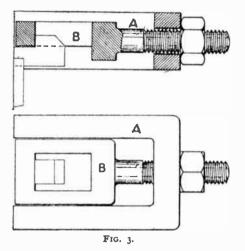
the key is to be drawn, and the slot hooked over the head of the key, it will be possible to extract by tightening on the nut with a spanner. There is only about an inch of draw allowed for, which should be ample to give the key a good start. If it is not easy enough to draw out by hand, after being pulled that distance, the nut may be eased back and some packing placed under the foot of the bridge.
