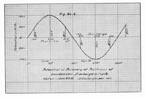
supply, the motor will vary accordingly, and the rotation of the spark gap will then be in proportion to the exciting potential of the transformer primary.
