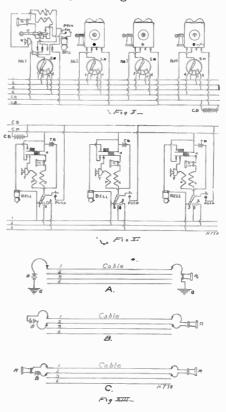
For regular telephone lines, No. 18 annunciator wire is generally employed for circuits not exceeding 600 ft. in length one way. For circuits longer than this No. 16 wire should be used.
