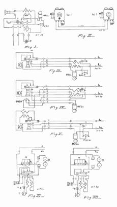
for a desk phone, and a flexible cable, of four wires, connecting it to a wall block, containing the induction coil, push button, call bell, battery and line terminals.
