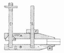
For heavy work the stud G is inserted in a seat that is counterbored in the under side of jaw B. This stud is re-movable, and its purpose is to support the tip ends of the clamps while drilling. These clamps may be applied in the manner above described in half the time the usual clamps require to adjust.
