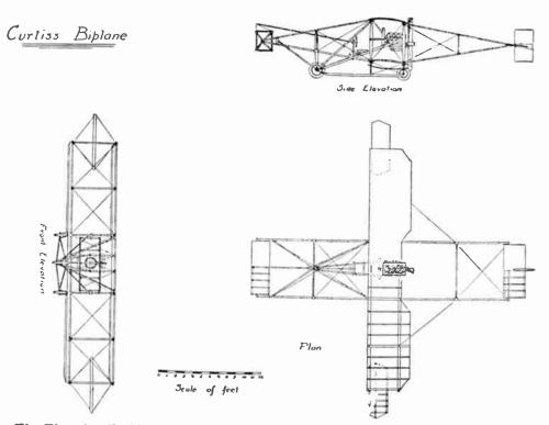
The Elevation Rudder.—The elevation rudder is a small biplane cell consisting of two identical surfaces, 24 sq. ft. in area, mounted at the front on bamboo outriggers. It is governed by a long bamboo rod attached to the stanchion on which the steering wheel is mounted. By pushing out on this, the rudder is turned down and the machine descends. By pulling in, the machine is caused to ascend.
