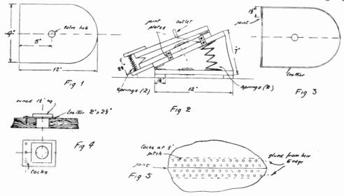
DETAILS OF CONSTRUCTION OF BELLOWS.
