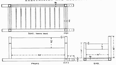
Bore the holes for the hanging staples as shown, the size of the hole depending upon the staples to be used.
