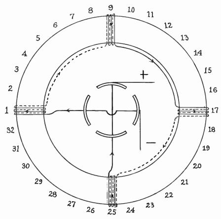
Fig. 6. Scheme of Winding a Ring Armature with Coils in Series for Use with Four-pole Field-magnet
