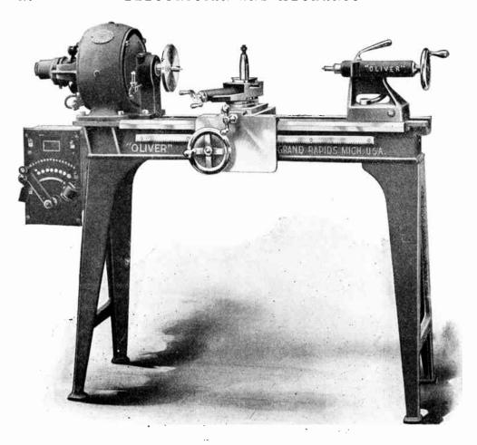
Fig. 2. Motor-head Speed Lathe
