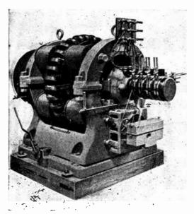
Fig. 7. Large Brush Arc Dynamo employing Winding shown in Fig. 6
