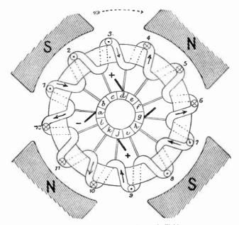
Fig. 4. Simple Ring Armature in Four-pole Field-magnet
