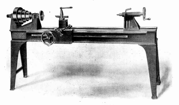
Fig. 3. Metal Bed Wood Lathe with Hand Feed Carriage
