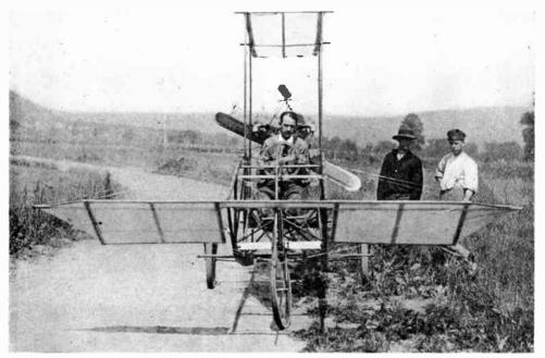
Showing Horizontal Rudder in Front and Propeller Blade in the Rear. G. H. Curtiss, Aviator
