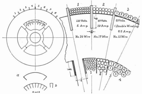
Fig. 8. Diagrams of Ring Windings for Small Dynamo
