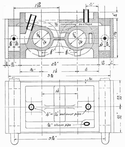
Fig 53.—Cross-section and Plan of Alternative Twin High-pressure Cylinders for Small Model Undertype Engine.
