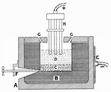
Fig. 128. Héroult's Furnace for Producing Aluminum
