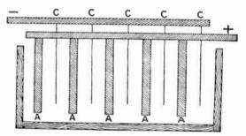
Fig. 126. Arrangement of Plates for Electrolytically Refining
