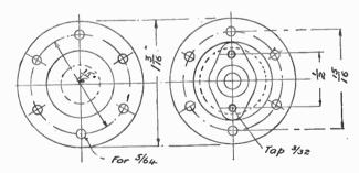
Fig. 55.—Covers for Twin High-speed Cylinders.
