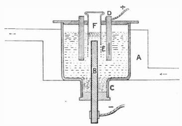
Fig. 132. Castner's Electrolytic Method of Producing Metallic Sodium
