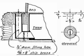
Fig. 57.—Filling Tube and Stopper for Water-tank. (Half full size.)
