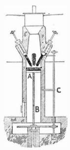
Fig. 130. Calcium Carbide Furnace for Operating with Three-phase Alternating Currents
