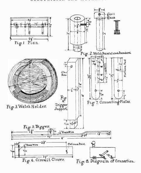
We next make the trigger support, Fig. 4. and glue it in the mortise we have previously made in the base. The wood part is now finished, and after thorough sand-papering, may be varnished.
