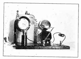
— the wire that is sealed in the end of the glass tube. Platinum is of a silver-white color, and so do not mistake the lead in copper wires of the glass tube for platinum wires, as they are very short and sealed in the glass, because the coefficient of expansion of the platinum is the same as that of glass. We use platinum at this point for the purpose of having a clean electric contact, as it does not corrode or oxidize under sparking as fast as other metals.
