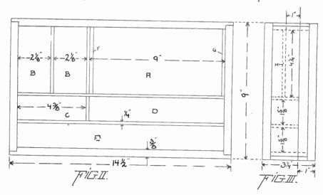
any special instruments outside of the case may be kept. As to the remaining spaces: B, B are for the reception of bottles of ink; C is for erasers, thumb tacks, etc.; D is for pencils, penholders, and brushes; and E is for scales. On the underside of the cover triangles may be fastened by means of small blocks of wood, screw-hooks, or screweyes.
