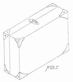
box is to be lined. Figure I gives a perspective view of the outside of the box as it should appear when finished, with the exception of the brass handle and padlock, these being left out for the sake of clearness.
