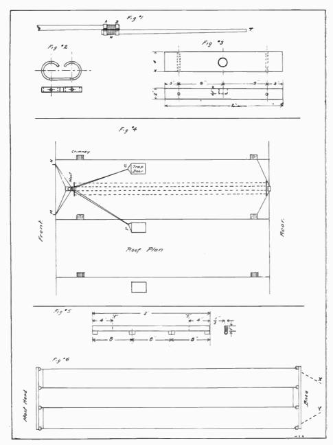
The mast having been erected, we will now turn our attention to the antenna. Get two pieces of well seasoned wood about  $1 \times \frac{1}{2}$  inch, and each 2 feet long. Fasten porcelain insulators to them, as shown in Fig. 5. These knobs can be tied to the wood with short pieces of wire running around groove on surface. The wood should then be given several coats of good paint.
