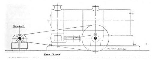
FIG. 1 Diagram Showing Engine Mounted on Baseboard and Connected to Drive a Small Dynamo
