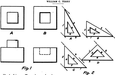
Shade Lines.—To make a drawing apparently stand out from the paper, shade lines are sometimes used. These indicate raised and depressed portions of an object. They are all of the same width and are about three times as wide as the original lines.
