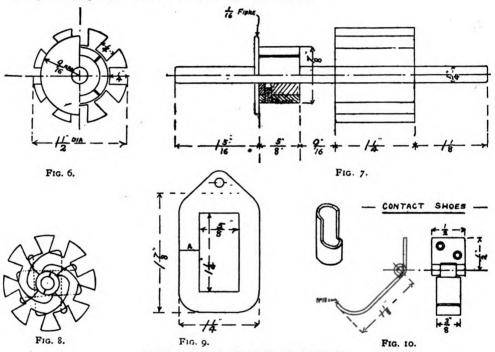
Details of Motor for Small Electric Locomotive
