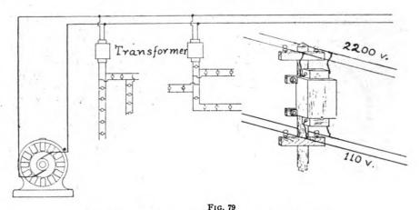
Transformer Alternating Current System for Multiple Circuits
