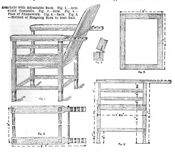
Generated on 2021-04-24 15:34 GMT / h<sup>-</sup> Public Domain, Google-digitized / htt<sub>l</sub> should have a shallow rebate to take the edge of the stuffing, showing ¾ in. on the bottom edge. The legs are mortised through the arms and wedged.
