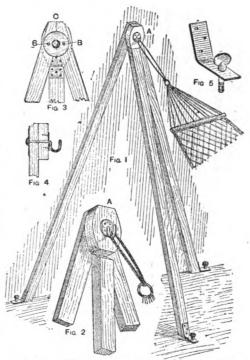
Support for Fixing Hammock in Room. Fig. 1.—View of Tripod Supporting One Ind of Net. Fig. 2.—Head of Tripod. Fig. 3.—Back of Head of Tripod. Fig. 4.—Vertical Section at C (Fig. 3) showing Shank of Hook riveted to Eack Plate. Fig. 5.—Bracket Iron and Thumbscrew.
