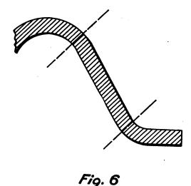
The edges to have shade lines may generally be determined by the eye; but if an edge away from the source of light is nearly in a 45 degree direction, the question of the shade line may be determined by placing a 45 degree tri-
