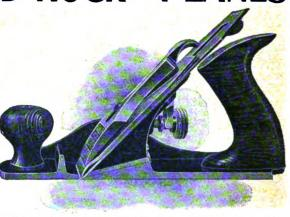
¶ In the "BED ROCK" plane we have perfected a design which allows a combination of the utmost solidity and rigidity, together with a wide range of adjustments.
