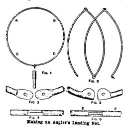
c 1 ft. 1½ in., and D 1 ft. ½ in. long. Both ends of A and B and one end of c and D should be hammered out and filed as shown in Fig. 3, and a shoulder set to half the thickness to make the joint come flush (see Fig. 4). The shoulders on the piece A are set both on one side, and on B on opposite sides. Then drill the holes for the rivet, which should be of iron wire. The wire for the rivet is now driven in, and should project slightly for riveting. The end c is hammered out 2 in. long and ½ in.
