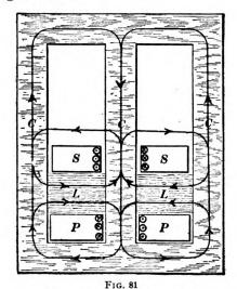
Magnetic Circuits of Constant-Current Transformer
