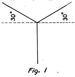
eye. This projection is used as a substitute for true perspective to save time and labor. Isometric drawing is based on the following fundamental
