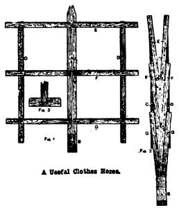
centre upright A can be pointed as shown, or cut flush at the top with C and D.—Work.
