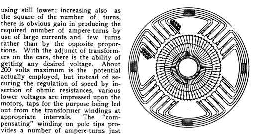
Fig. 74 Series-Wound Motor with Compensating Coils on Poletips. Railway Type
