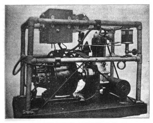
Portable Gasoline Engine and Generator for Field Wireless Telegraph
