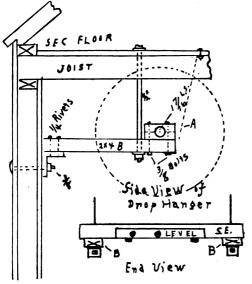
directly against the studding in the wall. If at any place you have a heavy pulley, put in a flat brace, A, which otherwise is not necessary.
