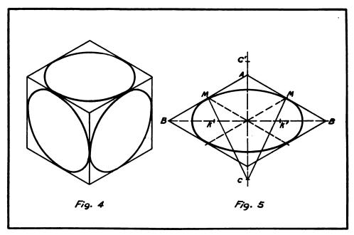
Right angles in the object are usually either 60 degrees or 120 degrees in the drawing. See Fig. 2.
