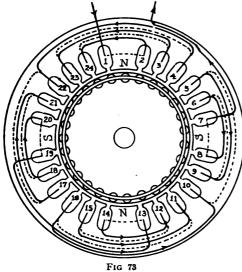
Diagram of Stator Winding for 4-pole Single-phase Motor, with Squirrel-Cage Rotor (not Self-starting)
