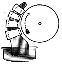
Short-circuited Coils on Pole Tips for Giving a Shifting Field Magnetism
