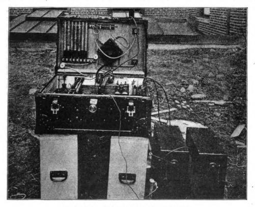
Portable Wireless Telegraph Apparatus for Field Service
