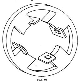
Single-Phase Fan Motor Field Magnet with Shading Coils on Pole Tips
