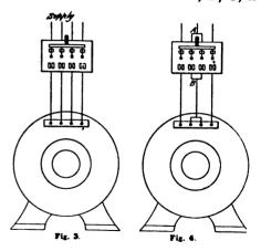
The wires A and B belong to one phase, and C and D to the other.
