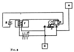
batteries will be needed to operate the apparatus, one set of five cells for the induction coil, and two sets of three cells each, one for the relay or coherer circuit, and the other for the local or sounder circuit.
