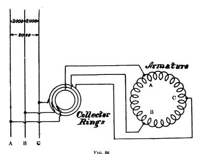
Connections for Three-Phase "Delta" (Mesh) Revolving Armature
