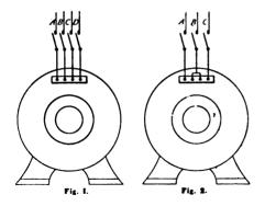
types exists entirely in the rotor, the stator being of the same construction in each case. In considering the stator connections, therefore — internal or external — any arrangement is applicable to either types. For reasons which will be duly given, however, the same starting arrangements in the stator circuit are not employed for both types.
