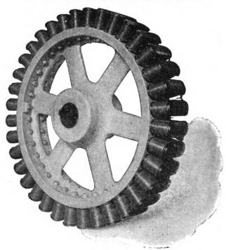
Revolving Field-Magnet (40 Poles) for Alternating Current Generator
