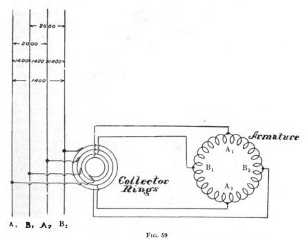
Connections for Two-Phase Closed-Circuit (Mesh) Revolving Armature
