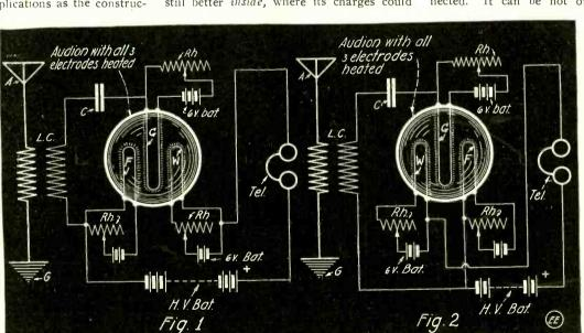
An Unusual Demonstration of the "Audion" as a Detector of Radio Currents as Given in Court by Dr. de Forest. All Three Filament Electrodes Were Heated; Figs. 1 and 2 Show How the Three Incandescent Electrodes Were Transposed in the Circuit; F Serving as "Filament," G the Grid and W the Wing.
