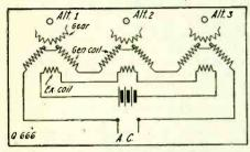
Connection of Three "Gear Type" High Frequency Alternators in Series with Battery Excited Fields.
