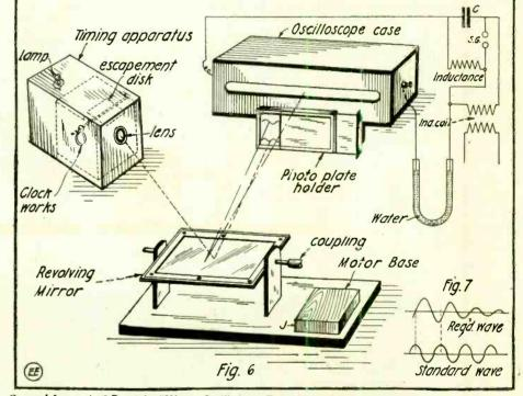
General Lay-out of Revolving Mirror, Oscilloscope Tube, Plate Holder, Spark Generator, and Timing Device Which Reflects a "Known Time Value" Curve on the Plate as Shown at Fig. 7.
