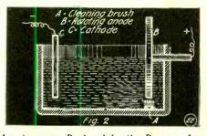
uminescence Produced by the Passage of an lectric Current Thru Sulfuric Acid—Another 'Cold Light'', Experiment which Can Be Made by Anyone.
