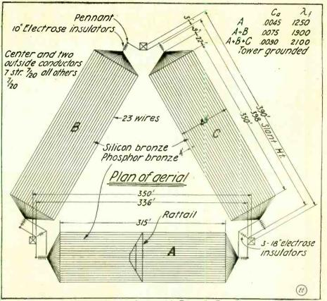
Plan View of the Main-Antenna Supported in Triangular Form Between the Three Masts at Arlington, with the Rat-tails Taken from the Middle of the 350 Ft. Central "T" Span. Fig. 5.
