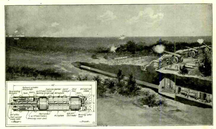
Sectional View of the Latest Advance in Military Science-the "Subterrane"-an Electrically Propelled Land Torpedo, and Its Mode of Attack. It Can Burrow for Miles and When Under the Enemy's Fort, a Press of the Button, and the Fort is No More.
