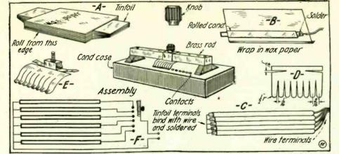
Details and Assembly of an Efficient, Adjustable, Fixed Condenser of the Multiple Switch Type. Can Be Made in Any Desired Size.
