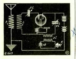
Hook-up for Using the "Audion" as a Radio-phone Generator and Transmitter.
