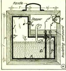
A Wet-Battery Portable Lamp Which Is Lighted by Placing the Case in the Position Shown. To Open the Lamp Circuit Turn it Over on Its Side.
