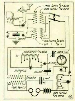
Details of Composite Audion Receiving Circuit Adapted to Long and Short Waves.
