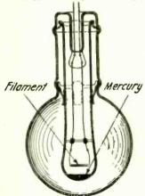
which is considerably above atmos-pheric pressure, allowing the car-bon filament to be worked at high current density. Mercury vapor is desirable for these lamps and is carried in a small cup as indi-cated. The gas filling may include some nitrogen or argon. Strong glass bulbs are specified, also a wire mesh glass, as a pro-tection against bursting of the chamber due to the high gas pres-sure.
