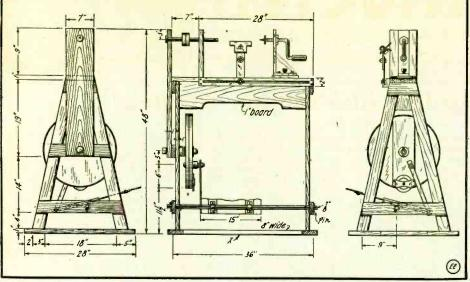
The Completed Lathe. It is Designed to Be Operated by Foot Power, but Can Be Readily Belted Up to a Motor or Engine. About ½ to ½ H. P. Will Drive It Nicely for Ordinary Work.
