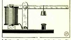
A Battery Gage that is Simplicity Itself. The Further Out the Weight Is, the Stronger the Battery Exchange the Magnet.
