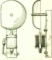
designed with an overhanging skirt on the head of the striker, so that no water can possibly enter the ar-mature chamber or that of the coil.
