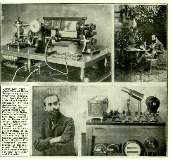
line to the receiving machine a certain strength of current. Moreover, the transmitting cylinder gradually moves past the sapphire point, being mounted on a threaded shaft. This accounts for the fine lines seen in the photos reproduced herewith. The process, however, takes but little time to perform the necessary steps in transmitting and recording a photo.
