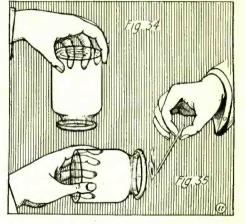
Bottles Filled with "Hydrogen" Should be Kept Inverted Owing to its Lightness and Tendency to Escape. Lower Figure-Experimenting with a Lighted Splint and "Hydrogen."
