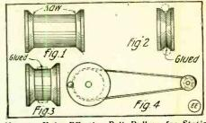
How to Make Effective Belt Pulleys for Static Machines from Common Thread Spools.
