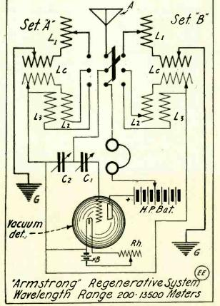
A Composite Regenerative Audion Receiving Hook-Up Adapted to Spark or Arc Signals at Wave Lengths of from 200 to 13,500 Meters. Requires Minimum of Apparatus and Has Been Tried Out Thoroly.
