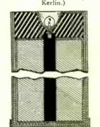
This invention is one of the most ingenious yet brought out. It in-volves the design of an extremely low-priced flashlight wherein the battery bulb and socket, as well as the switch are made up in the ordinary dry cell container. The reflector and socket elements are molded in the pitch filler at the top of the cell.
