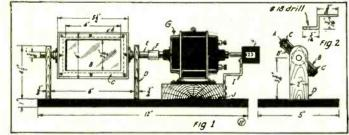
Working Drawing for Constructing Two-reflector Revolving Mirror Unit.
