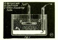
Experimental Production of "Cold Light" by Passing an Electric Current Thru a Potassium Bromid Solution.
