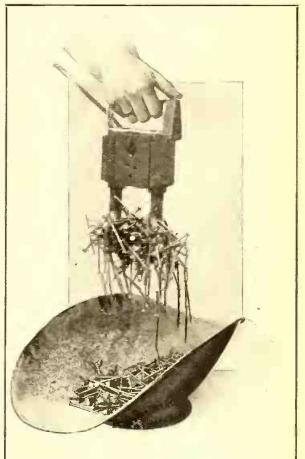
Useful Hand-Type Electro-Magnet for Lifting Nails, and Other Iron Pieces.
