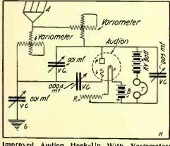
Improved Audion Hook-Up With Variometers for Sharp Tuning.
