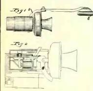
cause the switch springs, as per-ceived, to automatically control the cutting in and out of circuit of the telephone transmitter and receiver, instead of having to hang up the re-ceiver in the usual way. A very mod idea ceiver in good idea.
