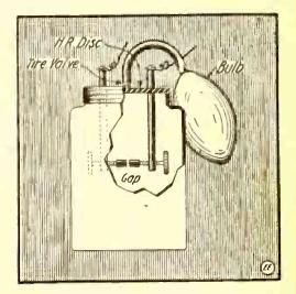
Fig. 2. Home-made Compressed Air Spark Gap.
