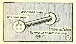
Fig. 2. Making Magnet Coil Spools.
