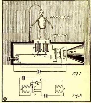
Fig. z. Diagram of "Dancing Doll" Apparatus Subject to Voice Control.
