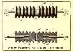
is inserted; the device may therefore be adjusted to tighten or loosen the wire without danger of shock even if one of the eye bolts is connected to a high-tension wire.
