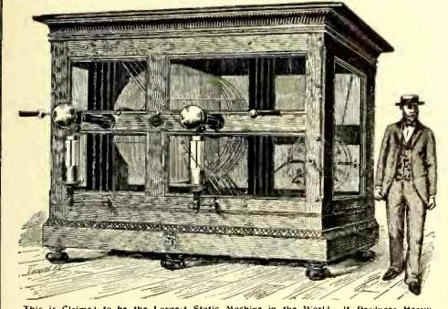
This is Claimed to be the Largest Static Machine in the World. It Produces Heavy 30-Inch Sparks.
