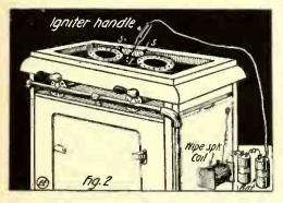
Fig. z. "Wipe" Spark Applied to Kitchen Gas Range.
