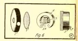
Fig. 6. Details of the "Watch-Case" Telephone Receiver.
