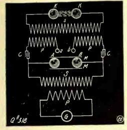
Imitating a Static Machine Spark with High Frequency Colls.
