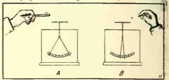
Fig. 2. Demonstrating How if Radium Is Brought Near Charged Electroscope (A) That It Will Be Discharged (B) Owing to Electronic Rays Shot Off by the Radium.
