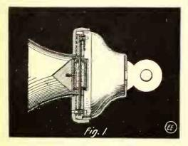
Fig. 1. Special 110 Volt Style Microphone Transmitter for Loud Talking Enunciator.
