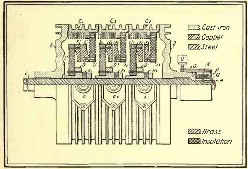
The Highly Efficient Rotary-Quenched Spark Gap (Hy-Tone) Produces 500 Cycle Tone Spark
