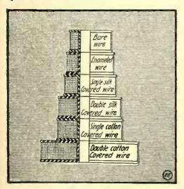
Showing Relative Volume of Various Kinds of Insulated Magnet Wire. Note Small Space Occupied by the Enameled Wire.
