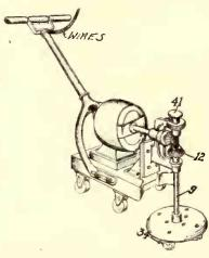
the polisher head to allow of its rising up and down as explained.
