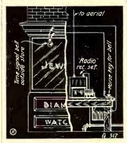
Electric Bell Signal for Radio Time Signals.
