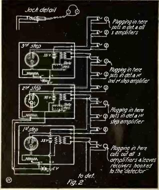
Fig. 2. Diagram of 3 Audion "Amplifier" Bulbs and 'Phone Jack Circuits.
