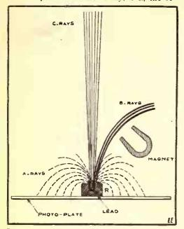
Fig. 1. Showing Effect of Magnet on the "Alpha" and "Beta" Rays.
