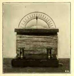
Photo of Complete Galvanometer. (Fou Being Used; Only Two Shown.) (Four Posts
