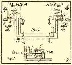
Ringing Circuits for Battery Telephones. Automatic Bell
