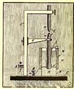
Construction of Simple Automatic Feed Lamp.
