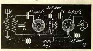
Fig. I. Double Audion "Detector" Hook-Up.
