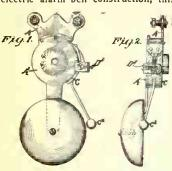
patentee arranges his bell very simply with a single magnet coil and the iron cheeks A and A<sup>1</sup> of the magnet bobbin attract the vibrating iron armature C, carrying the gong striker C<sup>2</sup>. The usual vibrator contact screw D<sup>3</sup> is placed outside of the bell, but the general design is indeed rugged and simplified.
