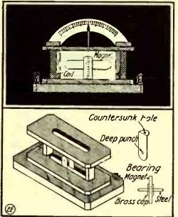
Assembly and Details of Sensitive Galvanometer.
