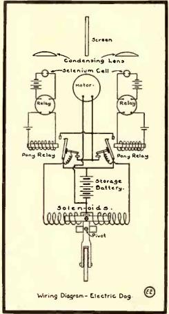
Diagram of Circuits Used in Electrically Controlled "Dog" Utilizing a Beam of Light and Two Selenlum Cells.
