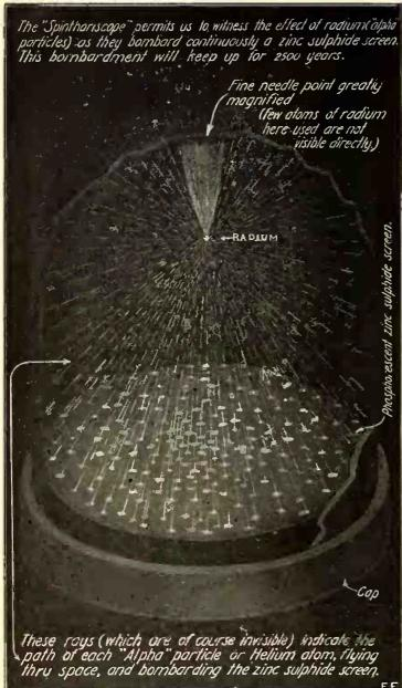
Fig. 11. Magnified Sectional View of Interior of Spinthariscope.
