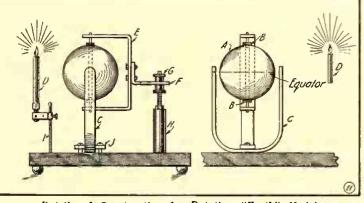
Details of Construction for Rotating "Earth" Model.
