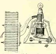
lamp is provided as well as special compact form of electro-magnetically operated bell. A single magnet coil attracts an iron armature 2 and this raises the striking hammer 37 in the bell. A spiral spring 43 helps to return the striking hammer.
