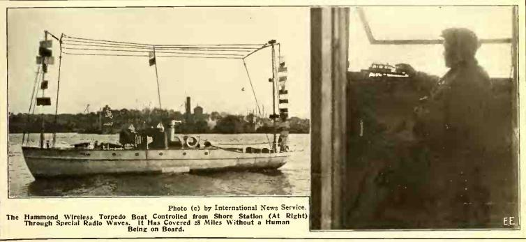
from time to time of the wonderful wire-less control effected by Mr. Hammond's invention, and we present herewith a photo of his latest torpedo boat, "The Natalia." The other photo shows Radio Operator Lee manipulating the wireless key at the Hammond laboratory on shore which controls the emission of wireless waves of various lengths, which when received by the radio antenna on board the automatic torpedo boat serve to make pos-
