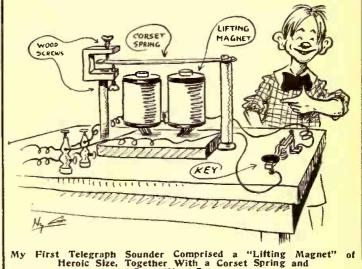
My First Telegraph Sounder Comprised a "Lifting Magnet" of Heroic Size, Together With a Corset Spring and Some Wood Screws.
