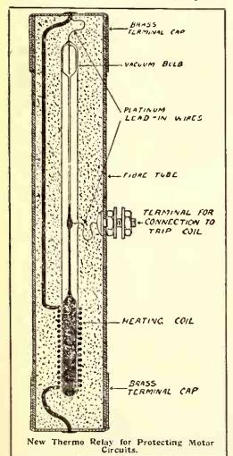
around the base of a glass tube, similar to a thermometer tube and which contains some mercury, then when a certain current passes through the circuit (and consequently
