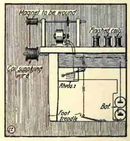
Simply Made Electric Winding Machine for Experimenters
