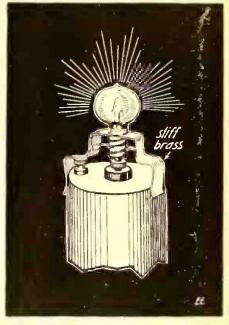
Simple Lamp Adapter for Dry Cells.
