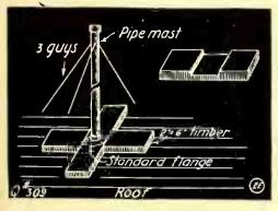
Mounting Iron Pipe Aerial Mast on Roof.
