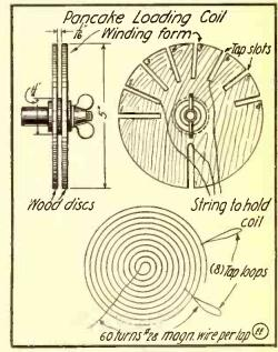
Details of Loading Coil for Loose Coupler Shown in Supplement.
