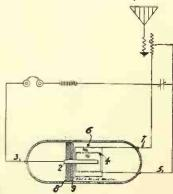
An electronic valve detector for wireless telegraphy, intended to utilize the electron radiations from some radio-active material, such as pitcb-blende, etc. As drawing shows, the wireless tuning circuits are hooked up by means of wires, 3, 5,
