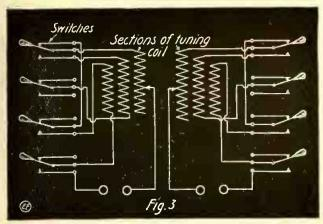
Fig. 3. Special Hook-Up of Loose-Coupler Windings to Prevent "Dead-Ends."
